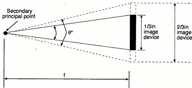
Fig. 2. Angle of view ( $\theta$ ) changes for different format size lens/image device.
