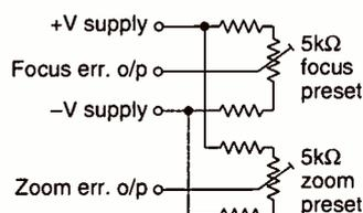
Fig. 11. Positional feedback from lens to control circuit enables a number of pre-set zoom (and associated focus) positions to be stored in memory. A similar arrangement would be used in the pan/tilt head to store in a 360° patrol area.
