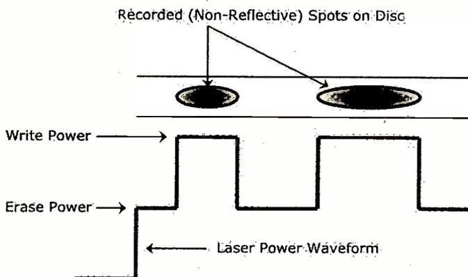
Fig. 2: The phase-change recording principle.
