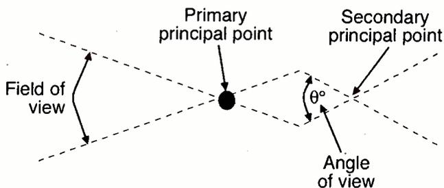
Fig. 3. Relationship between the angle view and the field of view.
