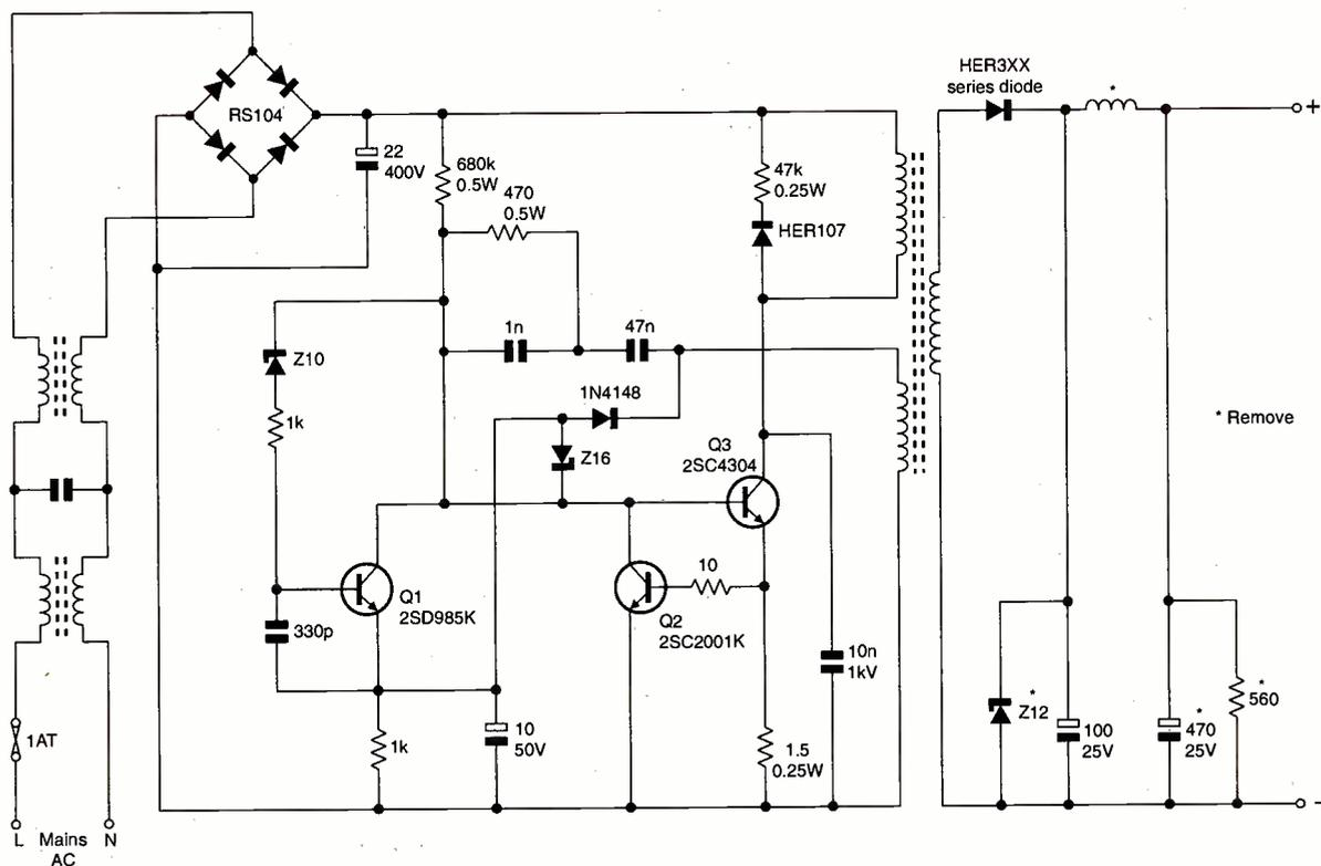
Fig. 1: Circuit diagram of the Olivetti LT7-700005-06 AC adaptor. This type of circuit is widely used in small PCs and AC adaptors.
