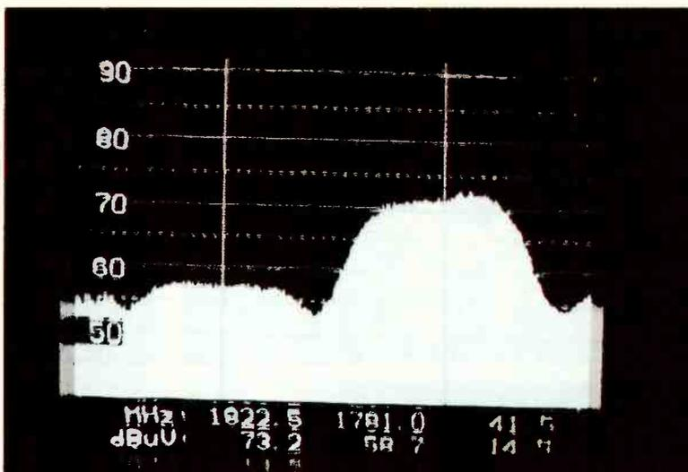
**Photo 3: Two digital carriers at approximately 1,781 and 1,822MHz. Marker A is on 1,781MHz, marker B on 1,822MHz. Signal levels are displayed on the bottom line. The last column shows the frequency and level differences between the two signals..**
