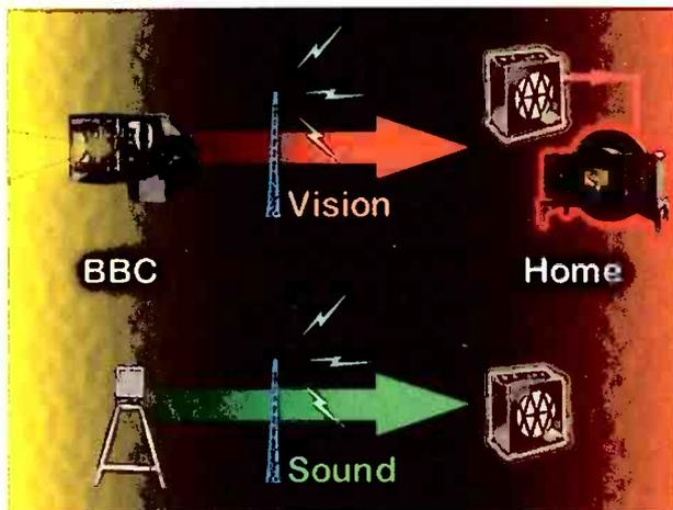
**Fig. 6. The BBC's first Television Service opened in 1932 with Baird's 30-line system, which was by then mature. With the vision signal so low in bandwidth that it could be treated like audio, the BBC Television Service only needed a camera in the studio, a spare medium-wave transmitter, an extra radio set in the home and a display adaptor – the Baird Televisor. The 30-line system's major benefit was that no new equipment or technology had to be developed.**
