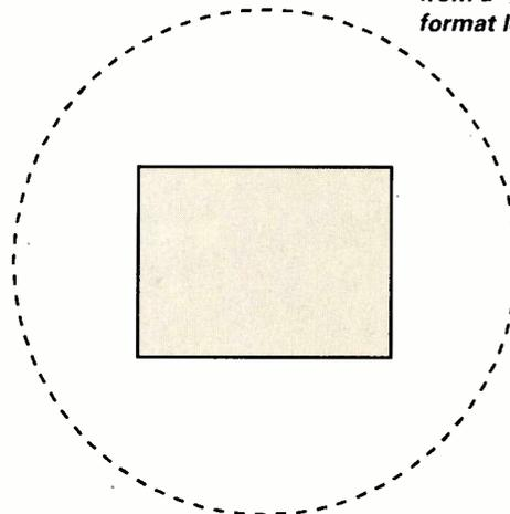
Fig. 5. Scale drawing showing the relative dimensions of a  $\frac{1}{2}$  inch format CCD against the circular image from a  $\frac{1}{2}$  inch format lens.
