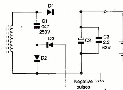
Fig. 3: Modifications to the secondary side of the switch-mode power supply to provide pulse charging.
