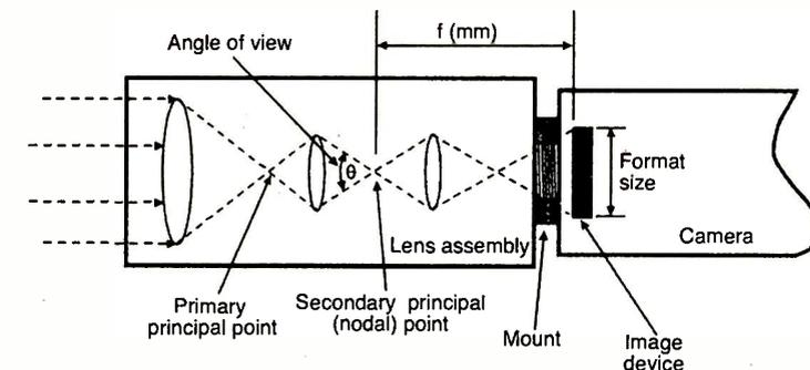
Fig. 1. Shows a simple fixed lens illustrating the main features of CCTV lens systems.
