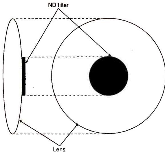
**Fig. 12. Principle of the neutral-density spot filter.**
