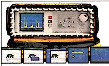
signal-strength meter, which is designed for use with both digital and analogue signals.
