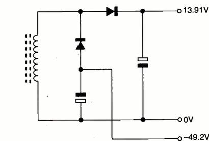
Fig. 2: Negative rectifier circuit added temporarily to measure the peak flyback voltage.
