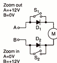
Fig. 10. Limit switch arrangement employed in zoom, focus and iris motor circuits. In telephoto mode, S<sub>1</sub> is open while in 'wide' mode, S<sub>2</sub> is open.
