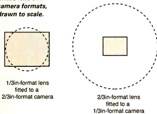
1/3in-format lens fitted to a 2/3in-format camera
