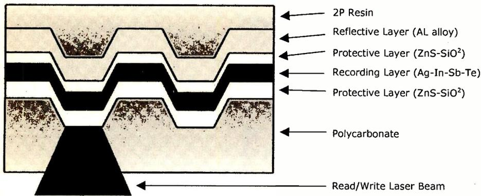
Fig. 1: Structure of a DVD-RW disc.
