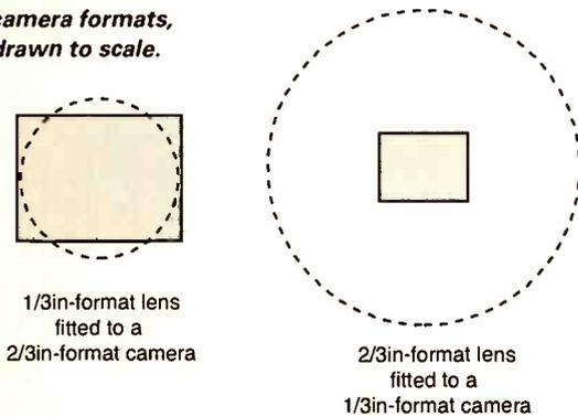
1/3in-format lens fitted to a 2/3in-format camera
