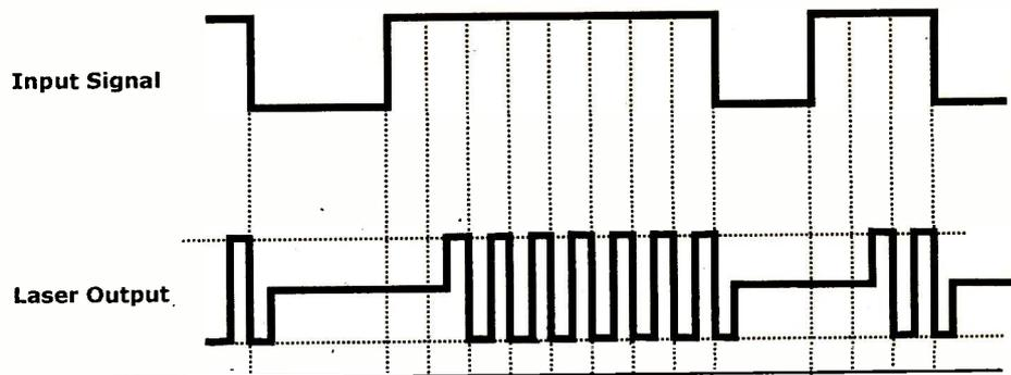
Fig. 3: Comparison between the input data signal and laser output for recording.
