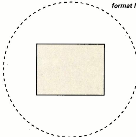
Fig. 5. Scale drawing showing the relative dimensions of a  $\frac{1}{2}$ in format CCD against the circular image from a  $\frac{1}{2}$ in format lens.
