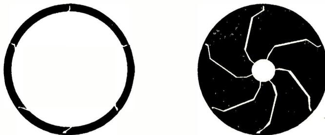
Fig. 4. Sliding plates perform the function of a mechanical iris.
