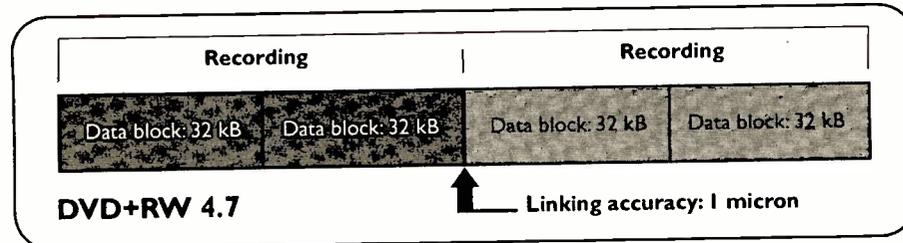
Fig. 6: Lossy and lossless linking.
