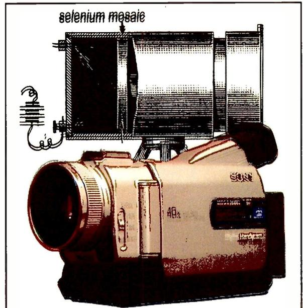
*Fig. 3. Ayrton & Perry in the UK and Carey in the USA proposed imaging systems using arrays of selenium photocells. Although 120 years of technological development separate today's digital camcorder from Carey's 1880 scheme, they both employ the same principle of using imaging arrays for the camera.*
