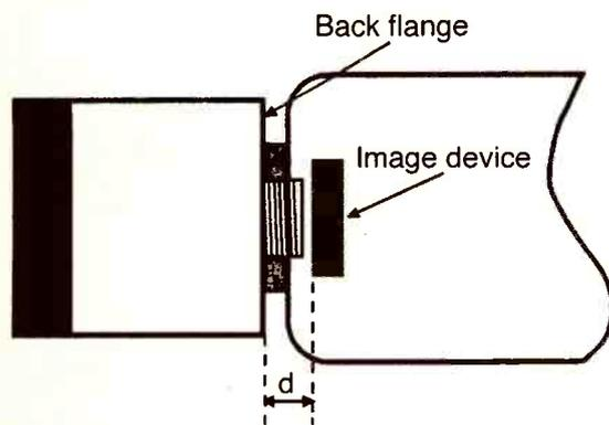
**Fig. 7. For a C mount, d is 17.5mm while for a CS mount, d is 12.5mm.**
