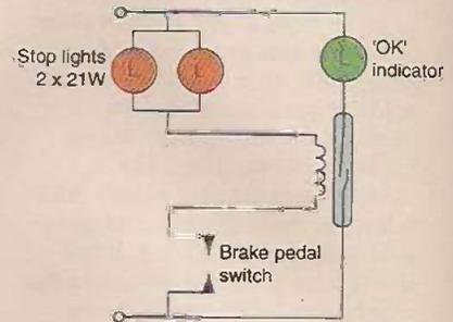
**Fig. 8. This simple application of a reed switch gives the driver of a car an indication of whether or not his or her brake lights are working.**
