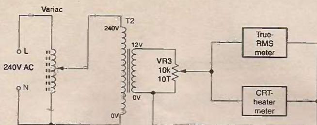
Fig. 2: Calibration set-up.
