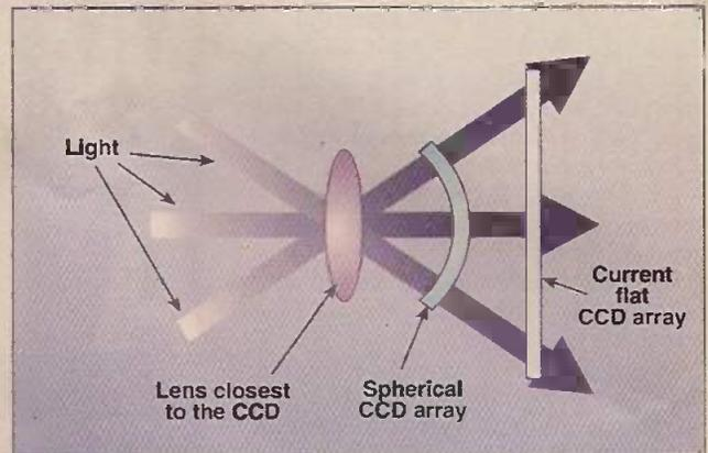
A spherical CCD photosensor enables the lens system to be greatly simplified.
