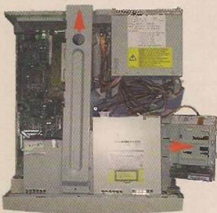
Photo 1. The PowerMac 4400. Arrows show the initial stage of dismantling.
