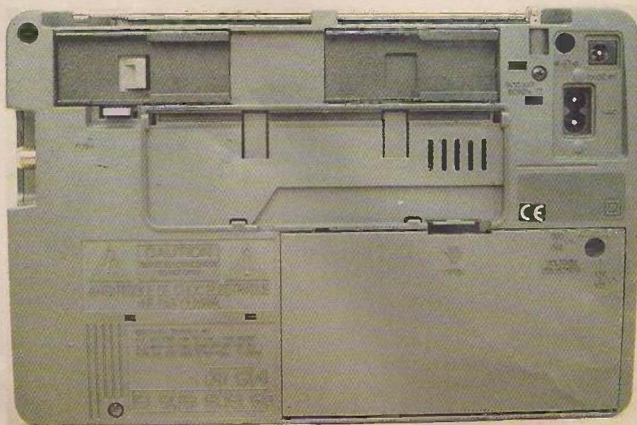
Photo 6: Rear view of the Hitachi Model KH-WS1. The mains and 6V DC input sockets are at the top right. The mains voltage adjustment is in the hole at the top, right-hand side of the battery compartment cover. The frame aerial slide/clip-in fixing lies horizontally along the top of the receiver, just below the telescopic aerial. The F input socket can be seen at the left-hand side.
