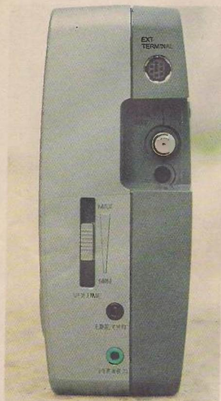
*Photo 4: Side view of the Hitachi Model KH-WS1, showing the slider volume control, the line and headphone output jack sockets (bottom), the F input socket for the L-band aerial and the data socket (top).*
