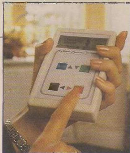
*Each power outlet in the JR Smart home can be controlled in several ways. This photo shows remote-control operation, which enables the user to send commands to any networked equipment via the power outlet.*
