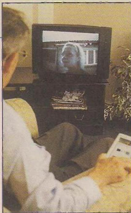
*Door-entry monitoring is a basic feature of the JR Smart home. The TV set automatically switches to display the input from a monitoring camera. There is provision for verbal communication, and in addition the security system can activate lights.*
