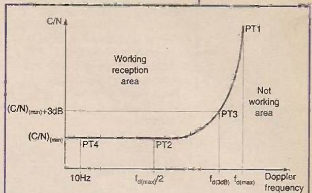
Fig. 1. Key response of carrier versus noise with doppler frequency, which can be used to define the limits of mobile reception.
