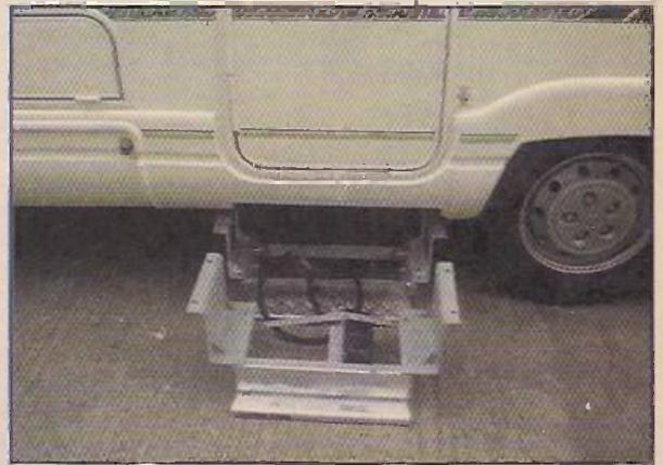
*The original and new steps shown beneath the door to the motor home.*
