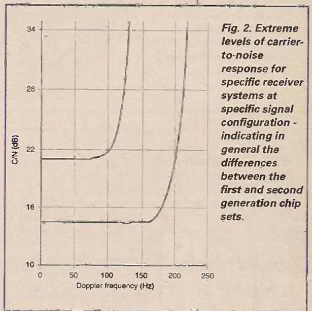
Fig. 2. Extreme levels of carrier-to-noise response for specific receiver systems at specific signal configuration - indicating in general the differences between the first and second generation chip sets.
