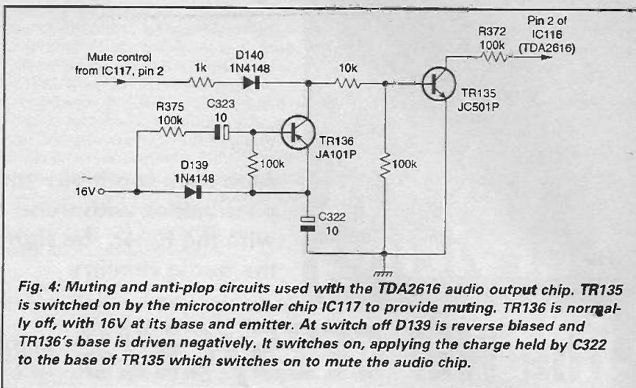
Fig. 4: Muting and anti-plop circuits used with the TDA2616 audio output chip. TR135 is switched on by the microcontroller chip IC117 to provide muting. TR136 is normally off, with 16V at its base and emitter. At switch off D139 is reverse biased and TR136's base is driven negatively. It switches on, applying the charge held by C322 to the base of TR135 which switches on to mute the audio chip.
