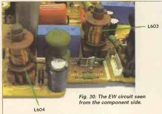
Fig. 30: The EW circuit seen from the component side.
