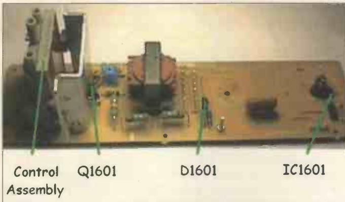
Fig. 26: Photo of the FW focus-modulator PCB.
