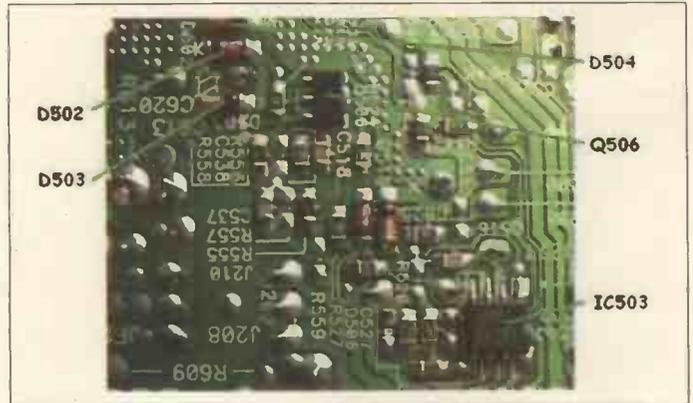
Fig. 29: The EW circuit seen from the print side.
