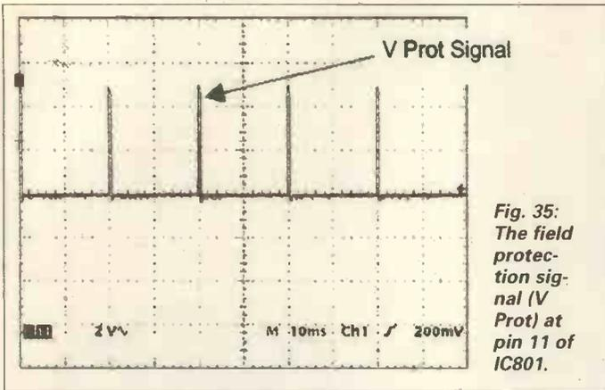
Fig. 35: The field protection signal (V Prot) at pin 11 of IC801.
