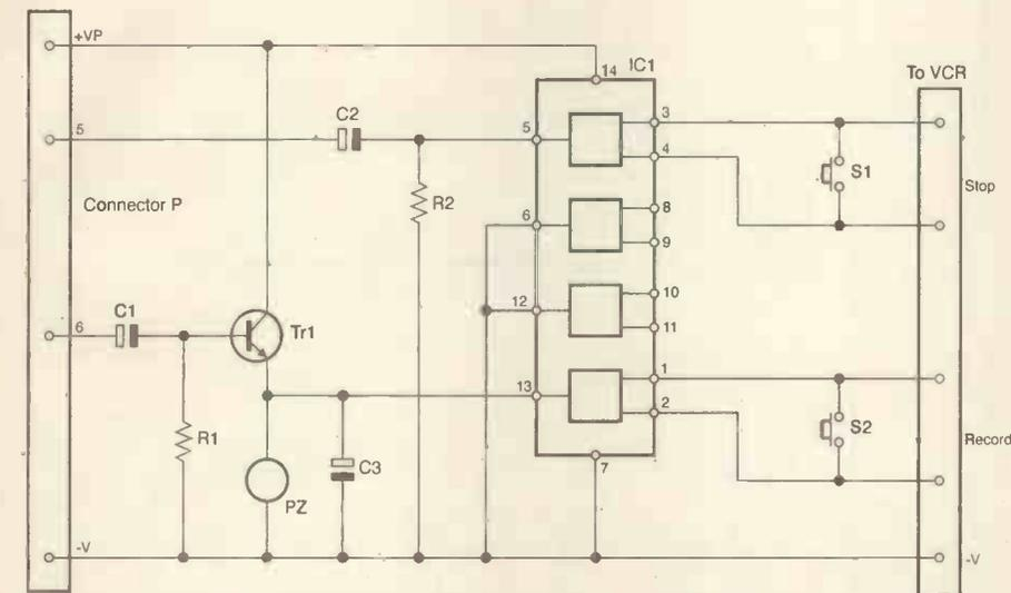
Fig. 9: The VCR control and audio alarm circuit.
