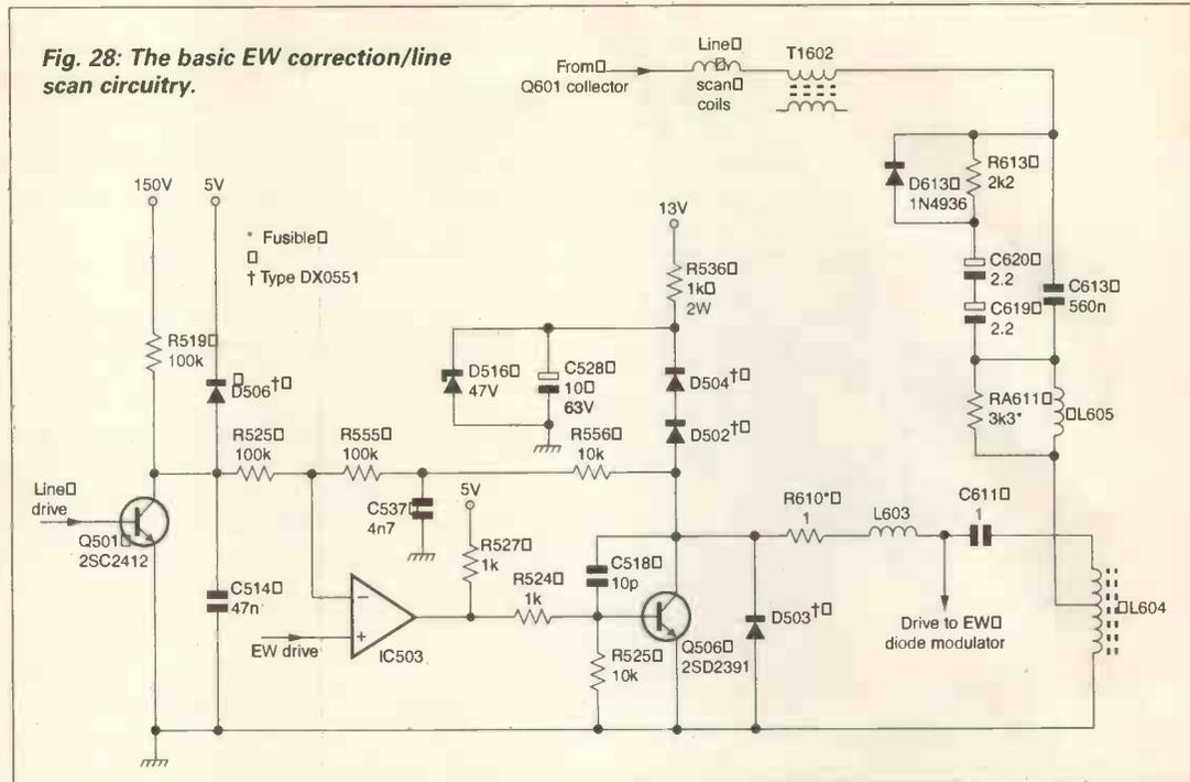
Fig. 28: The basic EW correction/line scan circuitry.
