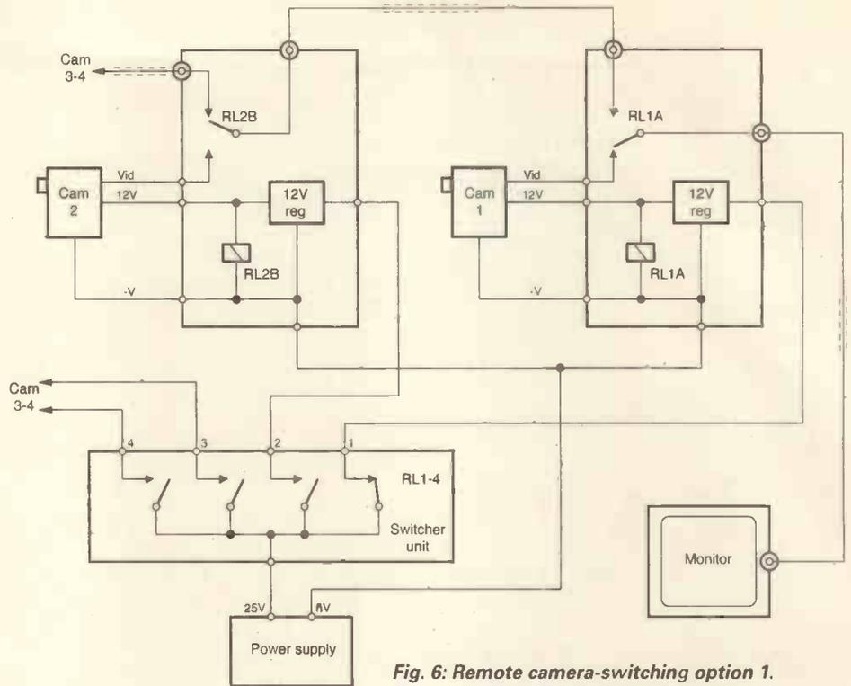
Fig. 6: Remote camera-switching option 1.
