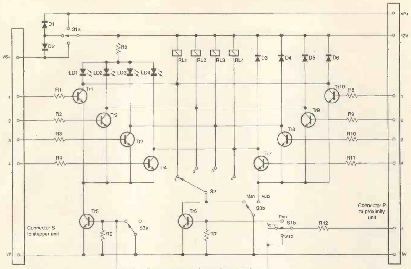
Fig. 4: The switcher unit circuit.
