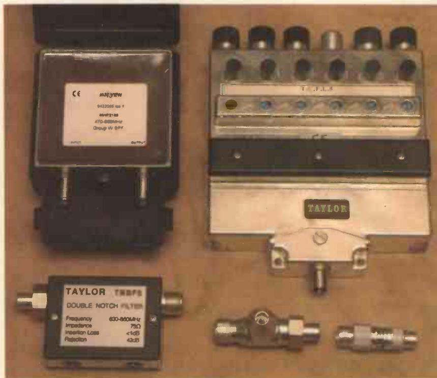
Photo 2: Various types of filter. Clockwise from the top left bandpass, channel-pass/leveller, high-pass, single-notch and double-notch.
