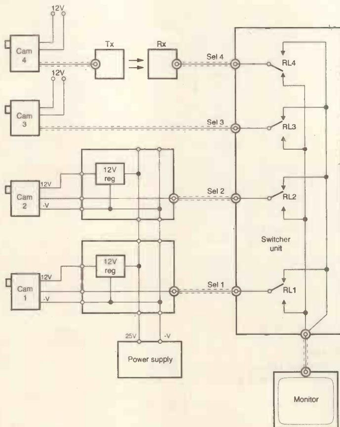
Fig. 5: Video switching with a four-camera system.
