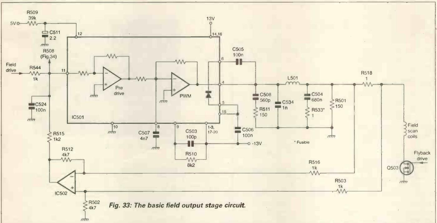
Fig. 33: The basic field output stage circuit.
