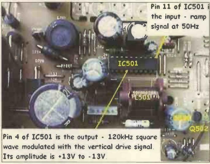
Fig. 36: The field output stage, component side of the PCB.
