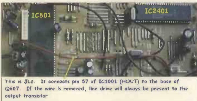
This is JL2. It connects pin 57 of IC1001 (HOUT) to the base of Q607. If the wire is removed, line drive will always be present to the output transistor
