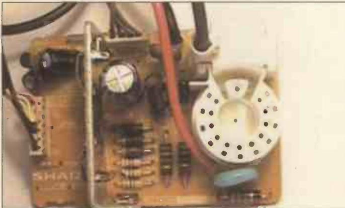
Fig. 32: The CRT PCB used in Model 56FW53H.
