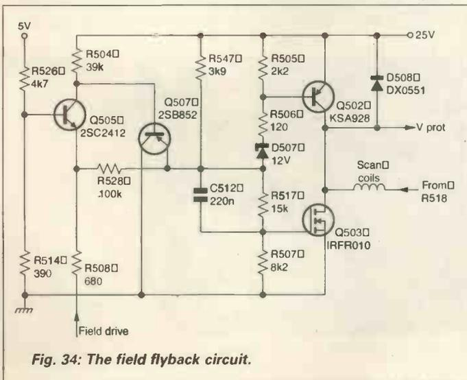
Fig. 34: The field flyback circuit.
