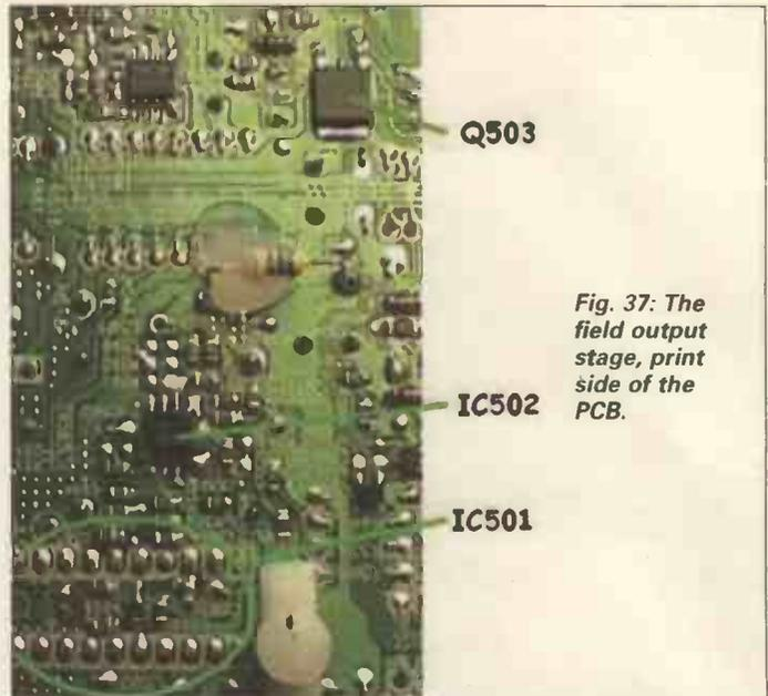
Fig. 37: The field output stage, print side of the PCB.
