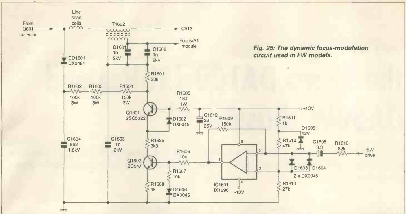
Fig. 25: The dynamic focus-modulation circuit used in FW models.
