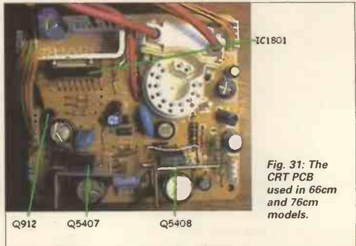
Fig. 31: The CRT PCB used in 66cm and 76cm models.
