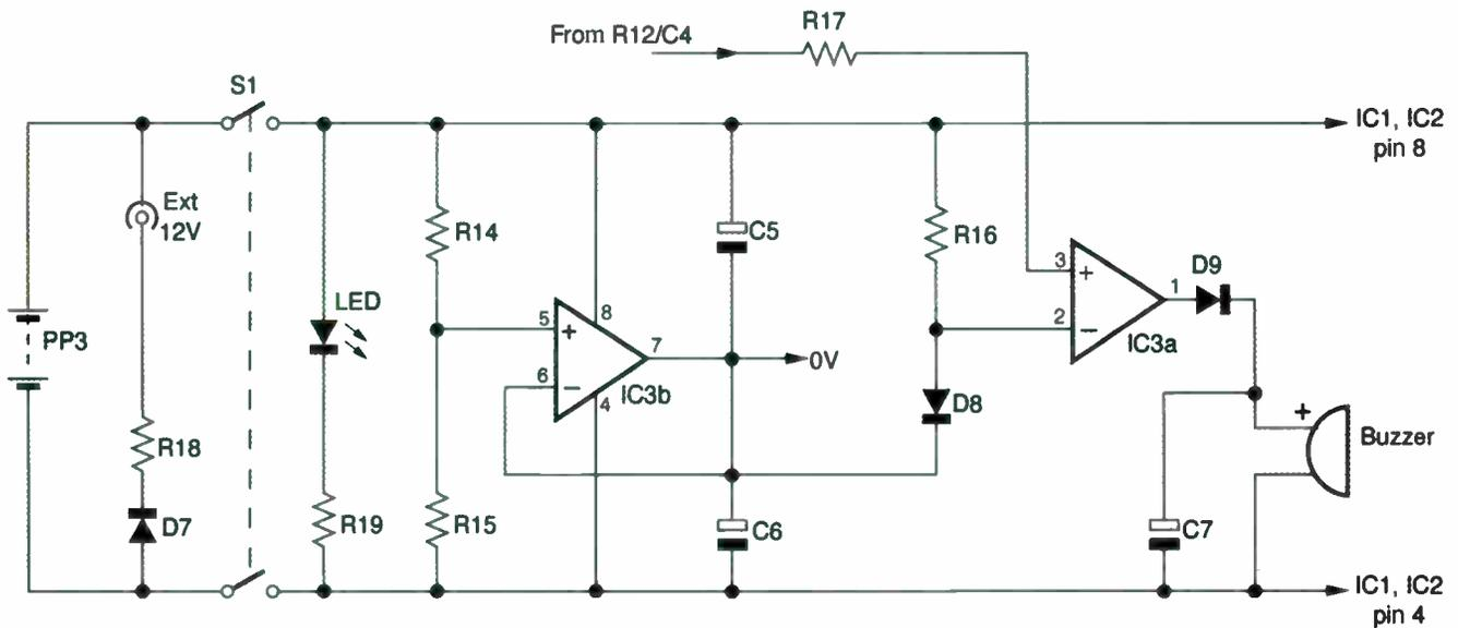
goes high, activating the buzzer. The ESR level at which the buzzer operates is set by the overall gain. This point can easily be changed by altering the value of R12. If its value is increased, the overall gain rises and the buzzer will operate at a higher ESR level.
