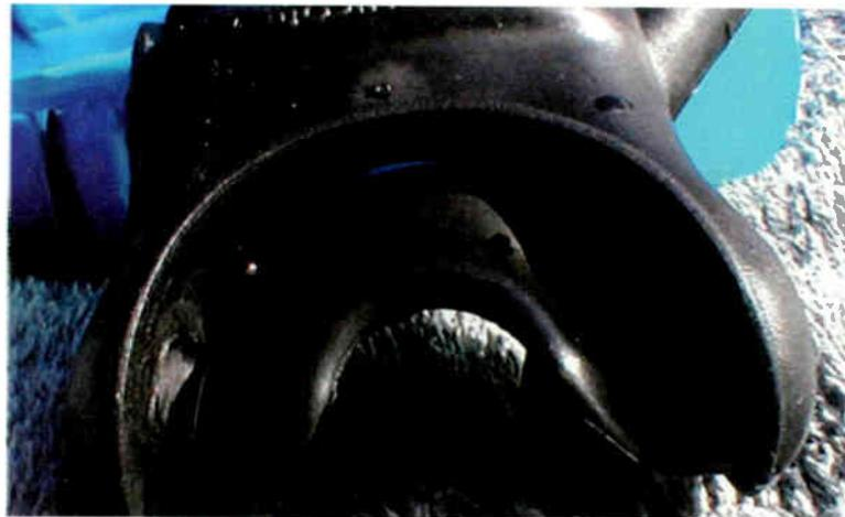
*Photo 1 (top): Close-up view of the mouthpiece. The odd 'leg' on the right-hand side is the electrical connection to the radio circuitry.*
