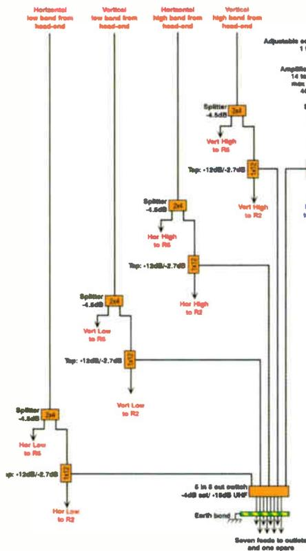
Fig. 31: A tap-off, multiswitch and amplifier combination. This is tap unit four in Fig. 26.
