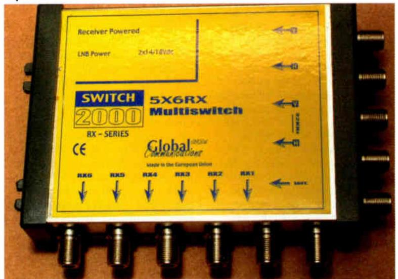
Fig. 34: The Global 5X6RX passive multiswitch.
