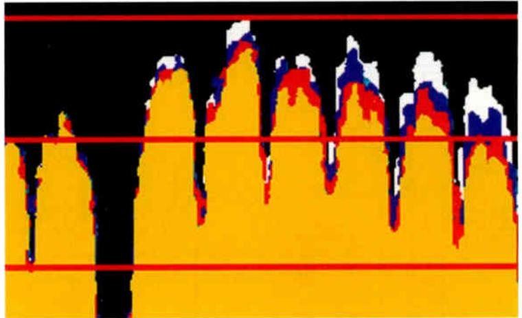
Fig. 32: An analyser display of one of the high-band polarisations. The whole satellite IF band is shown, with the low frequencies on the left. The horizontal red lines are 5dB divisions. The white, blue, red and yellow areas represent the response after 20, 40, 60 and 80m of CT100 cable respectively. The blue, red and yellow areas have been moved upwards, so that the response of the lowest multiplex is equalised. This highlights the extra signal loss at the higher frequencies.
