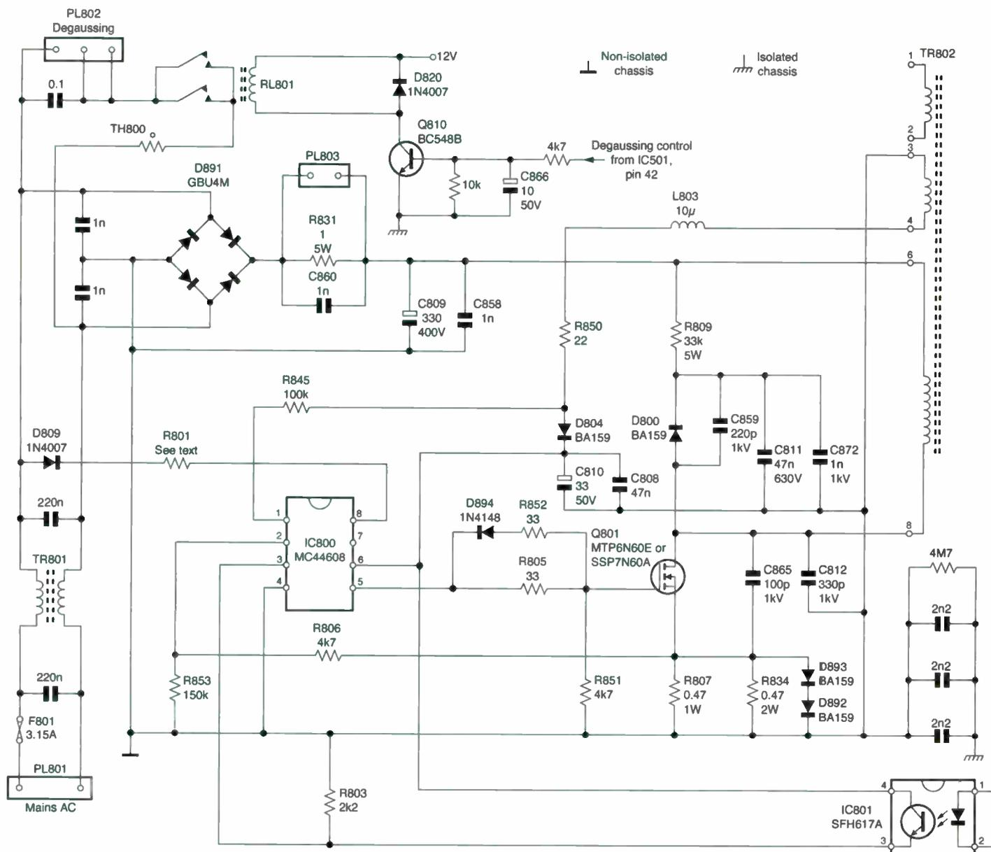
Fig. 1: Circuitry on the primary side of the chopper power supply in the Vestal 11AK37 chassis.
