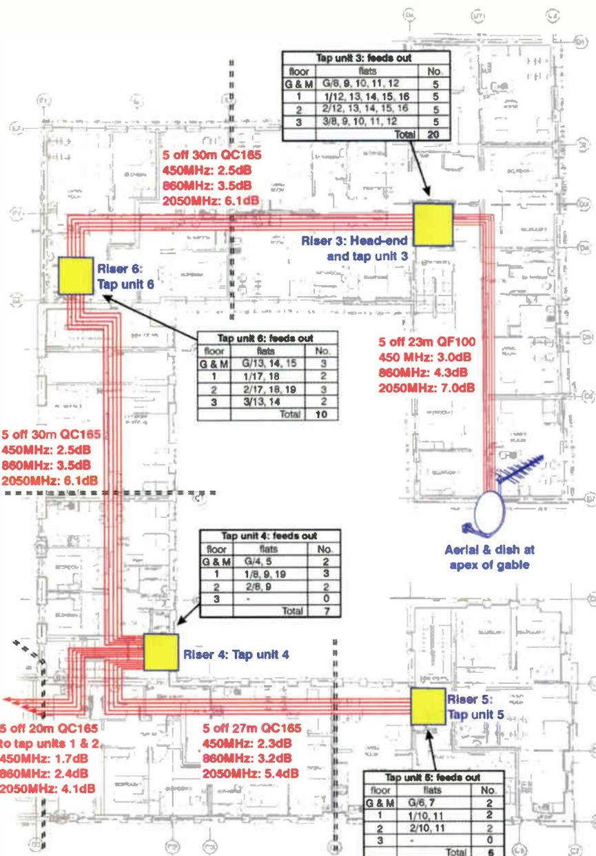
**Fig. 26:** Schematic of part of a system based on tap-off lines.
