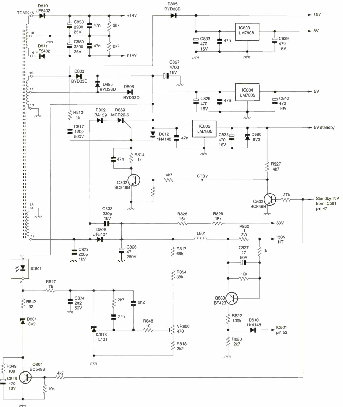
Fig. 2: Circuitry on the secondary side of the chopper power supply in the Vestel 11AK37 chassis.
