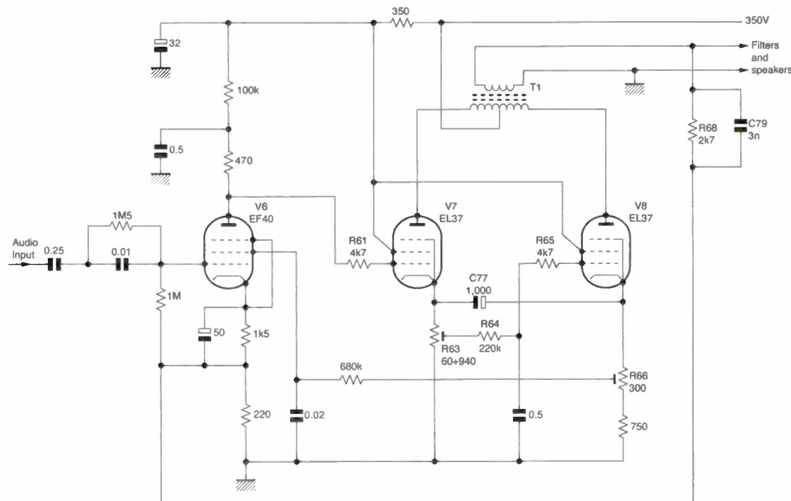
Fig. 1: The push-pull audio output stage in the Ferguson Model 500RG used cathode coupling.
