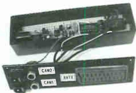
path can be used to provide switching between cameras. Ian Rees describes a relay-operated switcher that implements this option for a two-camera system.
