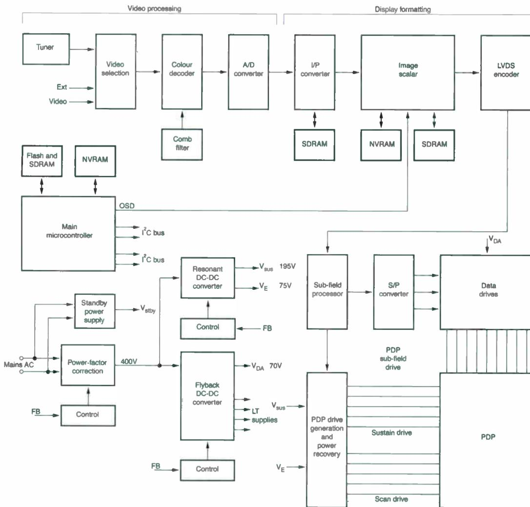
**Fig. 1: Basic sections of a plasma TV receiver.**
