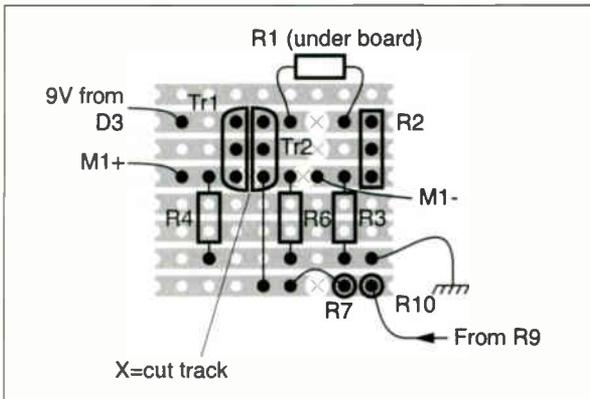
**Fig. 5: Layout of the meter board. R8, R9 and C3 are connected in free space off the board.**
