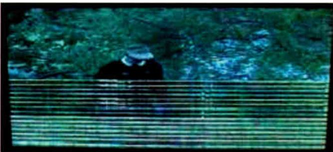
**Fig. 13: Effect produced by a dry-joint at the sub-field processor.**
