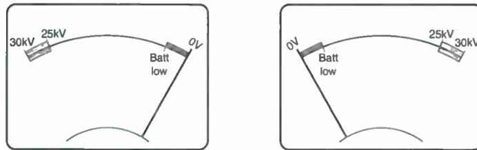
**Fig. 2:** Alternative meter scales. 25kV-30kV LOPT OK, otherwise LOPT faulty.
