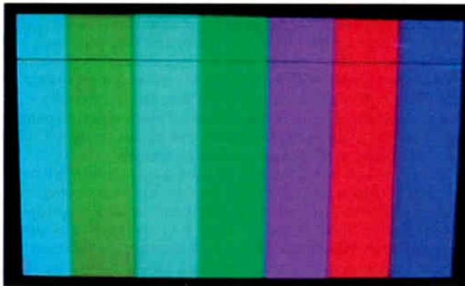
**Fig. 2: A single horizontal black line indicates a scan- or sustain-drive fault.**
