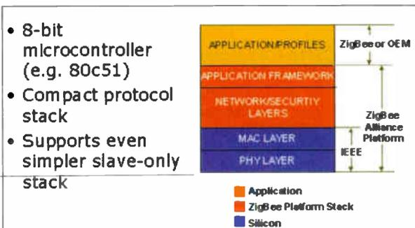
Fig. 2: The ZigBee protocol stack.
