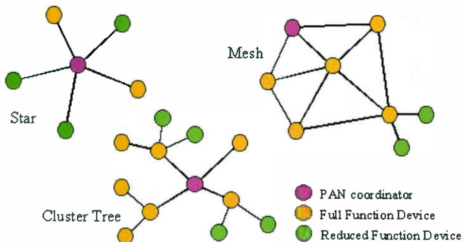
Fig. 3: How function varies depending on where a device is within the network and the network arrangement.
