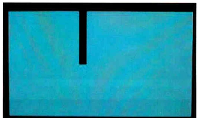
**Fig. 4: Vertical segment down the top half of a display. This indicates a data-drive fault with a dual-scan display.**
