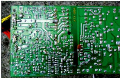
Left – Photo 2: Underside view of a typical ATX power-supply PCB, showing the clear demarcation between the primary and secondary sides of the circuitry.
