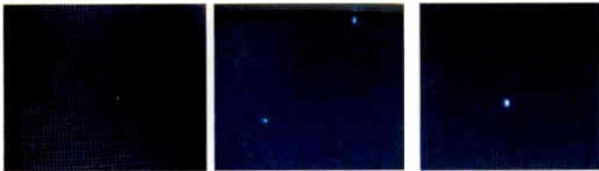
**Fig. 5:** (left) Central area pixel failure. **Fig. 6:** (centre) Several pixel defects. **Fig. 7:** (right) Pixel cluster failure.
