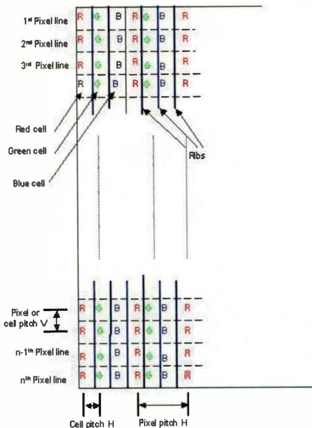
**Fig. 15: Cell and pixel pitch.**
