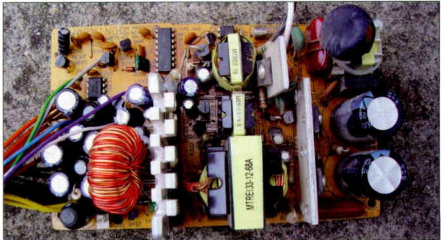
Photo 1: Top view of a typical ATX power-supply.
