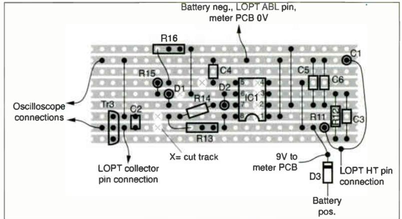
**Fig. 6: Layout of the main board.**
