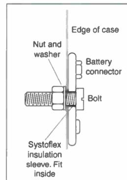
**Fig. 4:** Method of fitting the battery connector to the case.
