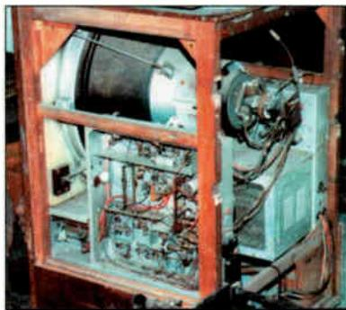
**Photo 6: An experimental Murphy PAL/NTSC colour receiver that was produced in 1959.**
