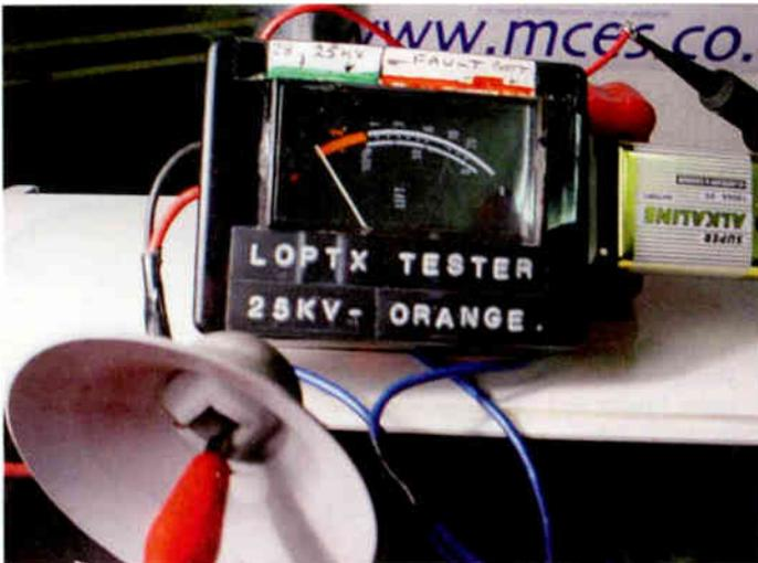
**Commercial LOPT testers cost about £90. This simple, easy-to-use tester, designed by Paul Coles, can be built for a fraction of that cost**
