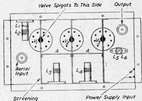
Fig. 3.—Layout of the main components—underside view.
