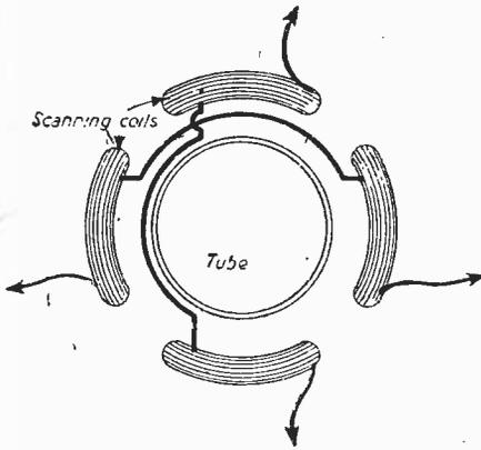
Fig. 10.—Arrangement of the scanning coils around the dissector tube.
