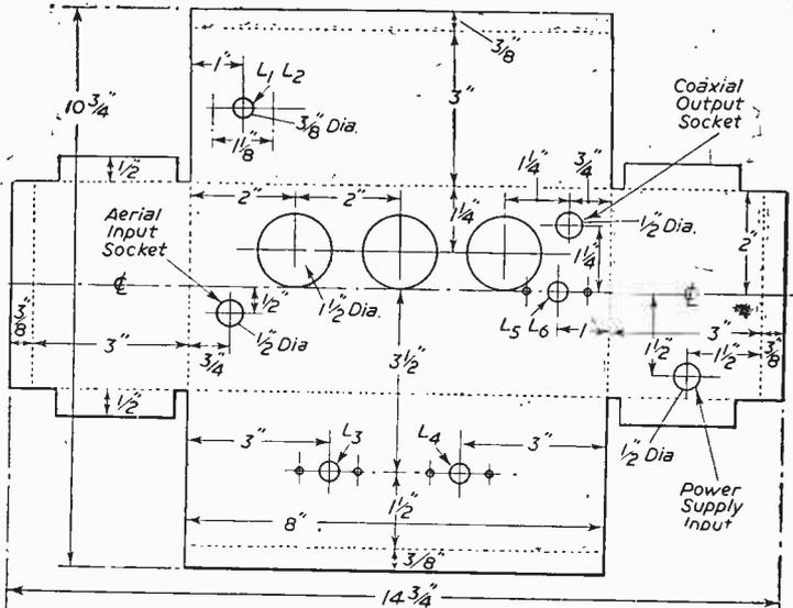
6BA Clearance Holes Drilled in All Flanges To Fasten Chassis Ends and Base Plate. Dimensions Of Coil Former Mounting Holes Are All As For L<sub>1</sub> L<sub>2</sub>. - Base Plate Size 4 3/4" x 8 3/4" Also Required.
