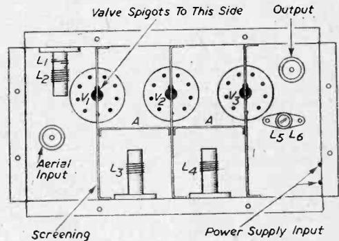
Fig. 3.—Layout of the main components—underside view.
