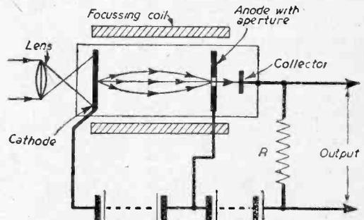
Fig. 9.—Diagram showing the principle of the image dissector.
