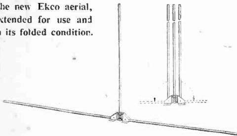
electric conduit, etc. It is permissible to tilt the aerial array where insufficient head-room is available. As an alternative the aerial may be suspended, and in extreme cases a further assembly may be positioned to act as a reflector. The down-lead should, of course, be taken in the most direct manner to the receiver. It is claimed that the aerial gives satisfactory reception within 15 to 20 miles of a transmitter. The price is 25s. (no Purchase Tax).
