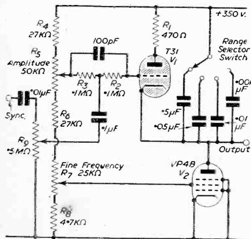
Fig. 6.—A thyratron time-base with linearising pentode.
