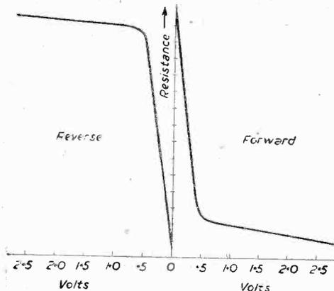
Fig. 1.—Rectifier characteristics.
