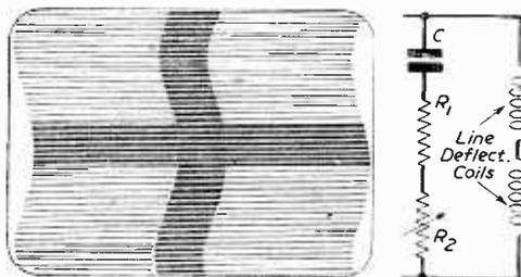
Fig. 2.—On the left is the effect produced by hum in the time-base circuits. On the right is the line-deflection coil and a common form of linearity or form control. Either R1 or R2 or both may be variable, and in some cases C also is variable.
