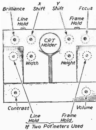
Fig. 6.—Front view of upper chassis and general layout.
