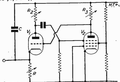
Fig. 7.—The basic circuit of the Puckle time-base.
