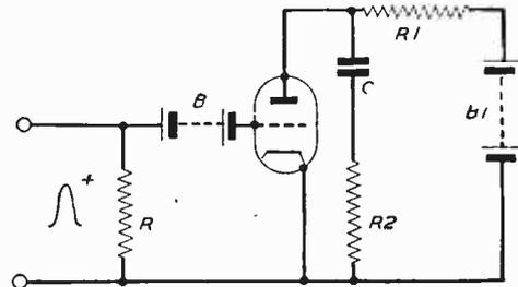
Fig. 22.—Circuit suitable for producing a voltage waveform of the shape shown in Fig. 18(c).
