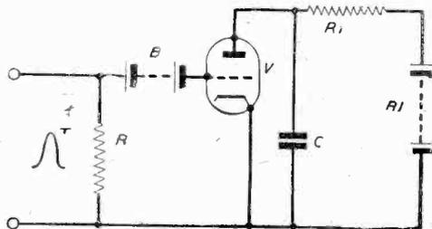
Fig. 19.—Circuit of a simple saw-tooth generator, triggered by a positive sync. pulse.
