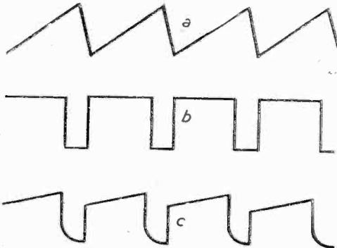
Fig. 18.—Voltage waveforms which must be applied to (a) resistance only ; (b) inductance only, and (c) resistance and inductance, in order to produce a pure saw-tooth current waveform.
