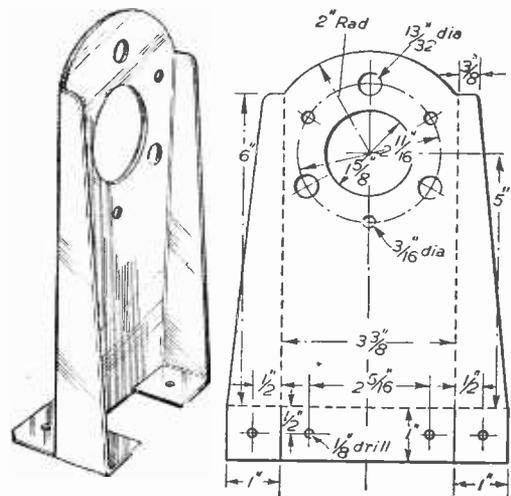
Fig. 5.—Support for the permanent magnet focusing unit.
