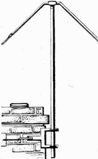
Type 4 (left).—Inverted "V" which is also suitable for use in a loft.
