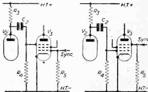
Fig. 3, (left) and Fig. 4 (right).—Two alternative circuits for introduction of the sync pulse.
