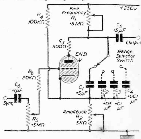
Fig. 5.—A practical thyatron time-base giving a frequency coverage of 25 c.p.s. to 25,000 c.p.s.
