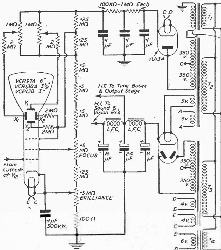
Fig. 7.—Tube and power supply. If the tube will not focus, remove or add one .5 MΩ resistor in the Brill./Focus resistor chain.
