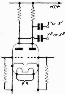
Fig. 3.—Push-pull operation of the X and Y plates of an electrostatic tube depends for good linearity on exact balancing of the characteristics of the push-pull valve or valves.
