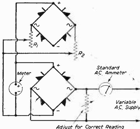
Fig. 5.—Circuit for calibration as an A.C. ammeter.
