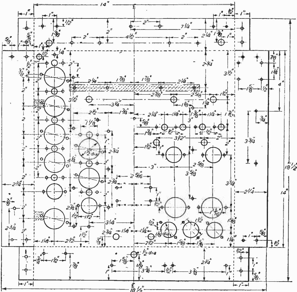
Fig. 2.—Main chassis details. The unmarked holes are either  $\frac{1}{8}$  in. or  $\frac{3}{8}$  in. in diameter and suit grommets, variable controls, and clearance for 6 BA bolts.
