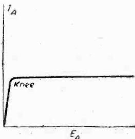
Fig. 2.—Anode current characteristic of a pentode.
