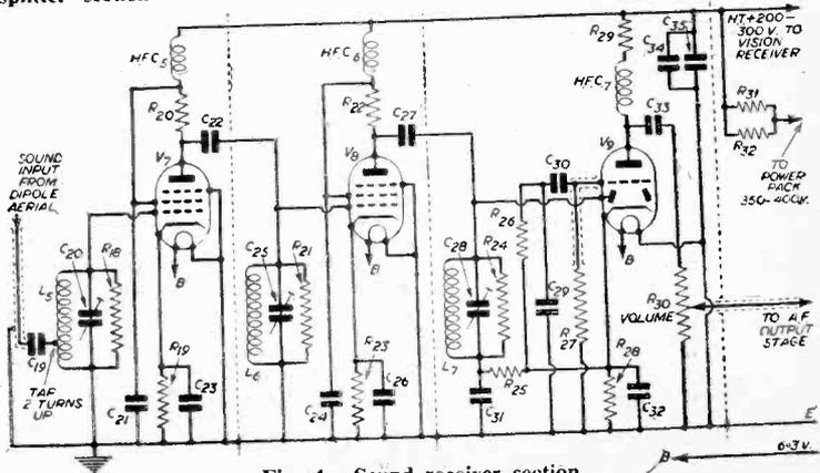
Fig. 4.—Sound receiver section.
