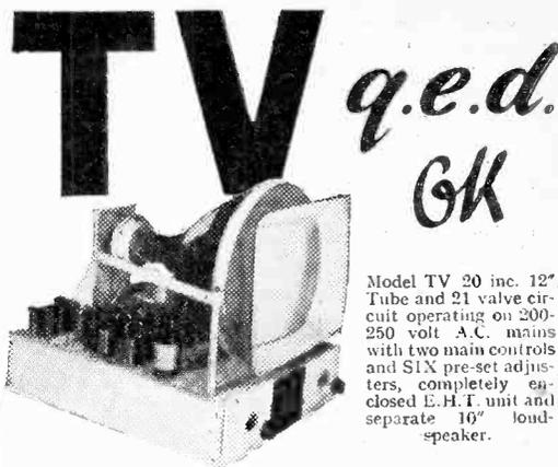
Model TV 20 inc. 12" Tube and 21 valve circuit operating on 200-250 volt A.C. mains with two main controls and SIX pre-set adjusters, completely enclosed E.H.T. unit and separate 10" loud-speaker.
