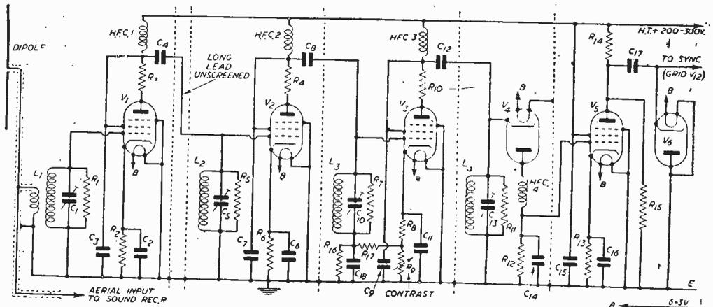
Fig. 1.—Vision receiver. If it is desired to have the contrast control (R9) on the front panel, it would be desirable to transfer it to V2.
