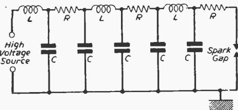
Fig. 1.—Equivalent circuit of the lead connecting distributor to plug.
