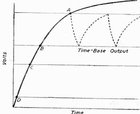
Fig. 4.—Charging curve of a condenser.
