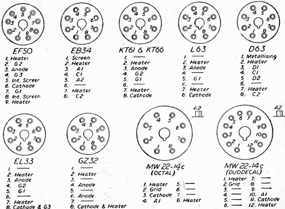
Fig. 7.—Details of valve bases for all the valves and tube used in the complete receiver. Existing stocks of the 22-14c tube are fitted with octal base, but this is being changed to the duodecal base. All views are of the valve or valveholder seen from the underside.
