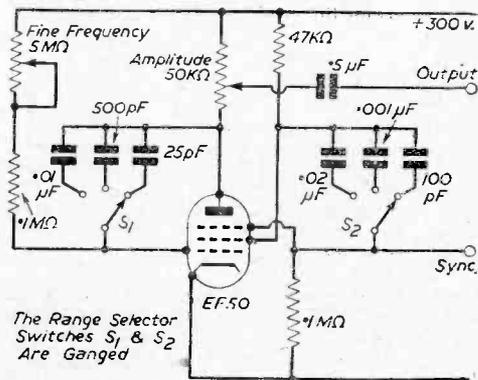
Fig. 12.—A practical Transistron-Miller time-base.
