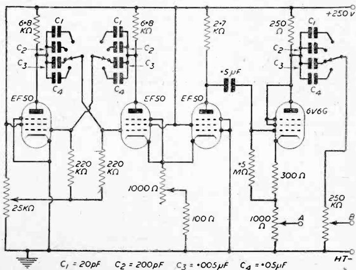
Fig. 1.—Theoretical circuit of the instrument described here.
