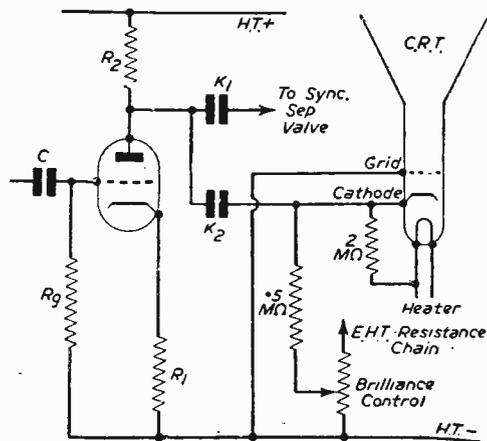
Fig. 2.—In this circuit the signal and sync pulses are taken from the anode of the video valve, and the cathode of the tube is modulated.
