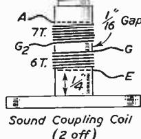
Fig. 7.—Details of the coils and the video corrector choke. The wire used for the coils is No. 28 D.C.C.
