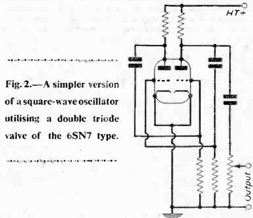
Fig. 2.—A simpler version of a square-wave oscillator utilising a double triode valve of the 6SN7 type.
