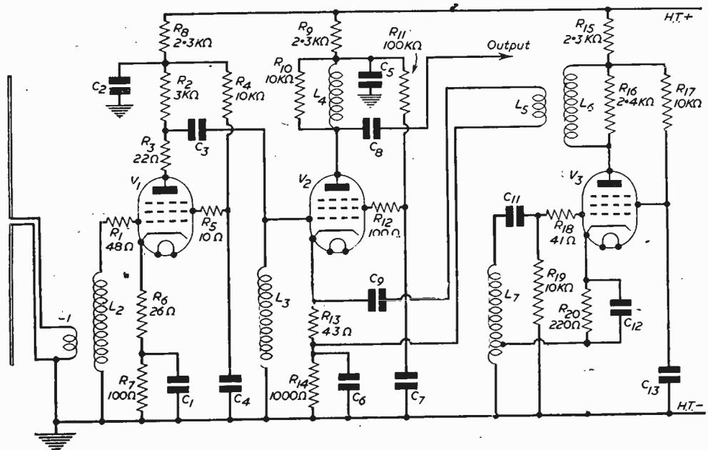
Fig. 1.—Original circuit of the RF24 Unit.
