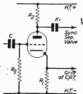
Fig. 1.—The most popular method of feeding the VCR97 as used in many ex-Service conversions.
