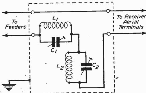
Fig. 1.—Circuit of the Wavetraps.
