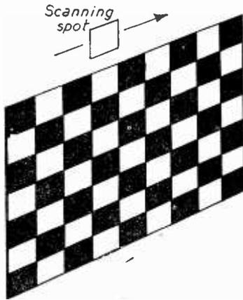
Fig. 23.—Example of rapid changes from black to white giving rise to ripple and distortion of vertical lines.
