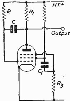
Fig. 9.—Basic circuit of Transatron-Miller time-base.
