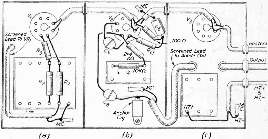
Fig. 3.—Underneath View. Only components and connections requiring alteration are shown in the drawing.
