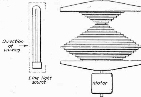
Fig. 2.—The mirror screw apparatus.
