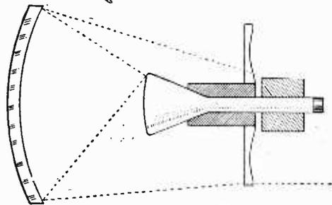
Fig. 4.—Obstruction of light by the scanning and focusing coils.
