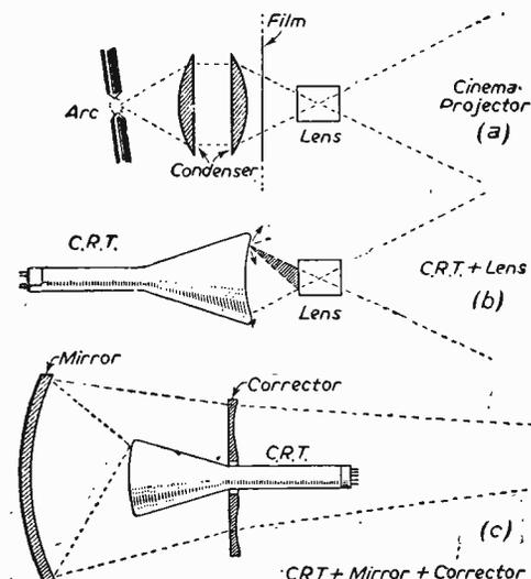
Fig. 3.—Projection systems: (a) Cinema projector. (b) C.R. tube and lens. (c) C.R. tube and mirror.
