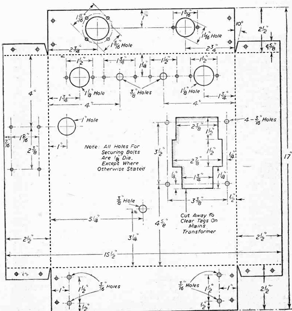
Fig. 1.—Cutting and drilling data for the chassis of the mains unit.
