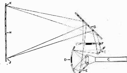
Fig. 5.—Optical system of the Mullard unit. A and B are two picture points on the face of cathode-ray tube C. D is the spherical mirror, E the 45 degree mirror through which the tube is placed. F is the correction lens, G a mirror in the lid of the cabinet, and H the viewing-screen. Light from A is focused at J and light from B at K.
