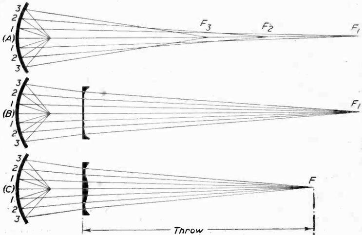
Fig. 6.—The principle of the correction lens.
