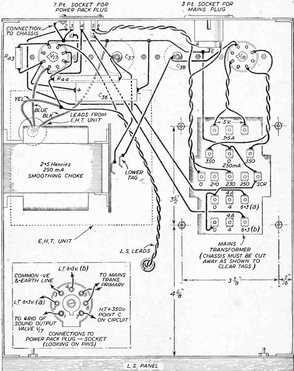
Fig. 3.—Wiring diagram of the power supply and audio output stage.
