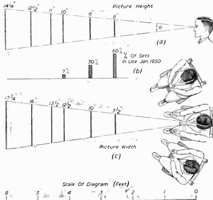
Fig. 1.—(a) Angle of view depends on the number of lines, not on picture size. (b) Most receivers in use have small pictures. (c) A large picture enables more people to view in comfort.
