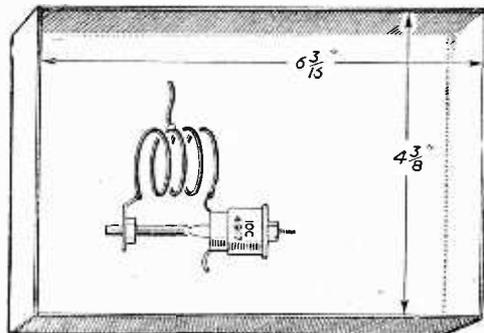
Figs. 2 and 3.—The "lid" for the chassis—showing dimensions, and details of the coils and their mounting.
