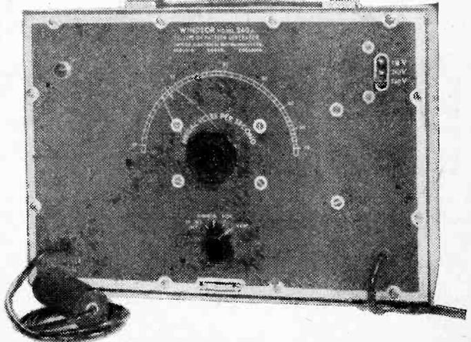
A pattern generator from the Windsor range of test instruments.
