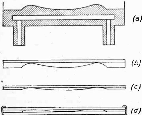
Fig. 7.—Manufacture of gelatine correction lens; (a) Mould; (b) Wet gelatine; (c) Dried gelatine; (d) Completed lens.
