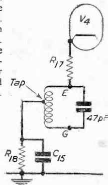
Fig. 1.—The rejector circuit in the fourth stage.
