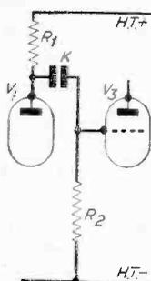
Fig. 2.—The coupling components of the circuit in Fig. 1.
