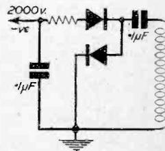
Fig. 2.—Two metal rectifiers used in place of a 6H6 or similar valve.
