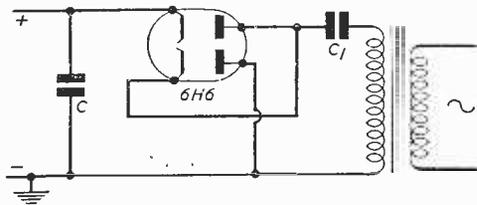
Fig. 5.—The values of C and C1 play an important part in the output rating.
