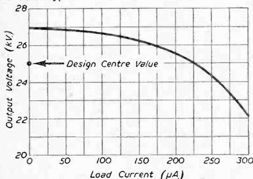
Fig. 11.—Limiting regulation curve of E.H.T. supply.
