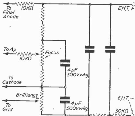
Fig. 2.—Additions to E.H.T. circuit which will help to remove 50 cycle ripple.
