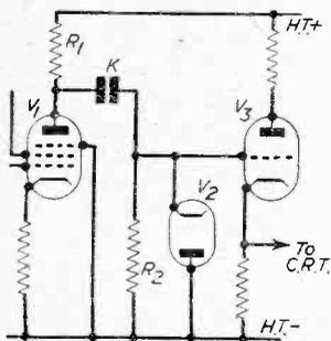
Fig. 1.—Condenser K affects the response of V3 compared with V1.
