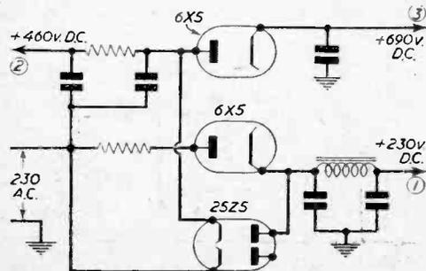
Fig. 1.—Obtaining various voltages without complicated networks.
