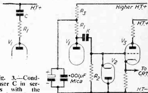
Fig. 3.—Condenser C in series with the anode load will result in a rising characteristic.
