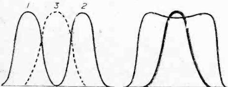
Figs. 3 & 4.—A "square" response is obtained by several single tuned circuits staggered about the main frequency, or by a "peaking" circuit and band-pass circuits.
