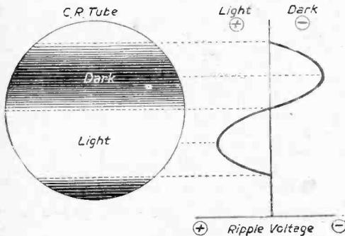
Fig. 1.—50 cycle ripple voltage and its effect on the picture. (Compare with Fig. 3.)
