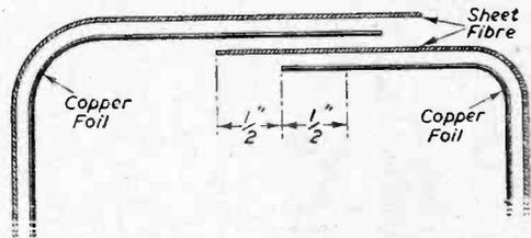
Fig. 2.—Method of insulating the screen.
