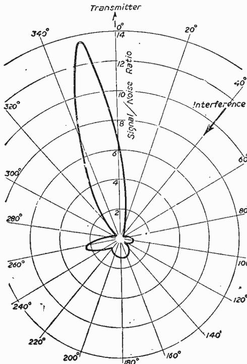
Fig. 7.—Polar diagram for signal/noise ratio for Fig. 6, with equal interference source at 40 degrees.
