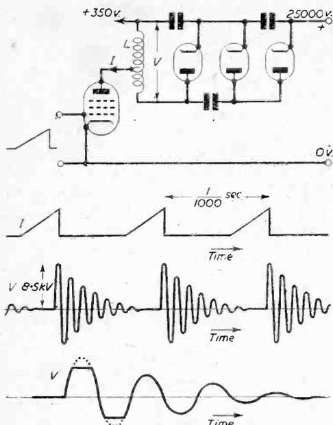
Fig. 14.—The voltage tripling circuit, waveforms of input voltage, and anode voltage.
