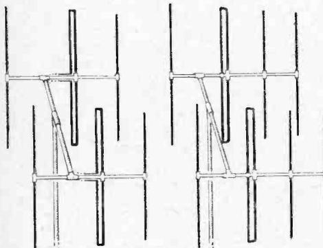
Fig. 3.—Multiple element arrays for use under difficult conditions.
