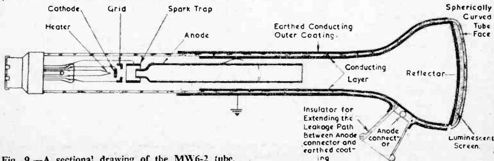
Fig. 9.—A sectional drawing of the MW6-2 tube.
