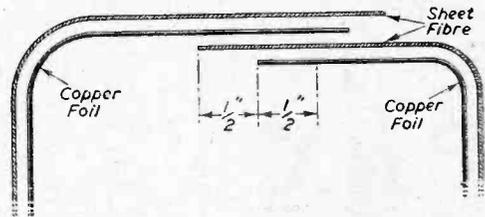
Fig. 2.—Method of insulating the screen.
