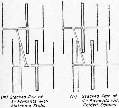
Fig. 3.—Multiple element arrays for use under difficult conditions.
