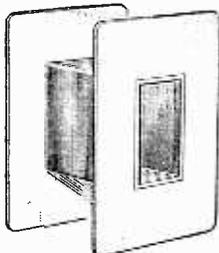
Fig. 3.—A typical transformer bobbin.
