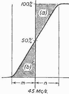
Fig. 6.—The critical part of the curve shown in Fig. 5 is indicated here. The sections  $m$  and  $n$  should be equal, as also should be areas (a) and (b).
