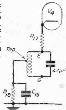
Fig. 1.—The rejector circuit in the fourth stage.
