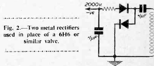
Fig. 2.—Two metal rectifiers used in place of a 6H6 or similar valve.
