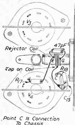
Fig. 2.—Practical arrangement of the rejector circuit.
