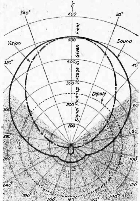
Fig. 8.—Polar diagram for sound and vision on a 3-element array.
