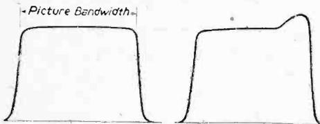
Figs. 1 & 2.—Ideal response curve of a vision receiver, and the type of curve most generally adopted.
