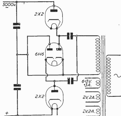
Fig. 6.—A circuit for providing E.H.T. voltages.
