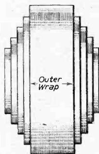
Fig. 8.—In construction the windings should be progressively stepped back as the windings go on, as in the illustration.
