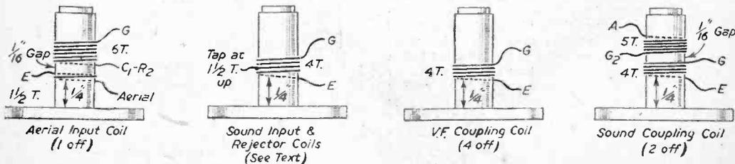
Fig. 5.—Details of the coils for the Sutton Coldfield transmission.
