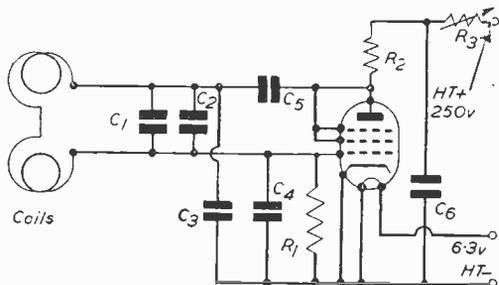
Fig. 3.—Circuit of the arrangement: R1 56 kΩ 1 watt; R2 10 kΩ ½ watt; R3 50 kΩ variable resistor; C1 100 pF; C2 50 pF variable trimmer; C3 50 pF; C4 50 pF; C5 500 pF; C6 500 pF; V—6F12, 8D3, 277, etc.
