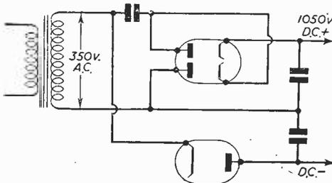
Fig. 4.—A half-wave rectifier used as a stabiliser.
