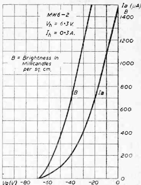
Fig. 10.—Anode-current and brightness characteristics of the MW6-2 Projection C.R. Tube.
