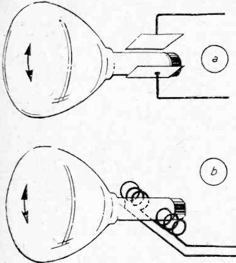
Fig. 2.—Arrangement of the main components for magnetic and electrostatic tubes.
