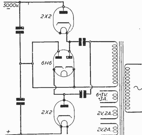
Fig. 6.—A circuit for providing E.H.T. voltages.
