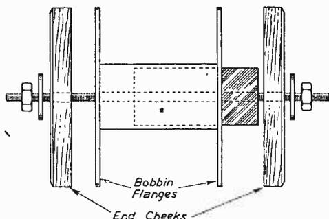
Fig. 4.—Assembly of the winding jig.
