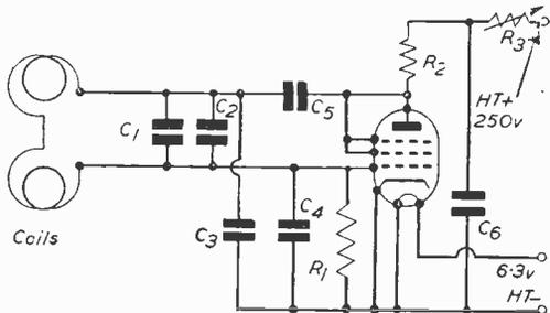
Fig. 3.—Circuit of the arrangement: R1 56 k $\Omega$  1 watt; R2 10 k $\Omega$   $\frac{1}{2}$  watt; R3 50 k $\Omega$  variable resistor; C1 100 pF; C2 50 pF variable trimmer; C3 50 pF; C4 50 pF; C5 500 pF; C6 500 pF; V—6F12, 8D3, 277, etc.
