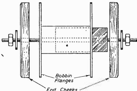
Fig. 4.—Assembly of the winding jig.
