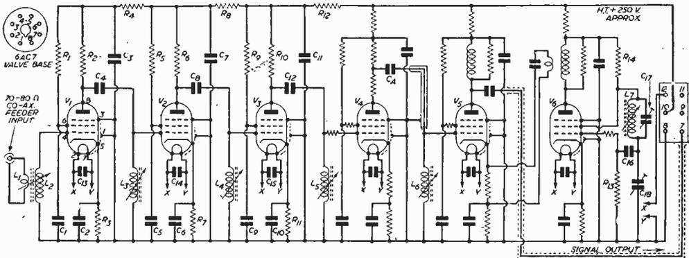
Fig. 1.—The circuit. Component values refer only to the new circuits. L1 should be earthed.
