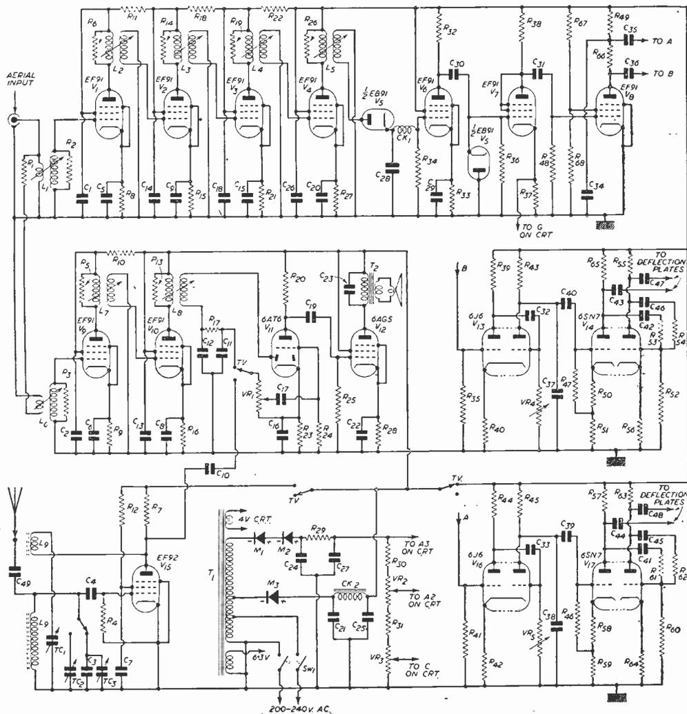
Circuit of the Completed Midget Television-radio Receiver built by the Author and illustrated on page 399. A full list of the components used in the original model will be found on page 395.
