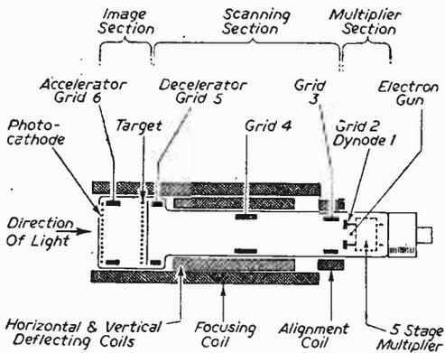
Fig. 2.—Schematic arrangement of the Image Orthicon.
