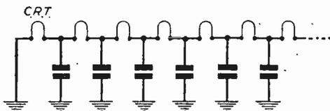
Fig. 2.—Decoupling condensers should be included in all H.F. circuits as shown here.
