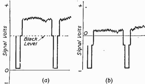
Fig. 3.—Effect on the D.C. component of the coupling condenser (a) without condenser, and (b) with condenser
