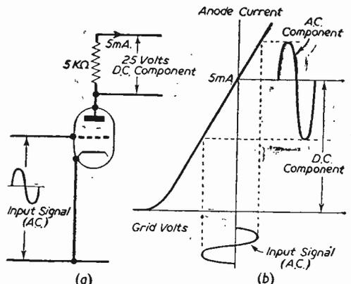
Fig. 1.—Simple triode circuit illustrating the D.C. component.
