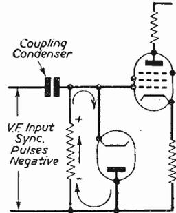
diode in each position, but it is quite possible to use a Westector type WX 6 in front of the tube grid and this dispenses with the necessity of a separate heater winding for the diode.
