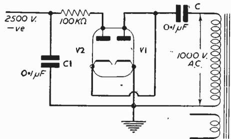
Fig. 3.—A simple doubler circuit.
