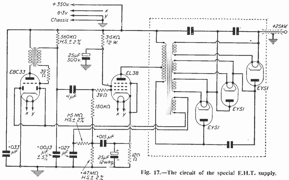
Fig. 17.—The circuit of the special E.H.T. supply.
