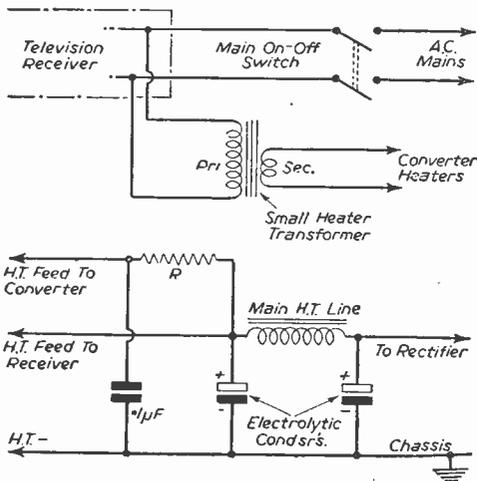
Fig. 2 (Top).—Use of additional heater transformer, and Fig. 3 (Bottom)—a decoupled H.T. feed for the converter.
