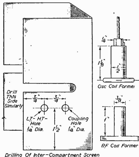
Figs. 3, 4 & 5.—Details of the inter-compartment screen and the coil-formers.
