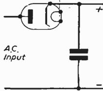
Fig. 1.—A standard half-wave rectifier circuit.
