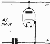
Fig. 2.—A variant used on some A.C./D.C. receivers.
