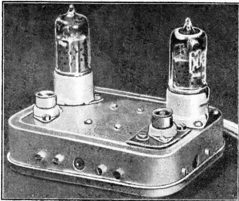
The finished unit, showing trimmers and co-axial connectors.
