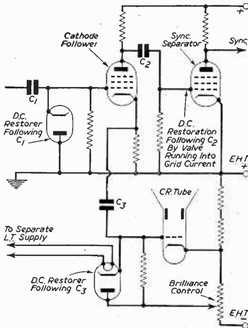
Fig. 5.—Circuit of a cathode follower video stage feeding the tube from the cathode and the sync separator from the anode.
