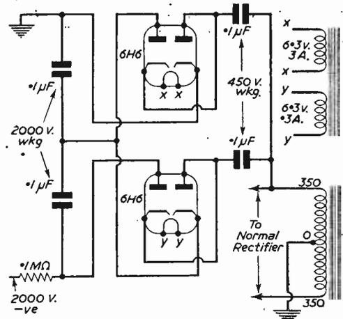
Fig. 5.—A high voltage quadrupler circuit.
