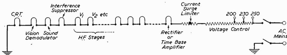
Fig. 1.—The arrangement of the heater circuits in a D.C. operated television receiver.
