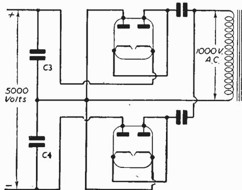
Fig. 4.—A quadrupler circuit—two doublers of the type shown in Fig. 3.
