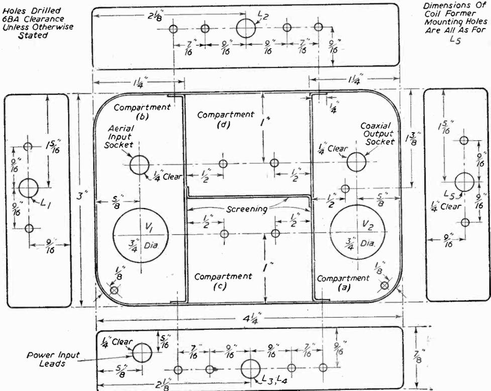
Fig. 4.—Top view of "chassis," showing position of screening. Holes are drilled 6BA clearance unless stated otherwise.
