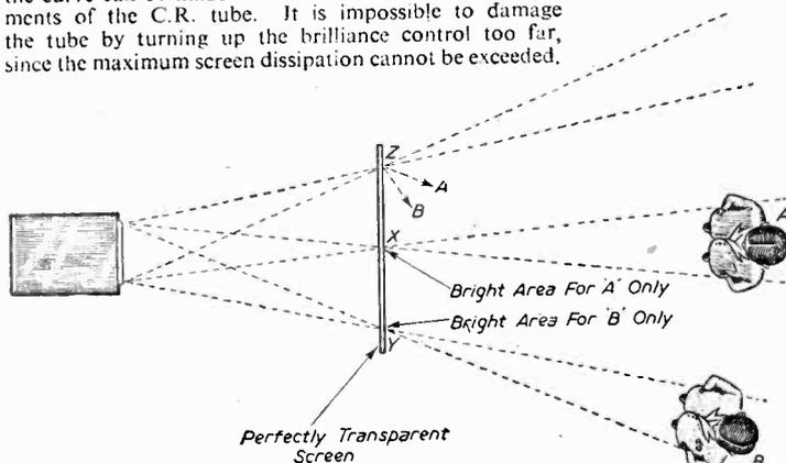
Fig. 19.—Diagram showing the function of a viewing screen.
