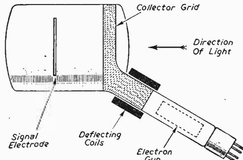
Fig. 1.—Schematic arrangement of the Iconoscope.
