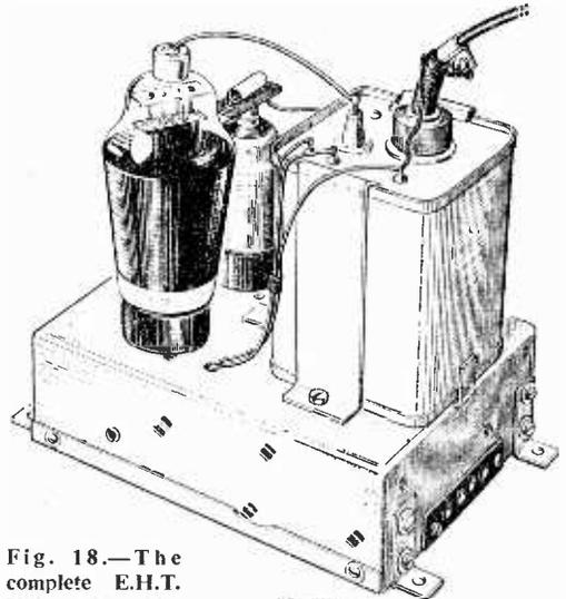
Fig. 18.—The complete E.H.T. Unit and special anode connector.
