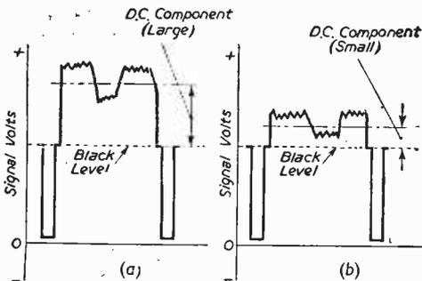
Fig. 2.—Video signal, D.C. component, and sync pulses.
