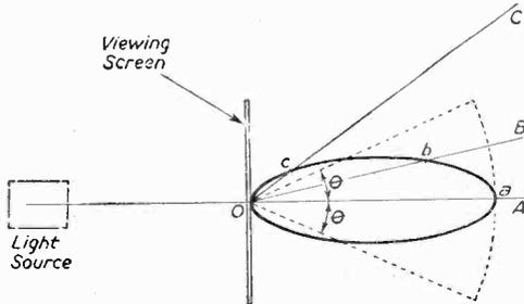
Fig. 20.—The polar diagram of brightness. The full-line curve is for an etched glass screen. The dotted curve is the ideal.
