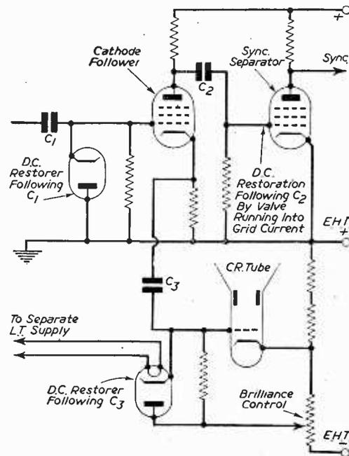
Fig. 5.—Circuit of a cathode follower video stage feeding the tube from the cathode and the sync separator from the anode.
