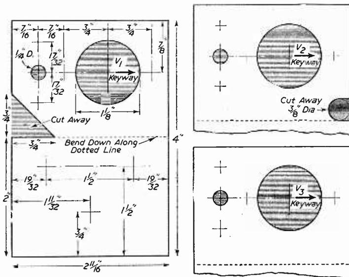
Fig. 2.—The sub-chassis, underside view. All dimensions are identical except for cut-away portions.
