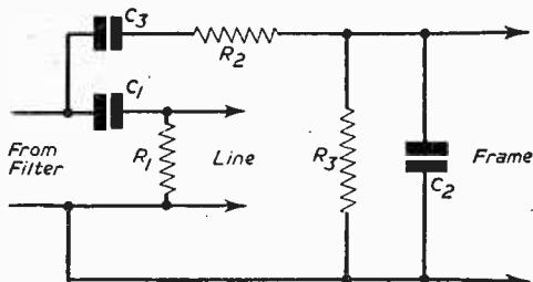
Fig. 1.—This is the basic integrator and differentiator circuit arrangements for use in frame and pulse separation. Although such an arrangement could be used following a limiter its efficiency would be low due to a variety of reasons. Compare this with the elaborate arrangement used in Figs. 4 or 6.
