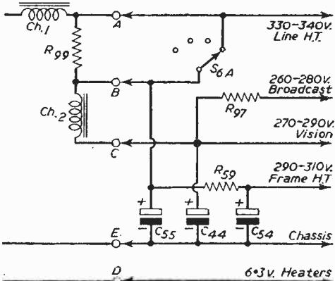
Fig. 4.—The voltage divider circuits
