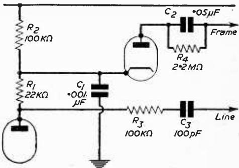
Fig. 3.—A simple form of frame pulse selector using a diode. This arrangement is used in the "Practical Television" receiver.
