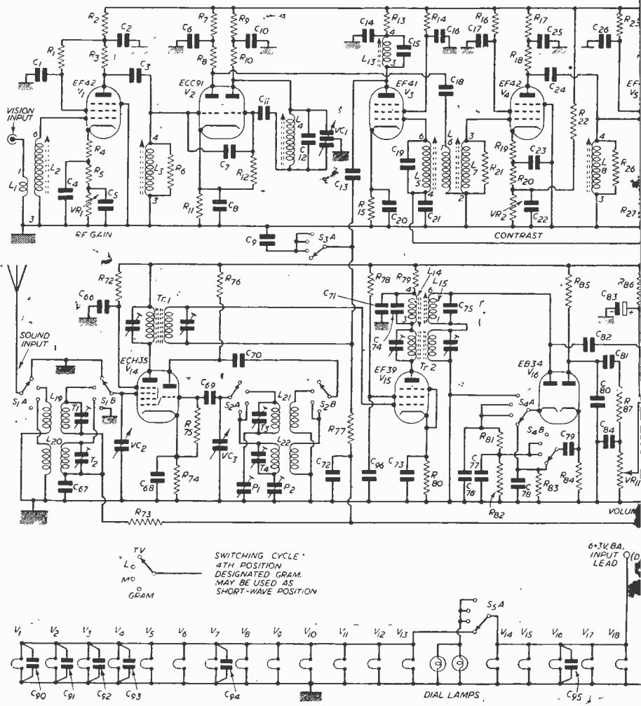
Fig. 1.—Theoretical circuit of the combined receiver, exo
