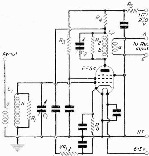
Fig. 1.—Single-valve pre-amplifier circuit.
