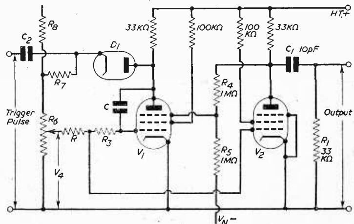
Fig. 2.—The Miller-Sanatron circuit.
