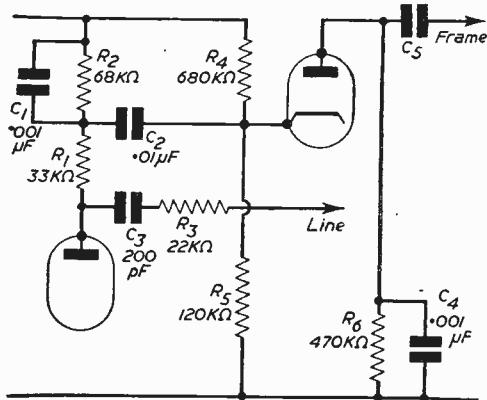
Fig. 4.—A more elaborate circuit, but still retaining the diode. This is the G.E.C. interlace filter arrangement.
