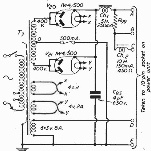
Fig. 3.—Theoretical circuit of the mains unit.
