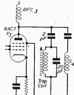
Fig. 5.—“Sucker” trap circuit to remove sound from the vision channel.
