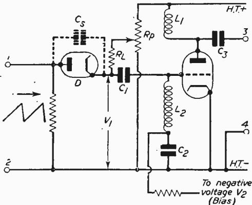
Fig. 1.—Multivibrator circuit for the production of marker pips.
