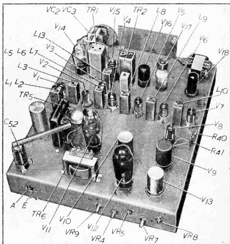
Fig. 2.—Chassis layout with essential component references.
