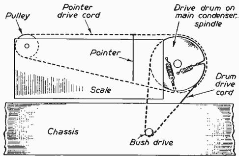
Fig. 3.—Suggested dial and condenser drive arrangement.
