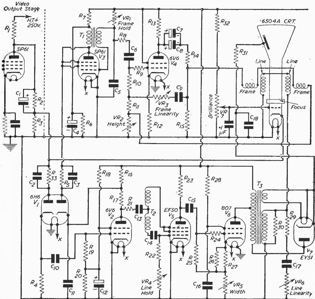
Fig. 2.—Complete circuit of the final arrangement.
