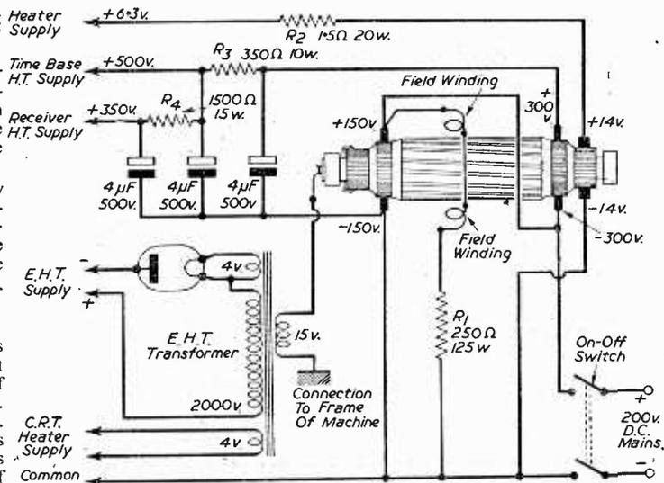
Fig. 5.—Complete circuit of power pack.
