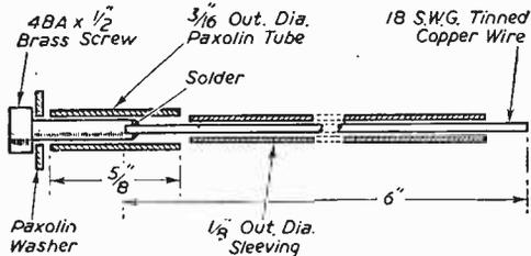
Fig. 4.—A.C. lead before insertion in armature.
