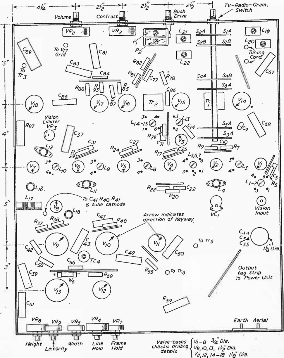
Fig. 2.—Details of chassis measurements, component positions, etc.
