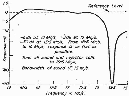
Fig. 4.—I.F. response after rejectors are tuned.
