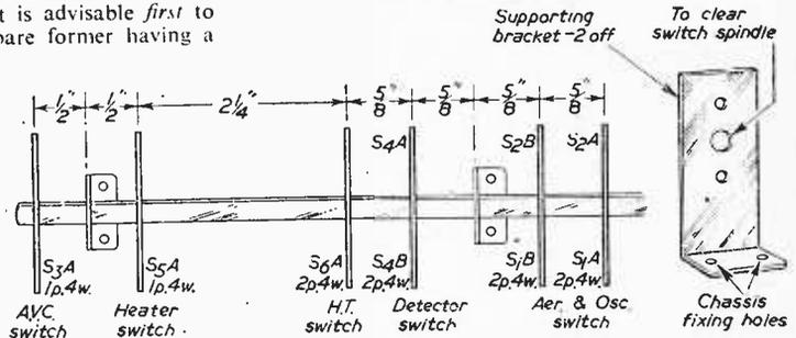
Fig. 5.—Ganged switch details.
