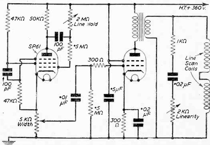
Fig. 1.—Experimental line time-base circuit.
