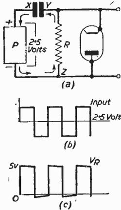
Fig. 7.—Action of circuit during D.C. restoration.
