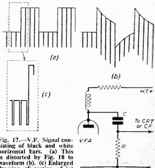
Fig. 17.—V.F. Signal consisting of black and white horizontal bars. (a) This is distorted by Fig. 18 to waveform (b). (c) Enlarged drawing of section of (a) to show sync pulses more clearly.
