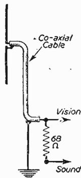
Fig. 1.—Coupling sound and vision receivers.
