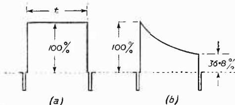
Fig. 19.—(a) Video signal, constant white line; (b) Video signal after C.R. circuit (Fig. 18), when C.R. is too small (0.0001 secs.).
