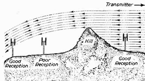
Fig. 1. Diagram illustrating the "shadow" effect of high ground.
