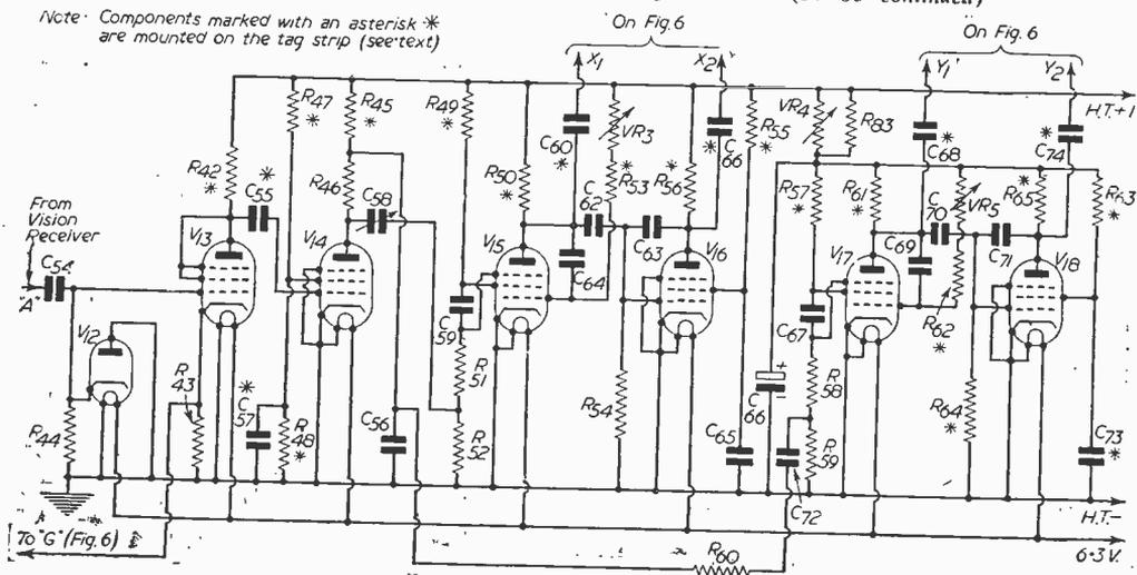
Fig. 4.—Circuit of the time-base section.
