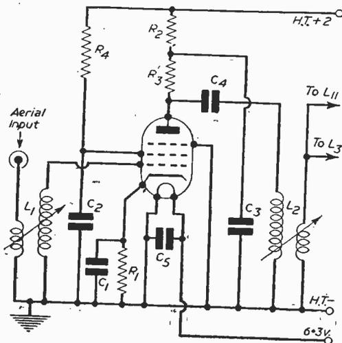
Fig. 2.—Circuit of the first R.F. stage.
