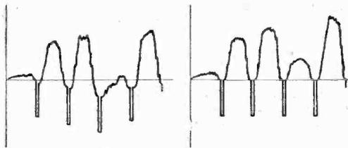
Fig. 16.—Signal after passing through coupling condenser.
