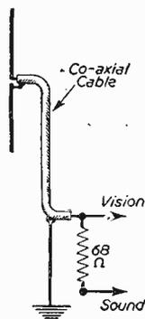
Fig. 1.—Coupling sound and vision receivers.
