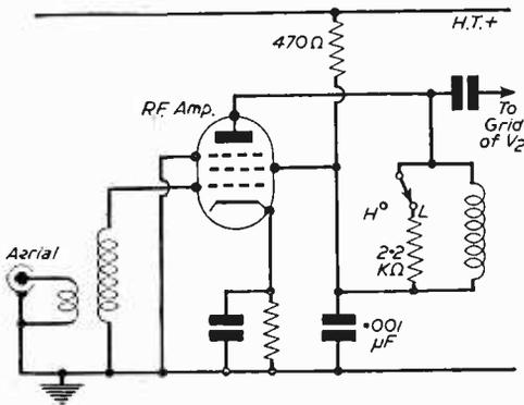
Fig. 1.—How to connect "High/Low" sensitivity switch to series circuit (tuned anode).
