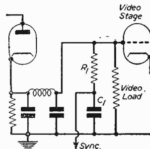
Fig. 2.—Taking off the sync pulse before the video stage.
