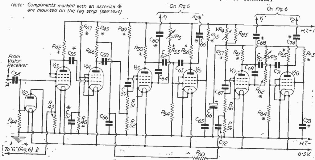
Fig. 4.—Circuit of the time-base section.
