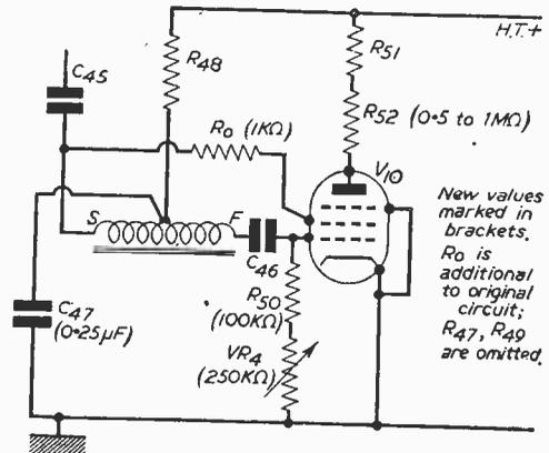
Modified circuit of the line oscillator stage in the Combined Televisor.
