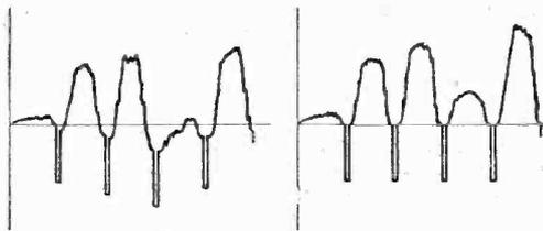
Fig. 16.—Signal after passing through coupling condenser.
