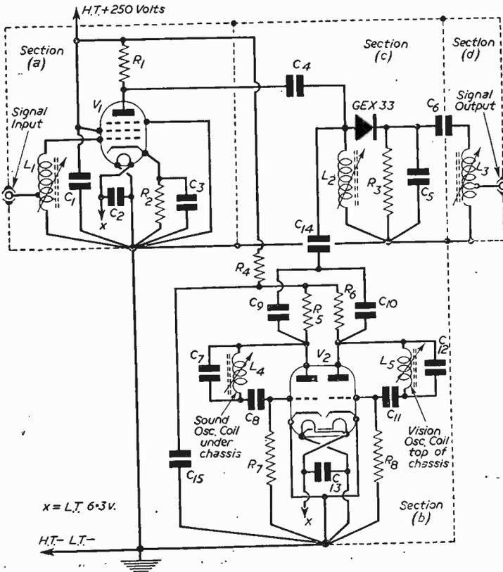
Fig. 3.—Theoretical circuit of the converter.
