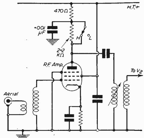
Fig. 2.—Sensitivity switch connections for parallel circuit (tuned grid).
