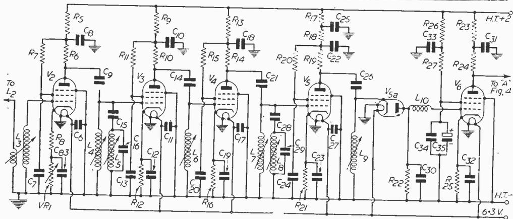
Fig. 3.—Circuit of the vision section.
