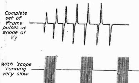
Oscillograms in connection with Interlace Filter.
