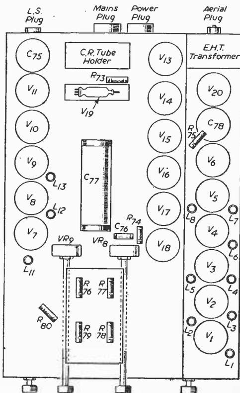
Fig. 1.—Layout of chassis top.
