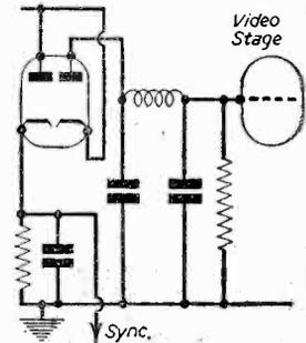
Fig. 3.—An alternative method of taking off the sync pulse and providing better rectification.
