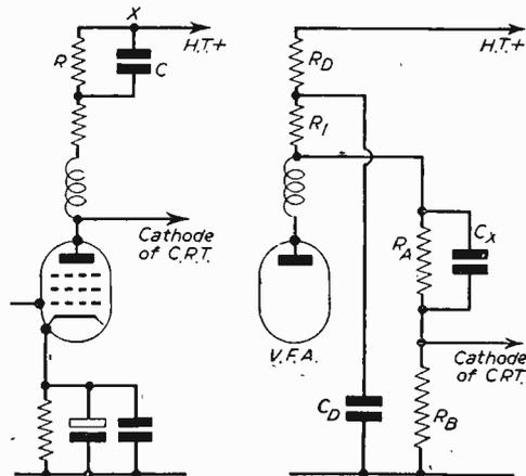
Fig. 20 (left).—L.V.F. Compensation for cathode bias circuit. Fig. 21 (right).—L.V.F. Compensation for decoupling, etc.
