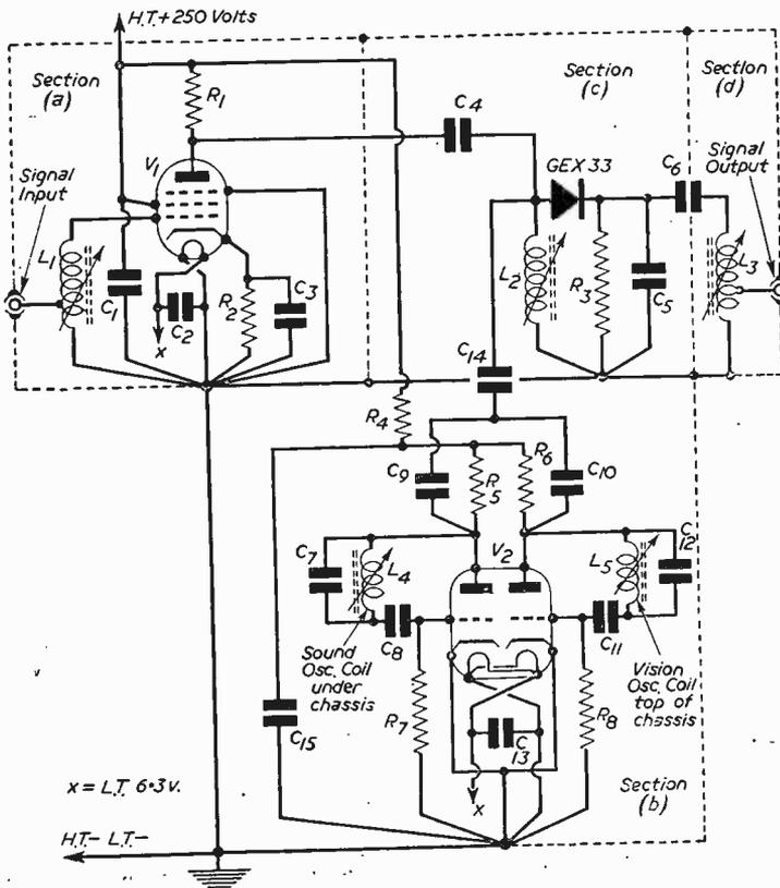
Fig. 3.—Theoretical circuit of the converter.
