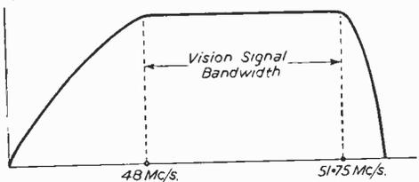
(a) Frequency characteristic of Channel 2 Vision Transmission
