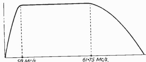
(b) Frequency characteristic of the converted Channel 2 Transmission as applied to a Channel 4 Receiver
