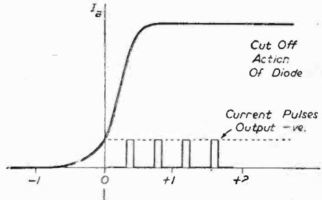
Fig. 3.—Negative-going output pulses.
