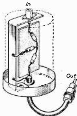
Fig. 4.—A practical interpretation of an attenuator of the type shown in Fig. 3—showing a suitable screening can.
