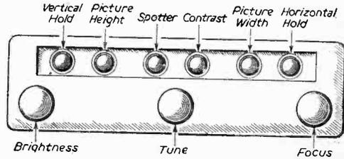
Fig. 3.—Controls on front of Model 901.
