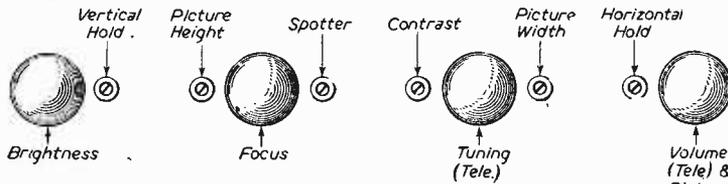
Fig. 5.—Controls on front of Models 912, 914.
