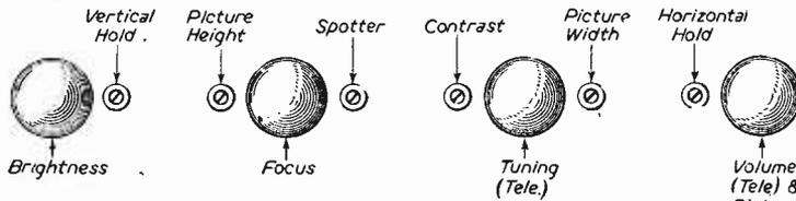
Fig. 5.—Controls on front of Models 912, 914.
