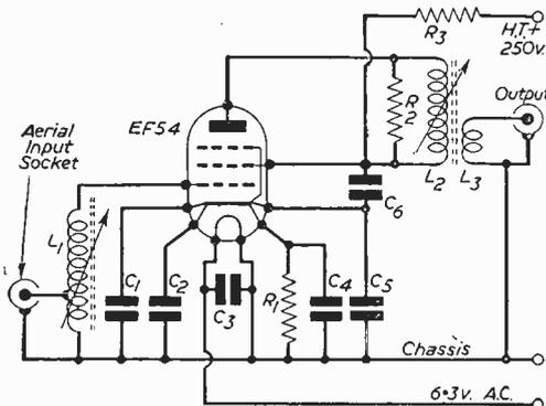
Fig. 1.—Circuit of the pre-amplifier.
