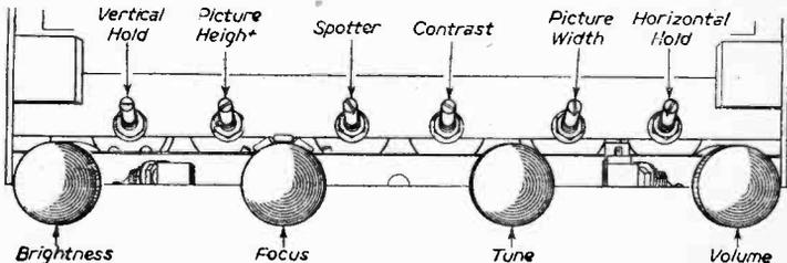
Fig. 4.—Controls on front of Model 902.
