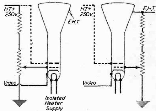
Note: Dotted connections necessary for tetrode tubes only
