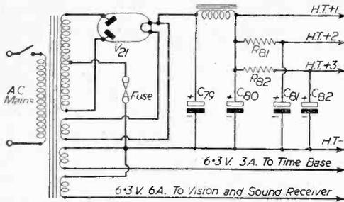
Fig. 7.—Circuit of the power pack.
