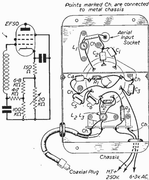
Fig. 5 (left). Contrast control circuit suitable for EF50, EF91, SP61. Fig. 6 (right). Underside of pre-amplifier.
