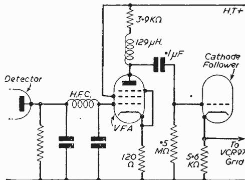
Fig. 22.—A complete video output stage.
