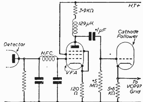
Fig. 22.—A complete video output stage.
