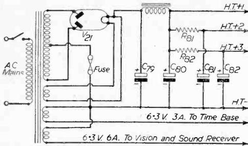
Fig. 7.—Circuit of the power pack.
