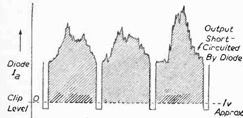
Fig. 2.—How the picture impulses are shorted and the negative pulses obtained.
