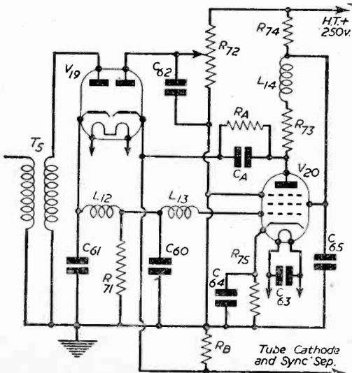
Fig. 1.—Video and noise suppressor stage.
