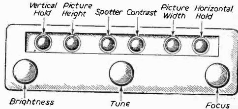
Fig. 3.—Controls on front of Model 901.
