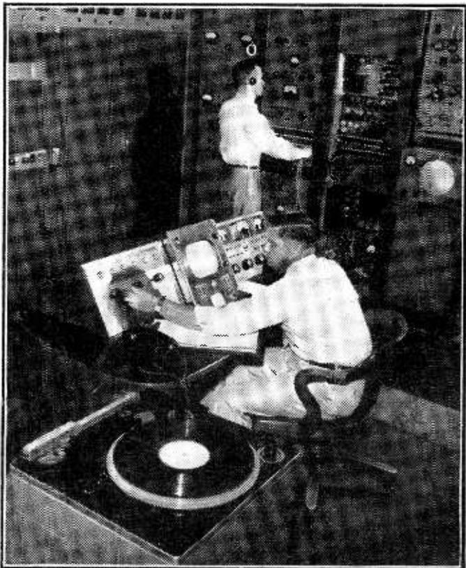
This compact control room contains all the equipment necessary to put a small Ultra High Frequency community television station on the air. It's located in RCA's experimental UHF television station at Bridgeport, as described above.
