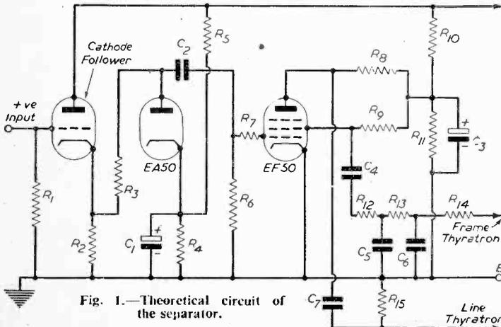
Fig. 1.—Theoretical circuit of the separator.
