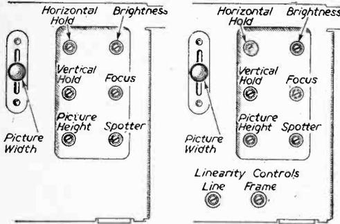
Fig. 1 (left).—Preset controls on back of models 916/917 and 923 (some models may also have the two linearity controls shown below on Models 918, 919, 920). Fig. 2 (right).—Preset controls on back of Models 918, 919, 920.
