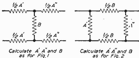
Fig. 6.—Networks for a balanced line.
