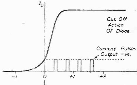
Fig. 3.—Negative-going output pulses.
