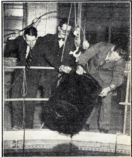
Engineers preparing to lower the underwater TV camera in its pressure casing, into the test tank.
