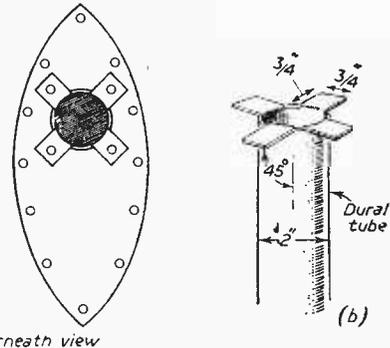
Fig. 6.—Details of the mounting required for the scheme shown in Fig. 5.
