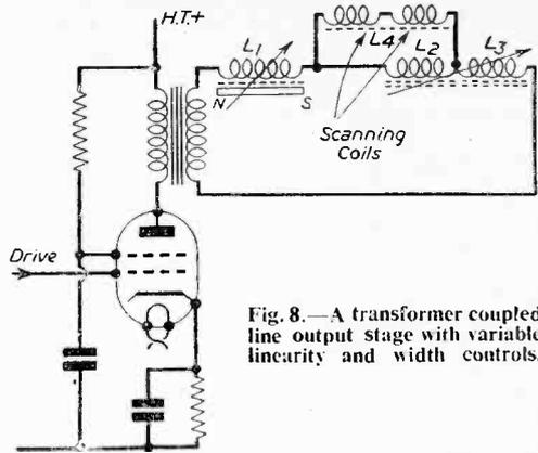
Fig. 8.—A transformer coupled line output stage with variable linearity and width controls.
