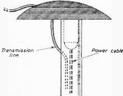
Fig. 5.—An alternative method of mounting the amplifier.
