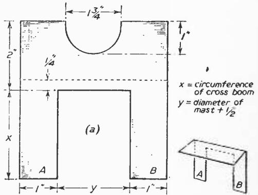
Fig. 4.—Details of the fixing clamp which can be seen in Fig. 3.
