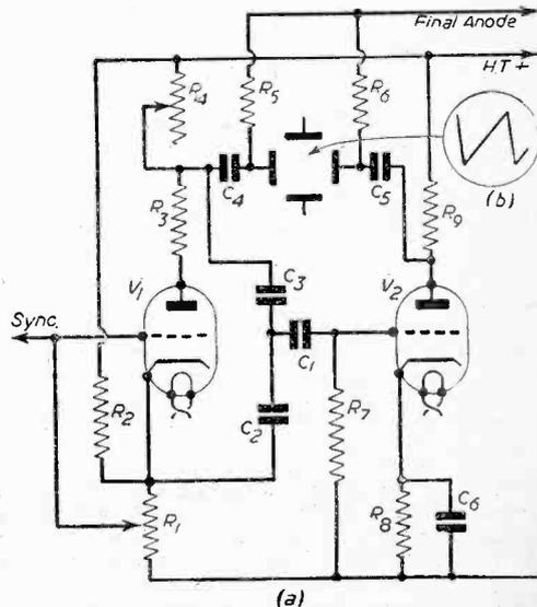
Fig. 2.—A self-linearising push-pull time-base.
