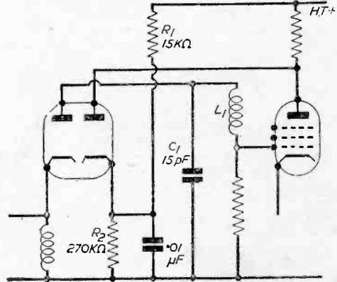
Fig. 14.—This is a Vidor arrangement.
