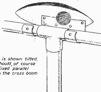
Unit is shown tilted. It should, of course be fixed parallel with the cross boom
