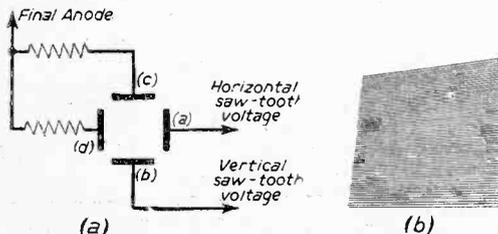
Fig. 1.—Showing the cause of trapezium distortion at (a) and its effect at (b).
