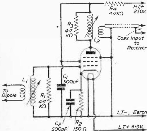
Fig. 1.—Circuit of the Aerial Pre-Amplifier.
