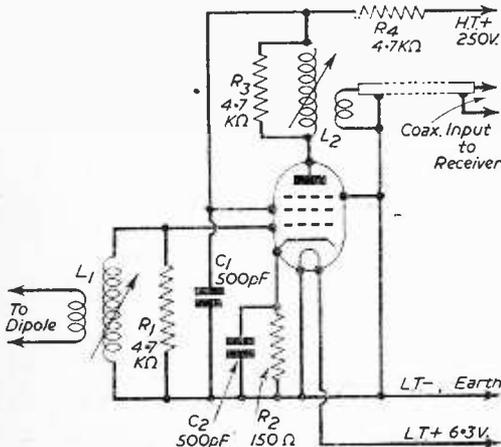
Fig. 1.—Circuit of the Aerial Pre-Amplifier.
