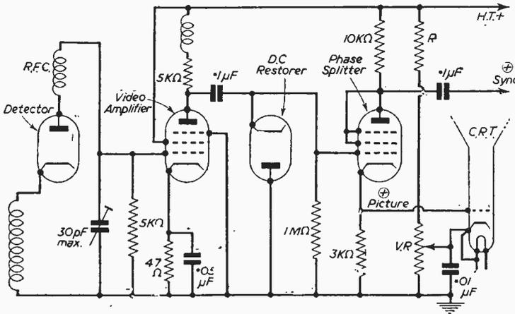
Circuit of the re-arranged tube-feed.
