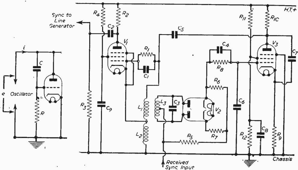
Fig. 3.—In this circuit capacitive or inductive effects are given by the relative positions of C and R.
