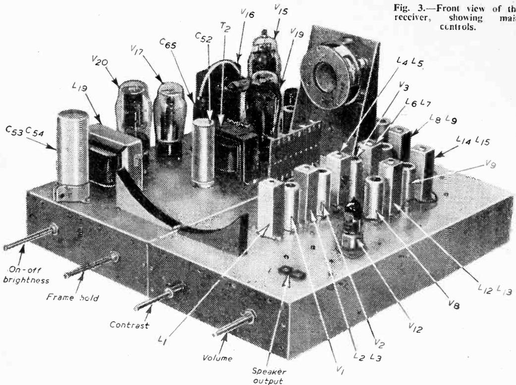
capacities are necessary even on D.C. supplies where ripple can sometimes be almost as severe as badly smoothed alternating current supplies. Choke L19 is rated at 5 henries, 250 mA. and its D.C. resistance is 50 ohms. A smaller resistance is permissible, but 50 ohms should not be exceeded, especially by those constructors whose mains supplies are below 220 volts. The sound receiver is separately fed through R56 and additionally decoupled by C52.
