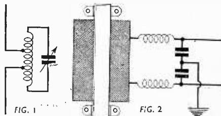
Figs. 1 and 2.—Trap coil and mains suppressor circuits.
