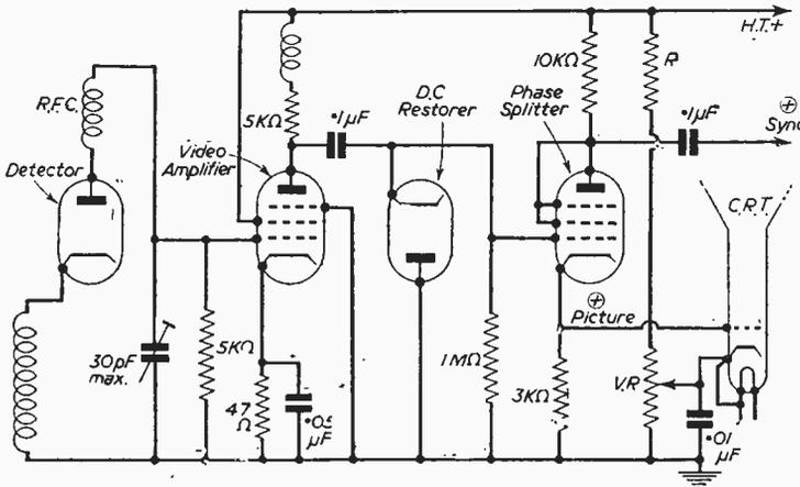
Circuit of the re-arranged tube-feed.
