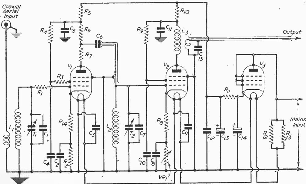
Fig. 1.—Circuit of the first A.C./D.C. Pre-amplifier.
