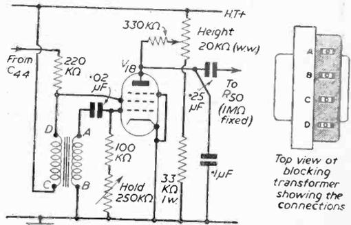
Fig. 4.—Alternative frame oscillator stage. When this circuit is used, the bias resistor of V19 is 160Ω.
