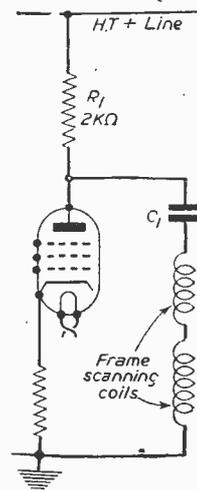
Fig. 2.—A R.C. coupled frame output stage. Note the importance of high insulation across C1.
