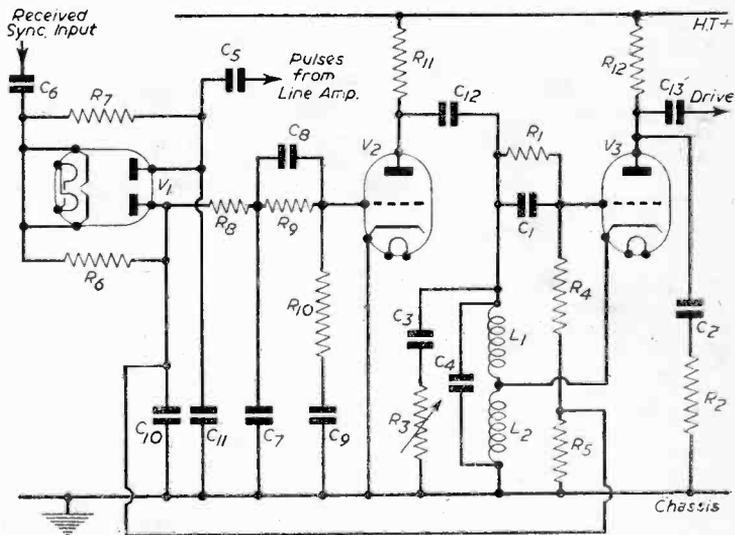
Fig. 2.—A G.E.C. circuit. Component values are :
