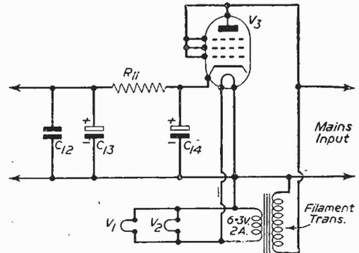
Fig. 7.—Modification when using the unit for A.C. operation only.
