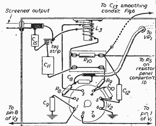
Figs. 4 and 5.—Above and below chassis wiring details.
