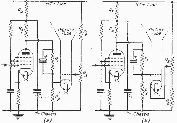
Fig. 1.—Methods of modulating the picture tube: (a) cathode modulation and (b) grid modulation.
