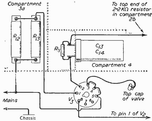
Fig. 6.—Wiring of the mains side.
