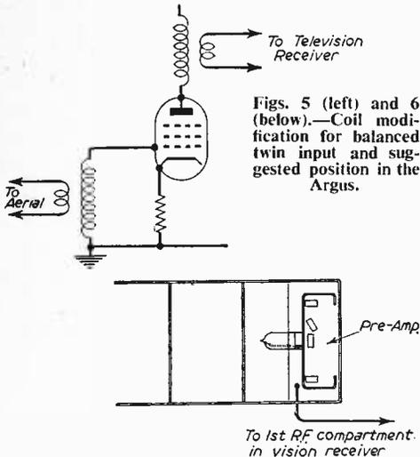
If the bandwidth is found insufficient it can be broadened by connecting a 4.7 K $\Omega$  resistor across L1 and another across the primary of L2.
