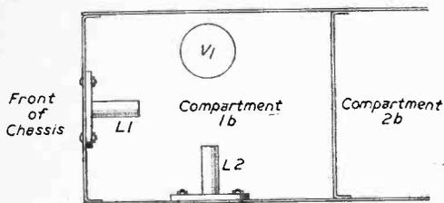
Fig. 9.—Mounting position for L2.
