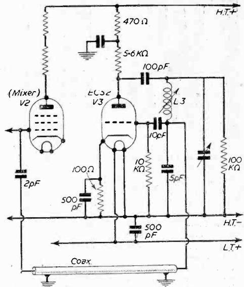
Fig. 13.—Modified oscillator stage. L3 consists of 5 turns 22 s.w.g. on  $\frac{1}{2}$ in. former with iron slug for channels 1 and 2; no slug for channel 3 and brass slug for channels 4 and 5.
