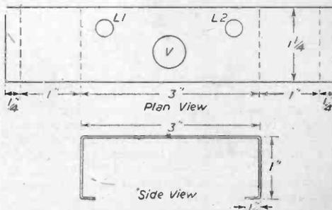
Figs. 2 and 3.—Coil-winding details and chassis data.
