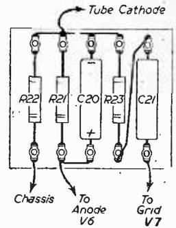
Fig. 12.—Tagboard fitted to tube rear support, showing component wiring.
