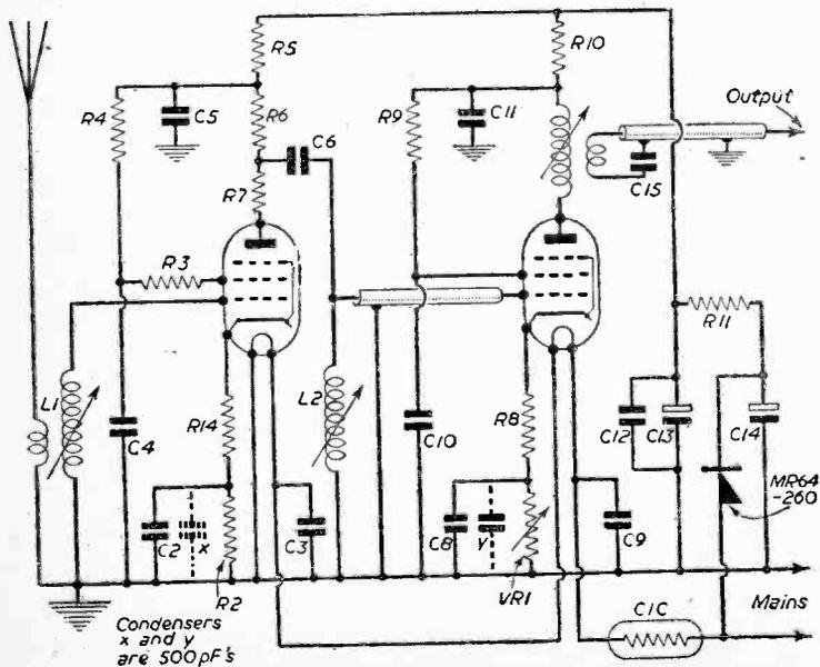
Fig. 8.—Circuit of the two-stage pre-amplifier.
