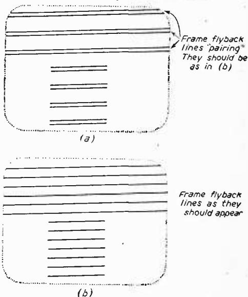
Fig. 2 (right).— Appearance of the flyback lines with correct and one form of incorrect interlacing. On the left is a table of VCR97 characteristics.
