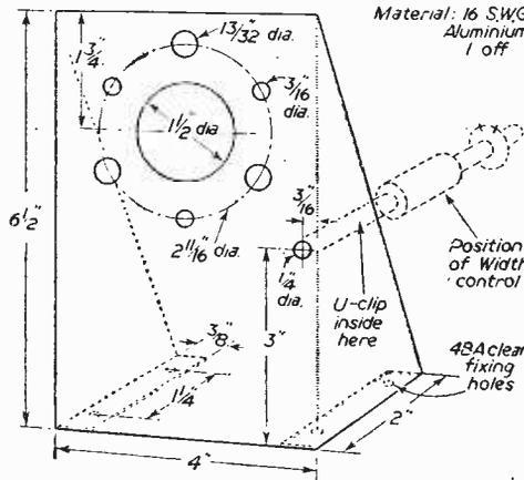
Fig. 13.—Tube and focusing magnet support.
