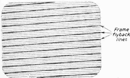
Fig. 1.—Normal appearance of a raster without picture detail.
