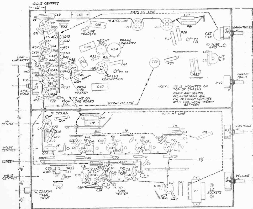
vision and sound receiver is built on one of these chassis, and the timebases and power unit on the other, and in construction each part can be built separately, the bolting together of the units taking place after most of the wiring is completed.
