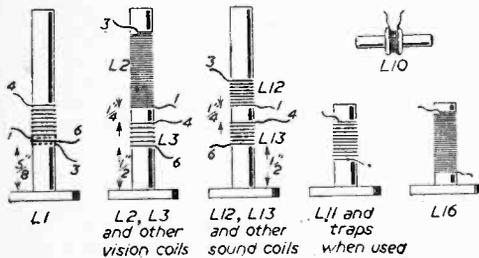
Fig. 8.—Coil winding details.
