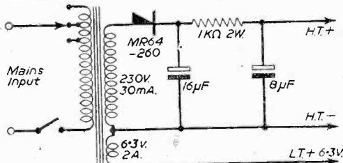
Fig. 11.—Theoretical circuit of the power unit.
