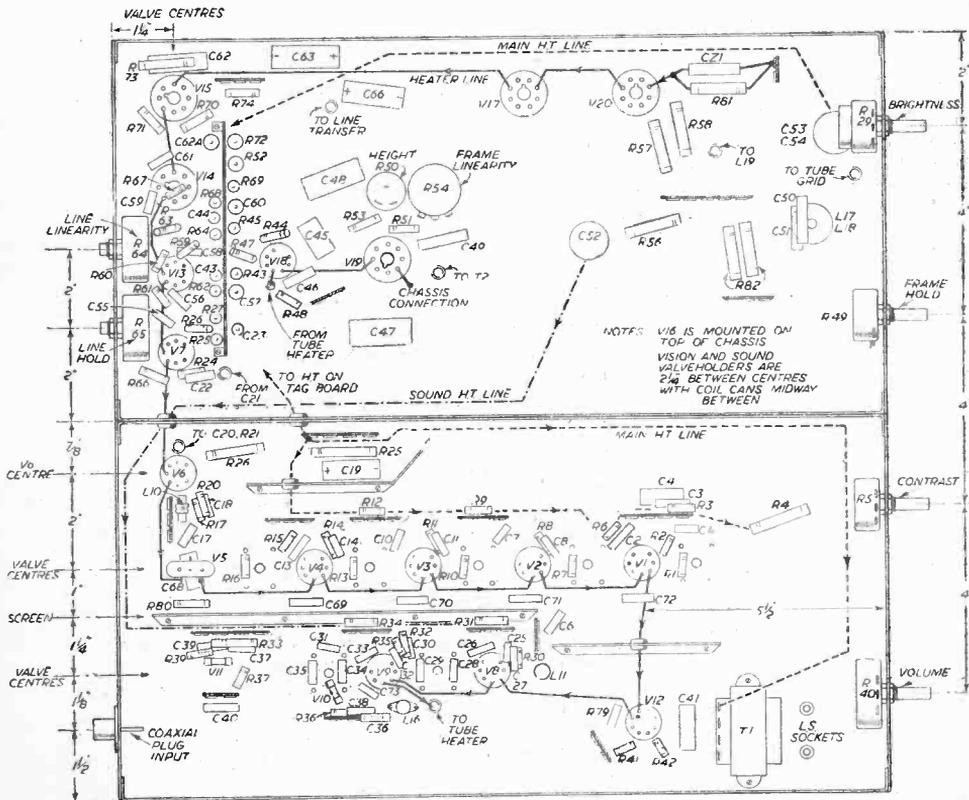
Fig. 6.—Underclass layout of valves and components, showing run of heaters and H.T. lines. This layout applies to the transitron frame oscillator. The principal measurements are given, but small changes are permissible to suit alternative components, etc.
