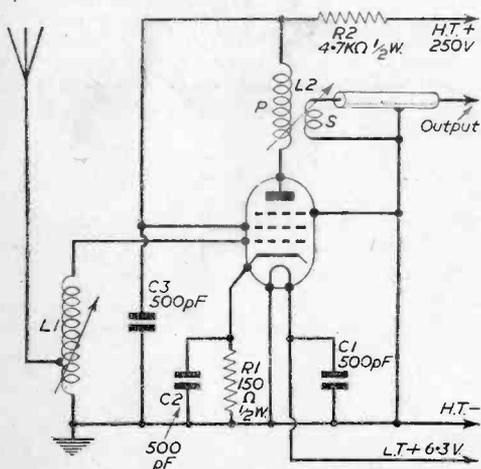
Fig. 1.—Theoretical circuit of the Pre-amplifier.
