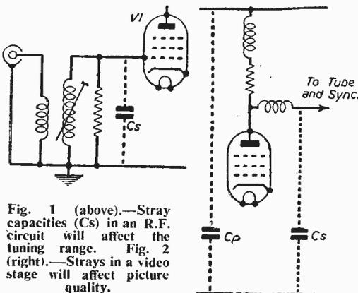
Fig. 1 (above).—Stray capacities (Cs) in an R.F. circuit will affect the tuning range. Fig. 2 (right).—Strays in a video stage will affect picture quality.
