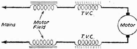
Fig. 1.—Simple form of suppressor.
