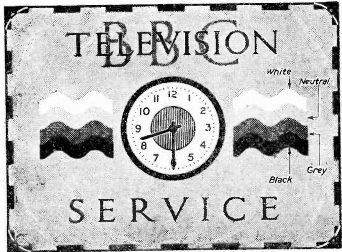
Fig. 3.—Details of the tuning signal.
