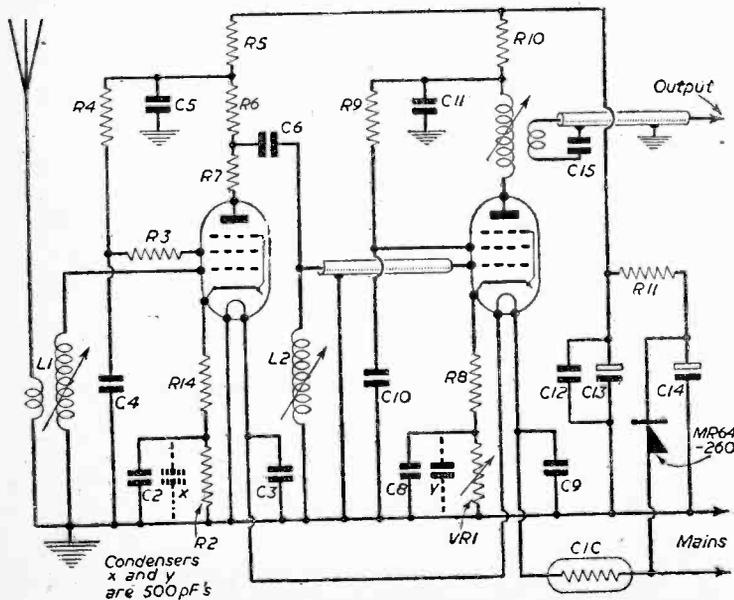
Fig. 8.—Circuit of the two-stage pre-amplifier.
