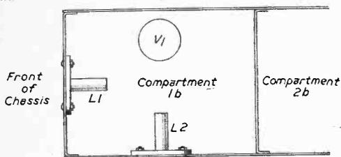
Fig. 9.—Mounting position for L2.
