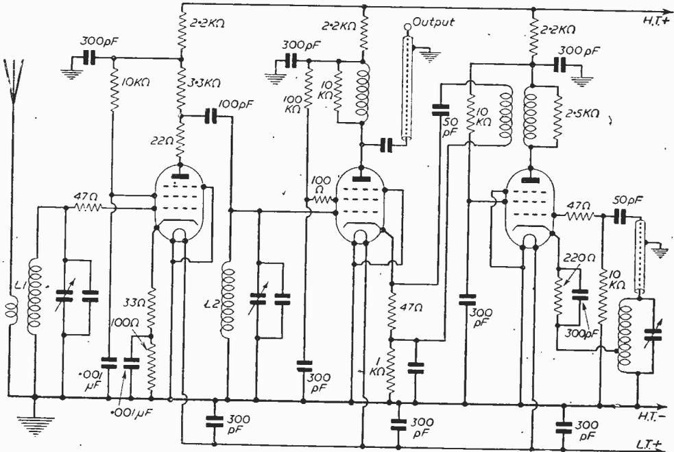
Fig. 10.—Circuit of a superhet converter.
