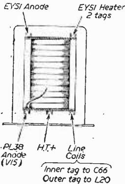
Fig. 11.—Line output transformer wiring.
