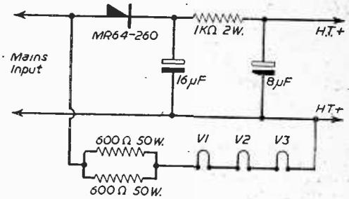
Fig. 12.—Modified circuit for A.C./D.C. use.
