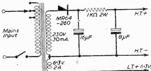
Fig. 11.—Theoretical circuit of the power unit.
