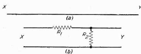
Fig. 1.—Diagram illustrating characteristic resistance of lines.
