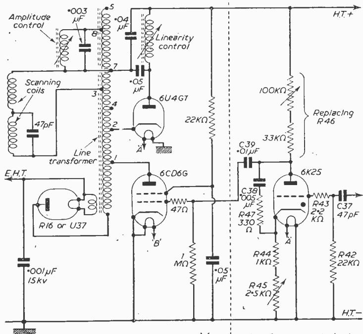
Fig. 2.—Circuit of the line timebase.
