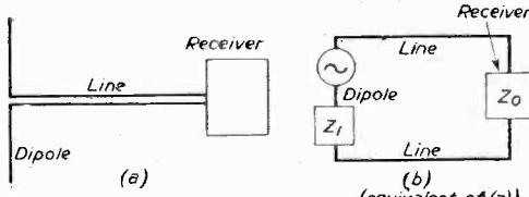
Fig. 9.—Normal television aerial feed and its equivalent circuit.
