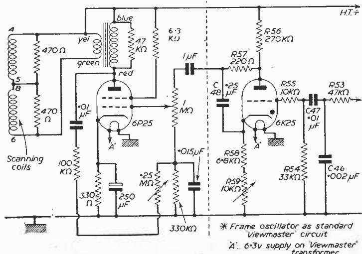
Fig. 4.—Circuit of the frame timebase.
