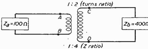
Fig. 10.—Effect of a transformer on the total impedance of a circuit.
