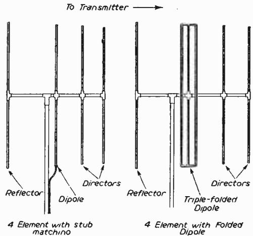
Fig. 9.—For fringe area reception aerials of this type are necessary.
