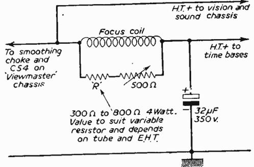
Fig. 5.—Details of the electromagnetic focus circuit.
