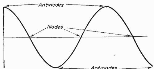
Fig. 12.—Nodes and antinodes in a standing wave.
