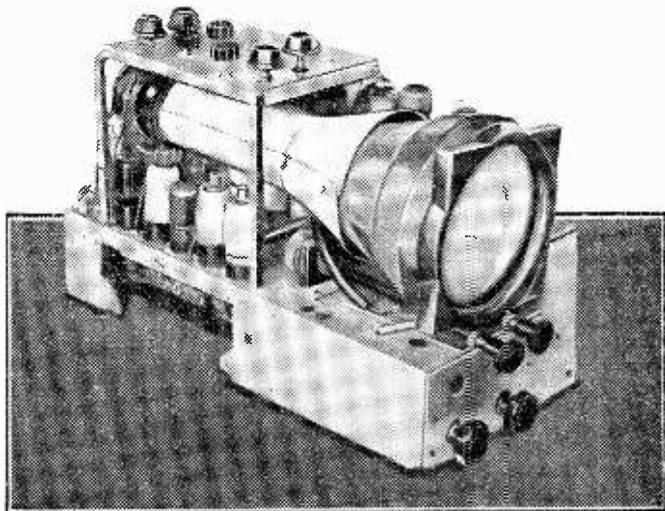
A typical converted ex-service unit complete with tube. This is the £9 television using a Type 62 unit.
