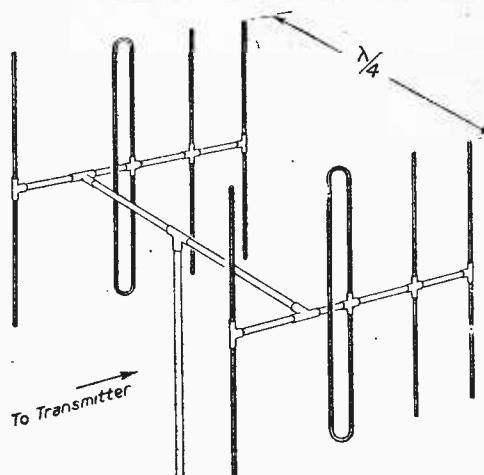
Fig. 10.—For areas of very weak signal strength an elaborate array of this type is not only desirable, but in many cases essential.
