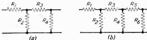
Fig. 2.—Rearrangement of line characteristic resistances.
