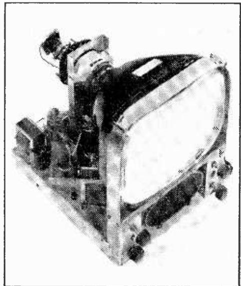
The use of elliptical speaker and rectangular tube enables the overall size of the receiver to be kept down.
