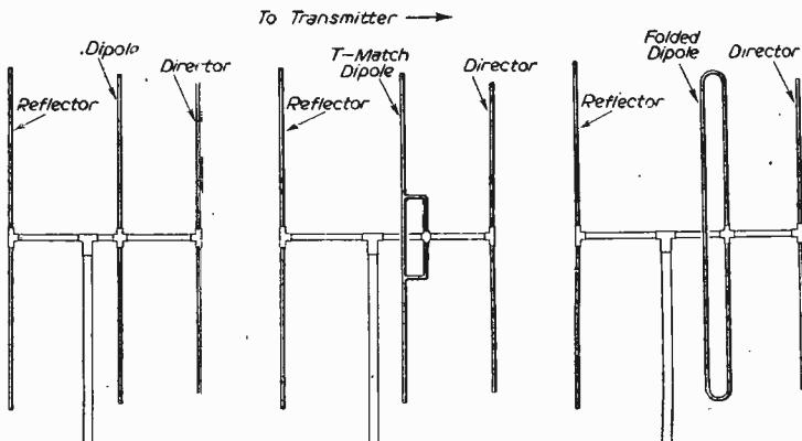
Fig. 8.—Three different forms of multi-array aerial for remoter districts.
