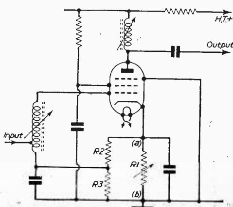
Fig. 2.—A typical contrast control circuit.
