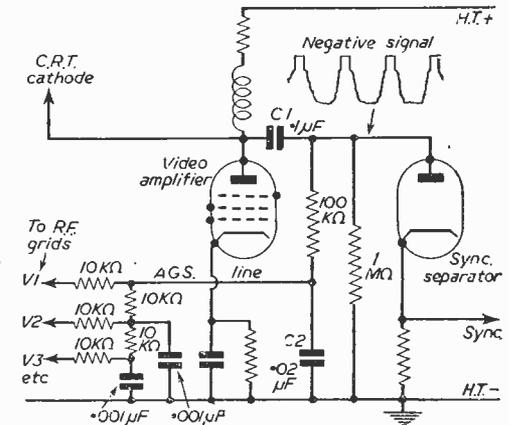
Fig. 1.—Conventional diode sync separator.
