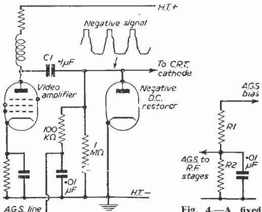
Fig. 3.—One method of obtaining A.V.C. from a restorer diode.
