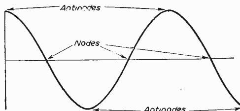
Fig. 12.—Nodes and antinodes in a standing wave.
