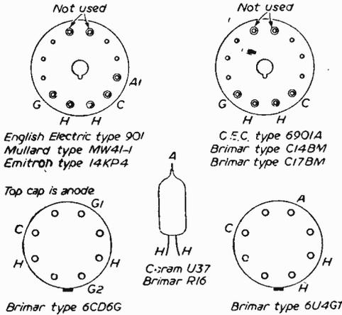
Fig. 3.—Valve base connections.
