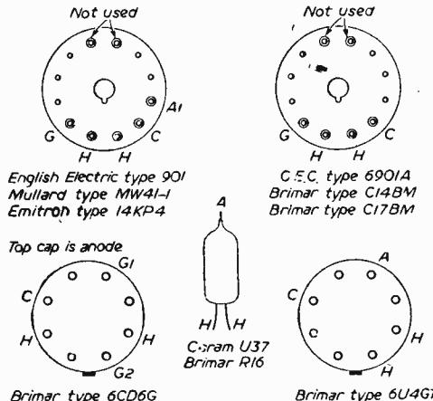
Fig. 3.—Valve base connections.
