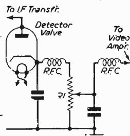
Fig. 4.—A rather unusual contrast control circuit by G.E.C. This resembles the ordinary A.F. volume control.
