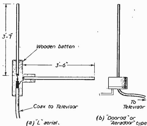
Fig. 2.—Two very simple forms of indoor aerial for areas close to the transmitter.
