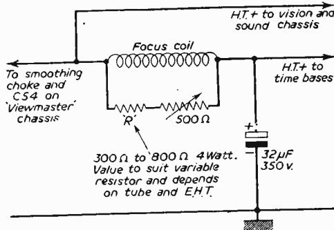
Fig. 5.—Details of the electromagnetic focus circuit.
