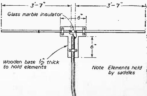
Fig. 6.—Constructional details of a dipole.
