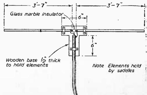
Fig. 6.—Constructional details of a dipole.
