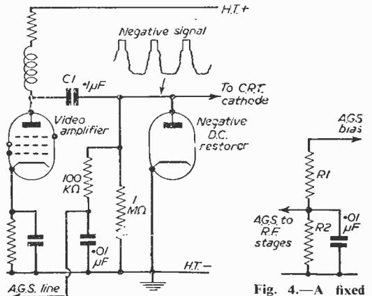
Fig. 3.—One method of obtaining A.V.C. from a restorer diode.
