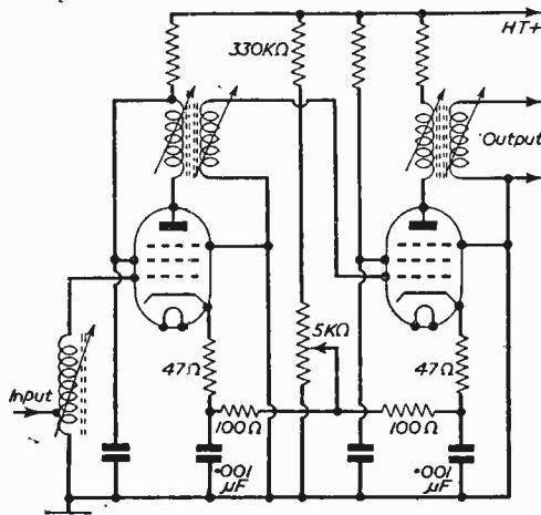
Fig. 3.—A circuit by G.E.C. showing how two stages can be controlled by a single potentiometer. The valves used are Z77's.
