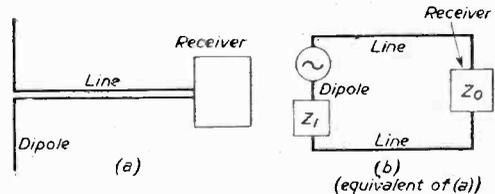
Fig. 9.—Normal television aerial feed and its equivalent circuit.
