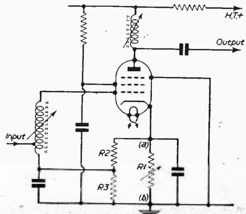
Fig. 2.—A typical contrast control circuit.
