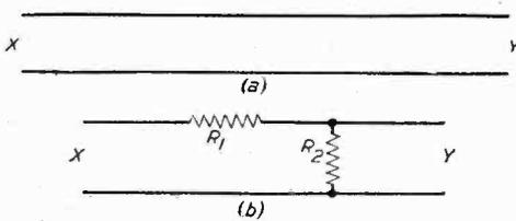
Fig. 1.—Diagram illustrating characteristic resistance of lines.
