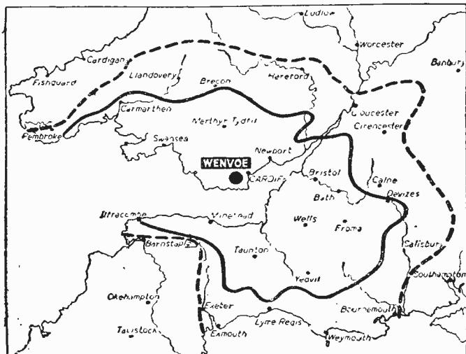
Fig. 1.—The Service area as plotted by the BBC. It may, of course, subsequently be found that results will differ slightly in certain districts, but the map may be taken as a reliable guide in planning the type of aerial which may be required.
