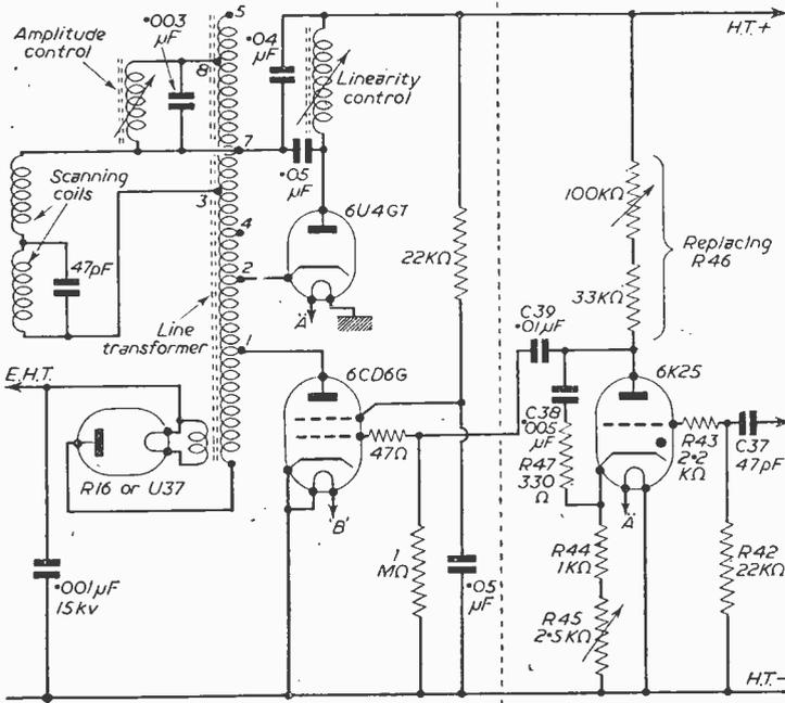
Heater supply for Line Amplifier 'B' to be taken from separate heater transformer to give 6.3V. at 2.5A. Line Oscillator as 'Viewmaster' circuit
