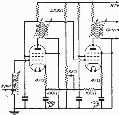
Fig. 3.—A circuit by G.E.C. showing how two stages can be controlled by a single potentiometer. The valves used are 2Z17's.
