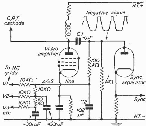
Fig. 1.—Conventional diode sync separator.
