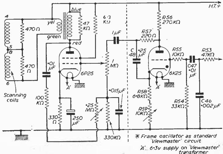
Fig. 4.—Circuit of the frame timebase.
