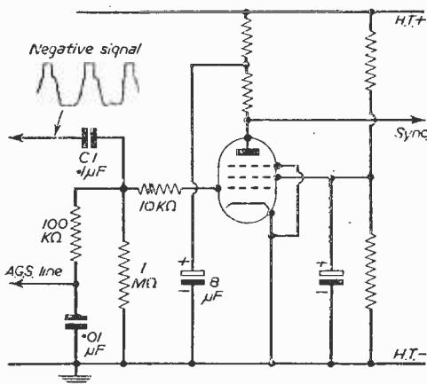
Fig. 2.—Modified saturated pentode sync separator.
