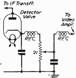
Fig. 4.—A rather unusual contrast control circuit by G.E.C. This resembles the ordinary A.F. volume control.
