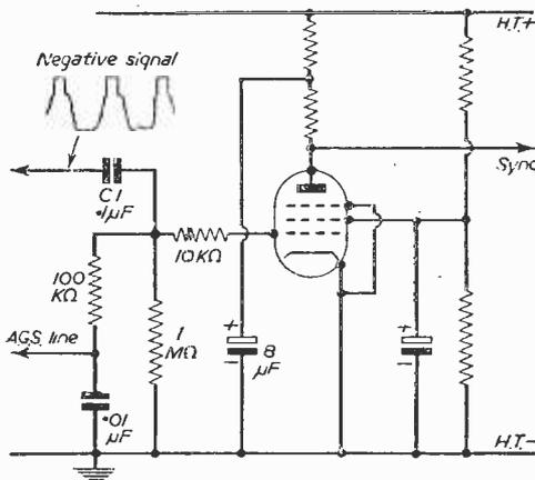
Fig. 2.—Modified saturated pentode sync separator.
