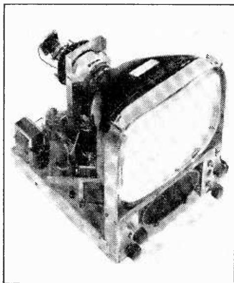
The use of elliptical speaker and rectangular tube enables the overall size of the receiver to be kept down.
