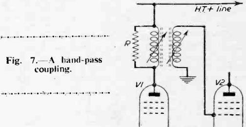
Fig. 7.—A hand-pass coupling.
