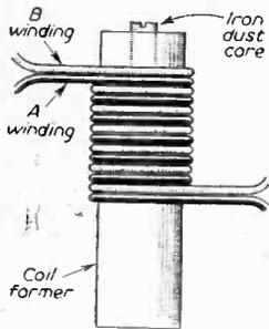
Fig. 3.—Details of a coil wound on the Bifilar principle.
