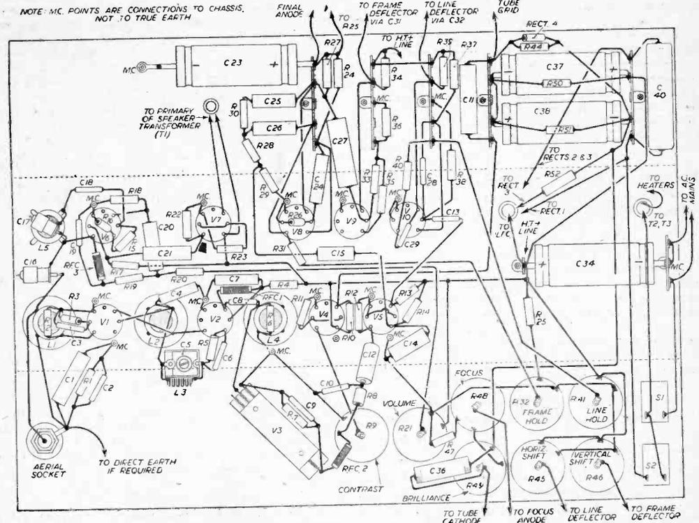
Fig. 8.—Under-chassis wiring.
