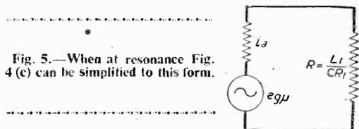
Fig. 5.—When at resonance Fig. 4(c) can be simplified to this form.
