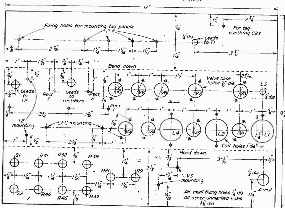
Fig. 4.—Chassis drilling diagram.
