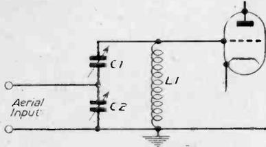
Fig. 3.—Stabilising arrangement for the grid circuit.
