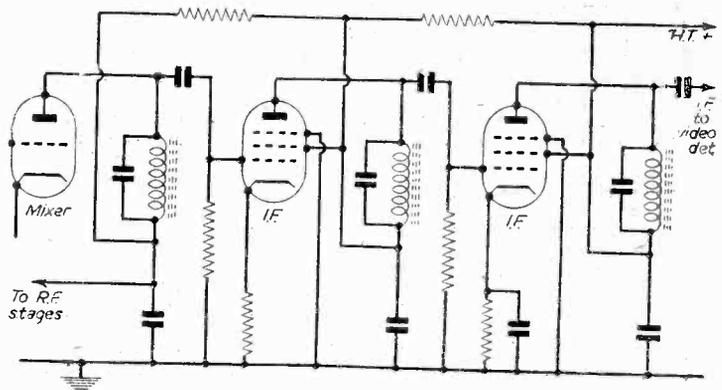
Fig. 1.—Basic single tuned stagger type amplifier.
