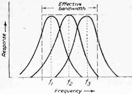
Fig. 6.—Illustrating how any desired pass-band may be obtained by the use of stagger-tuning.
