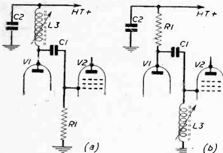
Fig. 4.—Showing at (a) a tuned anode circuit, at (b) a tuned grid circuit, and provided C1 has negligible impedance at the operating frequency, both circuits are equivalent as shown in simplified form at (c).
