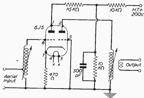
Fig. 1.—A simple grounded-grid amplifier circuit.
