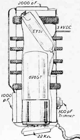
E.H.T. Coil with 6V6GT and EY51 inside coil (other components mounted outside)
