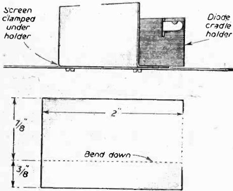
Fig. 7.—The detector screen.
