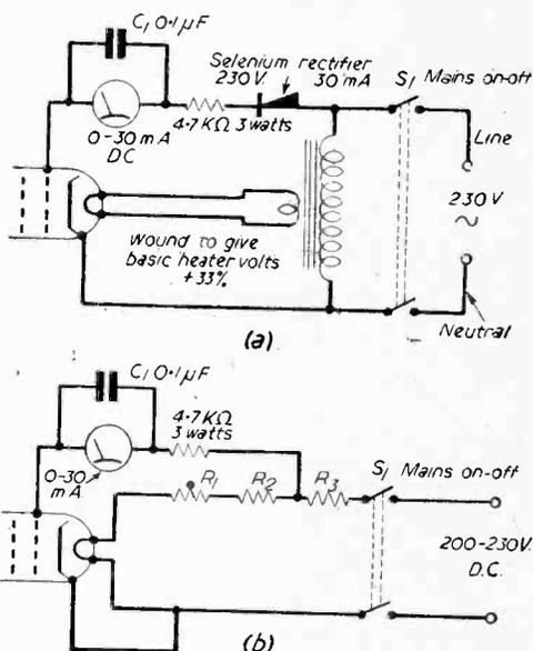
Fig. 4 (a).—Rejuvenator for A.C. supplies. (b) for D.C. supplies. Here, for 0.3A tubes R1 = CZ6 Brimistor, and R2, 3 are 260  $\Omega$  50 W each. For 0.6 A tubes R1 = CZ4 Brimistor and R2, 3 are 130 $\Omega$  90 W each.
