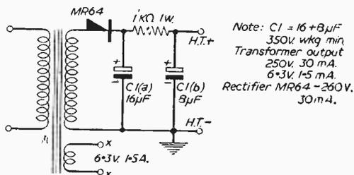
Fig. 2.—Power supply for an additional stage.
