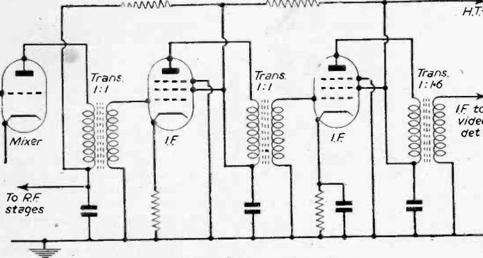
Fig. 2.—Basic Bifilar amplifier circuit.
