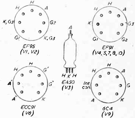
Fig. 9.—Valve-base data.
