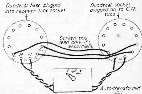
Fig. 3.—Typical arrangement of brightener unit.
