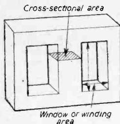
Fig. 2.—Transformer core showing the cross-sectional area and window.
