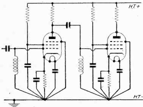
Fig. 4.—Common earthing points aid efficiency.
