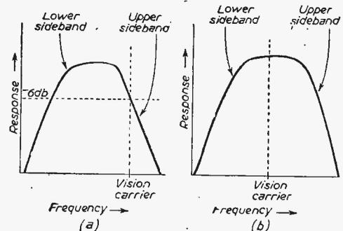
Fig. 12.—The characteristics of the vision transmissions at (a) single sideband (channels 2 to 5), at (b) double sideband (channel 1 only).
