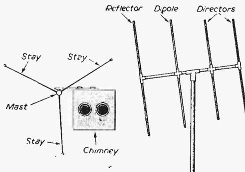
Fig. 1.—Strengthening a mast by 3 stays.
