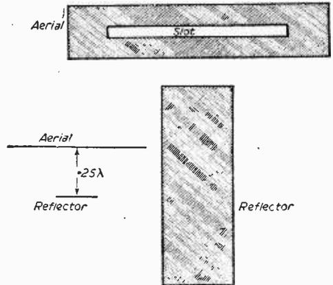
Fig. 4.—The "slot" aerial—made from wire netting.
