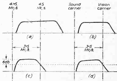
Fig. 1.—Showing the frequency characteristics of channel 1 at (a) and other channels at (b), while (c) and (d) show the receiver response for single sideband working.
