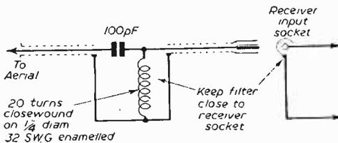
Fig. 1.—A simple high-pass filter.
