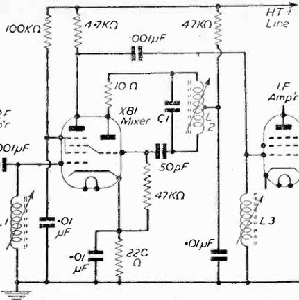
Fig. 13.—A frequency changer circuit styled round a triode-hexode valve.
