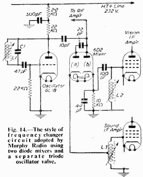
Fig. 14.—The style of frequency changer circuit adopted by Murphy Radio using two diode mixers and a separate triode oscillator valve.
