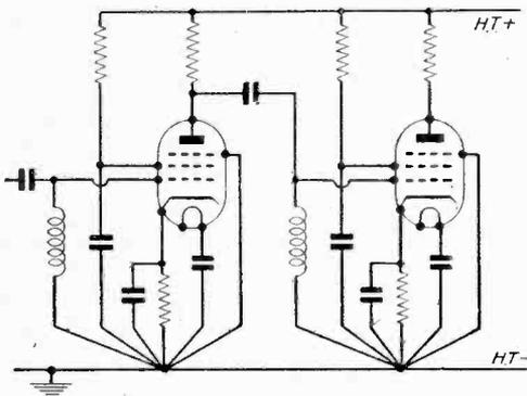
Fig. 4.—Common earthing points aid efficiency.
