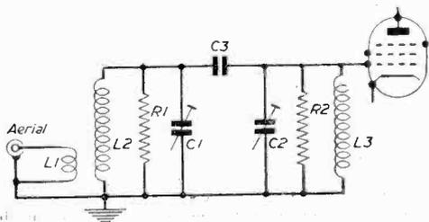
Fig. 1.—Typical H.F. stage.
