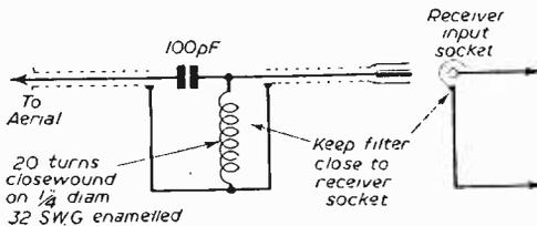
Fig. 1.—A simple high-pass filter.
