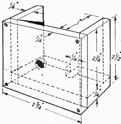
Fig. 10.—A form of junction box made of wood or paxolin.
