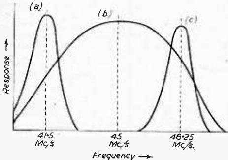
Fig. 11.—A vision channel response without rejection at (b) embraces the accompanying and adjacent sound signals at (a) and (c) respectively.
