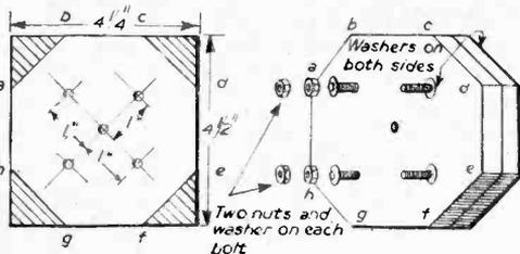
Fig. 1 (left).—Diagonals are drawn and 1 in. corners cut off. Fig. 2 (right).—Four bolts are added to accommodate two nuts.
