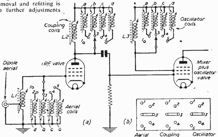
Fig. 3.—A five-channel conversion system by Pilot Radio.
