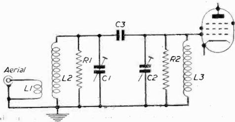
Fig. 1.—Typical H.F. stage.
