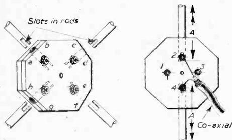
Fig. 3 (left).—Holes are drilled from corner edges in direction of diagonals. Fig. 4 (right).—Shows the dipole.
