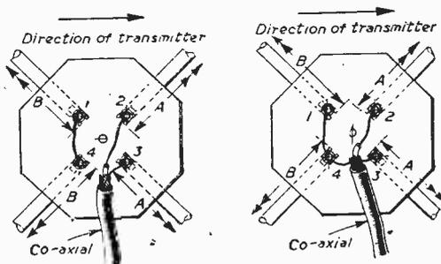
Fig. 7 (left).—"X" aerial. Fig. 8 (right).—Type 2 connection.
