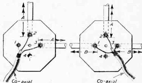
Fig. 5 (left).—Vee or L aerial. Fig. 6 (right).—Inverted "Tee" aerial.
