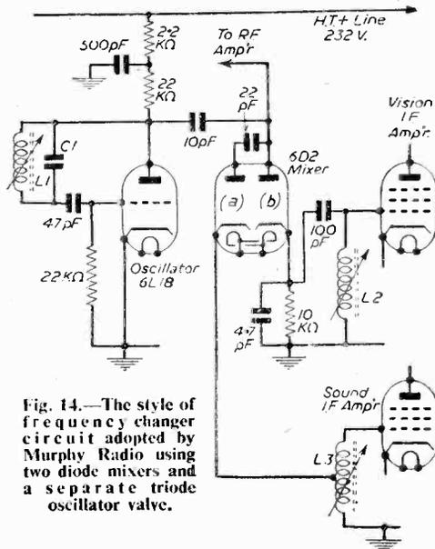
Fig. 14.—The style of frequency changer circuit adopted by Murphy Radio using two diode mixers and a separate triode oscillator valve.
