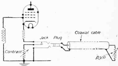
Fig. 5.—Remote control can be fitted as shown here.
