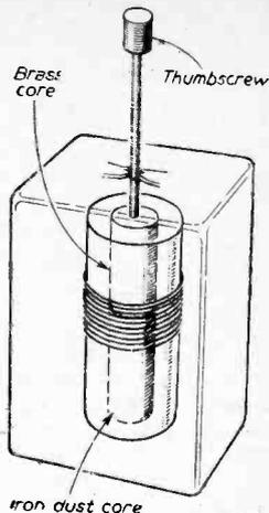
Fig. 5.—The coil construction used in Cosmor receivers.
