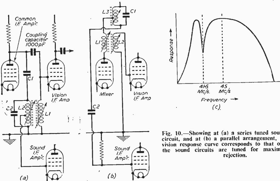
Fig. 10.—Showing at (a) a series tuned sound pick-up circuit, and at (b) a parallel arrangement, the overall vision response curve corresponds to that of (c) when the sound circuits are tuned for maximum sound rejection.
