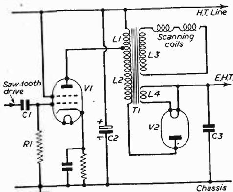
Fig. 1.—A typical line output circuit.
