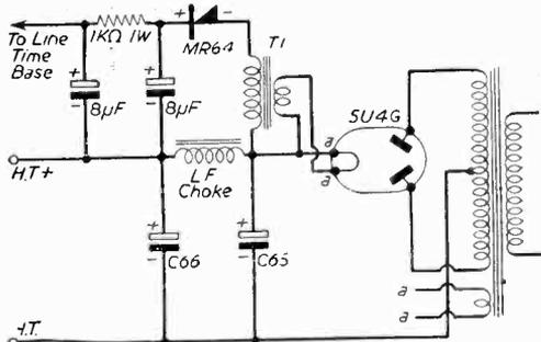
Fig. 2.—Modified H.T. boost circuit.
