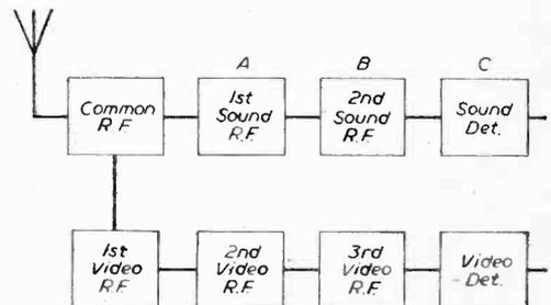
Fig. 3.—Typical block diagram of a modern television superhet set.
