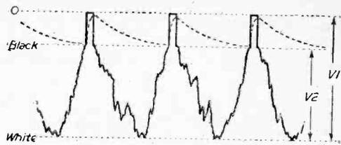
Fig. 2.—Waveform at video amplifier anode.
