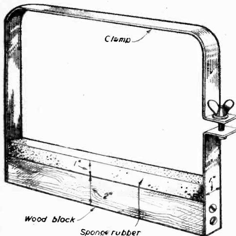
Fig. 2.—Ideal mounting arrangement for rectangular tubes.
