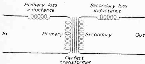
Fig. 4.—Showing how the loss inductance is included when considering a practical transformer.
