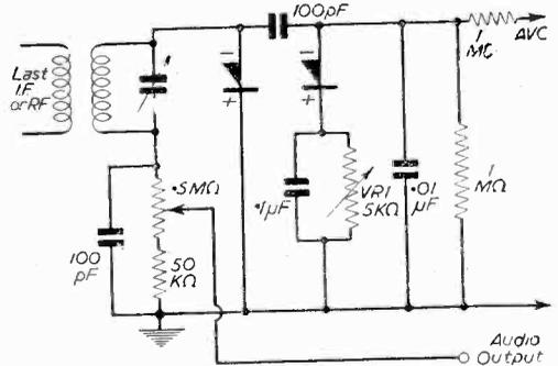
FIG. 6.—In this circuit A.V.C. is obtained as well as rectification.
