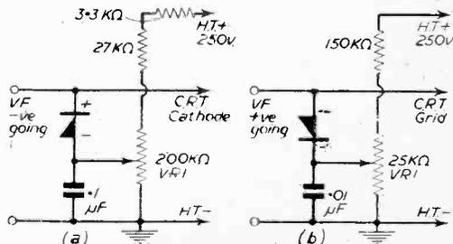
Fig. 3.—Vision interference circuits using the diode.
