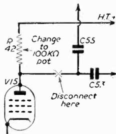
Fig. 4.—Modification to V15.
