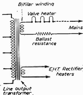
Fig. 6.—The inclusion of a bifilar winding to minimise valve failure.
