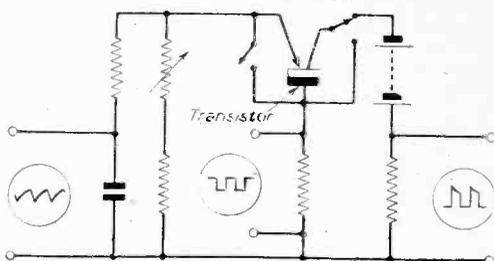
Fig. 10.—The transistor, or crystal triode, in an American experimental circuit.
