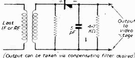
Fig. 2.—Typical vision detector circuit.
