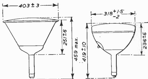
Fig. 1.—Main dimensions of the most popular rectangular tube (right) and the all-metal (left).
