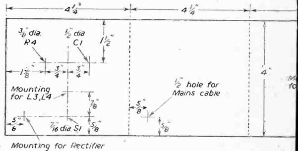
Fig. 4.—Chassis cutting and bend
