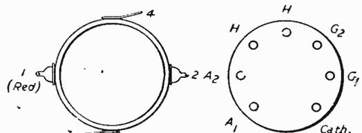
Fig. 6.—Details of coil and valve connections.
