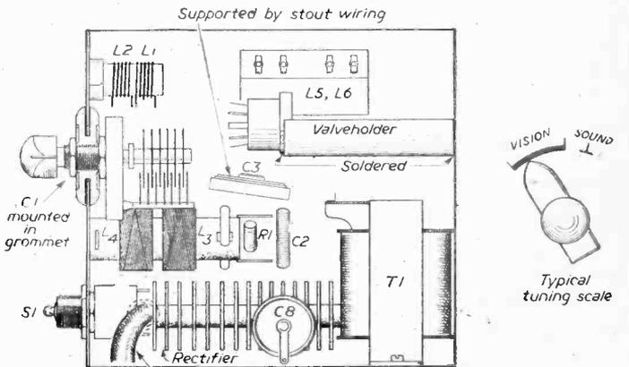
Fig. 3.—Wiring details, and the tuning control.
