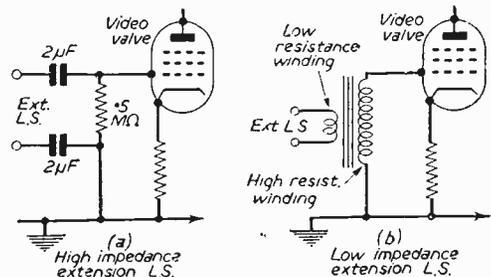
Fig. 1.—Checking the input to the video stage.
