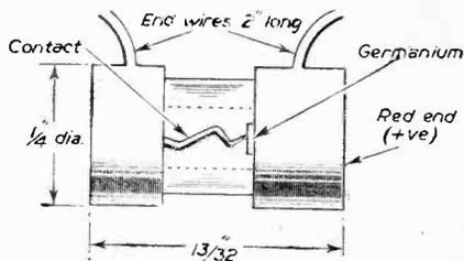
Fig. 1.—General details of construction of the B.T.H. pattern Germanium crystal diode.
