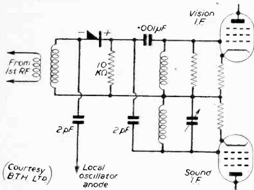
Fig. 9.—The customary mixer valve is replaced in this frequency changer circuit by a diode.
