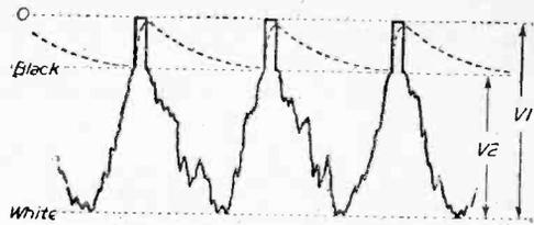
Fig. 2.—Waveform at video amplifier anode.
