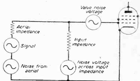
Fig. 16.—Showing in simplified form how the various noise voltages are distributed in the first stage input circuit.
