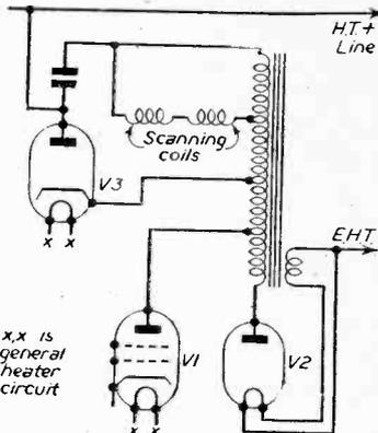
Fig. 5.—A basic line output stage circuit showing the auto-transformer principle.
