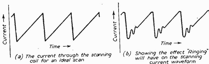
Fig. 2.—Waveforms in the line circuit.
