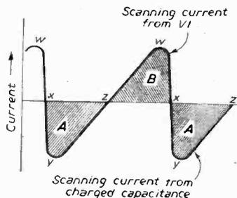
(b) Illustrating the principle of the reclaim circuit
