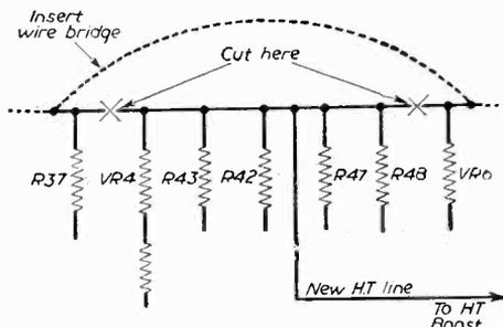
Fig. 3.—Method of connecting boost circuit to line amplifier.
