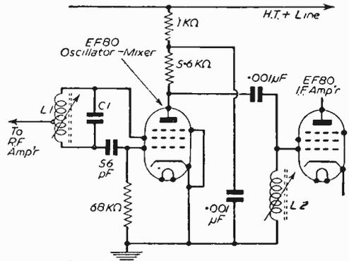
Fig. 15.—A typical frequency changer system of the modern receiver.
