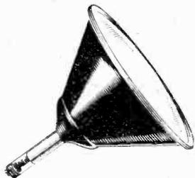
*Magnetic focus and deflection (70° angle). Almost flat face-plate. Wide angle scanning. Wide contrast range. Picture focussing over whole of screen area. Fitted ion trap. Length 17.11/16".*
