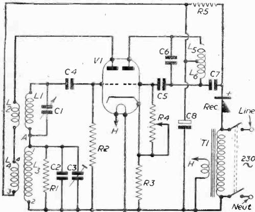
Fig. 1.—Theoretical circuit of the Telesquare.
