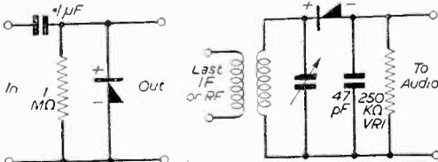
FIGS. 4 and 5.—Typical D.C. restorer and sound detector circuits.
