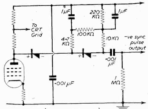
FIG. 8.—A sync separator circuit using two diodes.
