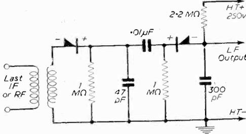
FIG. 7.—Interference limiting and sound detection are shown here.
