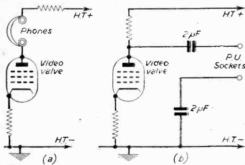
Fig. 2.—Checking the output from the video stage.
