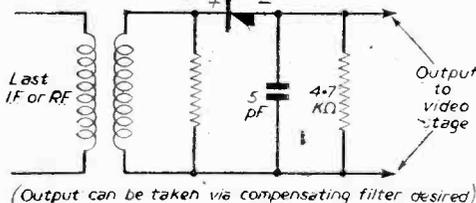
Fig. 2.—Typical vision detector circuit.
