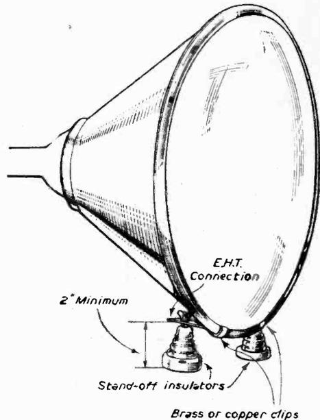
Fig. 3.—Metal tubes are best mounted as shown here.
