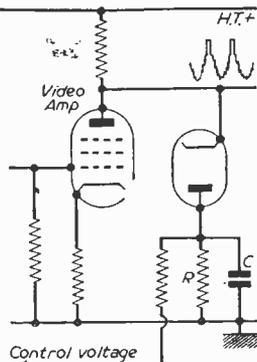
Fig. 1.—A simple circuit for A.C.C.
