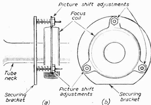
Fig. 1.—Illustrating a method of focus-coil mounting.
