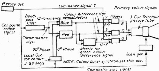
Fig. 5.—Block diagram of the receiver colour circuits. All sections of the receiver in front of the colour unit are conventional.
