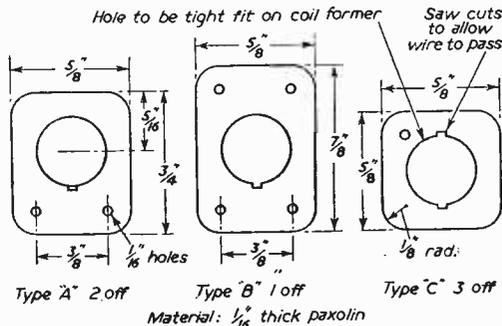
Fig. 4.—Details of paxolin washers.
