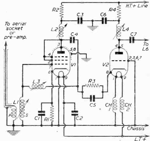
Fig. 4.—The first two R.F. stages.
