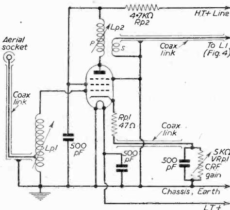
Fig. 3.—The pre-amplifier stage. Coil-winding data will be given next month.
