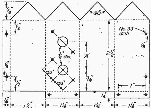
Note: Dimension 'A' is 1" for 1st IFT, and 1 5/8" for 2nd IFT. Omit bottom coil fixing holes in L1 coil can
