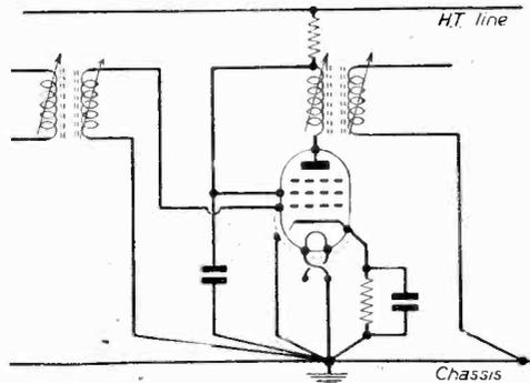
Fig. 4.—Single-point wiring is carried out as shown here.
