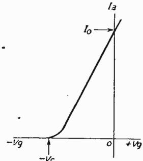
Fig. 2.—This is the operating characteristic of the triode mixer section.
