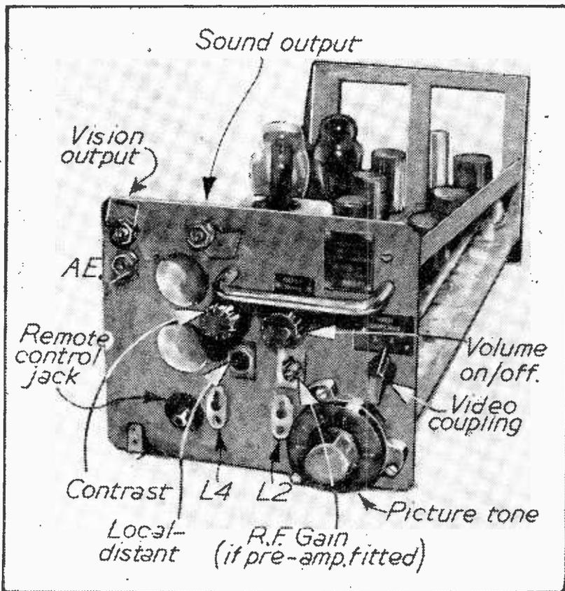
Fig. 2.—View of the front panel with all items identified.
