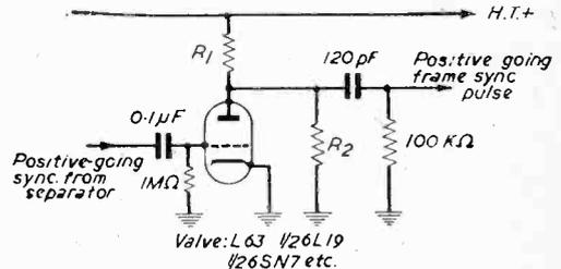
Fig. 8.—Positive pulse producing interlace stage. R1 and R2 depend on valve used.
