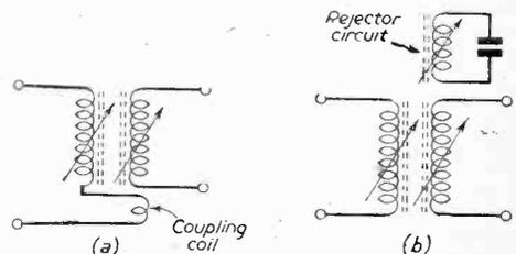
Fig. 3.—(a) Band-pass coupling with separate coupling coil, and (b) coupled rejector circuit.
