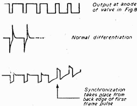
Fig. 9.—Frame pulses in which the back instead of the leading edge is used.
