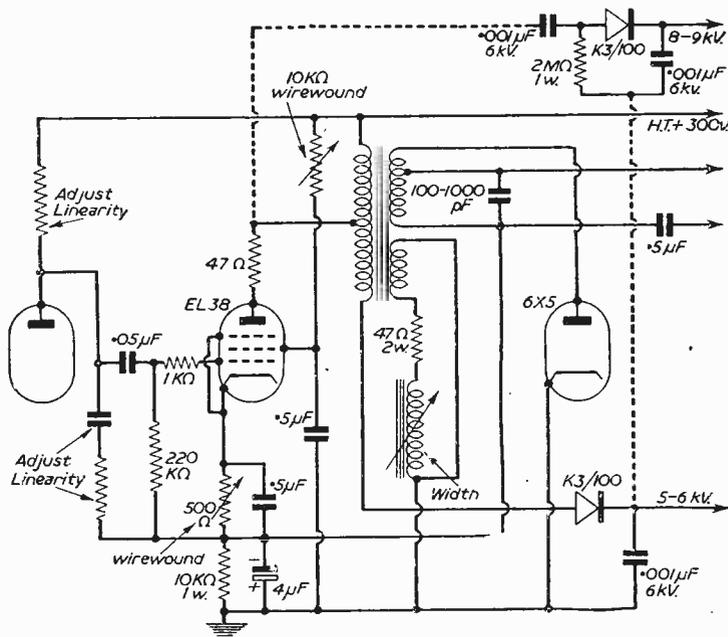
Fig. 2.—Line tunebase with efficiency diode, showing various controls which are required.
