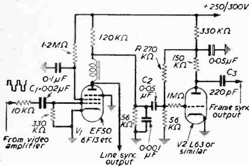
Fig. 5.—Sync separator and triode interlace valve.
