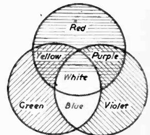
Fig. 6.—Colour combinations produced by blending coloured lights. This is known as *additive mixing*.
