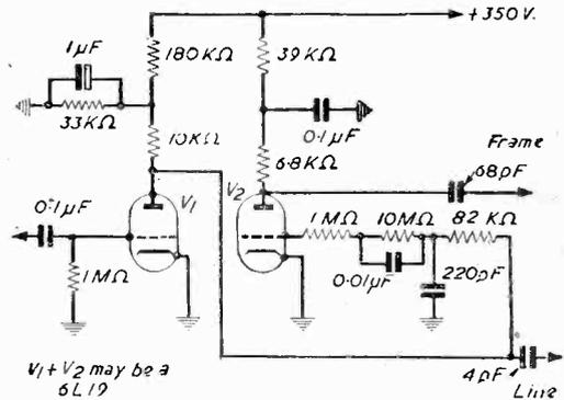
Fig. 10.—Two triodes are used in this positive pulse circuit.
