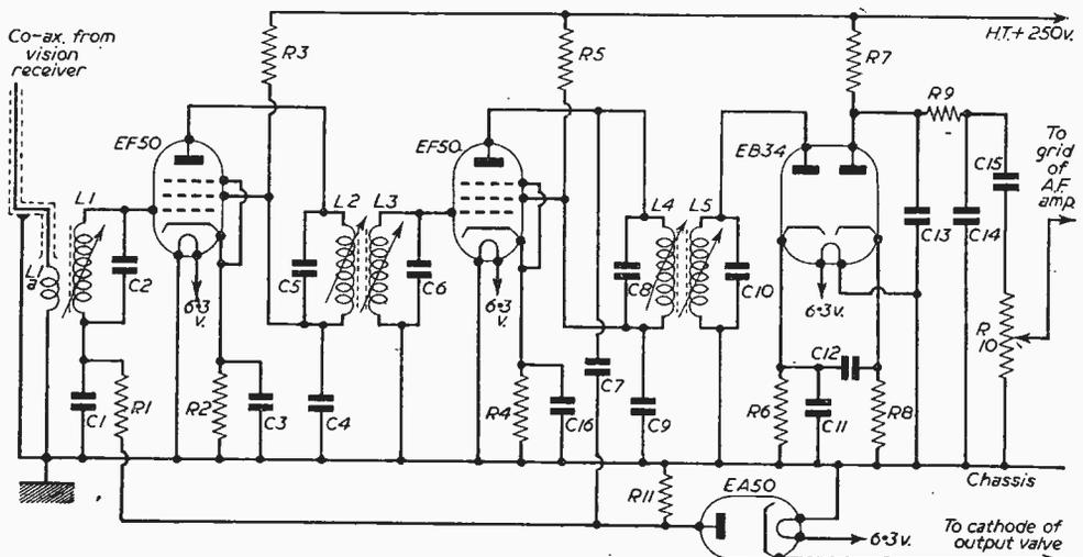
Fig. 1.—Suggested circuit for use with the I.F. transformers.
