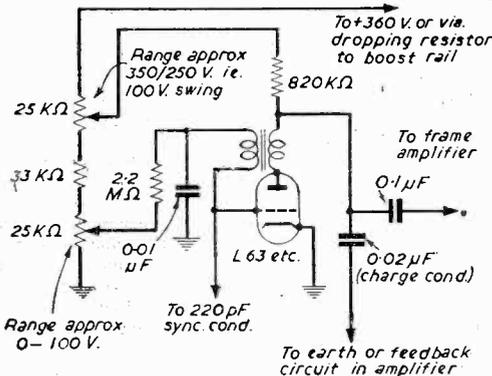
Fig. 7.—Frame blocking oscillator for use with sync circuit of Fig. 5.
