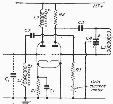
Fig. 1.—The basic double-triode mixer circuit from which design values are calculated.
