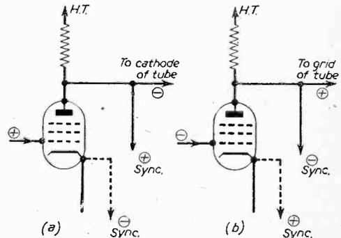
Fig. 2.—The output from the Video stage can be of either polarity, and the tube must be correctly connected.
