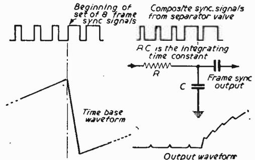
Figs. 3 & 4.—Frame pulses and waveform from sync separator.
