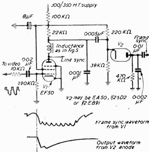
Figs. 11 & 12.—A circuit for producing a negative pulse and the waveforms associated with it.
