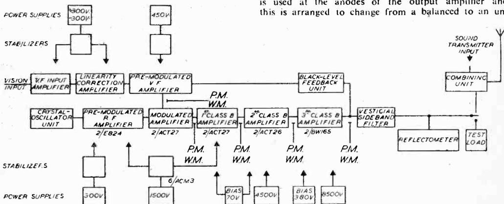
Fig. 1.—Block diagram of the essential units of the new transmitter.
