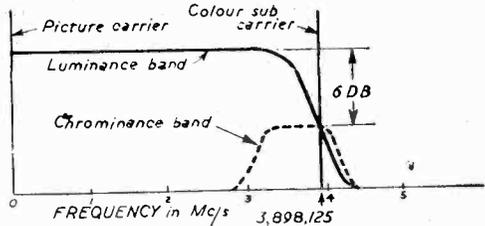
Fig. 3.—Relative positions of the picture carrier and the colour sub-carrier in the upper sideband of transmitted signal. The vestigial lower side-band and the sound carrier have been omitted.
