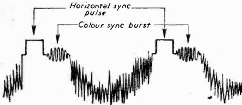
Fig. 4.—Colour-sync bursts consisting of nine cycles of the 3.898125-sub-carrier are sent on the unused "back porch" of each regular horizontal sync pulse.
