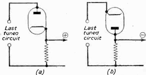
Fig. 1.—The Video detector can produce a positive or negative signal as shown here.
