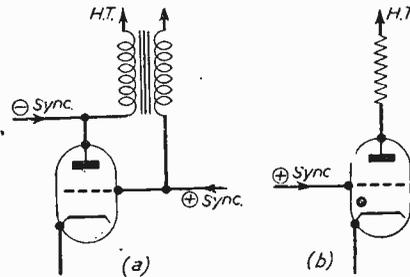
Fig. 3.—The sync pulses are applied to different electrodes, according to their polarity.
