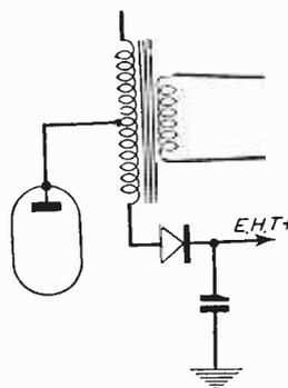
Fig. 1.—The usual circuit of an E.H.T. supply from the line output stage.
