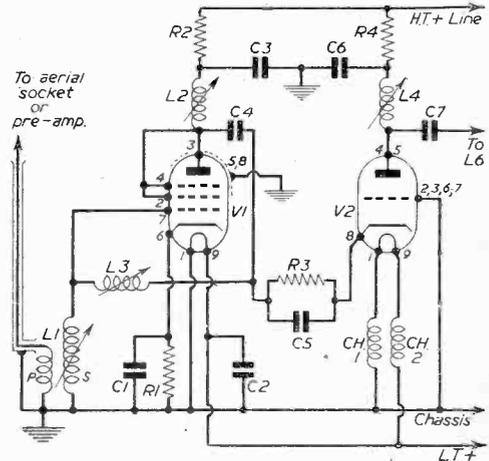
Fig. 4.—The first two R.F. stages.
