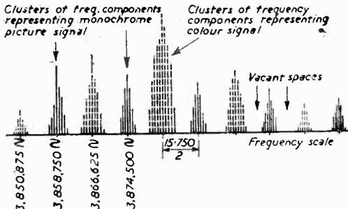
Fig. 1.—Black-and-white TV signal side-bands form clusters, separated by 15,750-cycle gaps. NTSC colour-TV system uses these blank spots to send colour signals.
