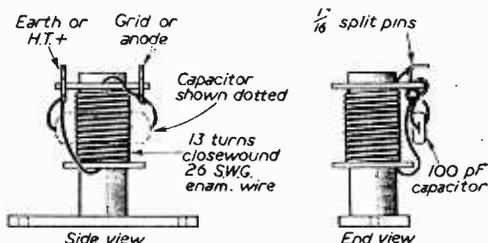
Fig. 3a (left).—Three views of the sound input coil. 3b (above).—Two views of L2-5 inclusive.
