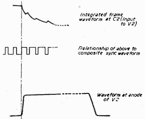
Fig. 6.—Frame pulse as integrated by the Fig. 5 circuit.
