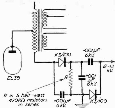
Fig. 3.—In this circuit the same two metal rectifiers are employed as a voltage doubler.
