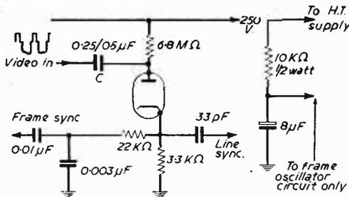
Fig. 1 (left).—Condenser C in this circuit must be of high quality. Fig 2 (right).—Additional decoupling circuit.
