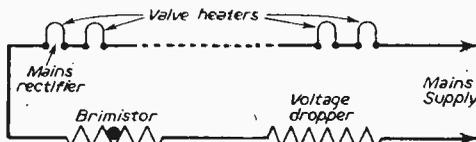
Fig. 4.—Showing how a Brimistor should be included in the heater chain.
