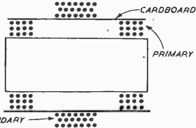
Fig. 4.—Details of the position of the secondary winding.
