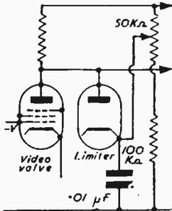
Fig. 3.—Circuit of a manually-set noise limiter for a vision receiver.
