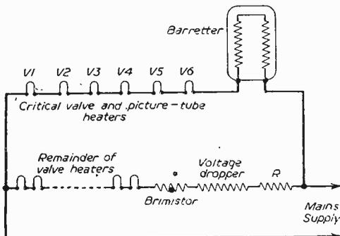
Fig. 5.—A method of counteracting mains voltage fluctuations.
