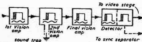
Fig. 5.—Block diagram of the vision R.F. section.
