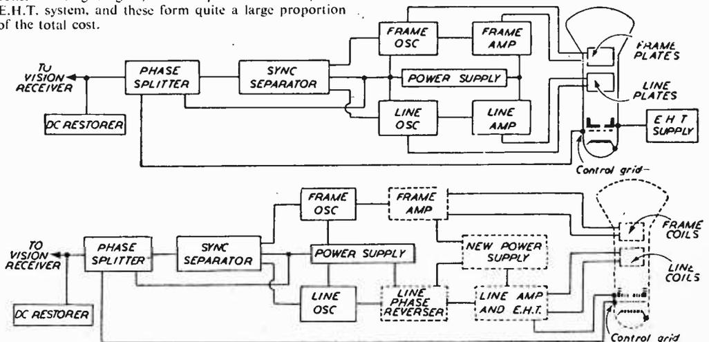
Fig. 1 (a) (above).—A standard electrostatic timebase, and below (Fig. 1 (b)), an electromagnetic arrangement.
