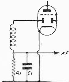
Fig. 1.—Load and filter elements of standard form.
