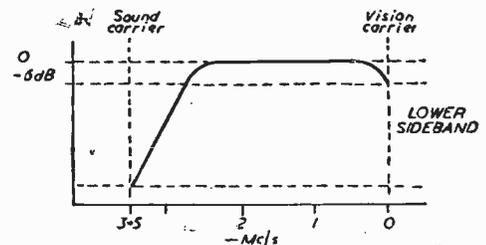
Fig. 2.—Response curve of a single sideband receiver.
