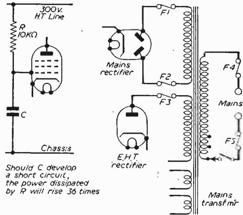
Should C develop a short circuit, the power dissipated by R will rise 36 times
