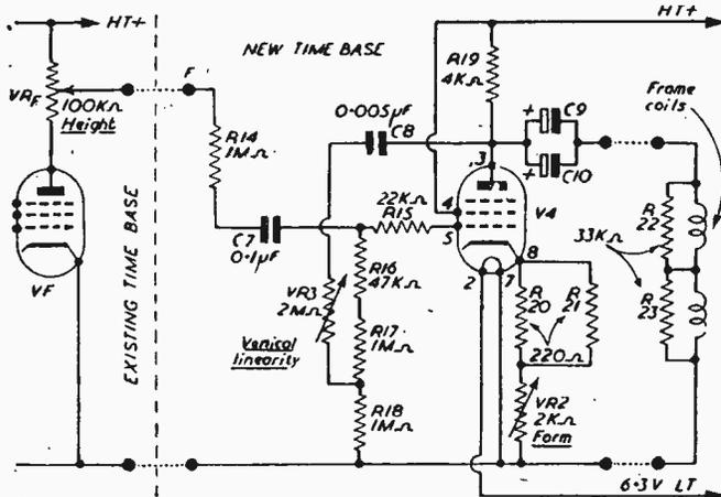
Fig. 2.—A frame timebase amplifier.
