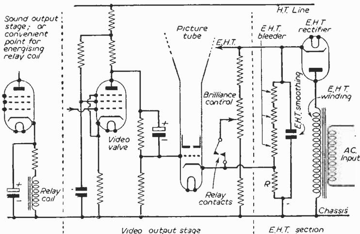
Fig. 1.—A picture-tube protection arrangement—for grid modulation.
