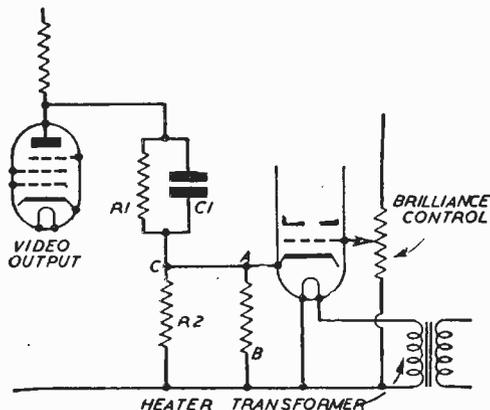
Fig. 1.—Circuit diagram illustrating the effect of the heater-cathode short-circuit on the video stage.
