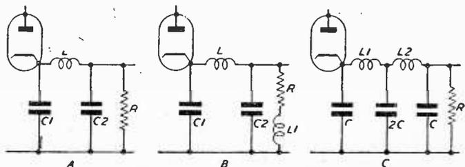
Fig. 2.—Networks as found in general types of television detector stages
