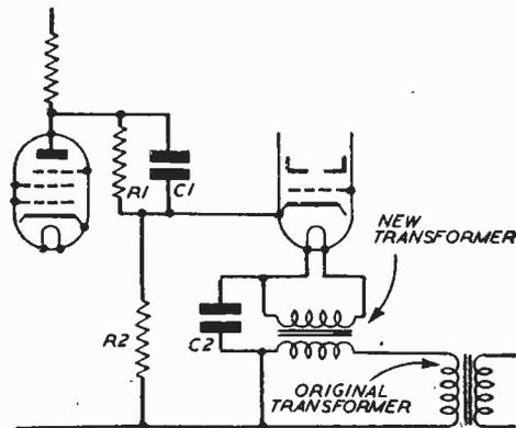
Fig. 2.— $C_2$  short-circuits the video signal here.
