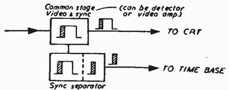
Fig. 8.—Illustrating the special requirements of the tube and sync stages.
