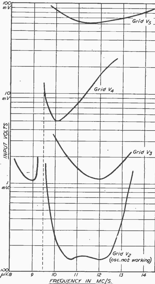
Fig. 2.—Response curves of vision I.F. stages.
