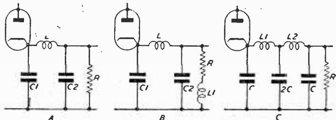
Fig. 2.—Networks as found in general types of television detector stages
