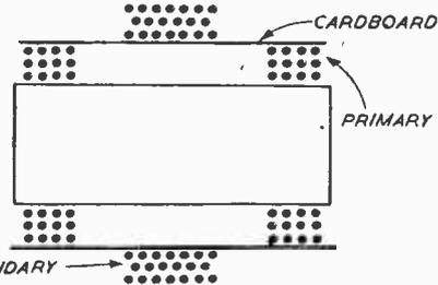
Fig. 4.—Details of the position of the secondary winding.
