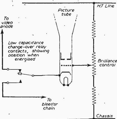
Fig. 2.—Showing how relay contacts should be modified for cathode modulated tubes.
