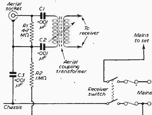
Fig. 8.—Showing a static discharge aerial circuit for A.C./D.C. style receivers.
