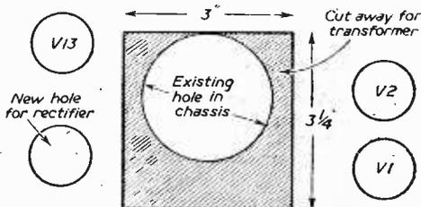
Fig. 15.—Cut-out to accommodate mains transformer.
