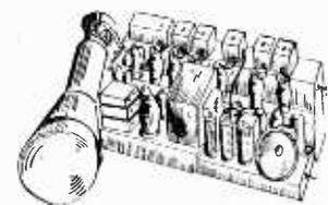
The now famous "New 1355 Conversion" enables you to construct a remarkably compact, self-contained television: Sound, Vision, Time bases, Speaker and power pack on one 1353 chassis—without the use of any expensive RF units. Data for all channels, 2/6 (2d. post). We can supply 1355 receivers, in original makers' cases, complete with 11 valves, 45/- Loose stored, 30/-.
