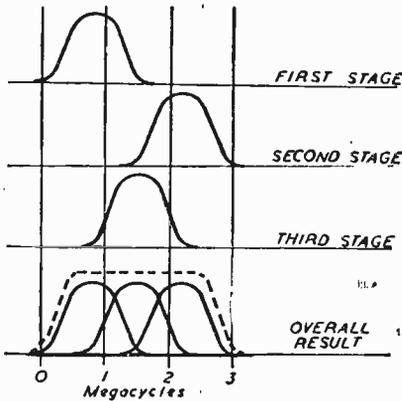
Fig. 7.—Diagram illustrating the effects of stagger tuning.
