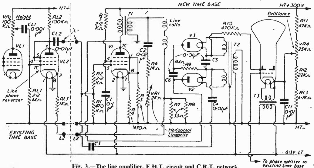
Fig. 3.—The line amplifier, E.H.T. circuit and C.R.T. network.
