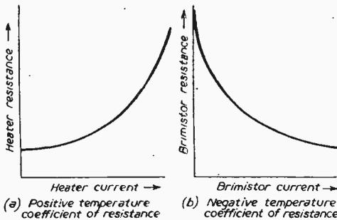
Fig. 3 (a).—A positive temperature coefficient of resistance. (b) A negative temperature coefficient of resistance.
