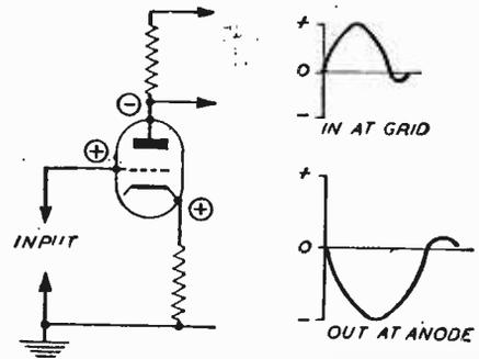
Fig. 10.—A video stage showing the reversed signals in anode and cathode circuits.
