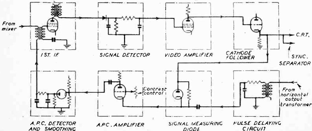
Simplified diagram of the arrangement incorporated in the new Pye receivers.
