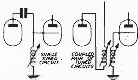
Fig. 6.—A single circuit and a coupled tuner.
