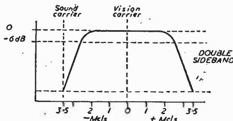
Fig. 1.—Response curve of a double sideband receiver.
