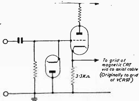
Fig. 4.—A typical phase-splitter as used in the VCR97 timebase.
