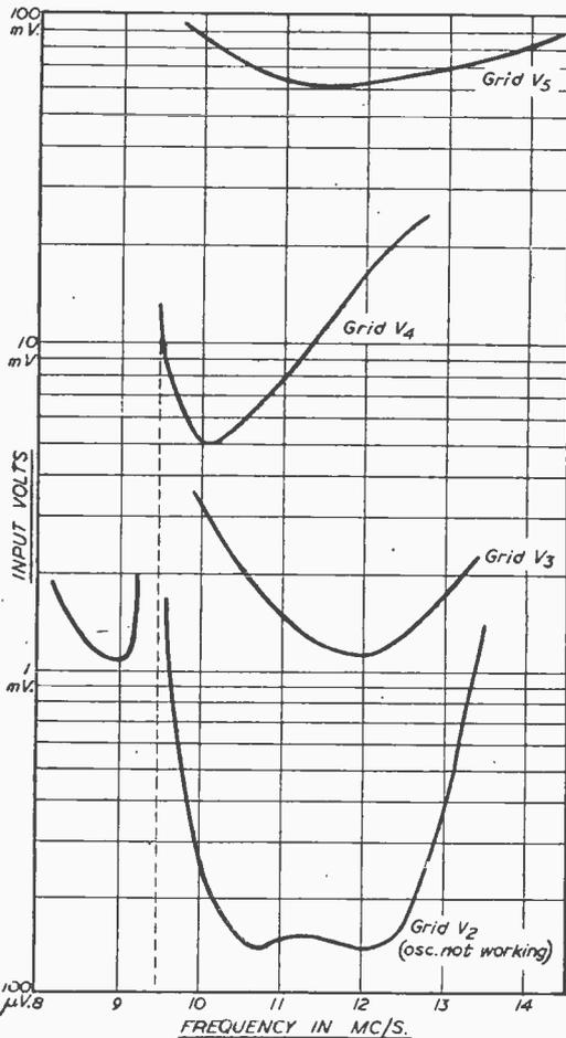
Fig. 2.—Response curves of vision I.F. stages.
