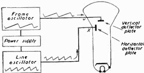
Fig. 15.—Basic deflection circuit.
