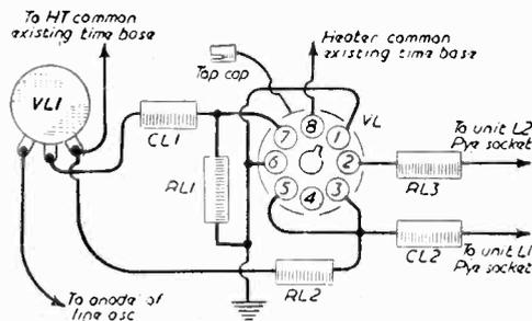
Fig. 13.—Wiring diagram of line phase-reversing circuit.
