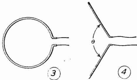
Figs. 3 and 4.—A circular and a "V" aerial. The angle  $\theta$  may be varied to find the most suitable one for the receiver and locality.
