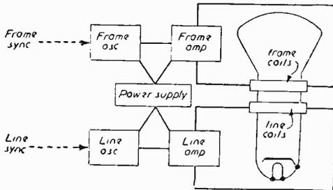
Fig. 17.—Schematic electro-magnetic deflection arrangement.
