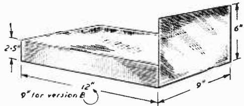
Fig. 9.—Chassis dimensions.
