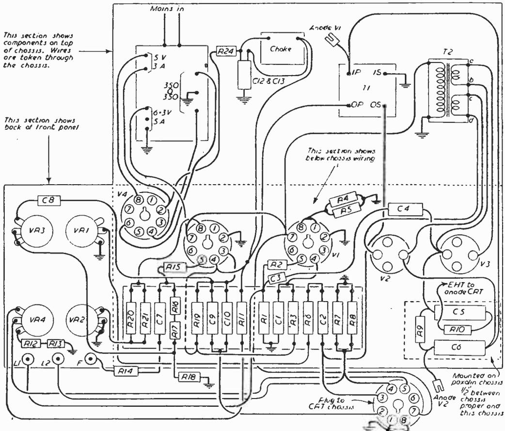
Fig. 15.—Wiring diagram of the unit.
