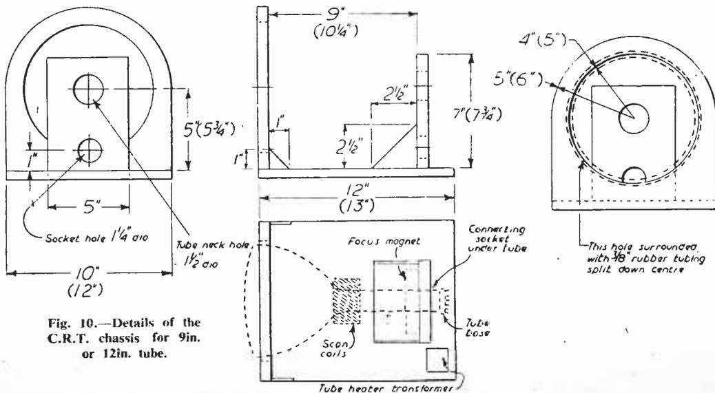
Fig. 10.—Details of the C.R.T. chassis for 9in. or 12in. tube.
