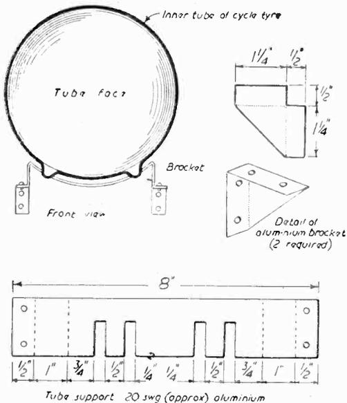
Figs. 11 and 12.—Details of the tube support, and method of mounting.
