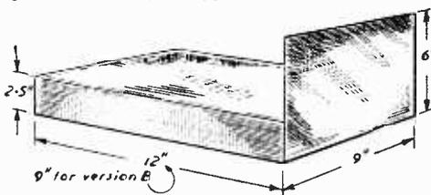
Fig. 9.—Chassis dimensions.
