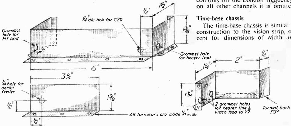
Fig. 2.—Details of the underchassis dividing screens.
