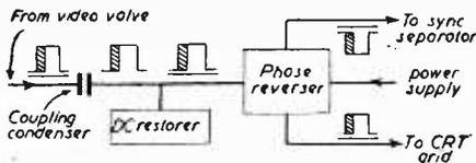
Fig. 21.—Illustrating the meaning of phase reversal.
