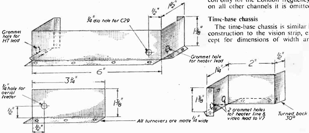
Fig. 2.—Details of the underchassis dividing screens.
