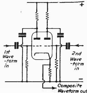
Fig. 12.—Basic waveform mixers.
