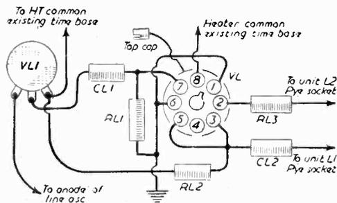
Fig. 13.—Wiring diagram of line phase-reversing circuit.
