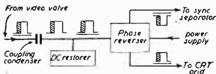
Fig. 21.—Illustrating the meaning of phase reversal.
