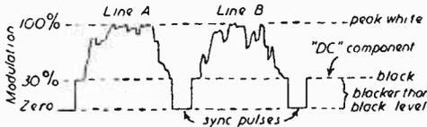
Fig. 19.—A portion of the vision signal waveform.
