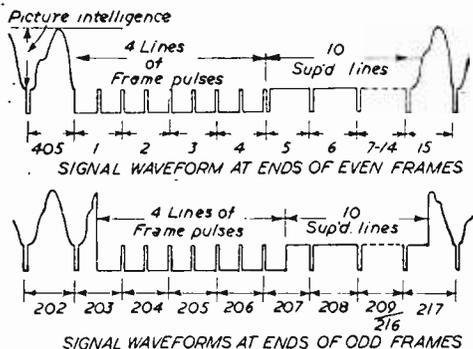
Fig. 1.—The standard BBC television waveforms.
