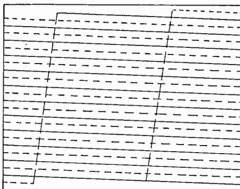
Fig. 2.—The interlaced half-frames.
