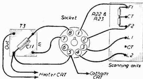
Fig. 14.—Wiring diagram of the C.R.T. chassis.
