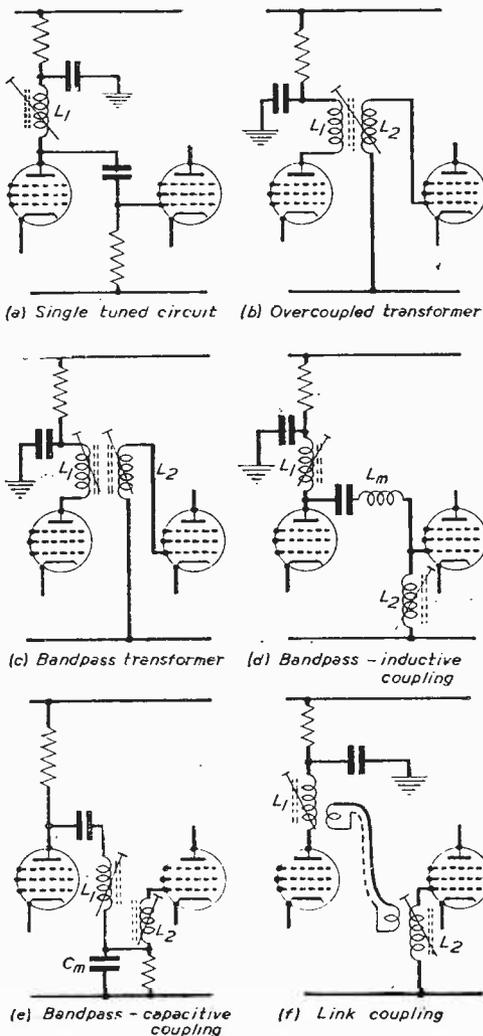
Fig. 1—The various types of interstage coupling.
