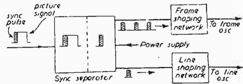
Fig. 20.—Diagram illustrating the action of the sync separator.
