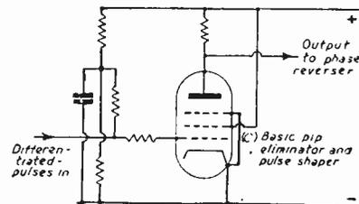
Fig. 9.—Obtaining line sync pulses.
