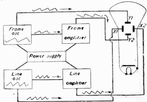
Fig. 16.—Schematic electrostatic deflection arrangement.
