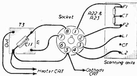
Fig. 14.—Wiring diagram of the C.R.T. chassis.
