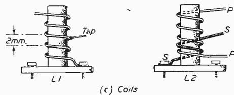
Fig. 22.—Details of the pre-amplifier and coils.
