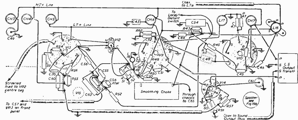
Fig. 20.—Wiring details of the sound section.
