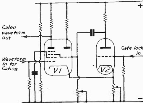
Fig. 11.—A gate circuit.
