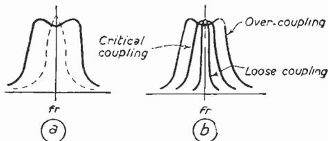
Fig. 2.—Response curves showing the effect of different degrees of coupling.
