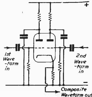
Fig. 12.—Basic waveform mixers.
