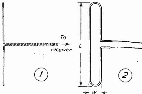
Figs. 1 and 2.—A dipole made from ordinary lighting flex and a folded dipole. L and W may be varied to find the best combination.
