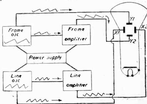
Fig. 16.—Schematic electrostatic deflection arrangement.
