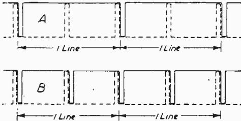
Fig. 3.—The relative timing of frame and line sync pulses.
