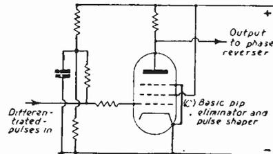
Fig. 9.—Obtaining line sync pulses.
