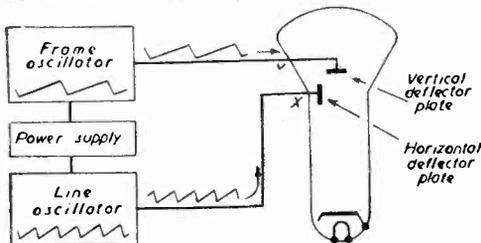
Fig. 15.—Basic deflection circuit.
