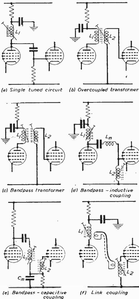
Fig. 1—The various types of interstage coupling.
