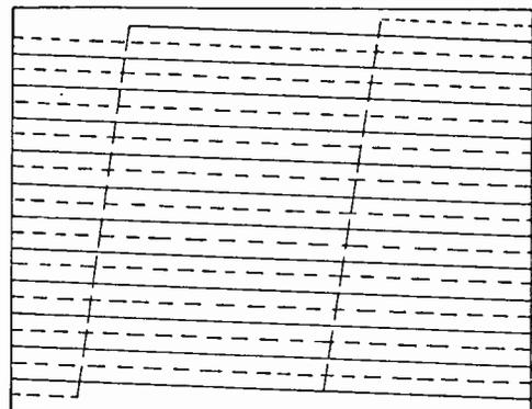
Fig. 2.—The interlaced half-frames.
