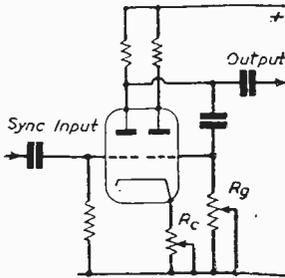
Fig. 8.—The basic master oscillator.
