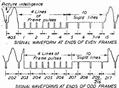
Fig. 1.—The standard BBC television waveforms.
