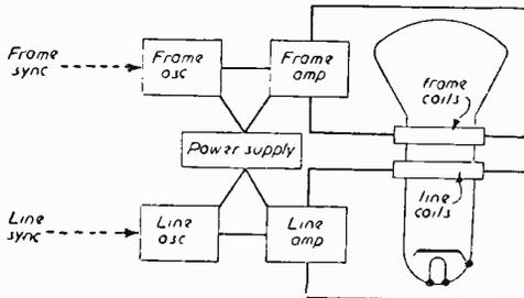
Fig. 17.—Schematic electro-magnetic deflection arrangement.
