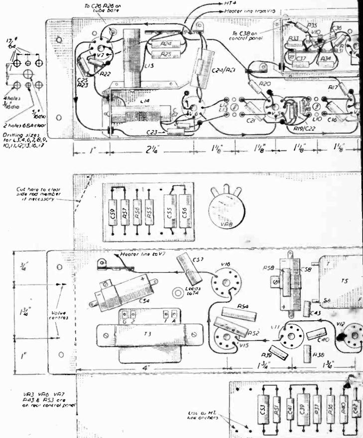
Fig. 1 (top).—Layout of the vision-sound strip, with wiring.
