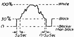
Fig. 1.—The signal corresponding to one scanning line of a television image.
