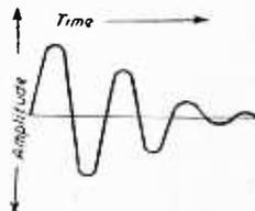
Fig. 3.—A damped oscillation.
