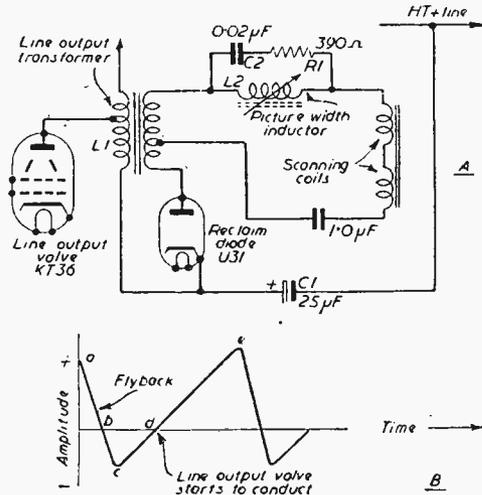
Fig. 6.—(A) Flyback damping and reclaim circuit as used in G.E.C. BT.2147 series receivers, and (B) curve which will be explained in the next article on this subject.
