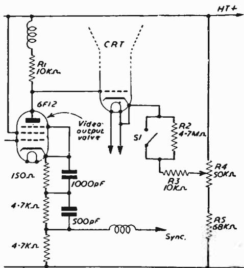
Fig. 2.—The picture-tube control circuit of an old-style Murphy receiver.
