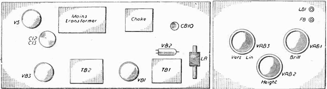
Fig. 20 (a) and (b).—Top view of chassis and panel of Model "B".
