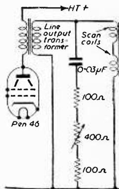
Fig. 5.—The flyback damping circuit as employed in the Murphy V114 and V118 receivers.
