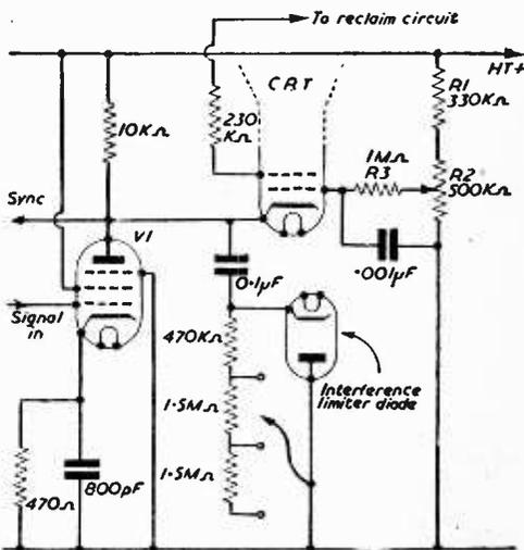
Fig. 3.—Picture-tube control circuit of the Ferguson Model 988T.
