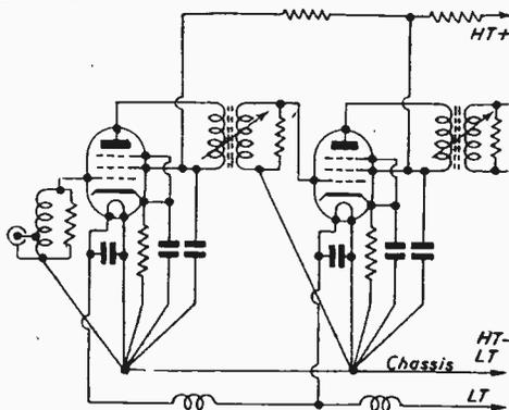
Fig. 3.—The use of double-wound coils and taking all chassis connections to one point for each stage eliminates chassis currents.
