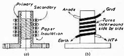
Figs. 2a and 2b.—Two methods of making 1 : 1 transformers.
