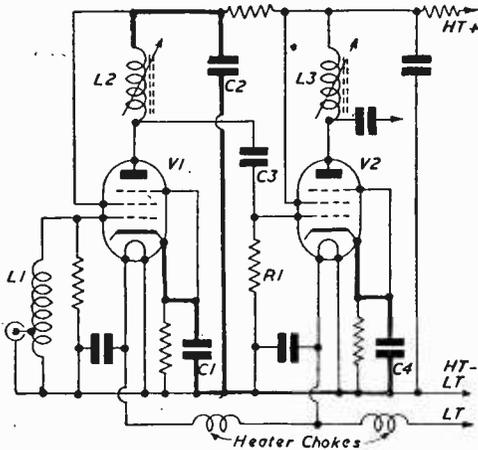
Fig. 1.—Section of circuit commonly used in amateur built receivers. Heavy lining indicates the earth return circuits of L2.
