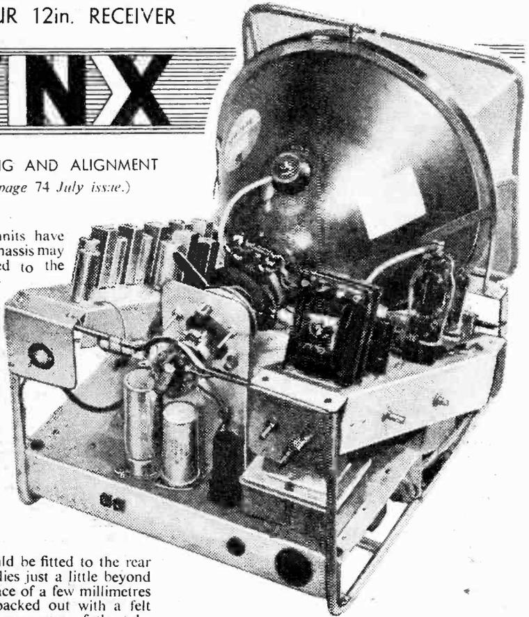
power supplies, scan coils, etc., by long leads, the units themselves being free of the framework so that they may be upended for alignment. Earthing leads should not be forgotten. The rear control panel, carrying VR3, VR6 and VR7, should similarly be "free" on the end of longish connecting wires for the present.
