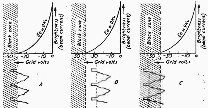
Fig. 1.—Diagrams showing the effect of picture contrast ratio for various brightness settings. (a) Correct, (b) too much and (c) too little brightness.
