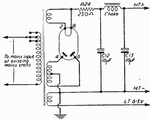
Fig. 16.—The power supply.
