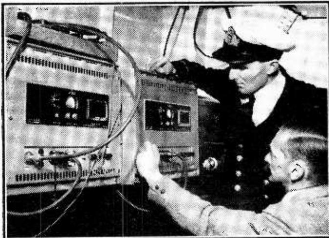
Two new G.E.C. frequency modulation V.H.F. transmitters in the communications room of H.M.S. "Eagle." They were employed for the ship-to-shore sound transmission of the BBC television broadcast of the Coronation Naval Review.
