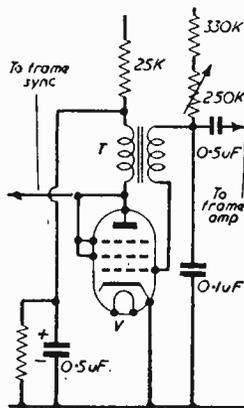
Fig. 17 (left).—The oscillator stage of Model "B".
