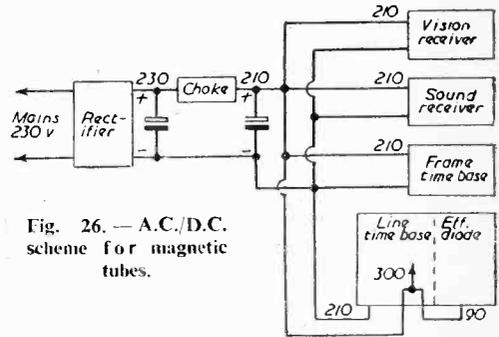
Fig. 26.—A.C./D.C. scheme for magnetic tubes.
