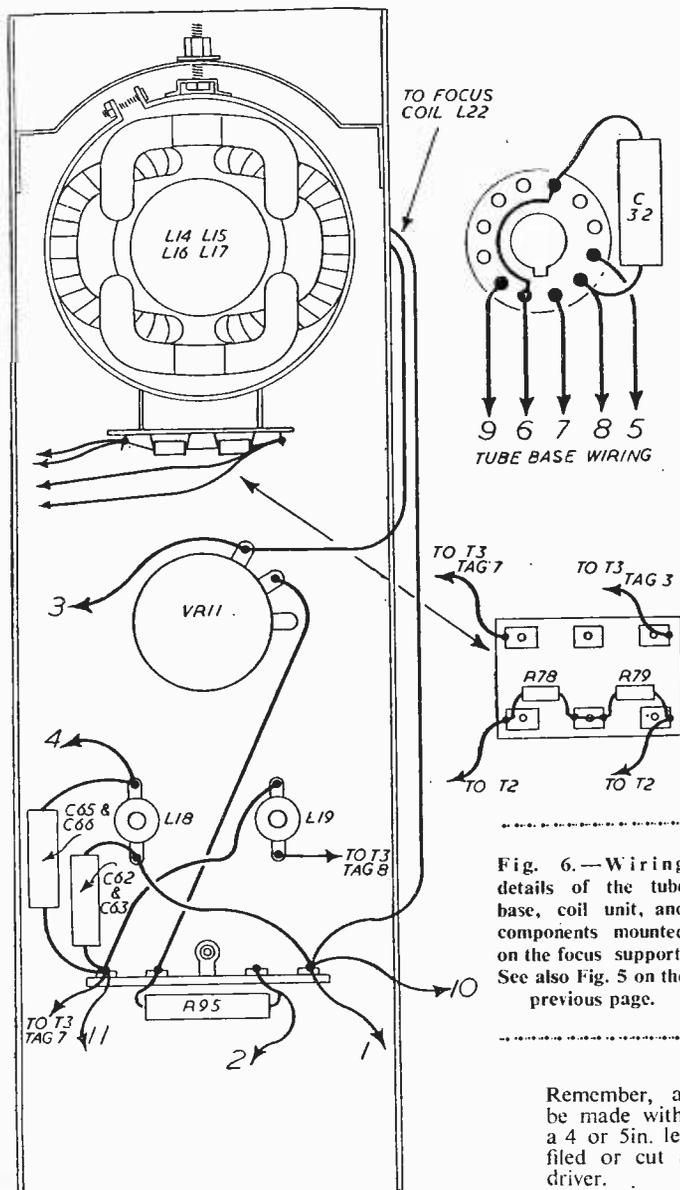
Fig. 6.—Wiring details of the tube base, coil unit, and components mounted on the focus support. See also Fig. 5 on the previous page.
