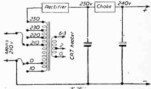
Fig. 27.—The auto-wound transformer arrangement.
