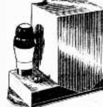
The NERA R.F., E.H.T. unit has been designed to provide a safe and reliable source of D.C. high voltage for all C.R.T.s including the new wide angle and aluminised types. The output is continuously variable between 8 to 12 Kv. at approximately 500 microamps.
