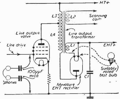
Fig. 12.—A typical line flyback E.H.T. circuit.
