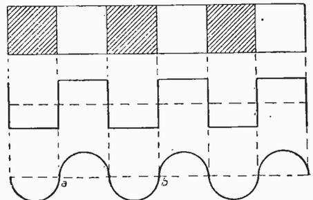
Fig. 2.—Type of wave giving the black and white pattern. One cycle is from a to b.
