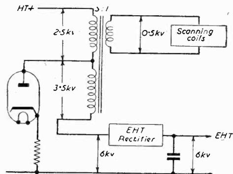
Fig. 30.—This is the flyback E.H.T. arrangement.
