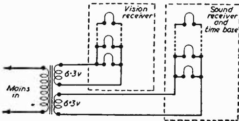
Fig. 22.—A parallel heater wiring arrangement.
