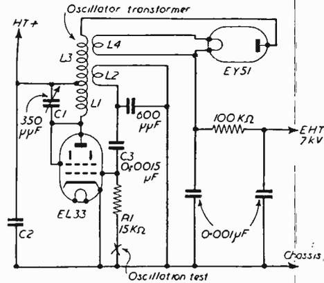
Fig. 13.—A typical R.F. E.H.T. unit by R.G.D. (Model B2 351T).
