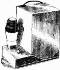
The NERA R.F., E.H.T. unit has been designed to provide a safe and reliable source of D.C. high voltage for all C.R.T.s including the new wide angle and aluminised types. The output is continuously variable between 8 to 12 kV. at approximately 500 microamps.
