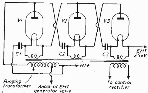
Fig. 15.—A cascade multiplier as used in projection E.H.T. receivers.
