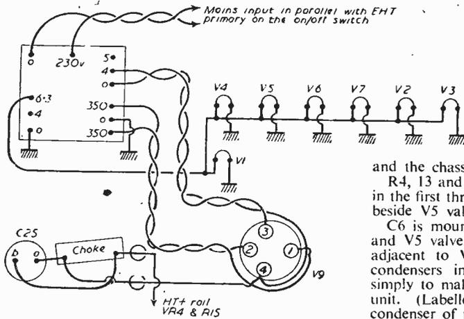
Fig. 8.—Wiring diagram of power supply.
