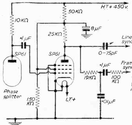
Fig. 2.—The sync separator circuit.
