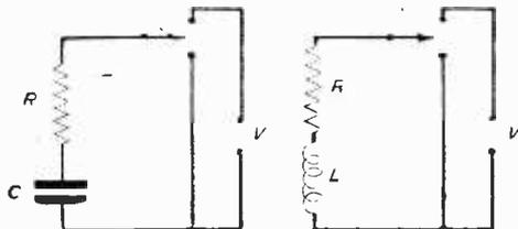
Fig. 1.—A simple R-C circuit.
