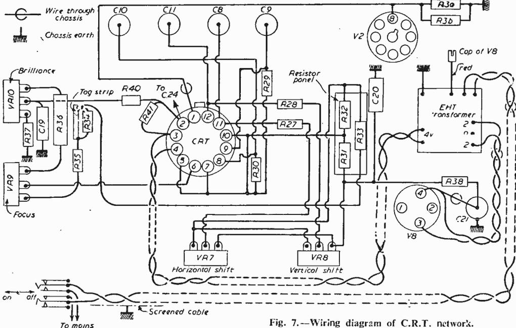
Fig. 7.—Wiring diagram of C.R.T. network.
