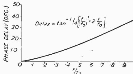
Fig. 1 (left).—Gain and phase delay characteristics for a single uncompensated stage. Fig. 2 (right).—Phase delay characteristic for a single-stage compensated circuit.
