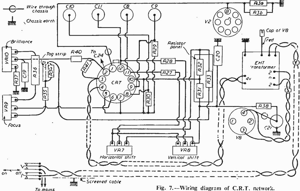
Fig. 7.—Wiring diagram of C.R.T. network.
