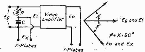
Fig. 4. — System providing the delay to the input voltage.
