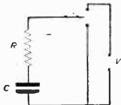
Fig. 1.—A simple R-C circuit.
