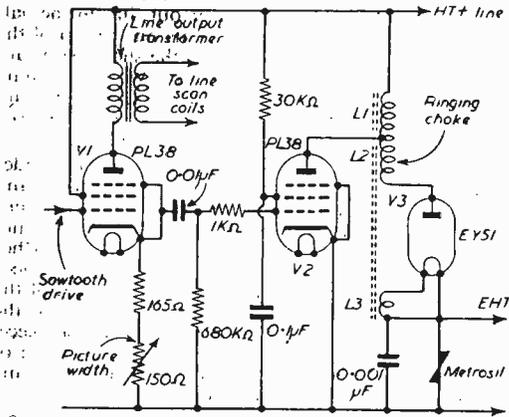
Fig. 14.—A typical "ringing" choke E.H.T. system by Invicta (Model T102).
