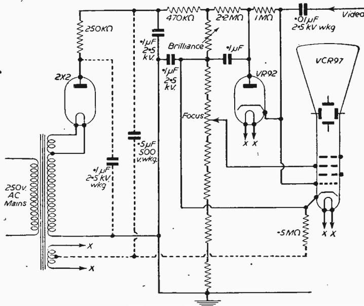
Fig. 6.—Modifications (shown dotted) carried out on tube network to reduce hum on picture.
