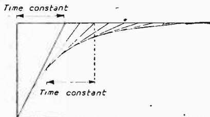
Fig. 4.—Method of constructing the curve in Fig. 3.
