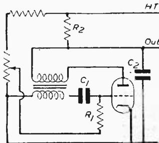
Fig. 6.—A typical blocking oscillator circuit.
