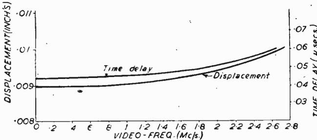
Fig. 3. — Curve of the actual horizontal displacements of the picture elements at the different video frequencies.
