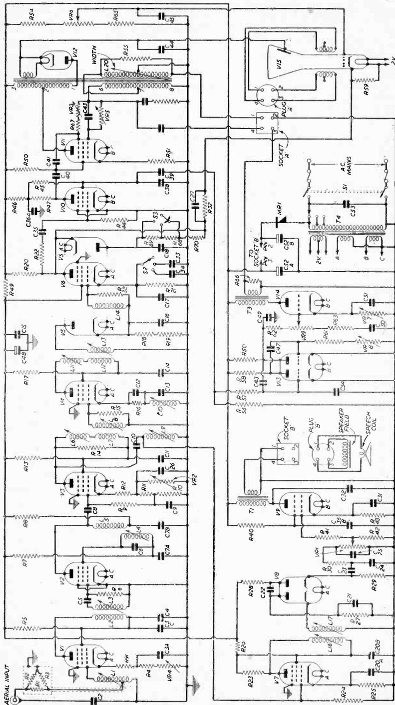
Complete circuit diagram of the Plessey chassis, which forms the basis of a number of popular commercial receivers. A complete list of components cannot be supplied by us, neither can we supply values of resistors, etc. Many of these are self-evident or may be ascertained by reference to circuits published in these pages.
