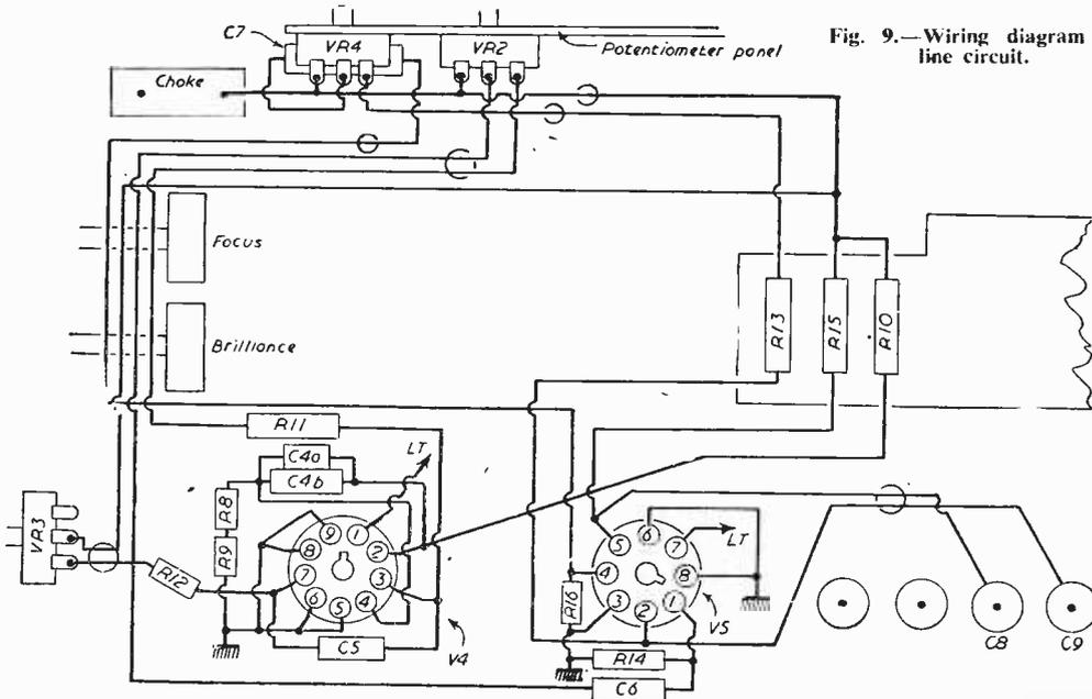
Fig. 9.—Wiring diagram of line circuit.
