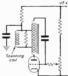
Fig. 7.—A sawtooth current generator.
