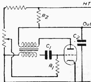
Fig. 6.—A typical blocking oscillator circuit.
