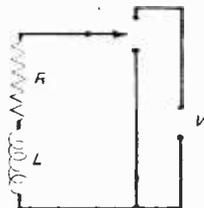
Fig. 2.—A basic R-L circuit.
