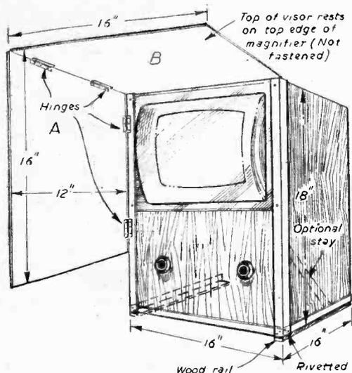
Fig. 1.—Constructional details of the magnifier and visor.
