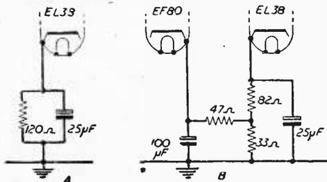
whilst the modified circuits recommended by Mullard, Ltd. for their projection circuits are shown in 2b, 3b and 4b. It will be appreciated that the modification is in all cases simple.
