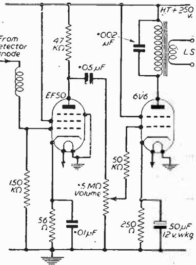
Fig. 4.—Conventional output stage from Pye strip to 6V6.
