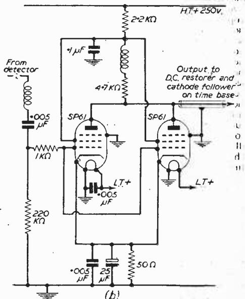
Fig. 5(a).—Original output stage of 1355 receiver and (b) modified output stage showing two SP61 valves wired in parallel.
