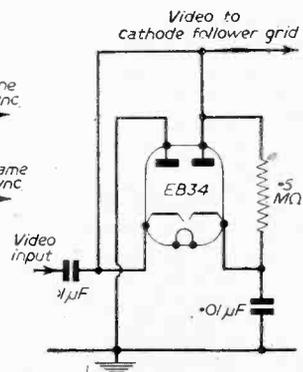
Fig. 3.—D.C. restorer and noise limiter.
