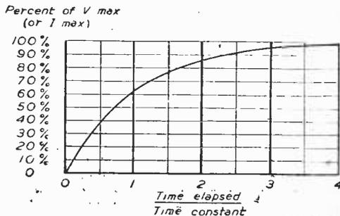
Fig. 3.—A generalised time-constant curve.
