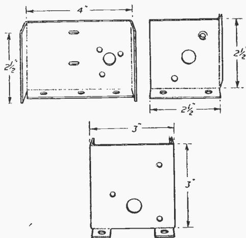
Fig. 4.—Details of the mounting brackets.
