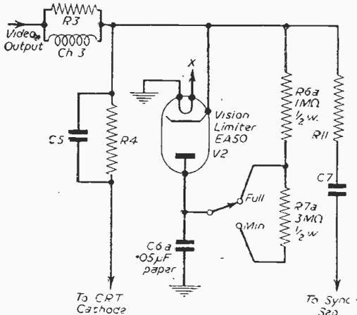
Fig. 2.—An alternative vision interference limiter circuit.
