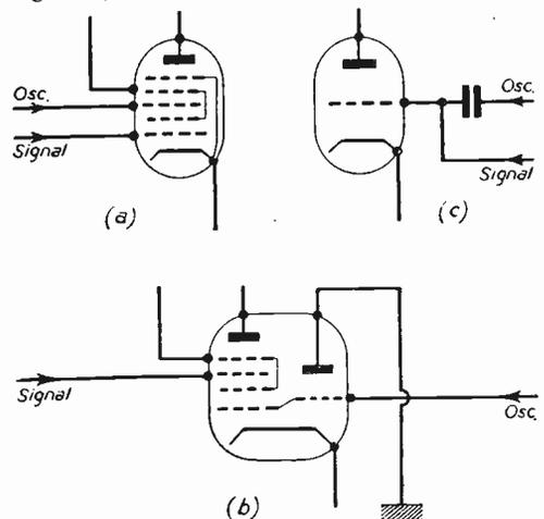
Fig. 1.—Mixer circuits suitable for television receivers.
