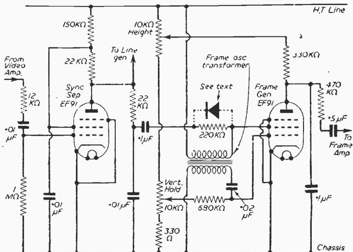
Fig. 50.—The frame synchronising section and frame blocking oscillator of the Ferguson 941T.
