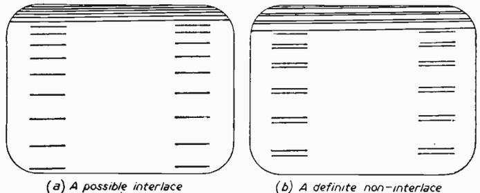
Fig. 48.—The formation of flyback lines, showing possible and non-interlace.
