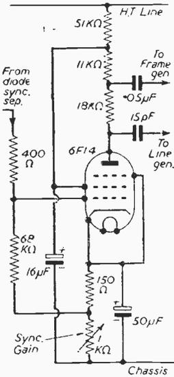
Fig. 49.—The sync amplifier stage of the Decca Projection Model 121.
