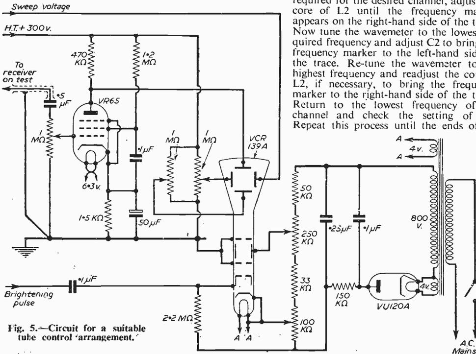
Fig. 5.—Circuit for a suitable tube control arrangement.
