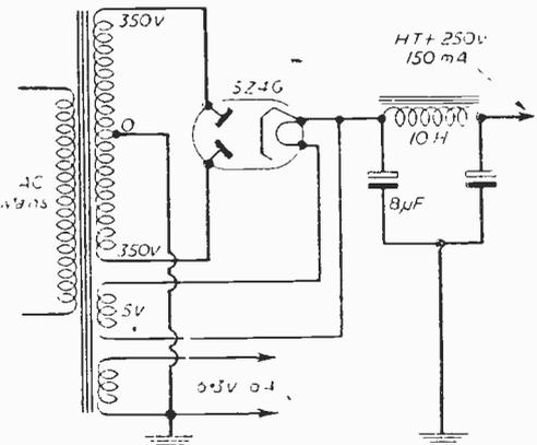
Fig. 9.—Circuit of a suitable mains unit.
