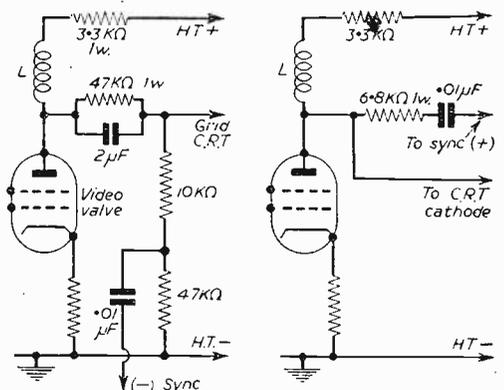
Fig. 5.—Alternative methods of feeding the tube.
