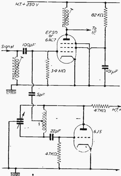
Fig. 2.—A practical mixer circuit using a pentode as a mixer with separate triode oscillator.
