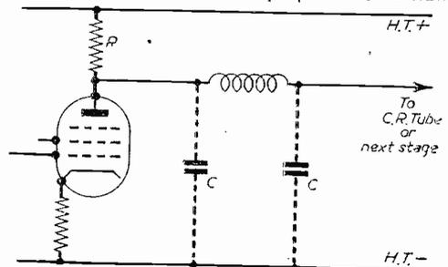
Fig. 1.—A simple video compensating circuit, making use of unavoidable stray capacities in a filter coupling.
