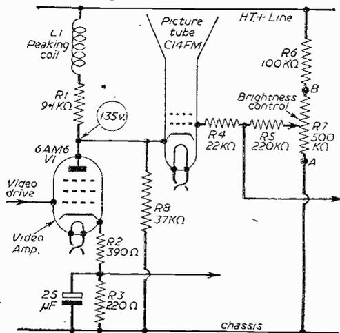
Fig. 51.—The picture-tube control network of the K.B. Model KV35.
