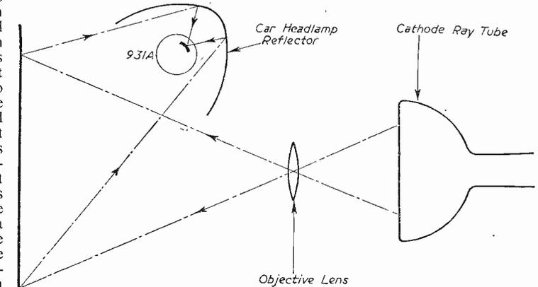
Fig. 6.—Obtaining maximum light by the use of a condenser and car headlamp reflector.
