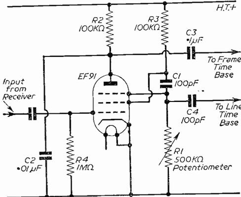
Fig. 1.—Circuit of the transitron sync separator.
