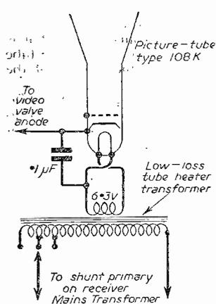
Fig. 53.—A method of restoring picture quality after a heater to cathode fault has occurred in the tube.
