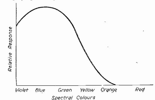
Fig. 3.—The response curve of the 931A cell.
