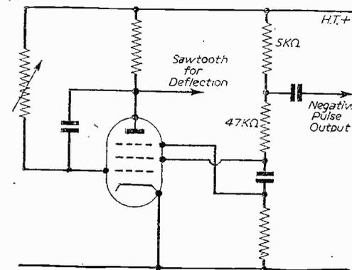
Fig. 1.—Circuit for obtaining pulses from the timebase.
