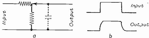
Fig. 1.—A normal volume control and its effect on the waveform.
