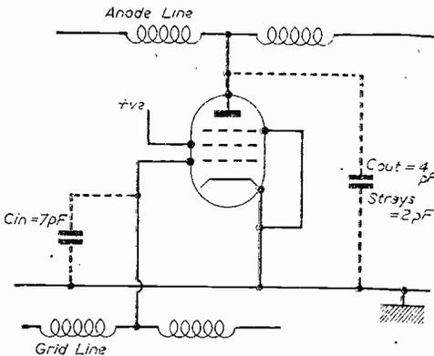
Fig. 4.—A circuit with capacities to illustrate the design procedure.
