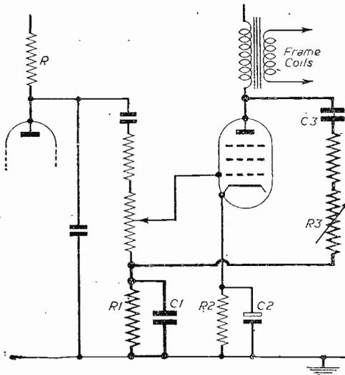
Fig. 3.—Frame timebase by Haynes. The feedback is shown in heavy lines.
