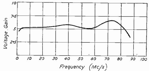
Fig. 5.—Bandwidth-gain curves of a simple four-valve single-stage amplifier.
