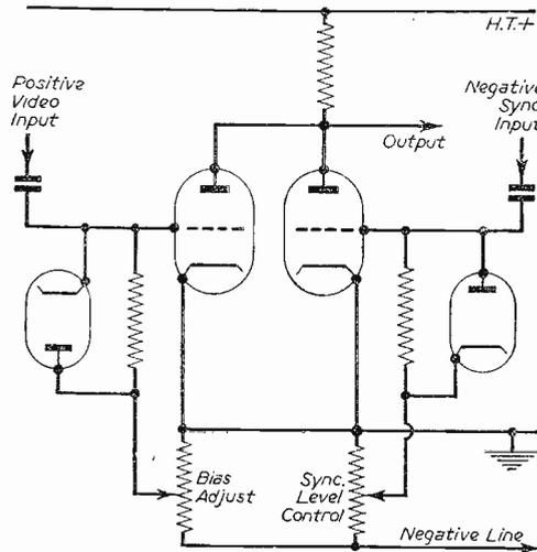
Fig. 2.—The additive mixing of sync and video signals.
