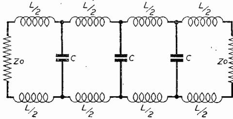
Fig. 2.—Representation of a two-wire transmission line as a series of low-pass filters.
