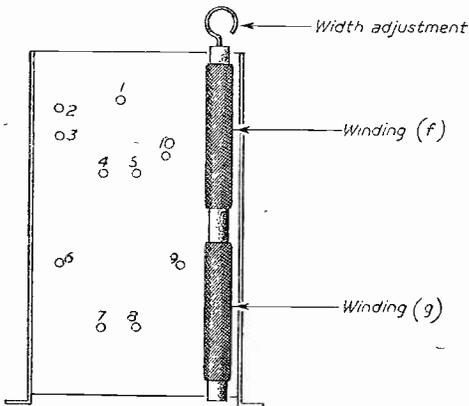
Fig. 4.—Wiring connections for line output transformer. The transformer is Plessey Type SL7 (Part No. CP 72036/2). The earlier CP72036 may be found to have tag 10 missing. In this type, the appropriate additional connection to tag 9 must be separated if the shift controls are desired. If shift controls are not desired, tag 9 (and 10 if fitted) should be returned to chassis.
