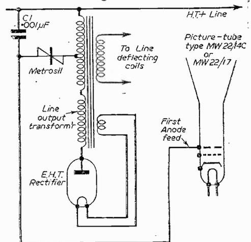
Fig. 54.—A method of obtaining picture-tube first anode potential in the Ferguson 941T.
