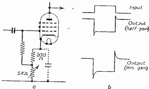
Fig. 2.—Controlled negative feedback and its effect on waveform.
