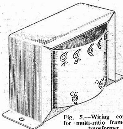
Fig. 5.—Wiring connections for multi-ratio frame output transformer.
