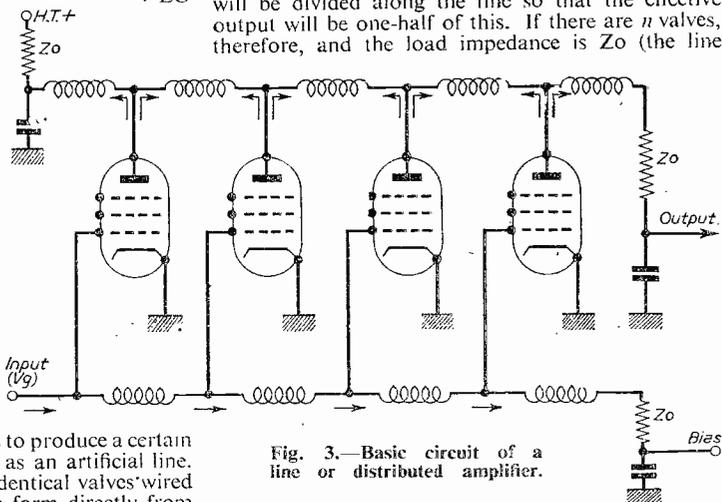
Fig. 3.—Basic circuit of a line or distributed amplifier.
