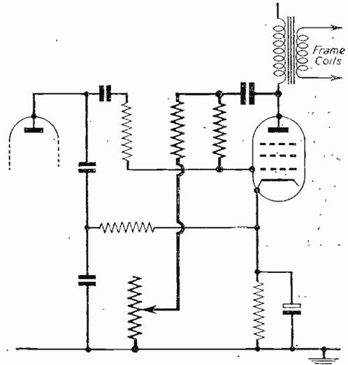
Fig. 4.—This is the Super-Visor frame timebase. Again the feedback is shown by heavy lines.
