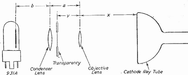
Fig. 5.—Diagram showing the optical layout of a slide scanner.
