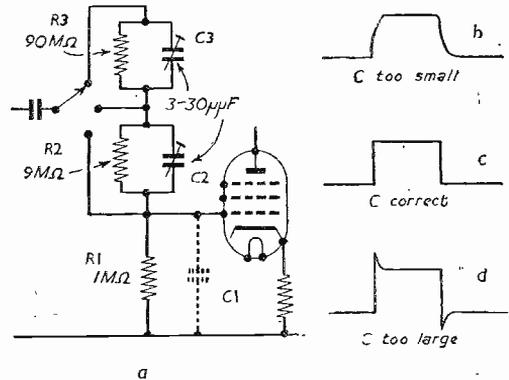
Fig. 3.—A solution. The three switch positions are, bottom 1, centre  $\div 10$ , top  $\div 100$ .
