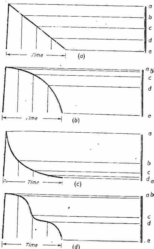
Fig. 2.—These illustrations show how a distorted waveform can result from a poor shaped saw-tooth input.
