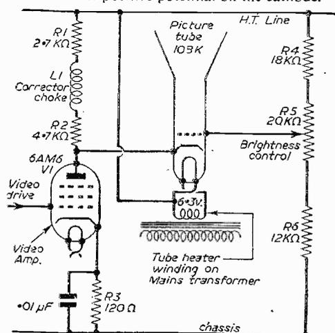
Fig. 52.—The picture-tube control arrangement as used in the Cossor Model 916-917 series.
