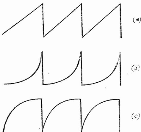
Fig. 1.—A saw-tooth and two distorted forms of it at (b) and (c).
