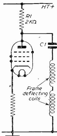
Fig. 55.—A R.C. coupled frame output stage. Note the importance of high insulation across C1.
