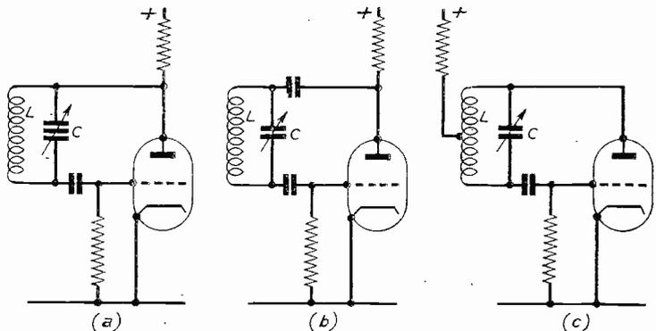
Fig. 1.—Showing (a) Colpitt's (b) Hartley, and (c) Ultraudion oscillators respectively.
