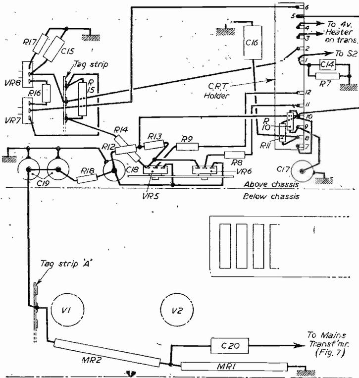
Fig. 6.—The E.H.T. and C.R.T. network.
