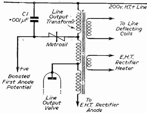
Fig. 3.—Circuit showing how Metrosil can be used to obtain a boosted first anode potential.
