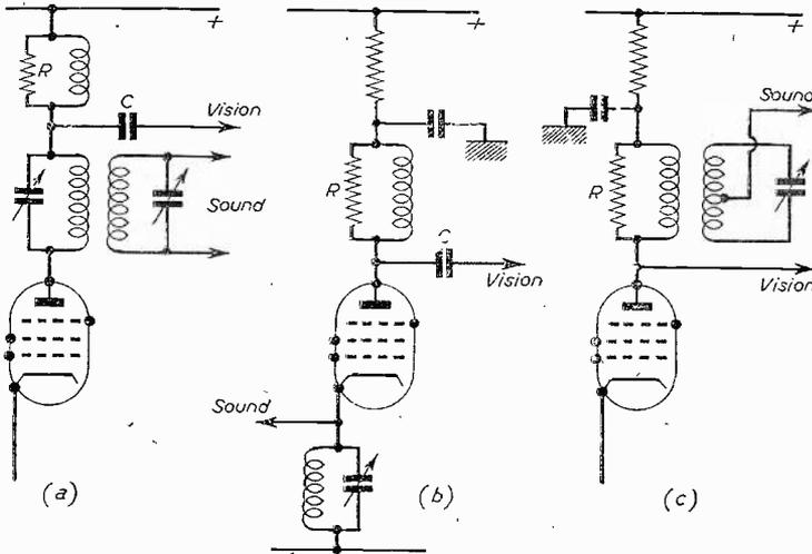
Fig. 2.—Methods of separating the sound and vision I.F.'s at the output of the mixer.
