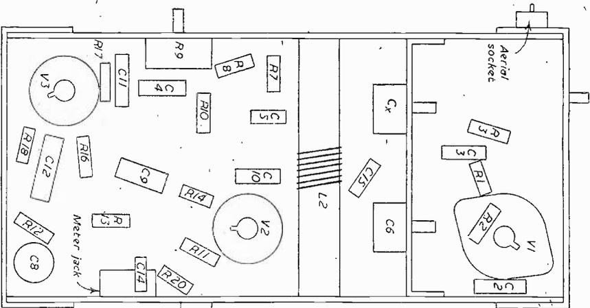
Underside and top chassis layouts for the unit. Note that C6 should be insulated from the chassis. Cx was an experimental condenser and is replaced by C15.
