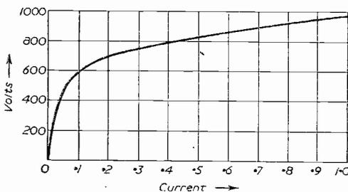
Fig. 1.—A graph showing the non-linear volt-ampere property of Metrosil.
