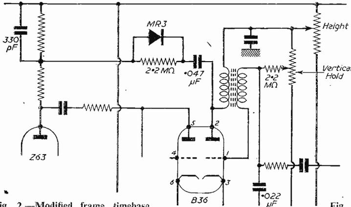
Fig. 2.—Modified frame timebase with component changes. Note addition of small rectifier shunted by 2.2 MΩ resistor.
