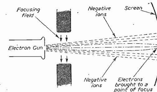
Fig. 61.—Showing how the negative ions are little influenced by the magnetic focusing field.
