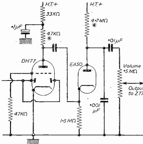
Fig. 4.—Valve-limiter circuit. The load resistor of the DH77 may be changed to 220 KΩ to minimise distortion with stressing of sibilants. Also the 4.7 MΩ resistor may be decreased to 2.2 MΩ.
