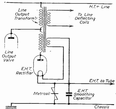
Fig. 2.—Showing how Metrosil can be used to enhance E.H.T. regulation.
