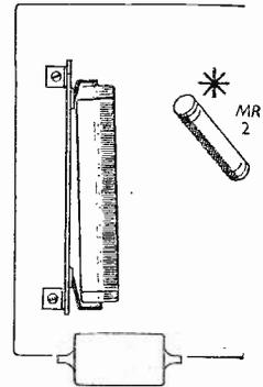
Fig. 3.—R.F. Unit—audio end. Note position of MR2 noise-limiter whose load resistor may be 3.3 MΩ in place of the 4.7 MΩ when valve-limiter is fitted.
