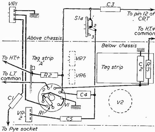
Fig. 4.—Wiring of the amplifier.
