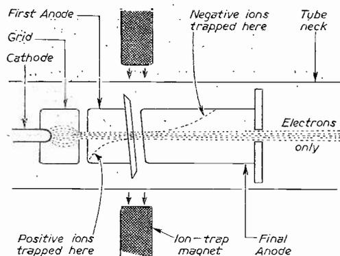
Fig. 62.—Illustrating the electron-gun assembly as used in the new Mazda tetrode tubes.
