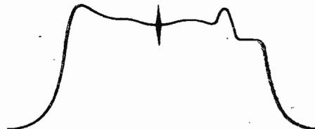
Fig. 4.—Appearance of marker pip from signal generator.
