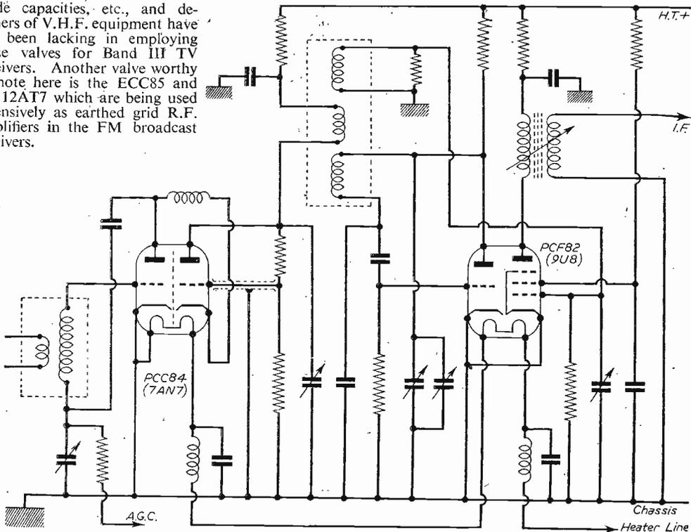
Fig. 2.—The cascode circuit as used in the latest KB receivers.
