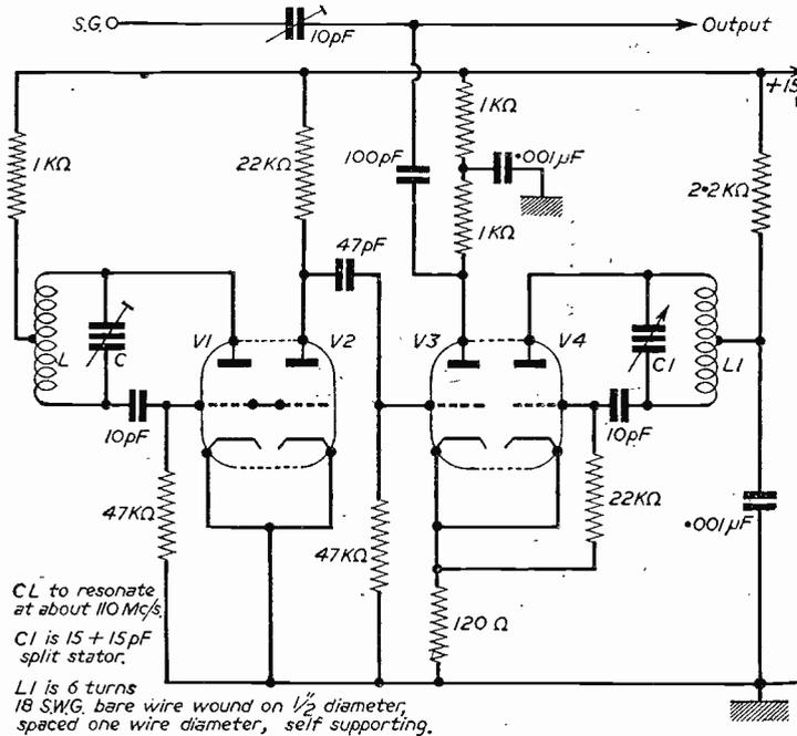
Fig. 3. — A simple sweep circuit.
