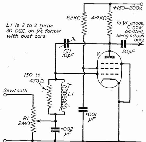
Fig. 5. — Electronic equivalent of the mechanical tuning systems.
