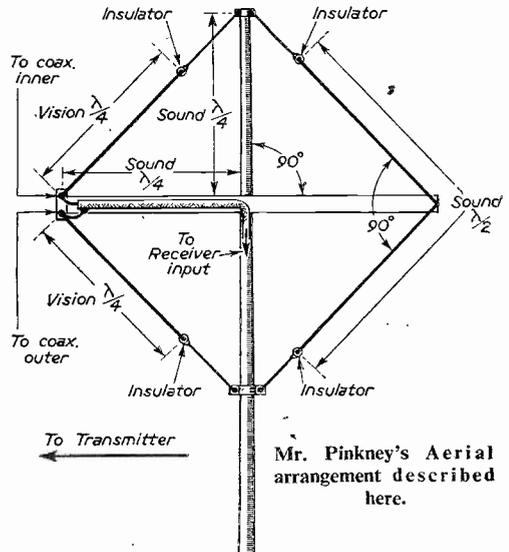
The copper wire reflector is taken from an insulator at the top of the pole over the rear end of the spreader and secured to an insulator at the same point as the lower end of the dipole cord. The reflector should be one half sound wavelength long. The whole thing should now be diamond shaped.
