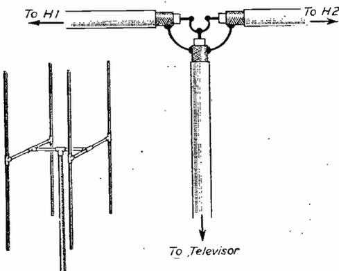
Figs. 6 and 7.—A double "H" aerial and the cable connections for a double "H."
