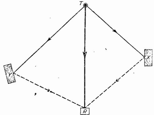
Fig. 5.—Reflection from two sources.
