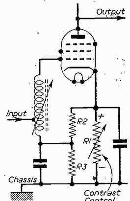
Fig. 72.—A typical contrast control circuit.
