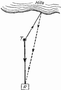
Fig. 4.—Diagram illustrating the result of reflection from an object behind the actual transmitter.
