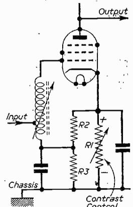
Fig. 72.—A typical contrast control circuit.
