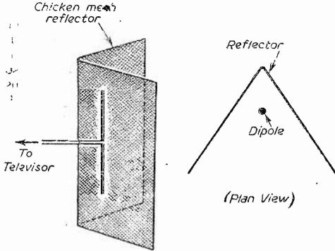
Fig. 8.—The corner reflector.
