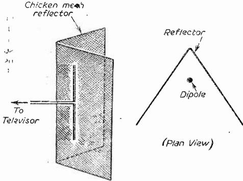
Fig. 8.—The corner reflector.
