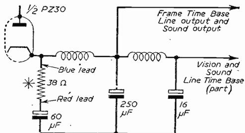
\* This resistor is mounted on the end of a paxolin panel on the left side of the upper chassis.
