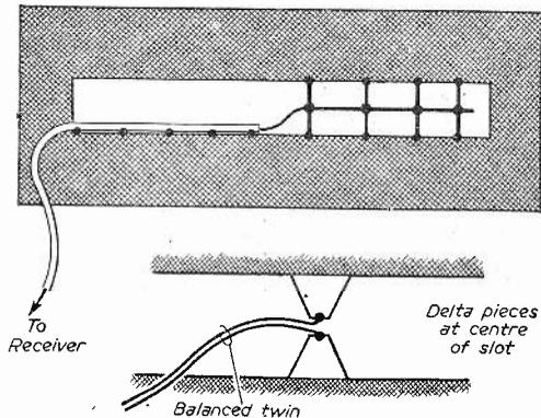
Fig. 9.—Details of the slot aerial.
