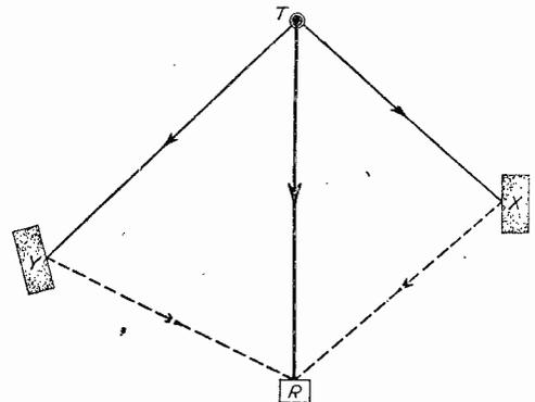
Fig. 5.—Reflection from two sources.
