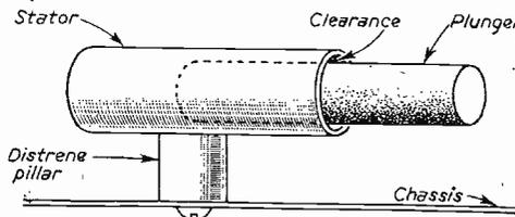
Fig. 1.—Mounting of a co-axial tuning system. The stator is best split to form a split-stator condenser.
