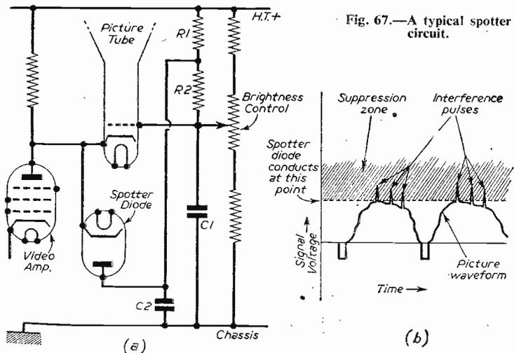
Fig. 67.—A typical spotter circuit.
