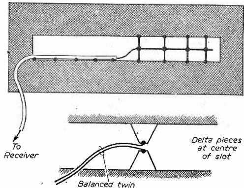
Fig. 9.—Details of the slot aerial.
