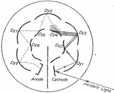
Fig. 4.—Diagram of the electrode structure of the 931A showing electron multiplication and the approximate path of the electrons through the tube.
