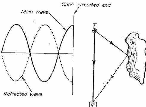
Fig. 2.—The reflected wave. Fig. 3.—Reception of one ghost.
