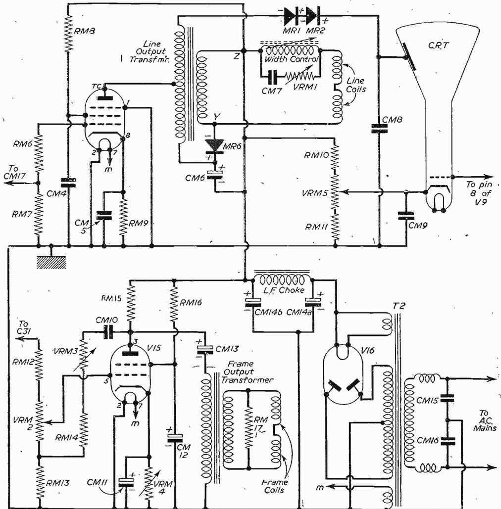
Fig. 1.—The timebase amplifier.
