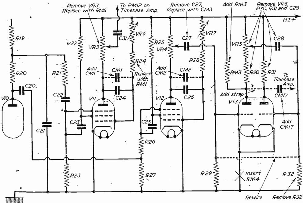
Fig. 2.— Modifying the existing timebase: R28 is replaced by RM2.
