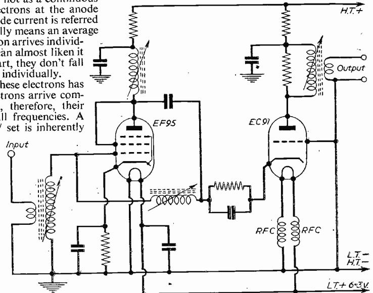
Fig. 1.—A Low-noise Cascode pre-amplifier.
