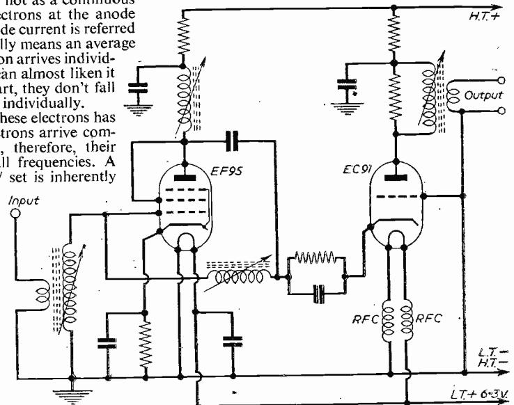
Fig. 1.—A Low-noise Cascode pre-amplifier.
