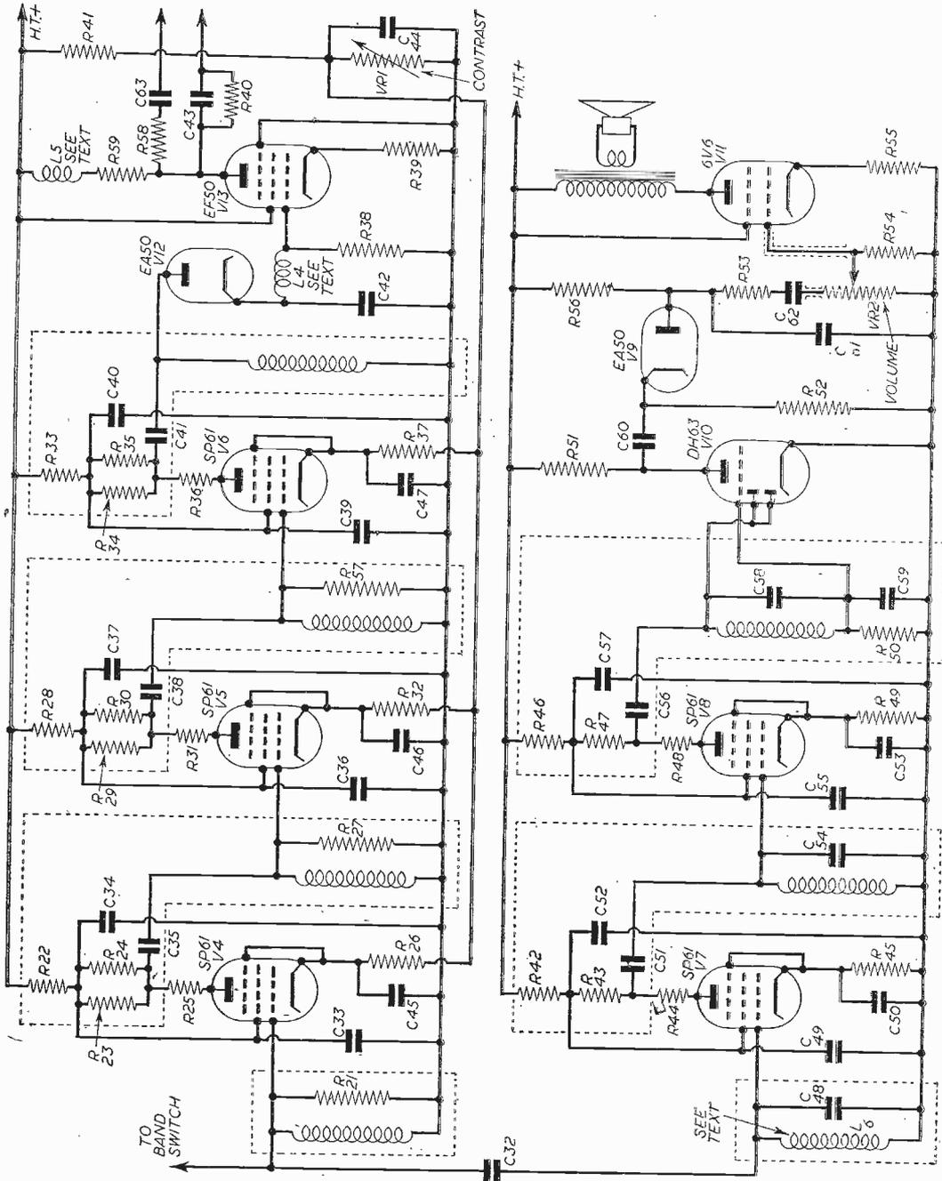
Fig. 6 — The completed, modified, video and sound receivers. The input marked "To Band Switch" is connected to the switch through condenser C63. A complete list of values was given in last month's issue.
