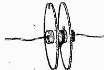
Details of Construction of Video Peaking Chokes. The cheeks are made from card or paxolin, and mounted on a resistor.
