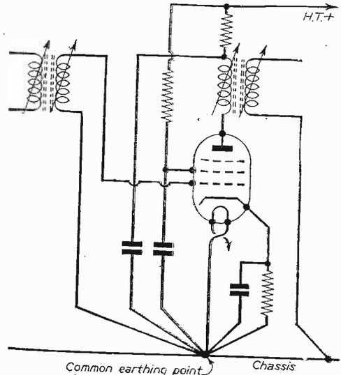
Fig. 79 (left).—A test for instability. Fig. 80 (right).—When replacing decoupling capacitors, ensure that they are returned to the common earthing point.
