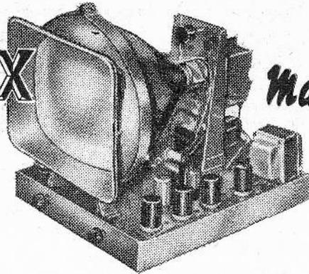
**A** FOUR-WAY tag strip is mounted on the tube holder for terminating the scanning coils and another one-way is used for mounting the width control.
