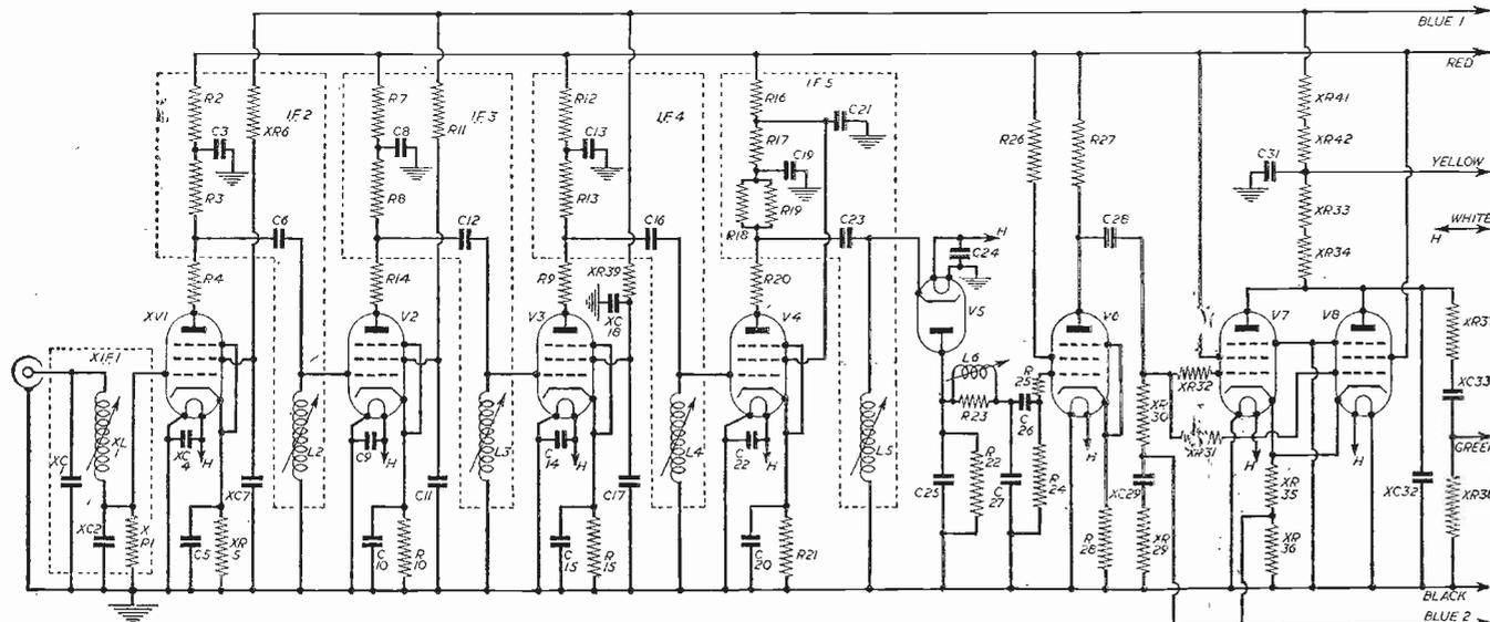
Fig. 2.—Complete circuit showing components, prefixed by "X," which have to be removed.
