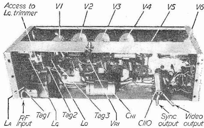
Fig. 5 (a)—View of the unit with various parts identified, after modification.
