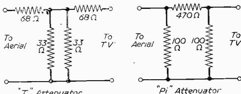
Fig. 4—Two simple types of signal attenuator.
