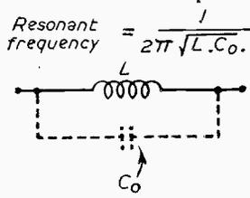
Fig. 2 (left)—A simple suppressor circuit. Fig. 3 (right)—The essential components of a suppressor.
