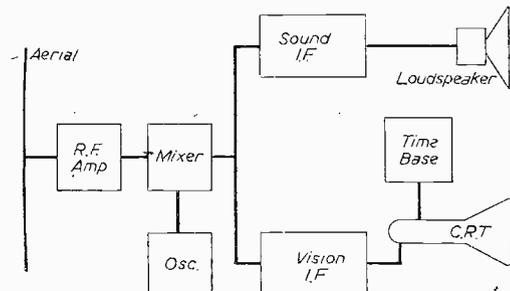
Fig. 1—Block diagram of a TV superhet.
