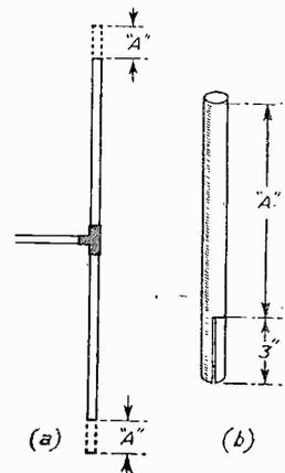
Fig. 3—Details of a standard dipole, and method of increasing its overall length by adding a further length of tubing.
