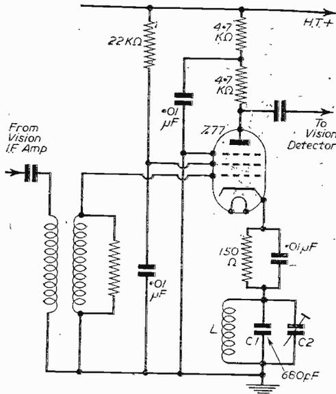
Fig. 84.—A cathode sound rejector circuit as used in G.E.C. BT1091 series receivers.
