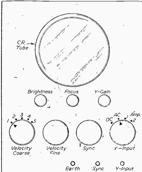
Fig. 2.—A suggested panel layout of knobs and input terminals.
