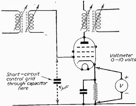
Fig. 81.—A method to prove which stage is oscillating.
