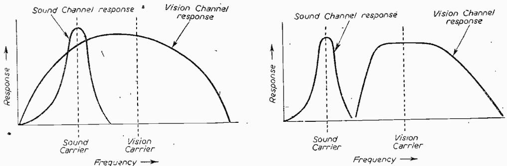
Fig. 82 (left). —Diagram showing how the vision channel response is liable to embrace the sound frequency and cause sound interference on vision. Fig. 83 (right). —The employment of a sound rejector provides a sharp cut-off at the low-frequency side of the vision channel response.
