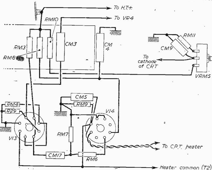
Fig. 12.—Under-chassis wiring of line amplifier and brilliance control.
