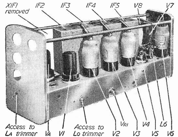
Fig. 5 (b)—Another view of the modified unit with further identifications.
