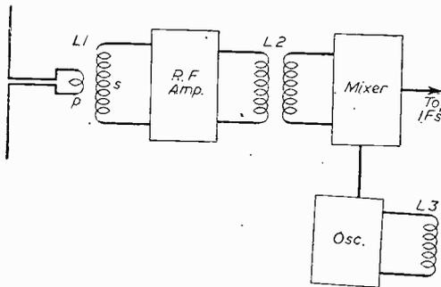
Fig. 2—Details of coil arrangements.
