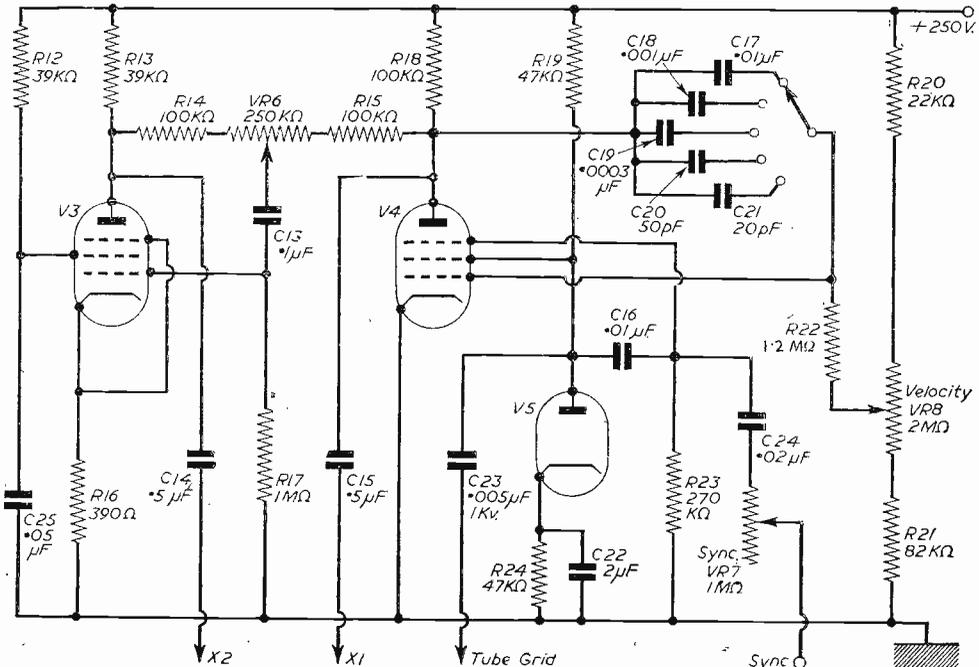
Fig. 1.—Time base circuit. All resistors are 1/2 watt and condensers paper, 350v. working, except C23.
