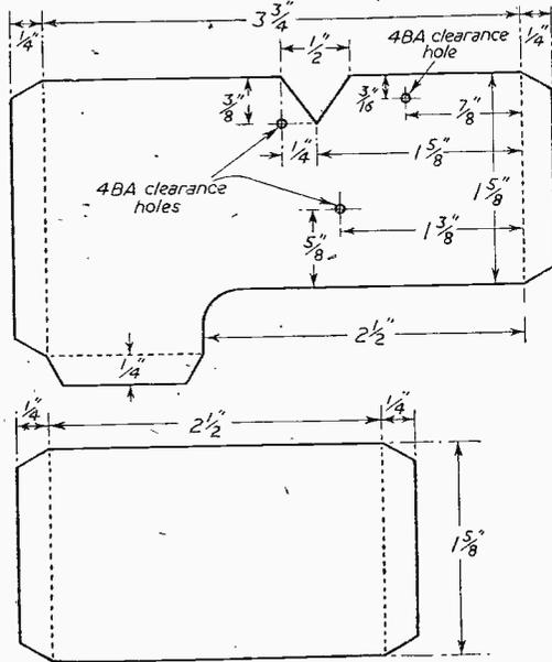
Fig. 4.—Details of the screen.
