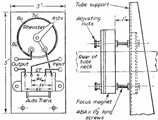
Fig. 2 (left).—Details of a brightener, and Fig. 3 (right).—the focus assembly.
