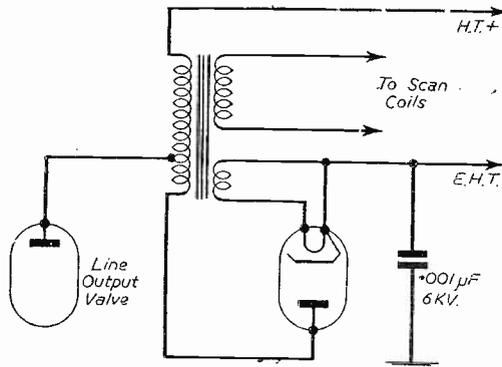
Fig. 6.—Typical flyback E.H.T. circuit.
