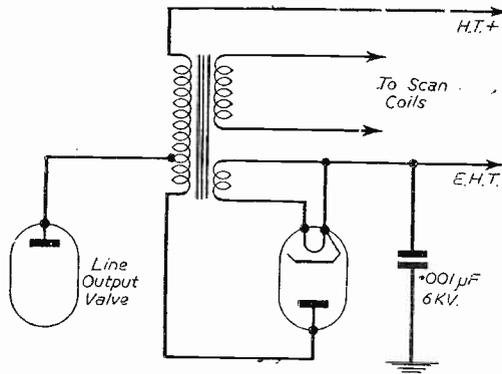
Fig. 6.—Typical flyback E.H.T. circuit.
