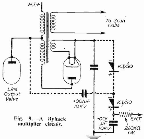
Fig. 9.—A flyback multiplier circuit.
