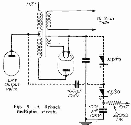
Fig. 9.—A flyback multiplier circuit.
