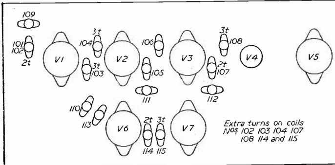
Fig. 1.—Layout of vision and sound sections.
