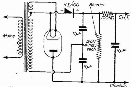
Fig. 2.—The standard doubler circuit.
