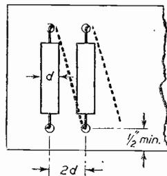
Fig. 5.—Method of mounting resistors to form the voltage-dropping chain.
