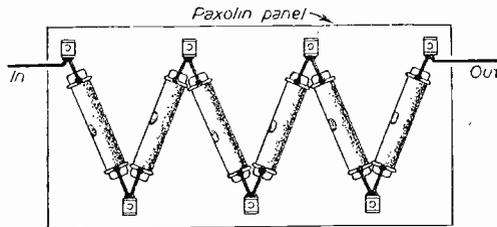
Fig. 4.—Arrangement of the bleeder resistors.
