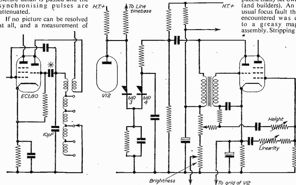
Fig. 1 (left).—Oscillator circuit. Condenser marked with an asterisk is 15 pF and is mentioned in the text. The 10 pF is less likely to cause the symptoms described. Fig. 2 (right).—Showing interlace MR3/MR4, frame oscillator transformer, and Brightness and Frame Hold potentiometer.
