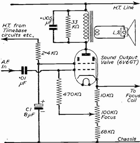
Fig. 89.—The sound output stage of K.B. FV30, FV40 and FV50 series receivers.
