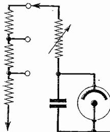
Fig. 4.—The circuit of Fig. 3 adapted for a range of supply voltages.
