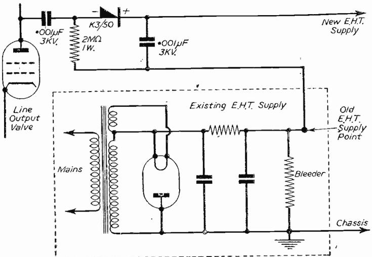
Fig. 5.—A typical flyback E.H.T. circuit.
