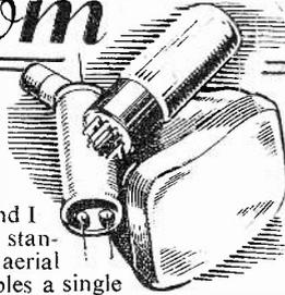
ments have to be made. The tube has a 6.3 volt heater, and would normally operate at a final anode voltage of 6 kV.—Mullard, Ltd., Century House, Shaftesbury Avenue, W.C.2.
