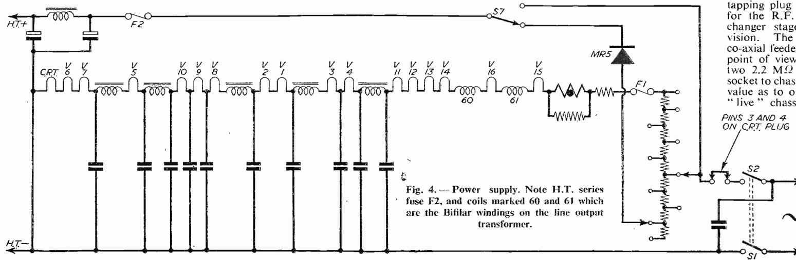
Fig. 4.—Power supply. Note H.T. series fuse F2, and coils marked 60 and 61 which are the bifilar windings on the line output transformer.
