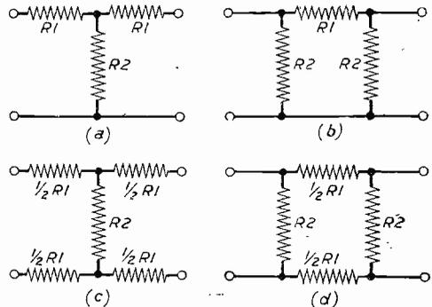
Fig. 88.—Attenuators: (a) "T" type for coaxial feeders; (b) "pi" type for coaxial feeders; (c) "T" type for twin feeders; (d) "pi" type for twin feeders.
