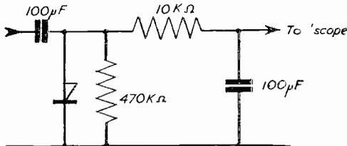
Fig. 1.—A simple detector set-up for the VSWR measurement system described.
