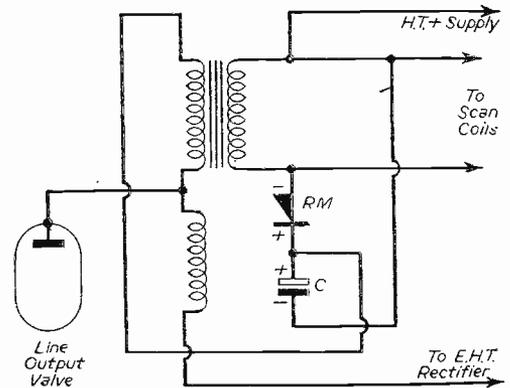
Fig. 11.—A recovery diode circuit.
