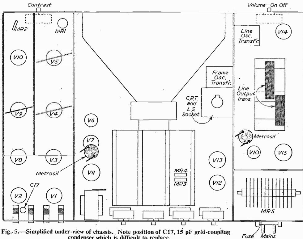
Fig. 5.—Simplified under-view of chassis. Note position of C17, 15 pF grid-coupling condenser which is difficult to replace.
