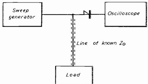
Fig. 2.—Block diagram of the test gear arrangement.
