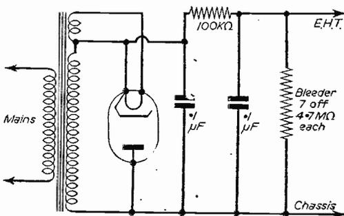
Fig. 1.—A standard mains E.H.T. circuit.
