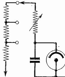
Fig. 4.—The circuit of Fig. 3 adapted for a range of supply voltages.
