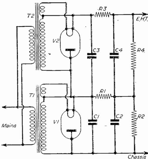
Fig. 3.—A doubler circuit using two transformers.
