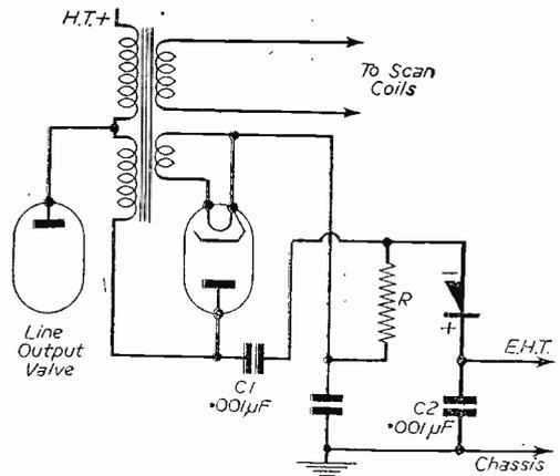
Fig. 8.—An E.H.T. doubler (Hyback) with selenium rectifier.
