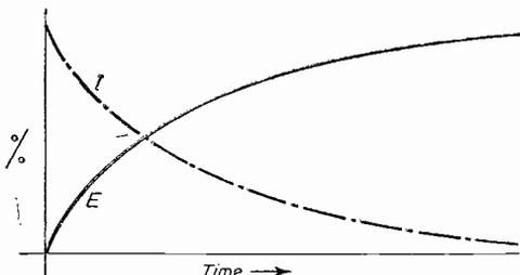
Fig. 2.—Voltage E across, and Current I, flowing into the condenser of Fig. 1 plotted against time.
