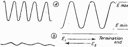
Fig. 3 (Left).—Oscillograms of mismatched and matched conditions of line load respectively. Fig. 4 (Right).—Measurement of VSWR.
