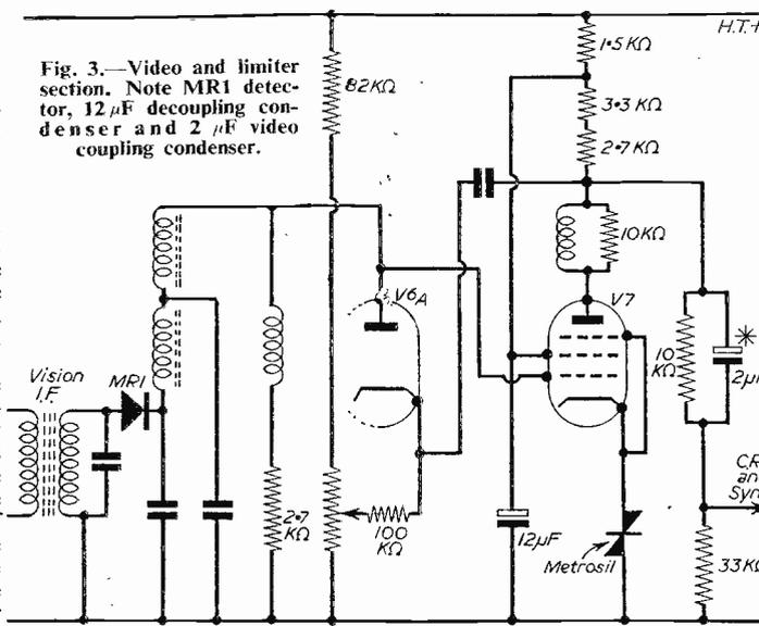
Fig. 3.—Video and limiter section. Note MR1 detector, 12 μF decoupling condenser and 2 μF video coupling condenser.
