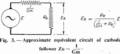
Fig. 3. — Approximate equivalent circuit of cathode follower  $Z_o = \frac{1}{G_m}$ .
