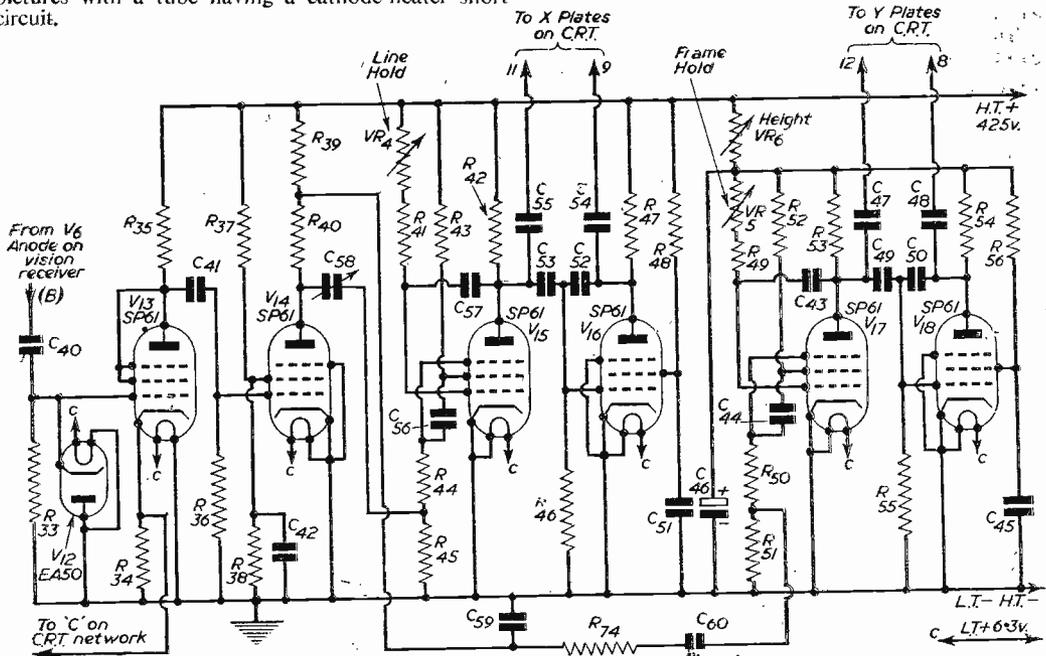
Fig. 1.—The original timebase circuit.
