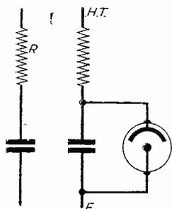
Fig. 1. (Left).—A simple condenser charging circuit. Fig. 3. (Right).—Constant voltage discharge method for a condenser.
