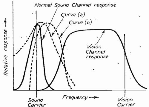
Fig. 90.—The sound and vision responses of a single sideband receiver, showing how the vision signal may gain admittance to the sound channel by curve (a) if the sound channel bandwidth is too wide, or by curve (b) if the sound channel is mis-tuned.
