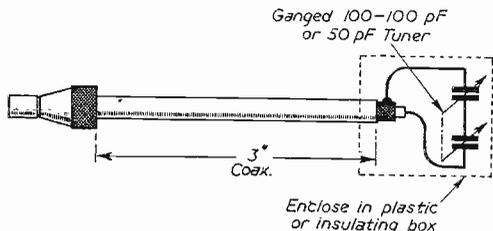
Fig. 6.—A variable capacity stub.
