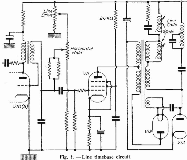
Fig. 1.—Line timebase circuit.
