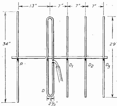
Fig. 2.—A Yagi array with folded dipole.
