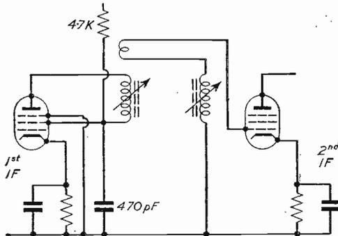
Fig. 7.—The coupled coil.
