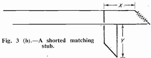
Fig. 3 (b).—A shorted matching stub.
