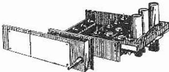
Input 300 ohm balanced line, coverage 54 Mc/s-89 Mc/s and 174 Mc/s-217 Mc/s. Vision I.F.: -45 Mc/s, sound 40.5 Mc/s. Uses 6AK5 RF valve, 6AK5 as mixer, and 6C4 oscillator. Provision for auto-gain control. Dimensions 9in. wide, 6 1/2 in. deep, 4 1/2 in. high, 9in. blank-space. Width including scale-overlap 14in. Four stages permeability tuned. Complete with 3 valves. P. & P. 3/- £2-19.6.
