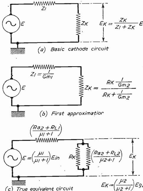
Fig. 3.—Development of the equivalent circuit of the long-tailed pair.
