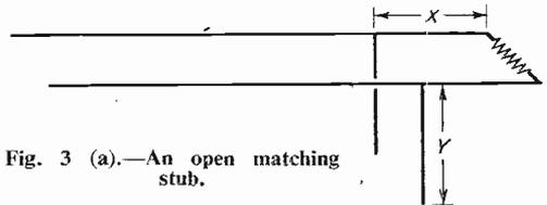
Fig. 3 (a).—An open matching stub.
