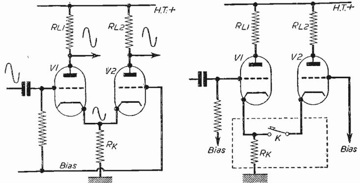
Fig. 1 (left).—Basic long-tailed pair circuit. Fig. 2 (right).—Development of the circuit.
