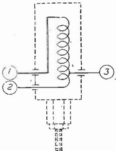
Fig. 5.—Coil Data. Coil LO: Insulate (3); use whole of coil, i.e., connections are (2) and (1).
