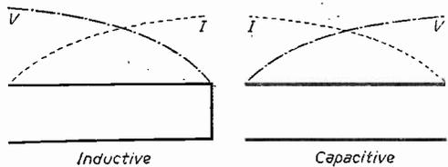
Fig. 4.—Current and voltage relationships in closed and open stubs.
