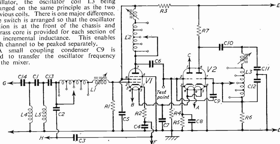
Fig. 1.—Complete circuit of the tuner.
