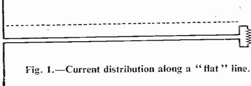
Fig. 1.—Current distribution along a "flat" line.
