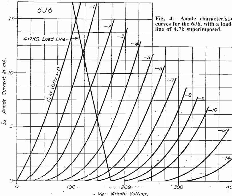
Fig. 4.—Anode characteristic curves for the 6J6, with a load-line of 4.7k superimposed.
