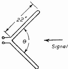
Fig. 3.—Details of a folded "Vee" aerial for Band III.
