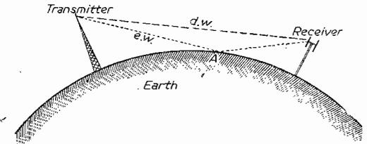
Fig. 3.—Illustrating the direct (dw) and indirect (ew) paths by which energy travels from transmitter to receiver.
