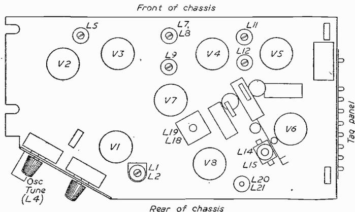
Fig. 5.—Top view of vision and sound unit as in Fig. 4, with coils and components shown.
