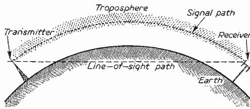
Fig. 2.—Illustrating the fringe area where a line-of-sight path does not exist and the signal is refracted around the curved earth by the influence of the troposphere.
