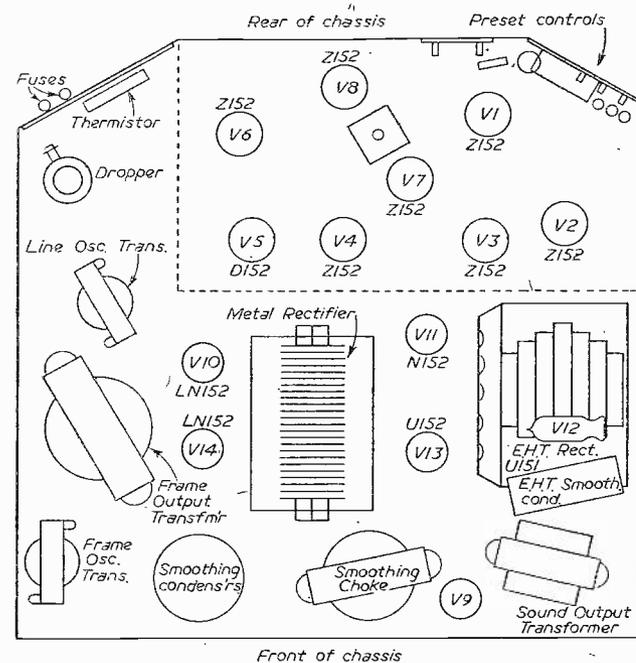
Fig. 4.—Top view of chassis which is mounted at an angle in console receivers.
