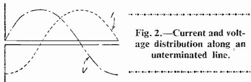
Fig. 2.—Current and voltage distribution along an unterminated line.
