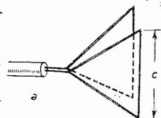
Fig. 4(a).—An arrangement for a semi-horn type of aerial.
