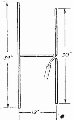
Fig. 1.—A simple half-wave dipole with reflector, showing dimensions.
