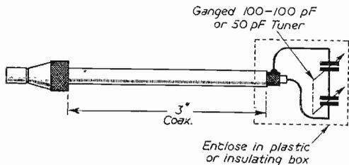
Fig. 6.—A variable capacity stub.
