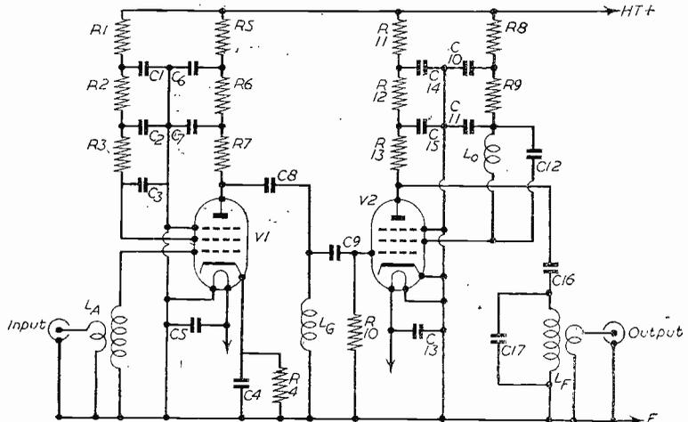
Fig. 2. — Circuit after modification.
