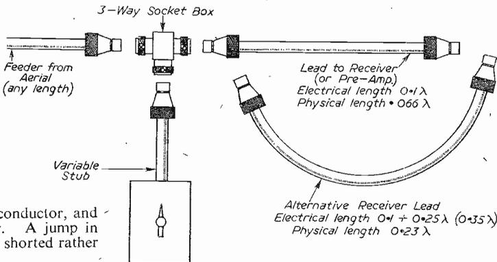
Fig. 7.—Coupling in the variable stub.
