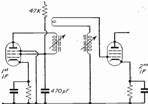
Fig. 7.—The coupled coil.
