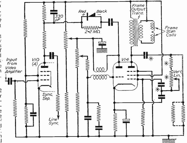
Fig. 3.—Sync separator and frame timebase circuit. (Note that the components marked with a star are linearity feedback components which can cause flashing or arcing at the valve base of V14 if faulty.)
