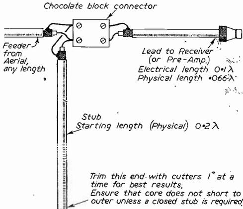
Fig. 5.—A simple matching stub arrangement.
