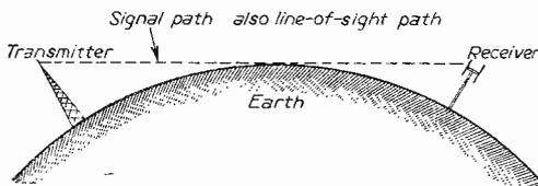
Fig. 1.—Illustrating the service area where the signal follows the line-of-sight path between transmitter and receiver.
