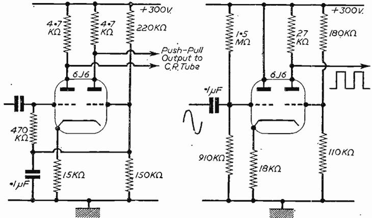
Fig. 5 (left).—Paraphase amplifier circuit for cathode ray tube. Fig. 6 (right).—Long-tailed pair clipper circuit.
