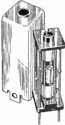
Fig. 6.—A completed coil unit.
