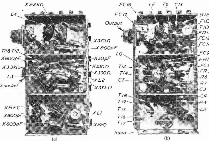
Fig. 4.—Details of the lower chassis. (Left, before modification; Right, after.)
