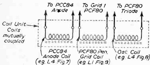
Fig. 9.—An inductively coupled coil unit.
