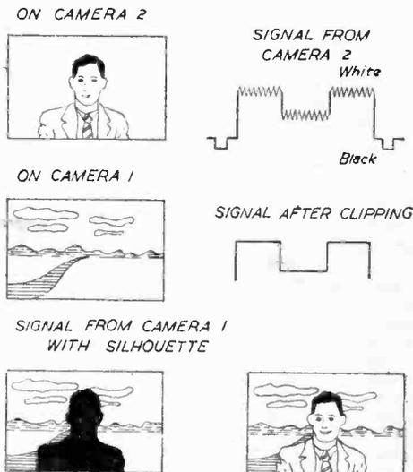
Fig. 6.—Principles of the arrangement known as “ Overlay ”.
