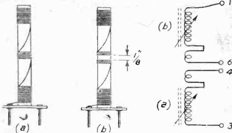
Fig. 8.—Details of the I.F. coils. (a) and (b) windings are identical.
