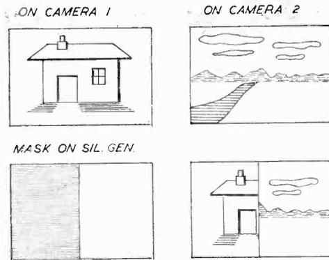
Fig. 4.—How a "wipe" is effected.
