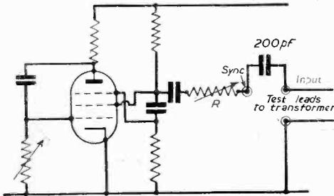
Fig. 1.—Exciting the transformer from a transitoron.
