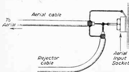
Fig. 1.—Connection of the rejector.
