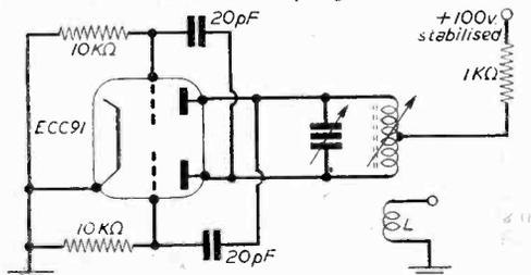
Fig. 4.—Twin triode push-pull oscillator. The coupling coil L comprises two turns wound centrally over the anode coil.
