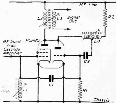
Fig. 8.—A Band III frequency changer circuit.
