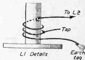
be used. Slip one end of the wire through the earth tag on V1 holder and wind one complete turn; now slip the wire from the former and make a twist at half a turn. Solder the twist and then replace on the former and wind the remaining turns, taking the top end to L2. Fig. 6 shows the method. The turns should be spaced about  $\frac{1}{16}$  in. to  $\frac{1}{8}$  in. apart.
