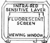
Famous wartime "cats eye" for seeing in the dark. This is an infra-red cell with a screen which lights up (like a cathode ray tube) when the electrons strike it. It follows that as light is rich in infra-red these cells will work as photo cell for burglar alarms, counting circuits. Price 5/- each. Data will be supplied with cells if requested.
