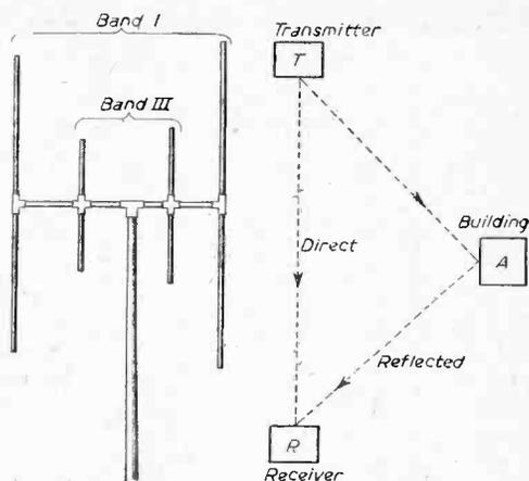
Fig. 9 (left).—A composite aerial for both Band I and Band III. Fig. 10 (right).—Reflected signals.
