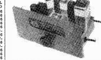
F.M. TUNER UNIT (87 mc/s—105 mc/s), by Jason: As tested and approved by Radio Constructor. Complete Kit of parts to build this modern highly successful unit, drilled chassis and d.b. dial, coils and cans. 4 BVA miniature valves and all components etc., for only **£8.10.0** post free. SUPERIOR TYPE (GLASS DIA.)—Calibrated in Mc/s and illustrated by 2 pilot lamps, 12/6 extra. Includes hand-book with full details, 2/- post free.
