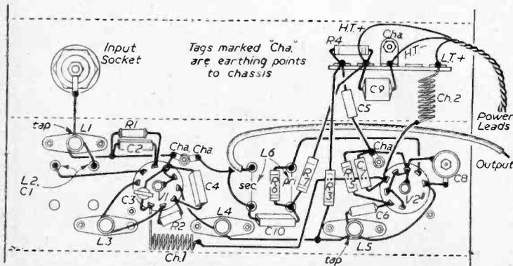
Fig. 7.—Wiring diagram for the fringe model.
