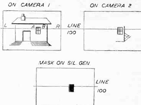
Fig. 1.—Principles of the arrangement known as 'Inlay.' The Inlay equipment described in this article is installed in several television studios and is often used for Inlay, for Wipes, and for Overlay. It is a valuable adjunct to the television service.
