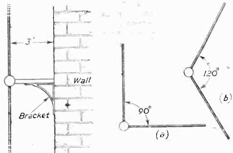
Fig. 3 (left).—Mounting the dipole. Fig. 4 (right).—"L" and "V" type dipoles.
