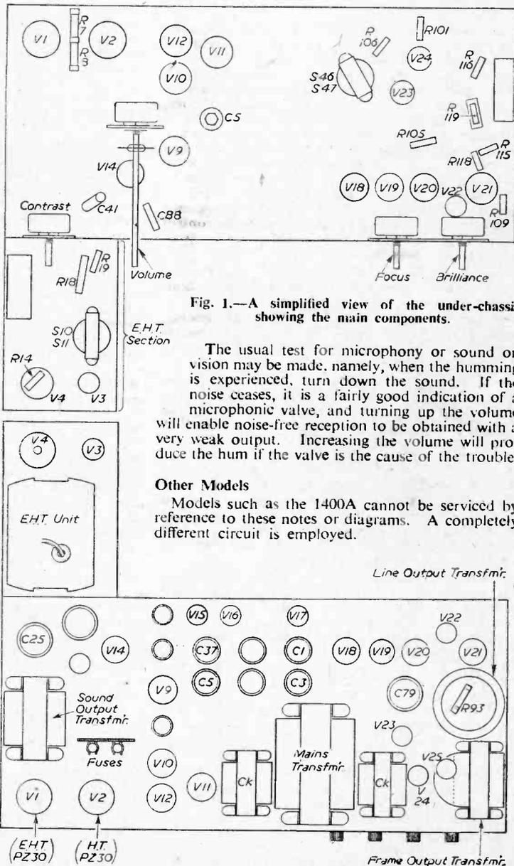
Fig. 1.—A simplified view of the under-chassis showing the main components.
