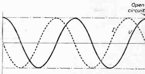
Fig. 2.—Reflected current and voltage.
