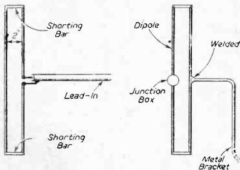
Fig. 5 (left).—A simple method of making a folded dipole. Fig. 6 (right).—Welding the bracket.
