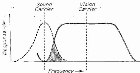
Fig. 2.—The overall response curve of a typical receiver. The vision response full line, and the sound response broken line. The shaded area shows the sound response curve embracing the vision channel passband.
