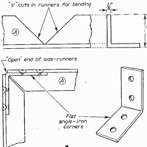
Fig. 2 (upper).—Angle aluminium used for side runners A and B. (Lower) Method of finishing off "open" ends of side runners by means of flat angle irons.
