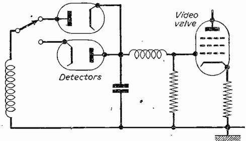
Fig. 4.—Switched grid input for positive or negative modulated carrier.
