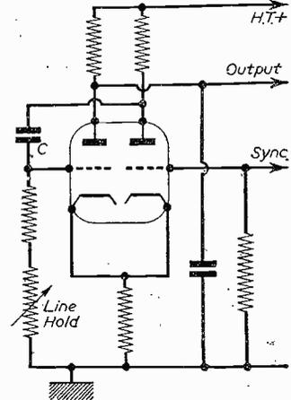
Fig. 8.—Cathode-coupled multi-vibrator.
