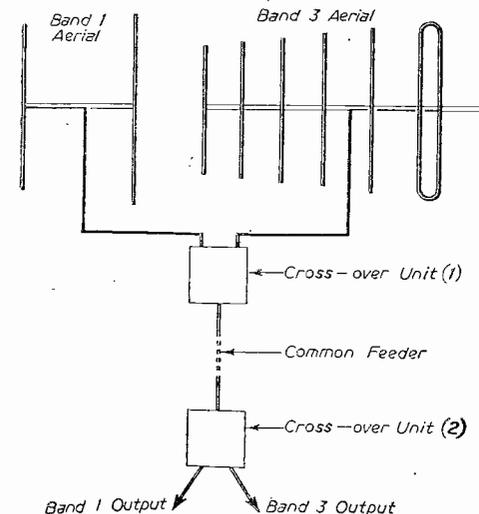
Fig. 19.—It is sometimes worthwhile to utilise two cross-over units to enable a single length of coaxial feeder to connect two aerials to a receiver having separate inputs.
