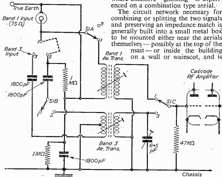
Fig. 16.—The two-band aerial input circuits used in Ferranti receivers.
