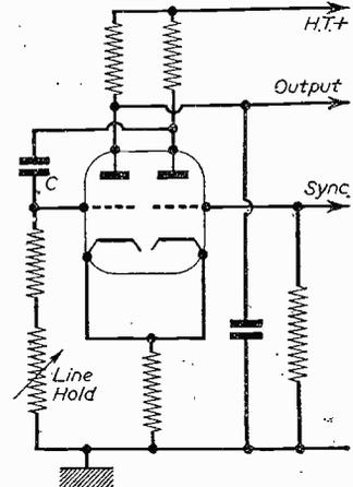
Fig. 8.—Cathode-coupled multi-vibrator.
