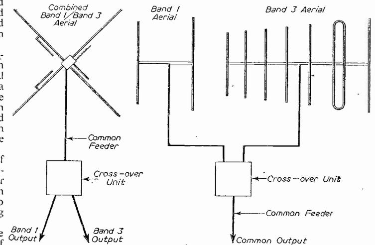
Fig. 17 (left).—A cross-over unit is necessary where a combined Band I/Band III aerial is used with a receiver having separate inputs for the two bands. Fig. 18 (right).—A cross-over unit is also required where separate Band I/Band III aerials are used with a receiver having a common input.
