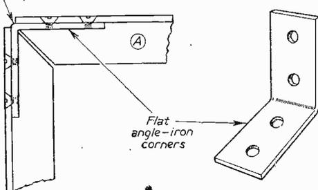
Fig. 2 (upper).—Angle aluminium used for side runners A and B. (Lower) Method of finishing off "open" ends of side runners by means of flat angle irons.
