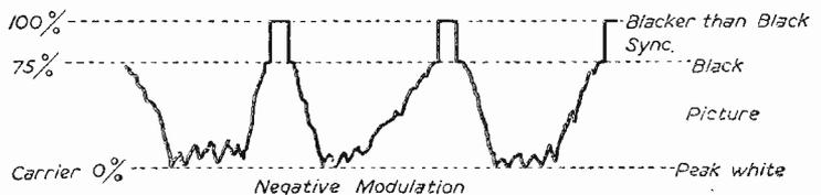
Fig. 1.—Positive and negative modulation.
