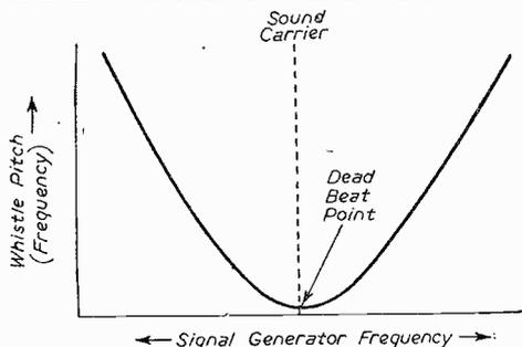
Fig. 5.—A diagrammatic illustration of the dead-beat point.
