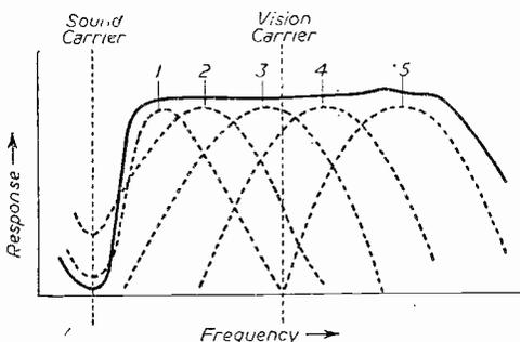
Fig. 3.—Showing how stagger-tuning in the vision channel can produce a substantially flat response curve. This is due to the added effect of five tuned circuits resonating about the vision carrier frequency.
