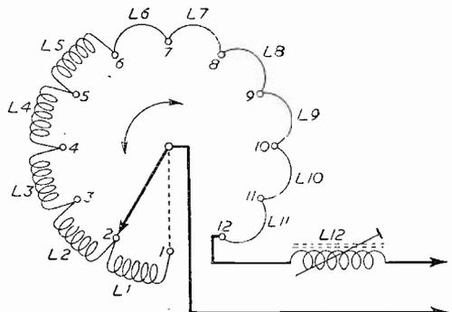
Fig. 15.—A single section of the channel switching arrangement used in Pye, Invicta and Pam receivers.
