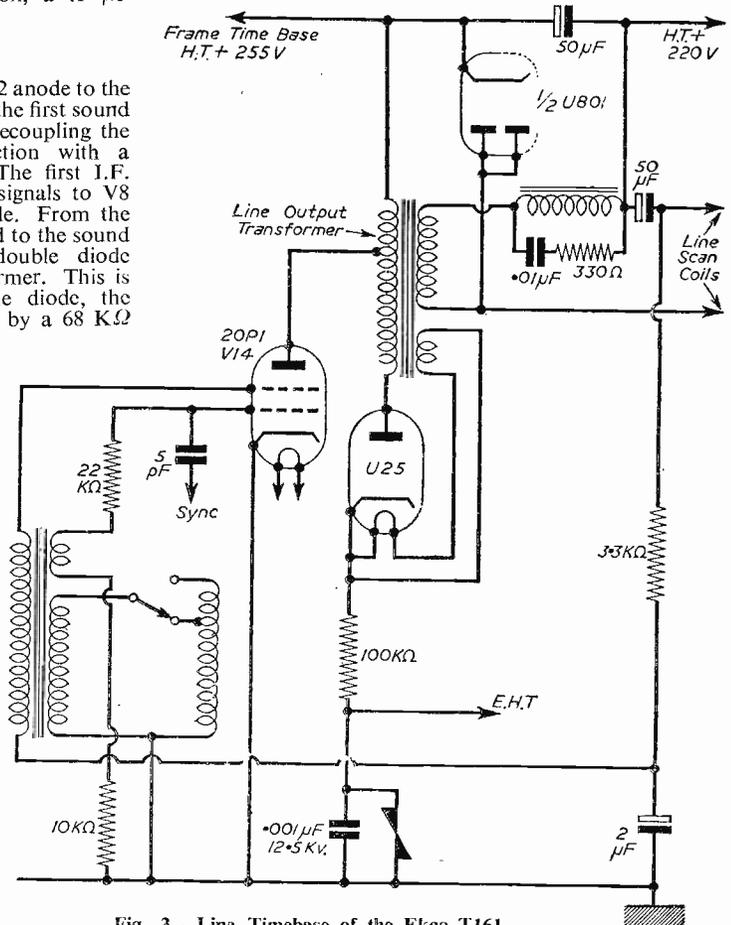
Fig. 3.—Line Timebase of the Ekco T161.
