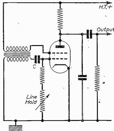
Fig. 7.—Typical blocking oscillator.
