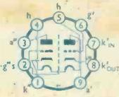
**B319/PCC84.** Double triode designed for use as a series cascode R.F. amplifier with the accompanying advantages of high gain and good signal to noise ratio. The high slope at low anode voltage ensures efficient operation at H.T. supplies of 180V. The maximum heater-cathode has been increased to 250V to meet the special requirements of this application.
