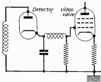
Fig. 2.—Negative grid input for grid-modulated tubes. (Negative modulated carrier.)
