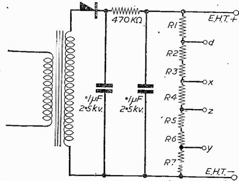
Fig. 2.—Circuit for location of the focusing anode.
