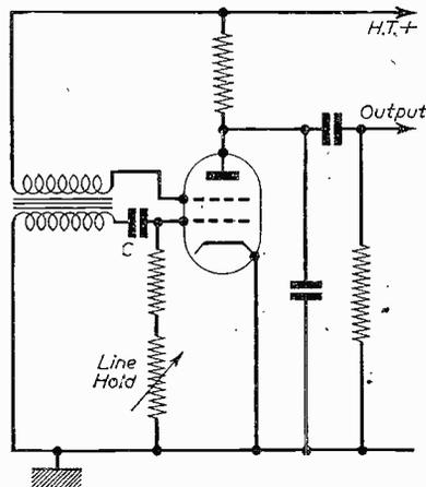
Fig. 7.—Typical blocking oscillator.
