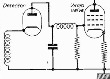
Fig. 3.—Positive grid input for cathode-modulated carrier. (Positive modulated carrier.)
