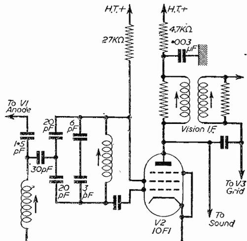
Fig. 1.—The Frequency Changer Stage.
