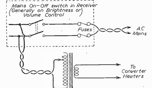
Fig. 27.—If a separate heater transformer is used the mains input should be arranged as shown here.
