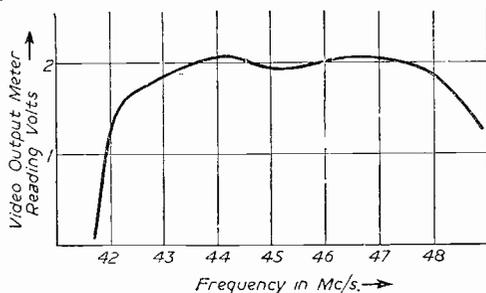
Fig. 4.—Showing how a graphic representation of an overall response curve can be obtained by plotting the generator frequency within the vision passband against the reading given on the video output indicator.
