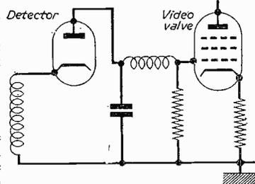
Fig. 3.—Positive grid input for cathode-modulated carrier. (Positive modulated carrier.)
