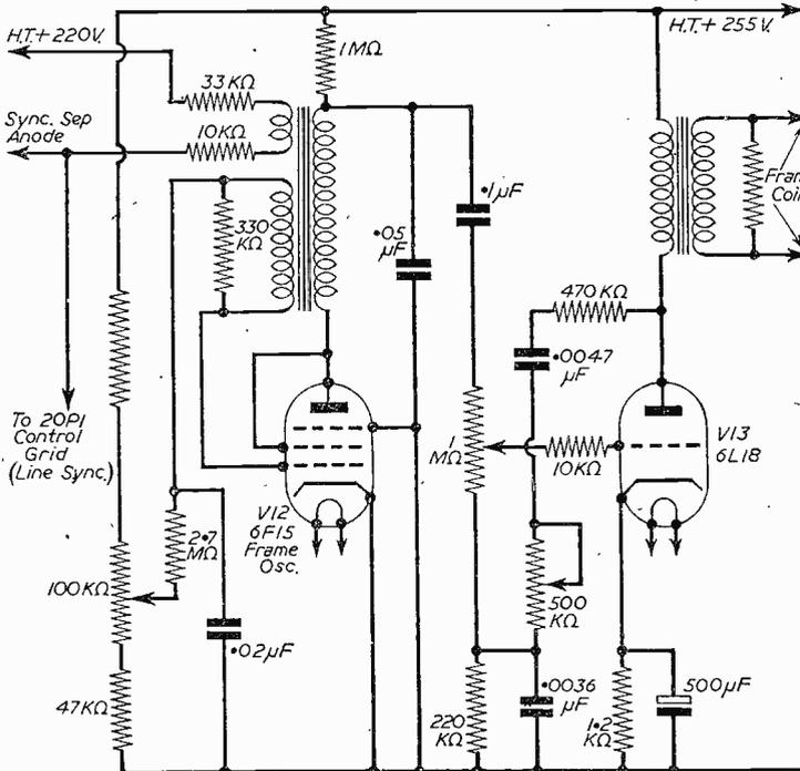
Fig. 4.—Frame Timebase and feed to sync separator.
