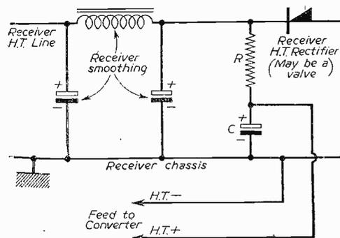
Fig. 25.—One method of feeding power to the P.T. converter.
