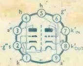
**B319/PCC84.** Double triode designed for use as a series cascode R.F. amplifier with the accompanying advantages of high gain and good signal to noise ratio. The high slope at low anode voltage ensures efficient operation at H.T. supplies of 180V. The maximum heater-cathode has been increased to 250V to meet the special requirements of this application.
