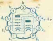
**LZ319/PCF80.** Triode pentode designed for use as a frequency changer following the B319/PCC84 cascode amplifier. The LZ319/PCF80 operates efficiently at H.T. voltage of 170-180, and gives a high conversion gain with standard circuitry.
