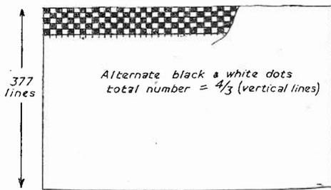
Fig. 1.—Checker board pattern.
