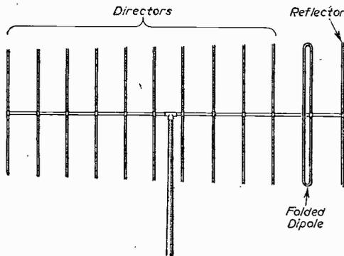
Fig. 3.—A 12-element array.
