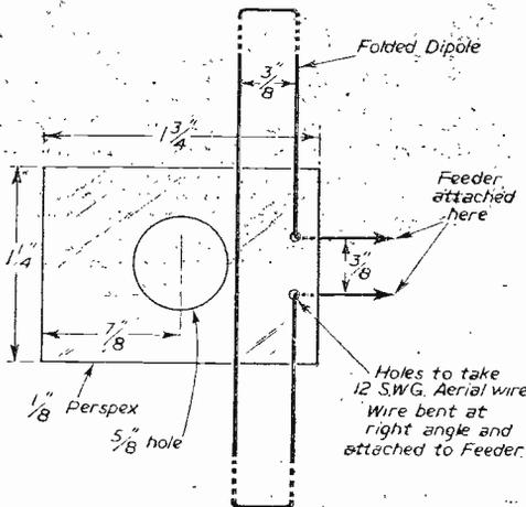
Figs. 2 and 3.—Method of connecting up the elements, and the folded dipole mounting block.
