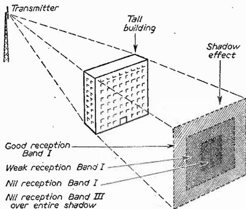
Fig. 1.—An illustration of the shadow effect.
