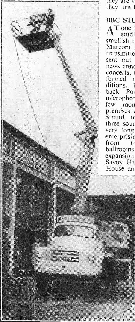
Destined to be known as "The Thing," this mobile hydraulic platform, mounted on a Bedford chassis, can raise a cameraman and camera up to heights of 40ft. or more. It is an Associated Rediffusion requirement. Its main advantage is that it obviates the necessity for erecting scaffolding when a high angle camera position is needed.
