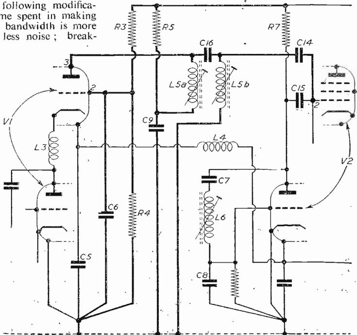
Fig. 2.—Modifications to the P.T. Converter shown in heavy lines.
