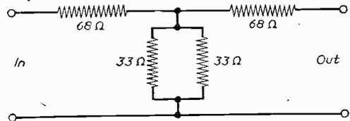
Fig. 6.—Circuit of an attenuator.
