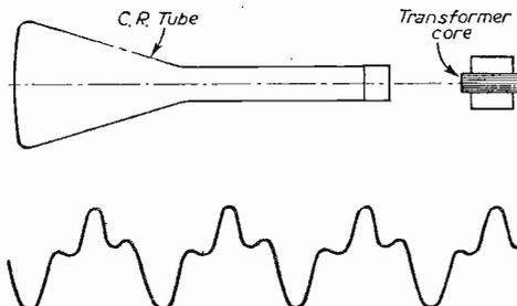
Fig. 21 (Top).—Positioning the transformer and tube base.
