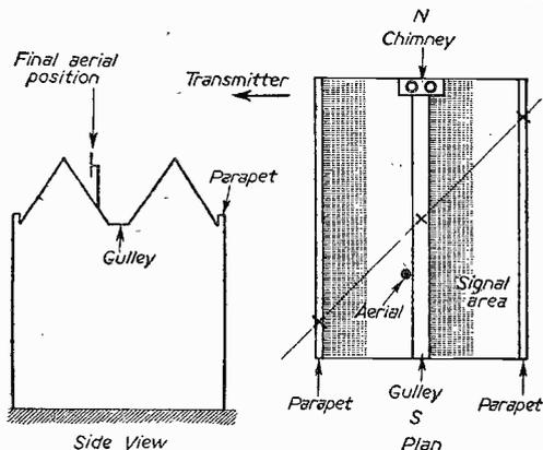
Fig. 2.—Illustrating the final positioning of an aerial.
