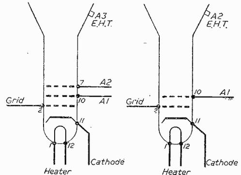
Fig. 1.—Showing pentode base and internal connections.
