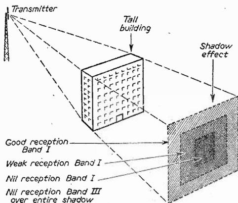
Fig. 1.—An illustration of the shadow effect.
