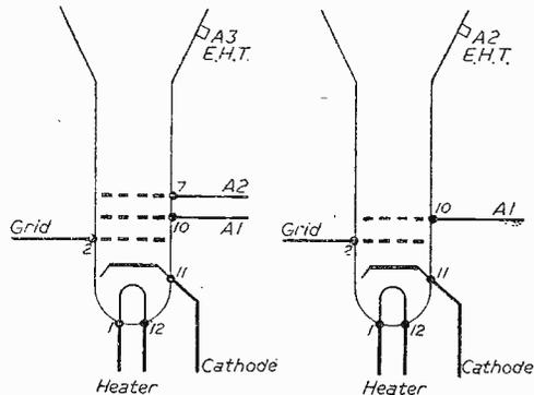
Fig. 1.—Showing pentode base and internal connections. Fig. 1a.—Showing tetrode base and internal connections.
