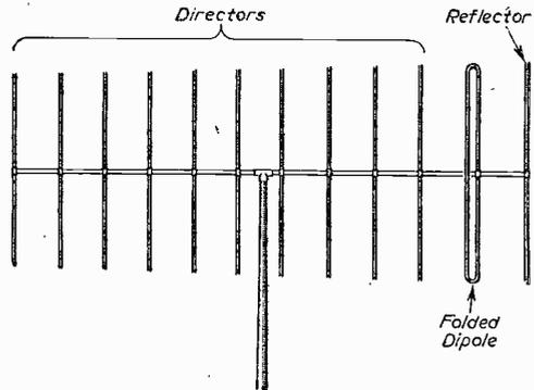
Fig. 3.—A 12-element array.
