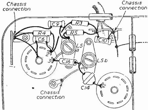
Fig. 1.—Location of the new coil L5a and new position of existing components in the P.T. Converter.
