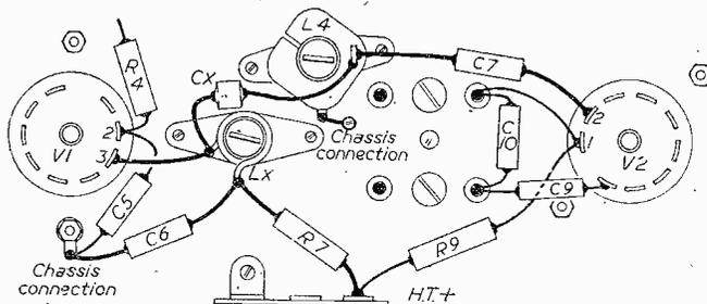
Fig. 3.—Modifications to the Teletron Converter. Note new position of L4.
