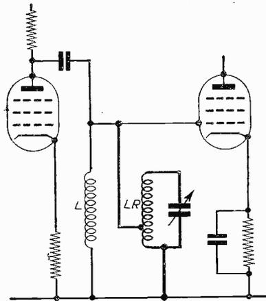
Fig. 4.—A grid rejector.
