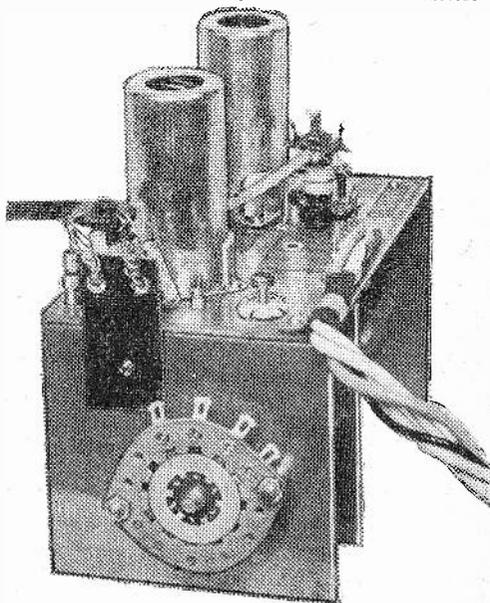
This rear view of the V.M. Tuner clearly shows switch SW5, referred to last month.
