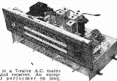
This is a 7-valve A.C. mains operated receiver. An exceptional performer on long, medium and short A.M. bands and on the new V.H.F. band. It is an ideal unit for a quality radiogram. Special features include magic eye tuning indicator, extra long scale and pointer travel—latest circuitry employing full A.V.C. feedback, etc., etc. Undoubtedly one of the finest AM/FM chassis available today. Chassis size 17in. x 6in. x 7in. Price £23.17/6. carriage, packing and insurance 20/- extra.
