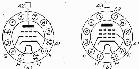
Fig. 2.—Showing tetrode base (a) and pentode base (b).
