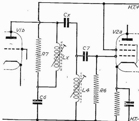
Fig. 4.—Circuit of the modifications to the Teletron Converter. Cx is 2 pF, and Lx consists of three turns widely spaced.
