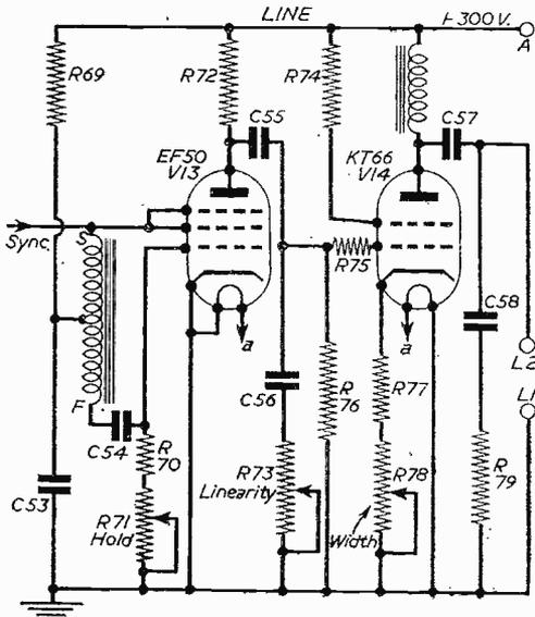
Fig. 12.—Typical simple form of line timebase.
