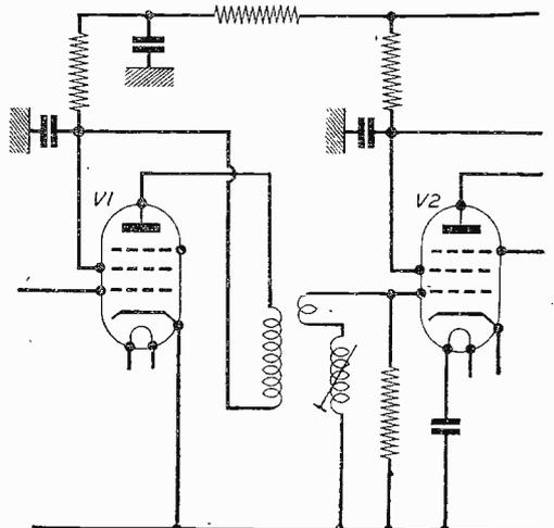
Fig. 2.—The coupling coil at the "top" of the grid coil.
