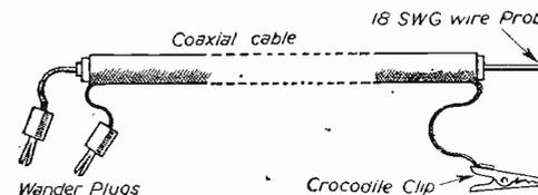
Fig. 20.—Details of the test lead.
