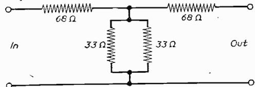
Fig. 6.—Circuit of an attenuator.
