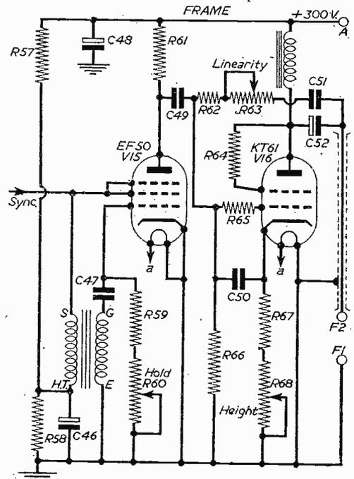
Fig. 13.—A simple frame timebase.
