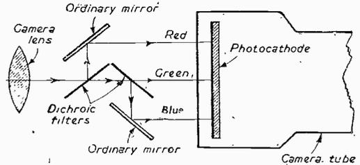
Fig. 3.—Showing how the three images are produced side by side for the line sequential system.
