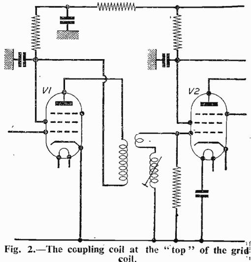
Fig. 2.—The coupling coil at the "top" of the grid coil.
