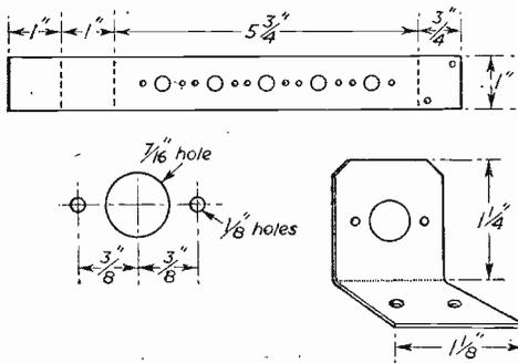
Figs. 14 and 15.—Details of the potentiometer bracket.
