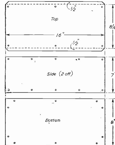
Figs. 17, 18 and 19.—Top, sides and bottom of chassis.
