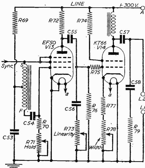
Fig. 12.—Typical simple form of line timebase.
