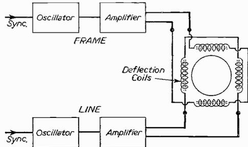
Fig. 14.—This block diagram shows how the two timebases are connected to the scanning or deflection coils in order to move the spot in two directions.
