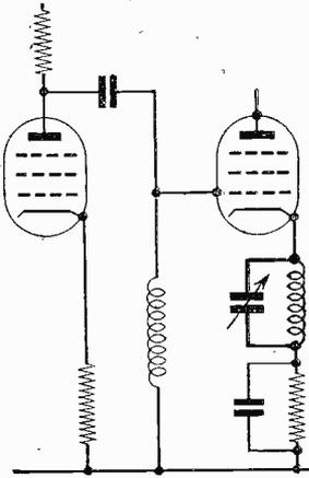
Fig. 5.—A cathode rejector.
