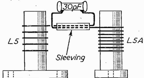
Fig. 5.—How the coupling condenser between L5 and L5A is arranged.
