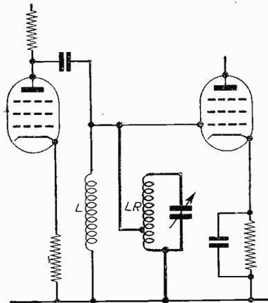
Fig. 4.—A grid rejector.
