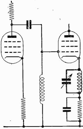
Fig. 5.—A cathode rejector.
