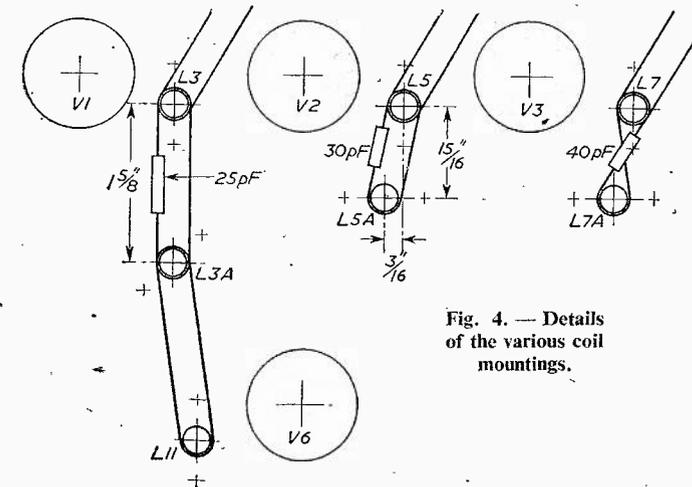
Fig. 4. — Details of the various coil mountings.
