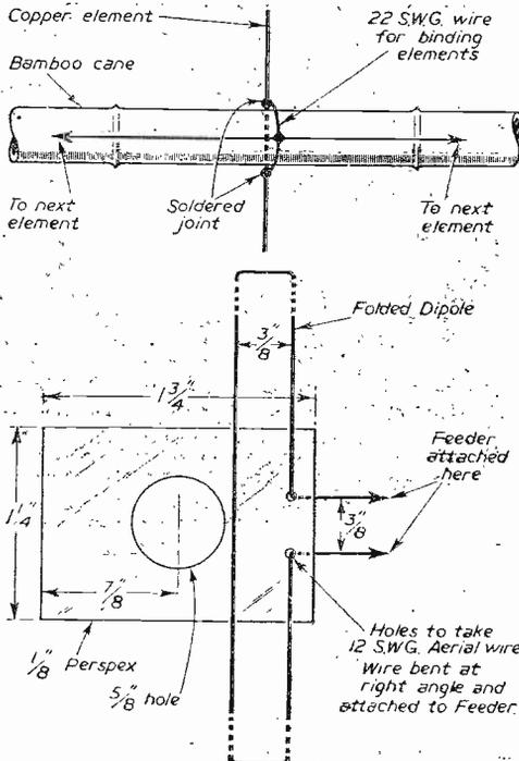
Figs. 2 and 3.—Method of connecting up the elements, and the folded dipole mounting block.
