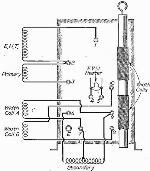
Fig. 3.—Details of the line transformer.
