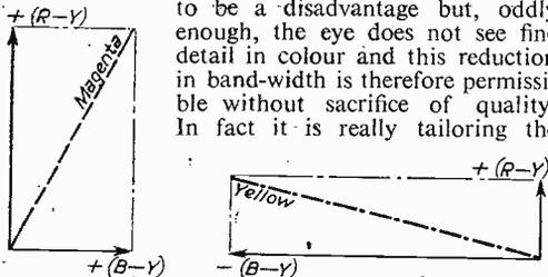
Fig. 3.—Showing how a variation of colour is produced by combining the signals of different amplitudes.
