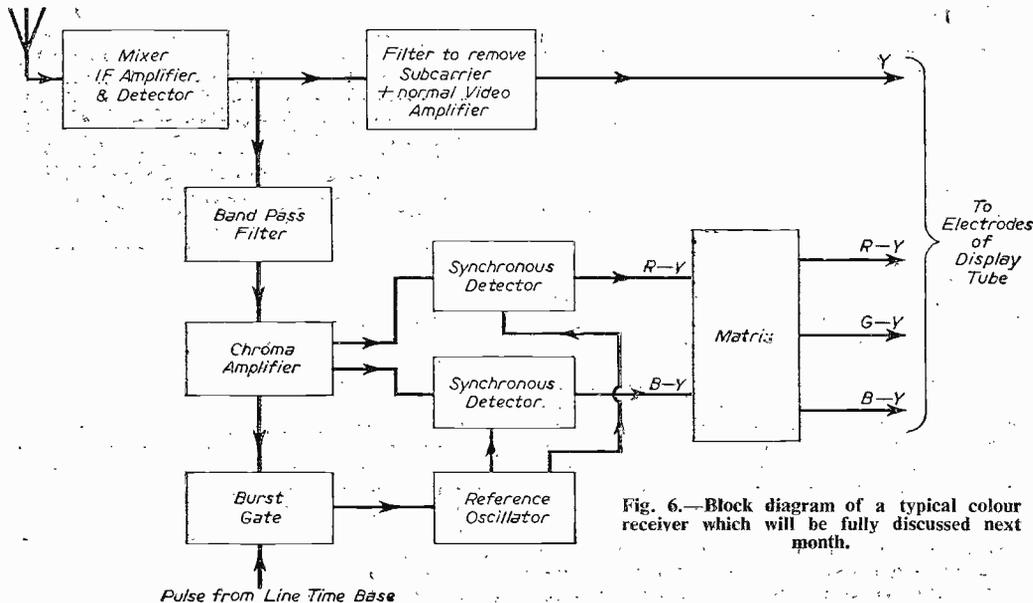
Fig. 6.—Block diagram of a typical colour receiver which will be fully discussed next month.
