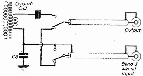
Fig. 3.—Output switching.
