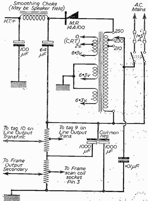
Fig. 5.—Details of the power supply.
