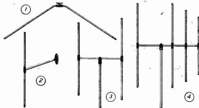
Fig. 17.—A typical range of television aerials. (1) Indoor or loft model; (2) single dipole; (3) "H," and (4) "H" with two directors.
