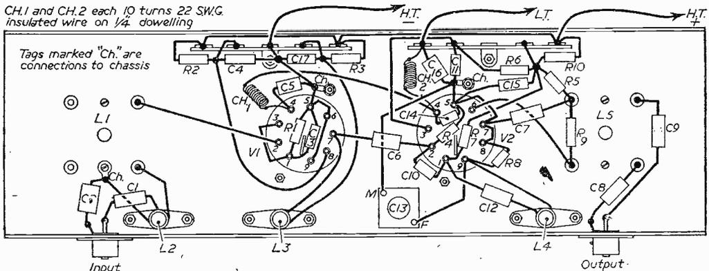
Fig. 1.—Layout and wiring of the converter.
