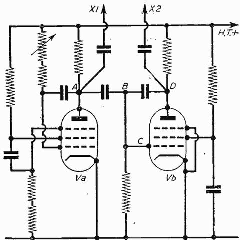
Fig. 6.—Typical paraphase circuit.
