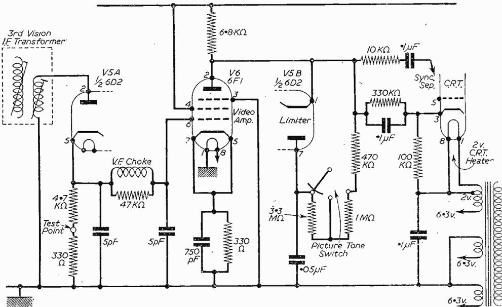
Fig. 2.—Circuit showing the C.R.T. wiring.
