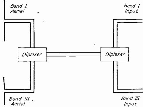
Fig. 6.—Method of using a single feeder.
