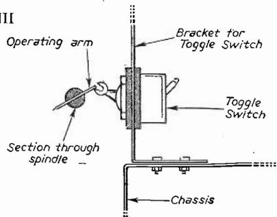
Fig. 5.—Method of mounting power supply switch.
