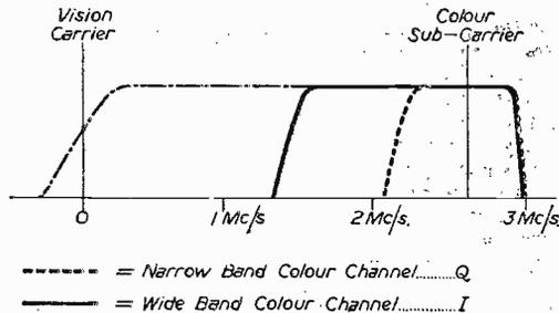
Fig. 5.—Narrow and wide bandwidth response curves.
