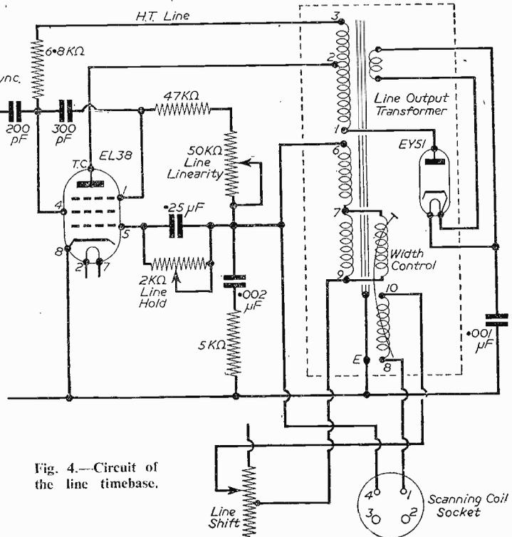
Fig. 4.—Circuit of the line timebase.
