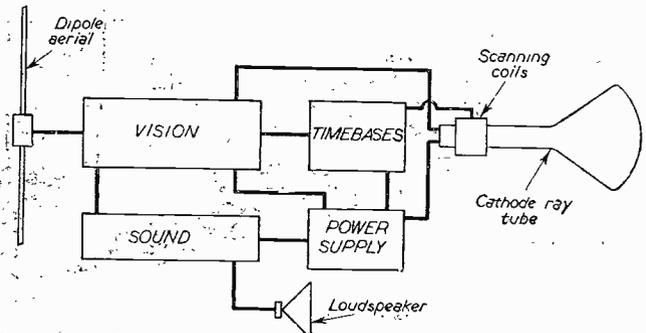
Fig. 15.—Block diagram of a modern television receiver showing the essential sections.
