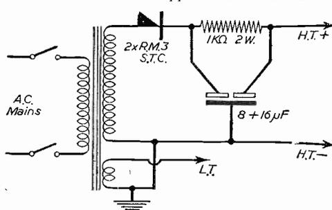
Fig. 4.—Suitable power supply unit.
