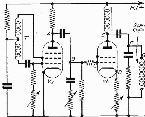
Fig. 7.—Blocking oscillator stage with amplifier.
