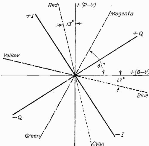
Fig. 2.—Phase diagram showing the relative phase of the (R-Y) and (B-Y) signals, and also of the I and Q signals.
