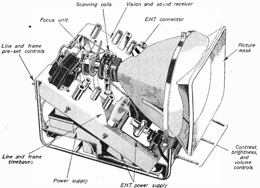
Fig. 16.—A home-built television receiver with the important parts identified.
