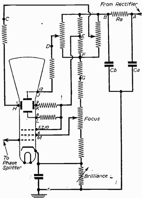
Fig. 2.—Testing points on electrostatic EHT.
