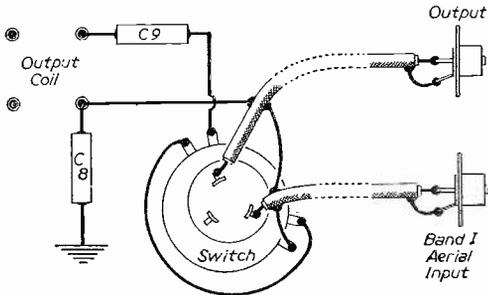
Fig. 8.—Practical arrangement of Fig. 3.
