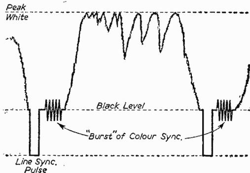
Fig. 4.—Position of the colour sync burst.
