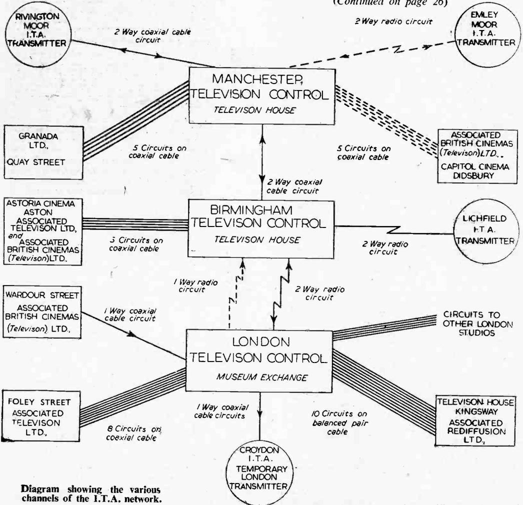
Diagram showing the various channels of the I.T.A. network.
