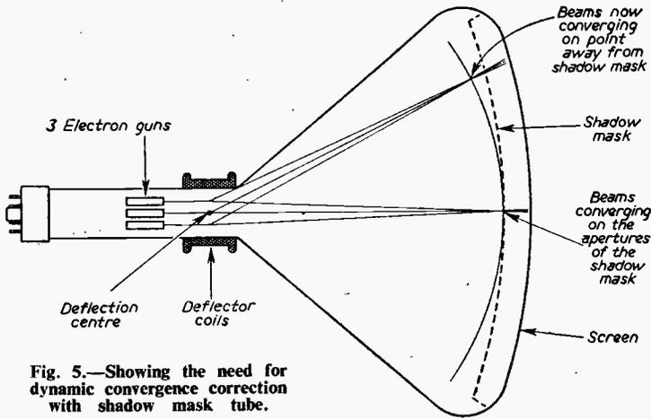
Fig. 5.—Showing the need for dynamic convergence correction with shadow mask tube.
