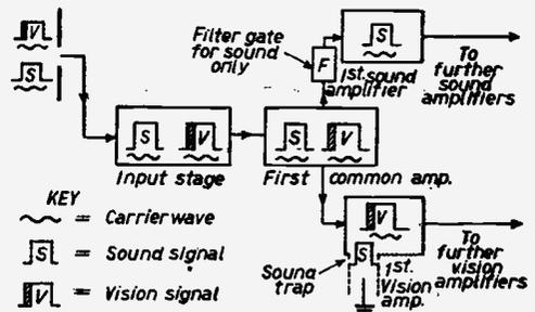
Fig. 19.—Block diagram in which the audio and video signals are traced through a "straight" receiver.
