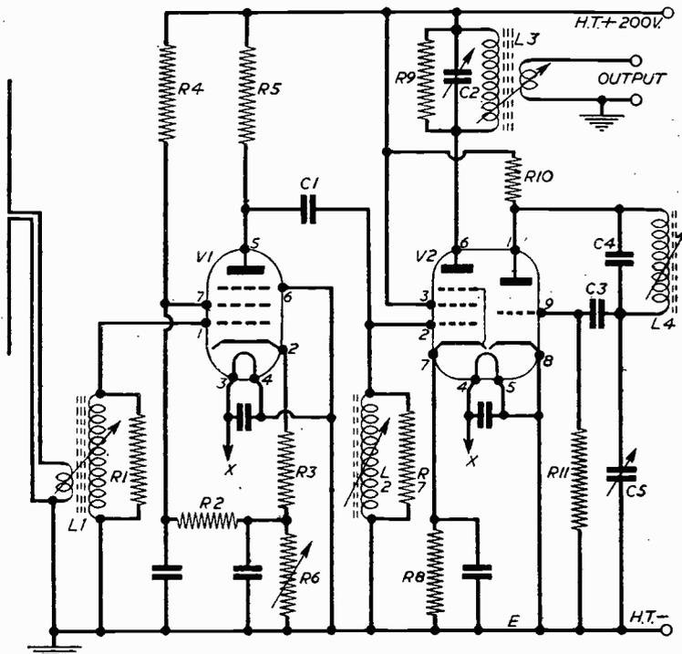
Fig. 6.—Circuit diagram of the Band I converter.
