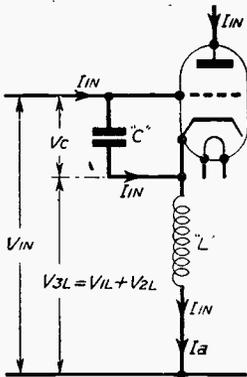
Fig. 2.—Grid-cathode capacity (C) and circuit constants.
