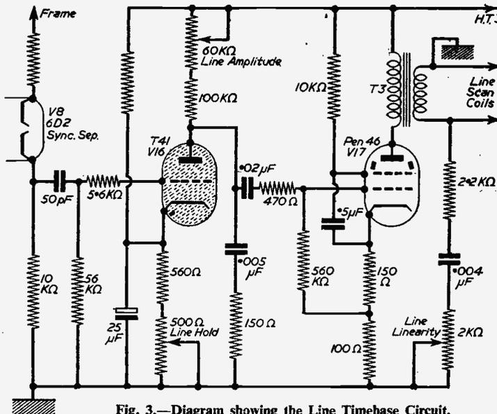
Fig. 3.—Diagram showing the Line Timebase Circuit.
