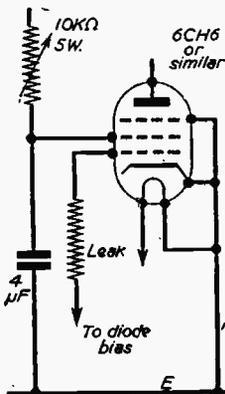
Fig. 12.—Video output with variable bias and variable screen volts.
