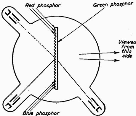
Fig. 1.—The Baird "Telechrome" tube.
