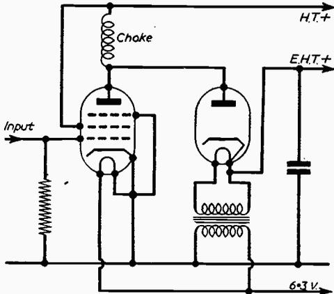
Fig. 1.—Ringing choke output circuit.
