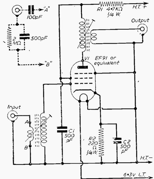
Fig. 1.—Circuit diagram of amplifier using EF91.
