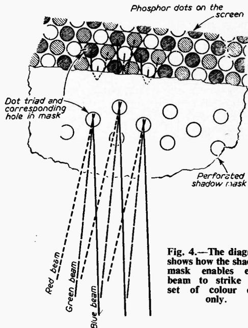
Fig. 4.—The diagram shows how the shadow mask enables each beam to strike one set of colour dots only.
