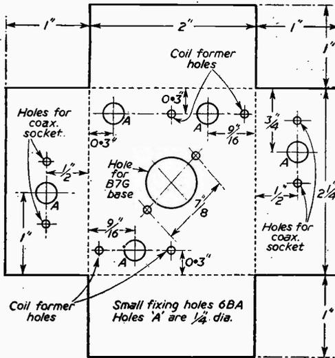
Fig. 2.—Showing drilling and fixing hole details.
