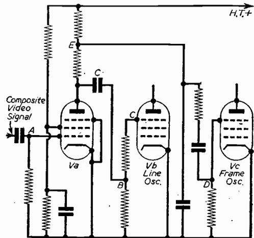
Fig. 8.—A typical sync circuit.
