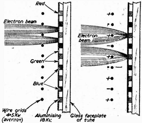
Fig. 2.—Showing the focus action of the wire grids.
