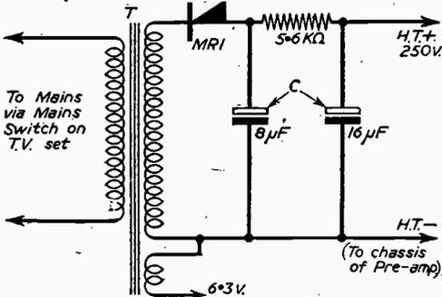
Fig. 4.—The circuit diagram of the power unit. MR1—Any metal rectifier or combination of rectifiers giving 250 volts at 15 mA. (2 RM1 in series.)
