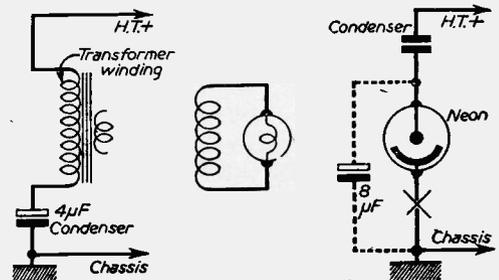
Figs. 9, 10 and 11.—Testing for continuity; an oscillator tester, and (right) a condenser test.
