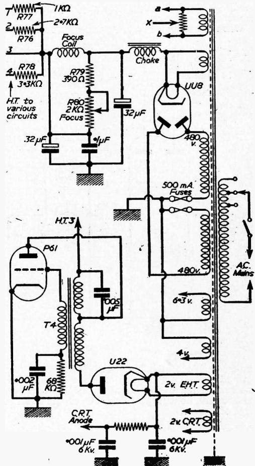
Fig. 1.—Diagram showing Mains supply H.T. wiring and E.H.T. circuit. Heater winding a-b supply sound valves V13 and V14 which are susceptible to hum.
