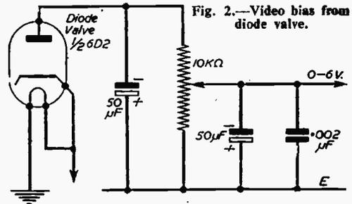
Fig. 2.—Video bias from diode valve.
