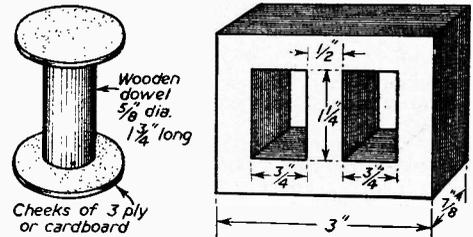
Fig. 2. (Left).—The choke former. Fig. 3 (Right).—Transformer core.
