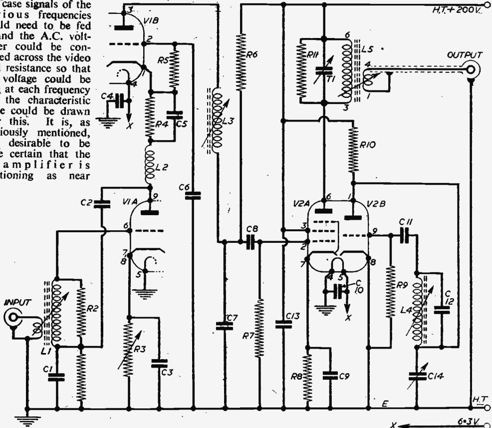
Fig. 4.—Circuit diagram of the Band III converter.
