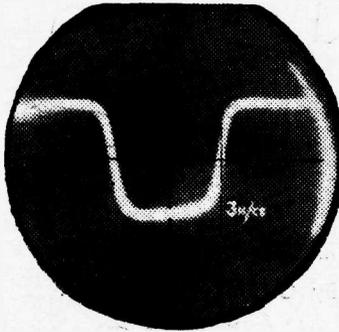
Fig. 3.—Shows the overall response of the I.F. unit.
