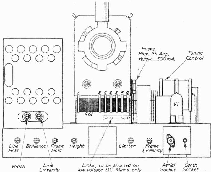
Fig. 2.—A rear chassis view.
