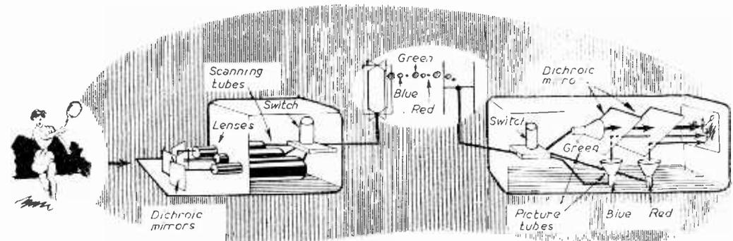
Fig. 37.—The dichroic mirror system of the R.C.A.
