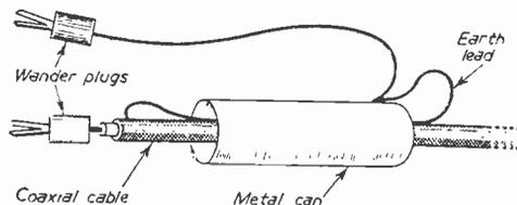
Fig. 18.—Simple screened connector.
