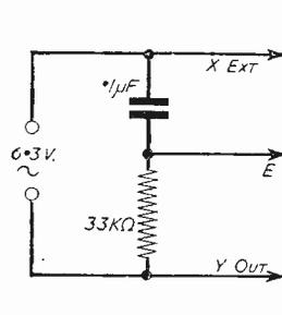
Fig. 26.—Circuit for checking phase displacement.
