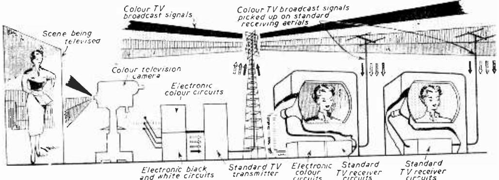
Fig. 34.—How the colour system used by R.C.A. is used to pick up a signal and reproduce it in either colour or black and white.
