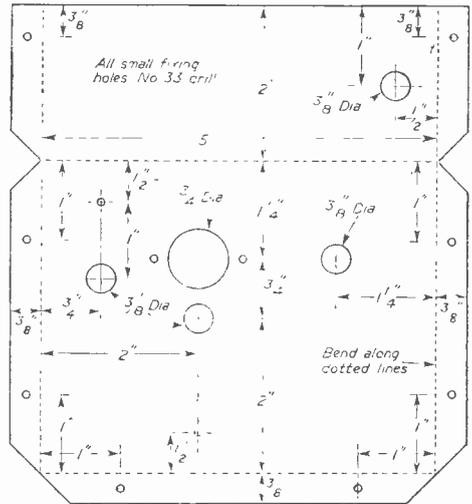
Fig. 2. Chassis bending and drilling details.
