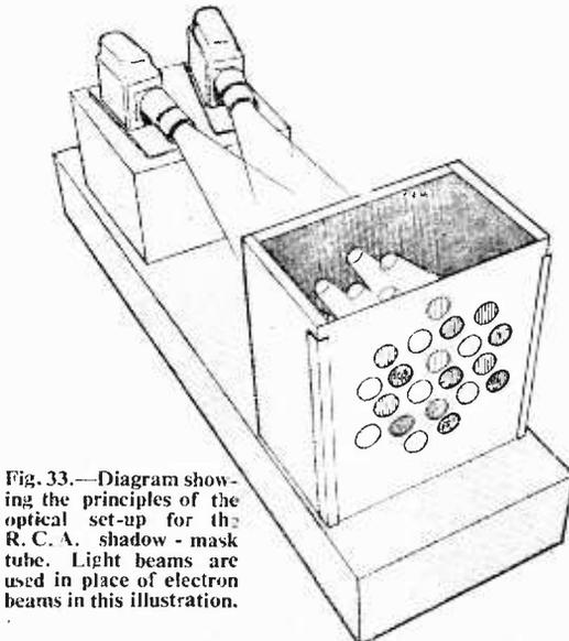
Fig. 33.—Diagram showing the principles of the optical set-up for the R. C. A. shadow-mask tube. Light beams are used in place of electron beams in this illustration.
