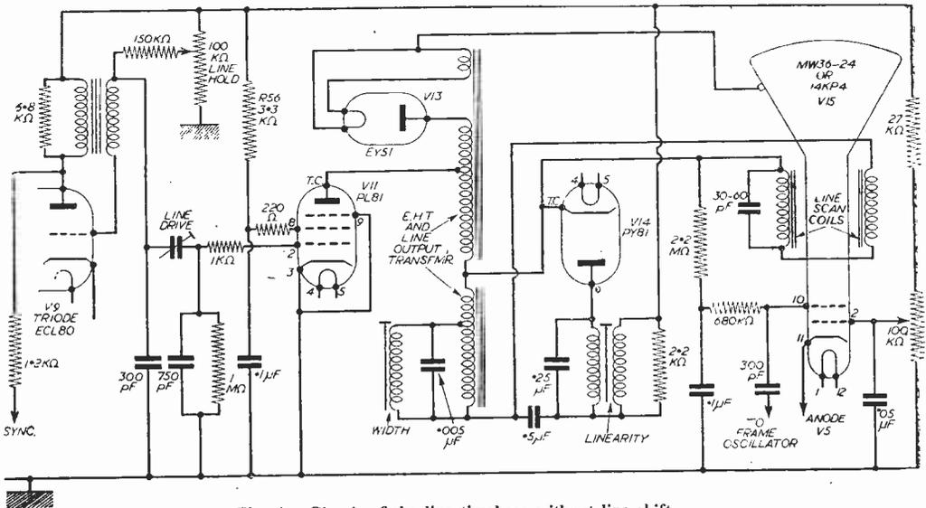
Fig. 4.—Circuit of the line timebase without line shift.
