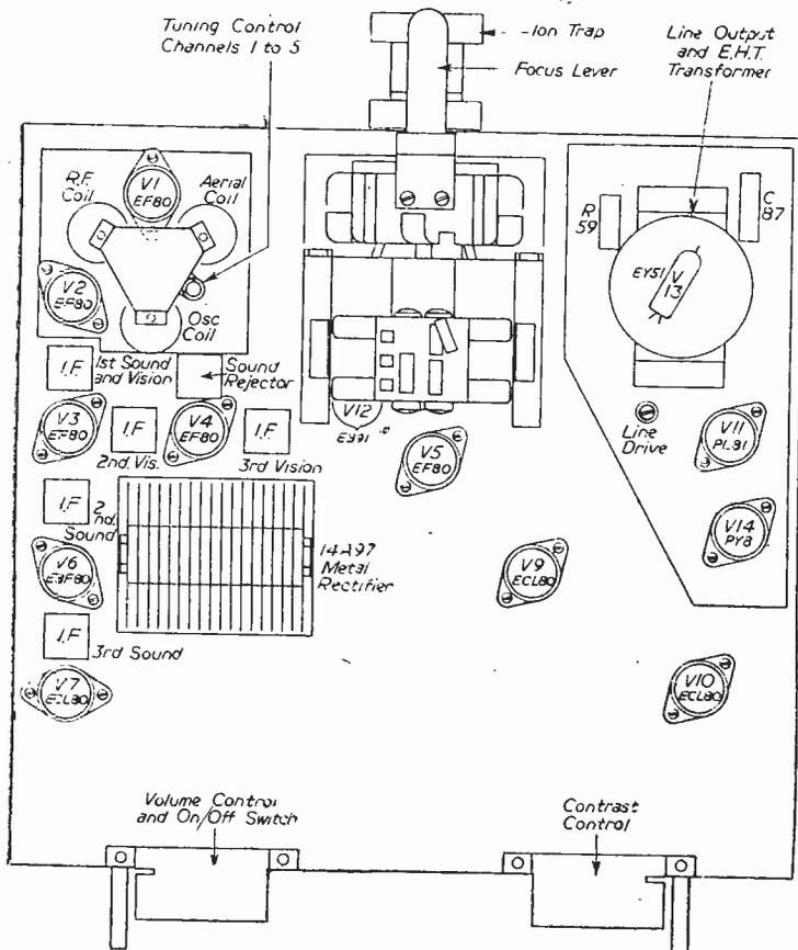
Fig. 1.—Above chassis view of the main parts.
