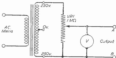
Fig. 17.—Circuit for sensitivity checking.
