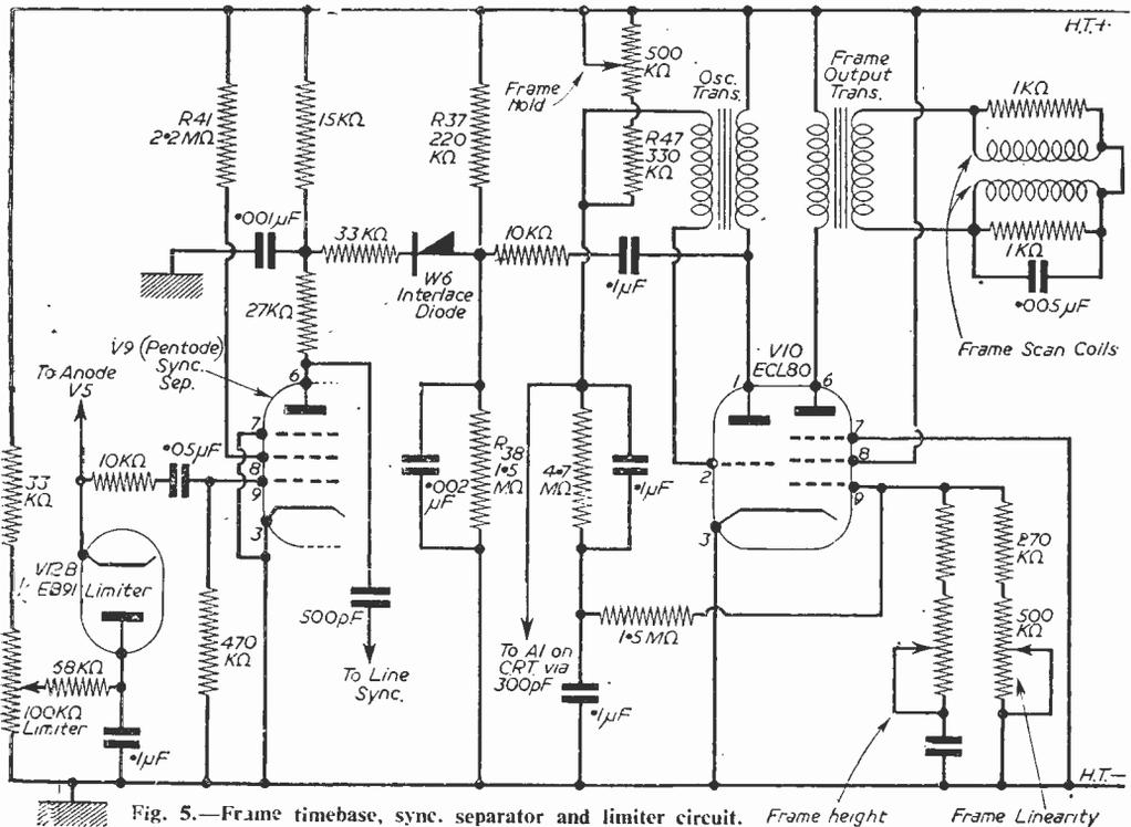
Fig. 5.—Frame timebase, sync separator and limiter circuit. Frame height Frame Linearity
