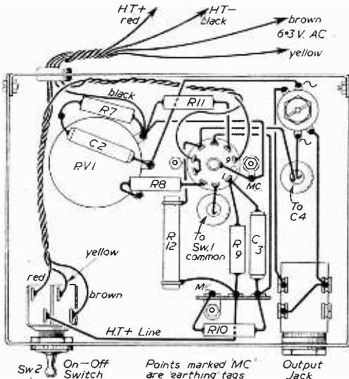
Fig. 4.—Under chassis wiring scheme.
