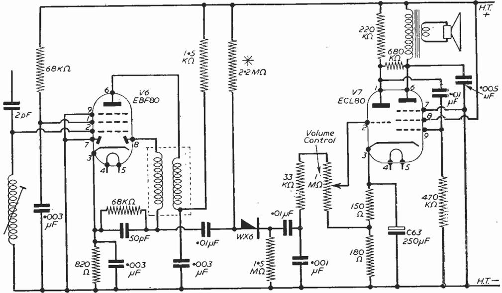
Fig. 7.—Sound I.F., detector, limiter and output circuit.
