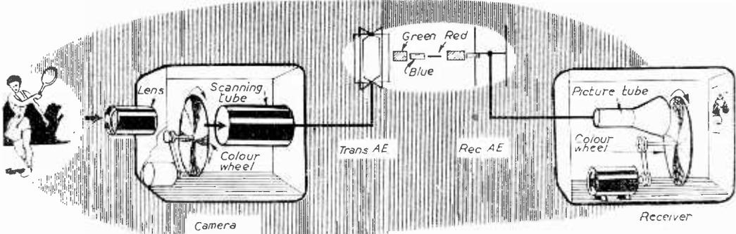
Fig. 36.—A disc colour system as used by the C.B.S. of America.
