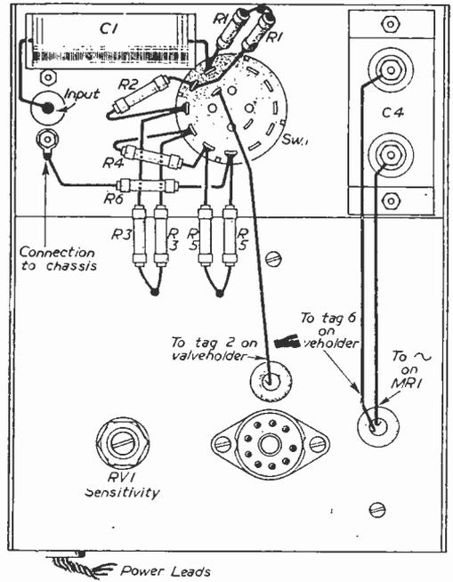
Fig. 5.—Above chassis and panel wiring details.
