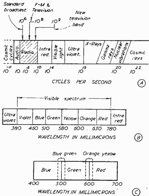
Fig. 32.—The complete electromagnetic spectrum (a); the visible spectrum (b) and (c) simplification for colour television.
