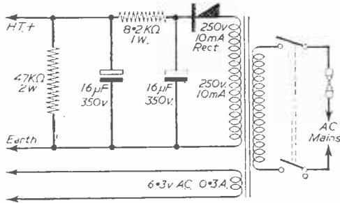
Fig. 3. A mains power supply unit.
