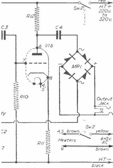
Fig. 1. Circuit diagram of the valve voltmeter.
