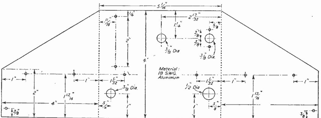
Fig. 6.—Case bending and drilling details.
