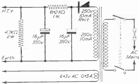
Fig. 3. A mains power supply unit.
