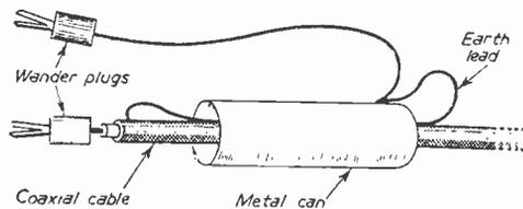
Fig. 18.—Simple screened connector.
