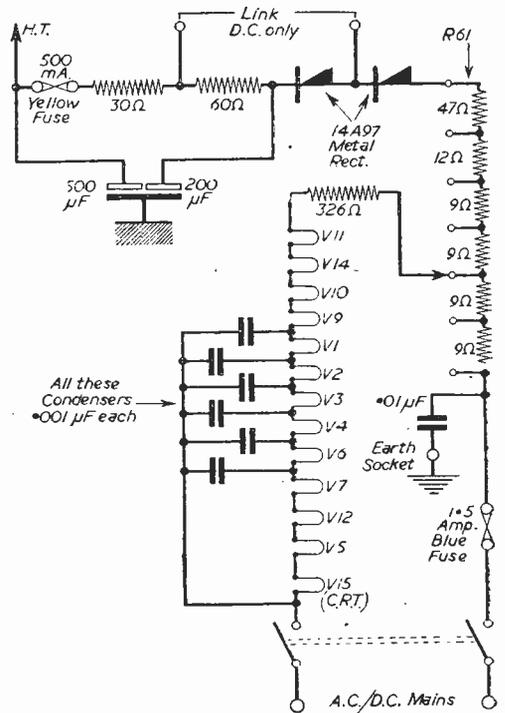
Fig. 6.—Circuit of the mains supply section.
