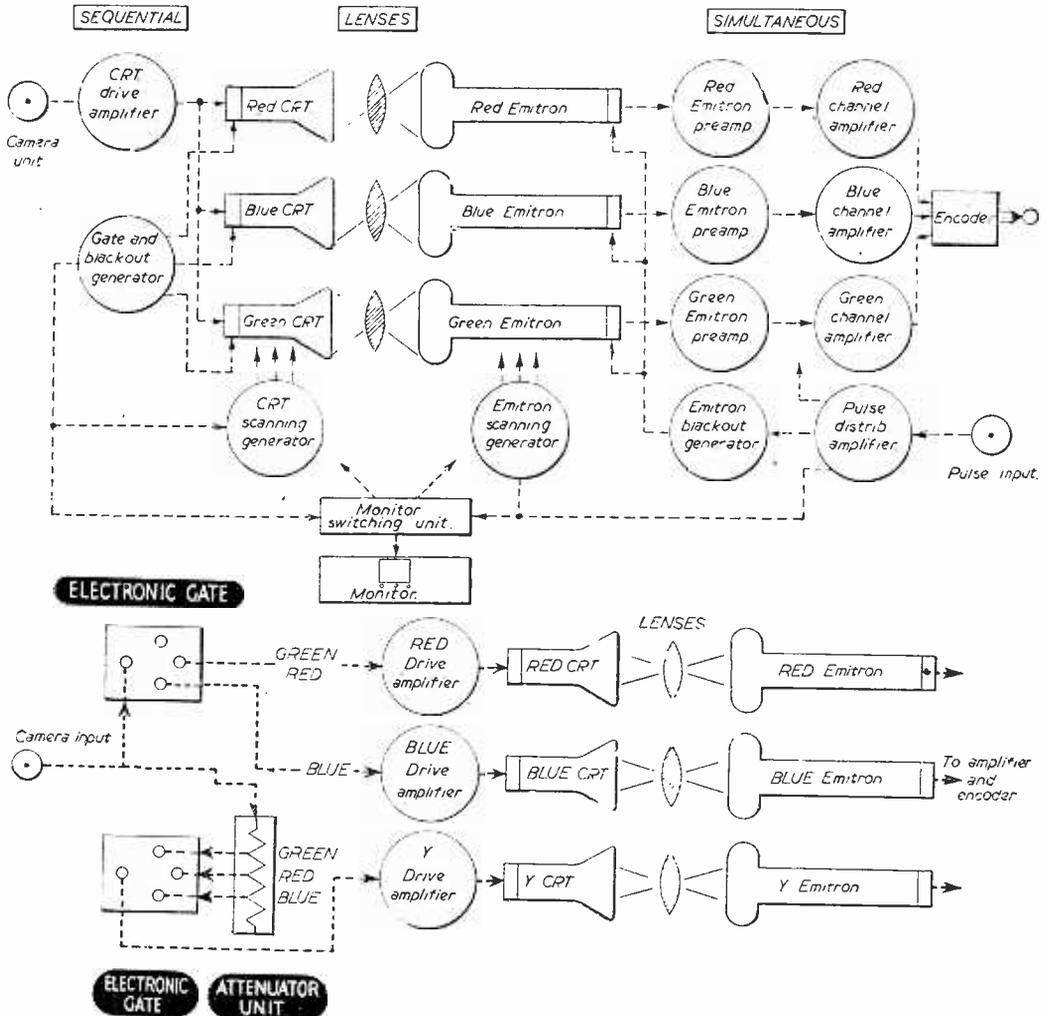
Fig. 35. — Schematic layout of the E.M.I. chromacoder, and below the modified R.Y.B. colour scheme.
