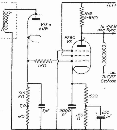
Fig. 3.—Detector and video amplifier circuit.
