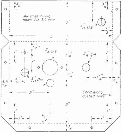
Fig. 2. Chassis bending and drilling details.
