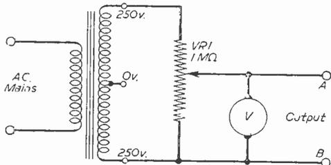
Fig. 17.—Circuit for sensitivity checking.
