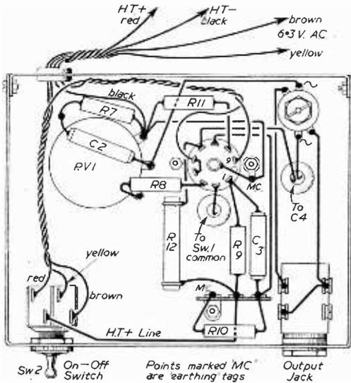
Fig. 4.—Under chassis wiring scheme.
