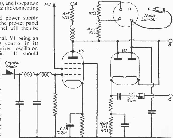
Fig. 2.—Video output, noise limiter and sync clipper.
