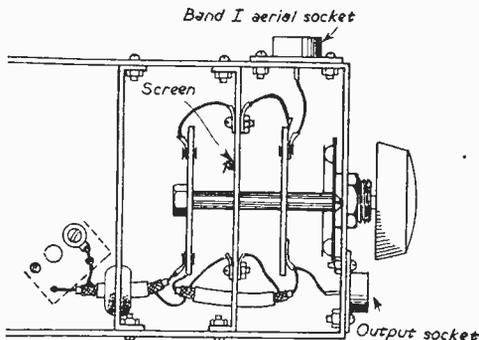
Fig. 3.—Switch installed in converter.
