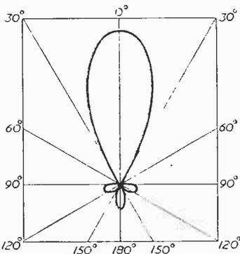
Fig. 1.—Polar diagram of Yagi array.
