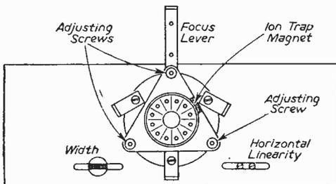
Fig. 3.—Details of the tube mounting bracket.
