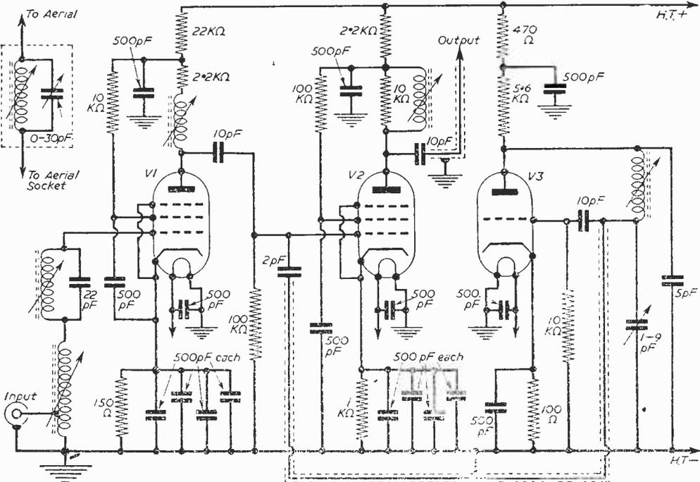
Fig. 2. The oscillator section.
