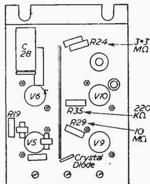
Fig. 4.—The front-end (underside) of the R.F. chassis.
