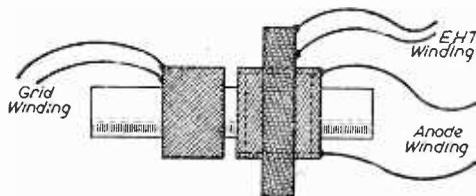
Fig. 2.—Details of the coil unit.
