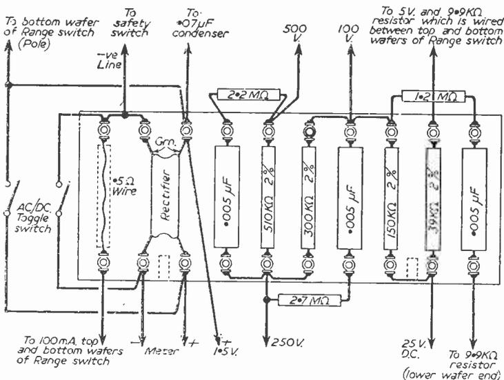
Fig. 3.—Details of the resistor mounting panel.
