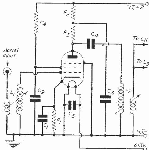
Fig. 2.— Circuit of the first R.F. stage.
