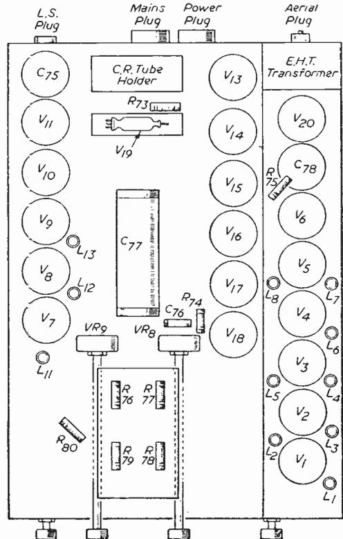
Fig. 1.—Layout of chassis top.
