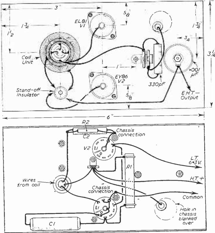
Fig. 4.—Top and bottom wiring details.
