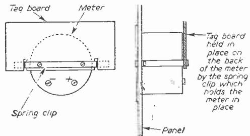
Fig. 5.—How the meter is mounted.
