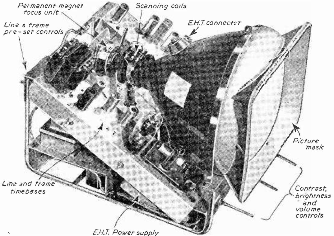
A typical home-constructor receiver, with essential parts marked.
