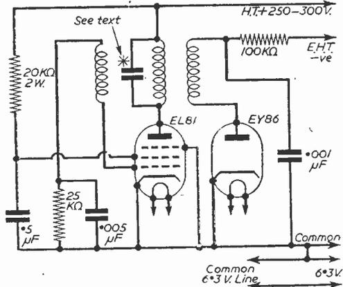
Fig. 4.—Circuit of the unit.
