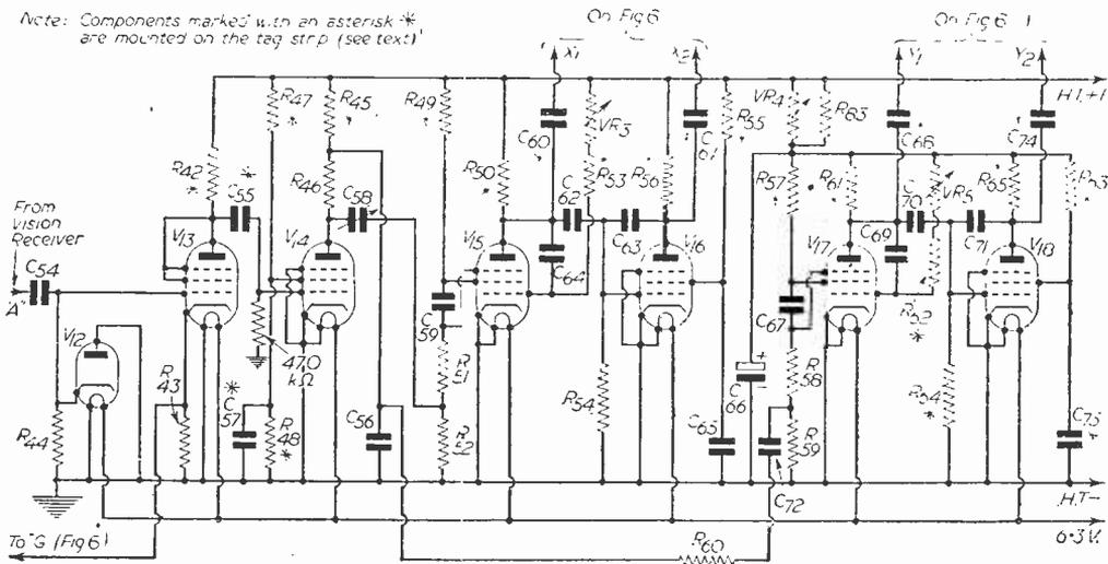
Fig. 4.—The timebase section.
