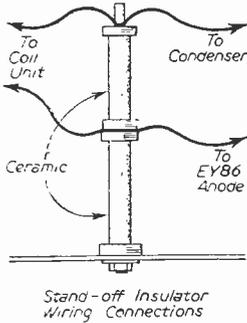
Fig. 5.—Details of the stand-off insulator.
