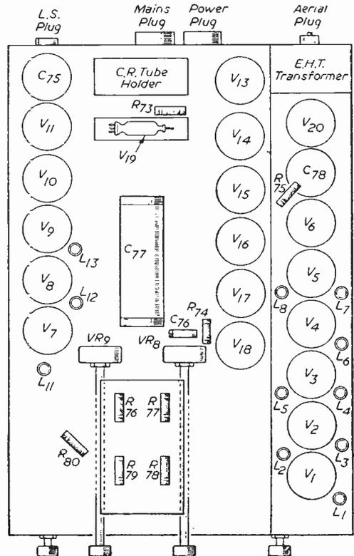
Fig. 1.—Layout of chassis top.
