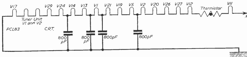
Fig. 1.—The heater wiring for the Pye models dealt with here. (A list of the valves will be found on page 420).
