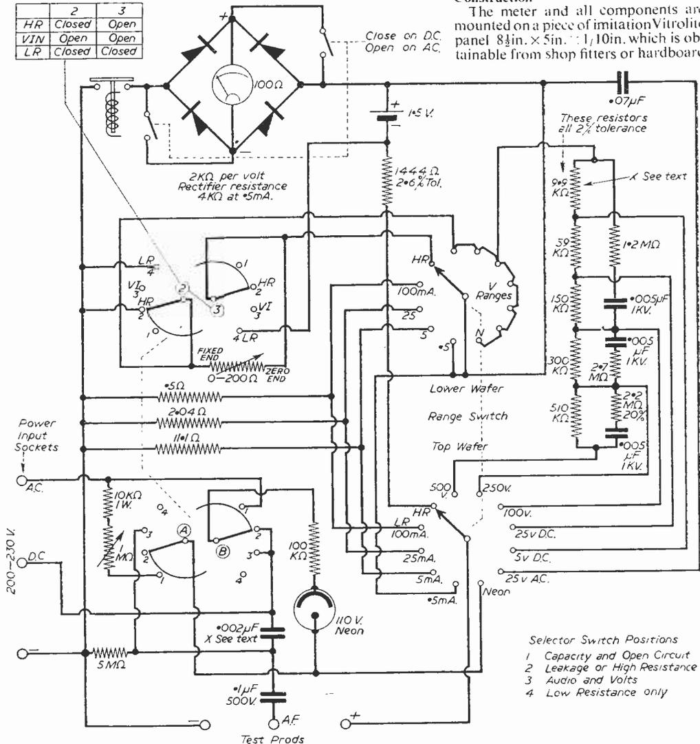
Fig. 1.—Complete wiring diagram of the test meter.
