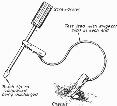
Fig. 7.—A simple method of earthing a charged component.
