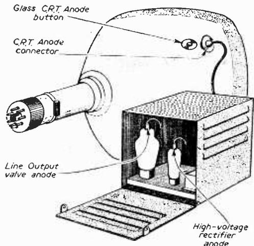
Fig. 8.—Key points to discharge in a high-voltage circuit before servicing.
