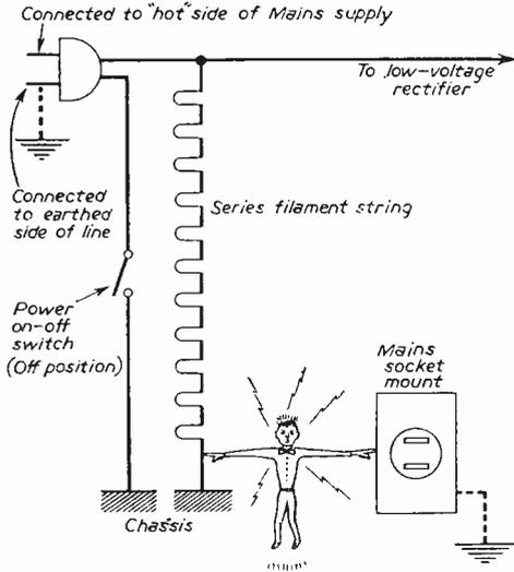
Fig. 3.—Showing how the possibility of shocks exists even with the mains switch "off."
