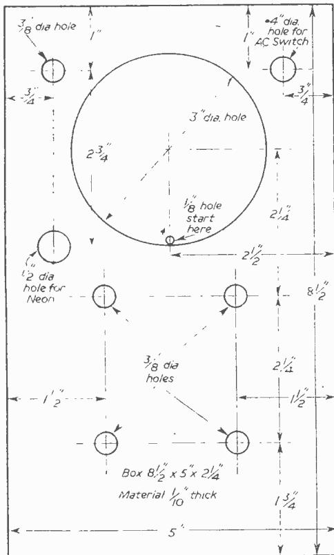
Fig. 6b. Panel drilling details.
