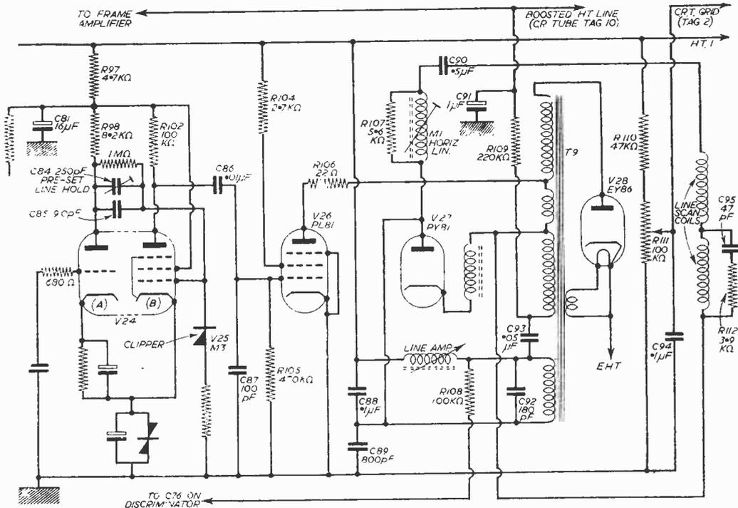
Fig. 3.—The line timebase.
