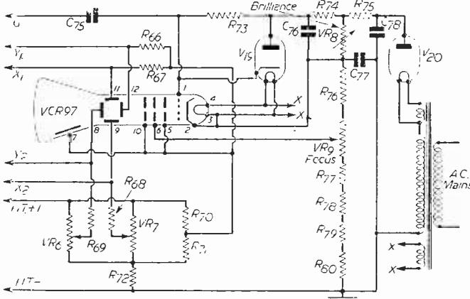
Fig. 6.—Circuit of C.R.T. network.
