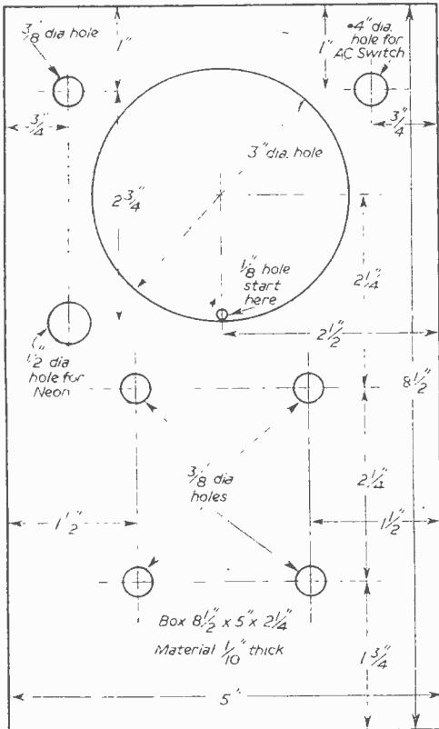
Fig. 6b. Panel drilling details.
