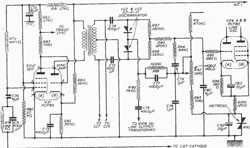
Fig. 2.—Sync separator and line discriminator stage.
