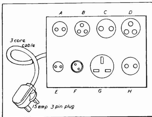
Fig. 2.—Details of a mains distribution board.
