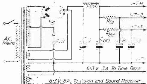
Fig. 7.—Circuit of the power pack.
