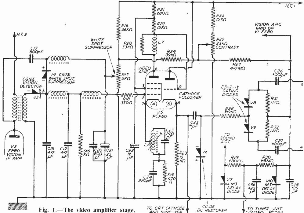
Fig. 1.—The video amplifier stage.
