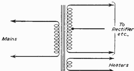
Fig. 1.—The normal A.C. mains input arrangement.
