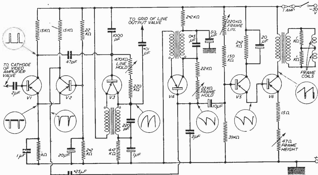
The transistorised timebase unit which was shown by the G.E.C.
