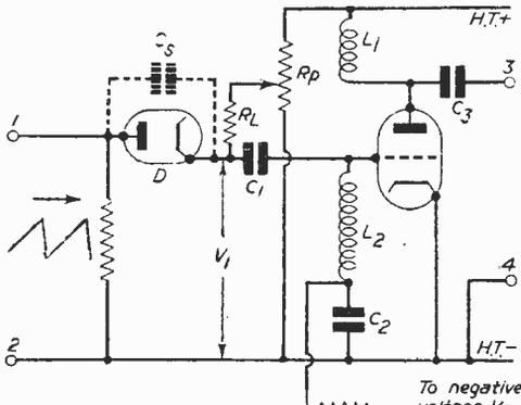
Fig. 1.— Multiar circuit for the production of marker pips.
