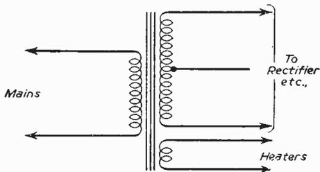
Fig. 1.—The normal A.C. mains input arrangement.
