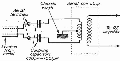
Fig. 9.—A shorted condenser can make an aerial "live" to earth.
