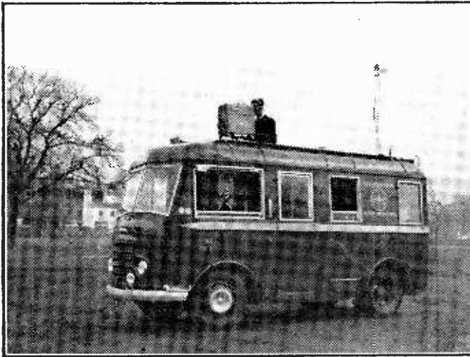
The new O.B. van which has been designed by the BBC Designs and Research Section. The mast at the rear is elevated in use to 45 feet.
