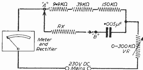
Fig. 9.—Adjusting the current shunts.
