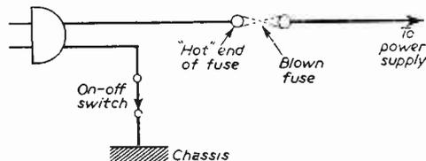
Fig. 5.—Showing how a shock could be received even with a blown fuse.
