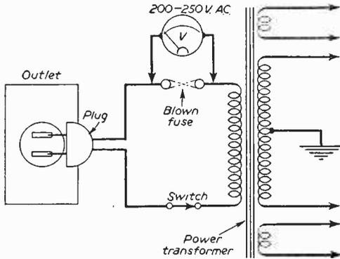
Fig. 6.—The full mains voltage is across the open fuse.
