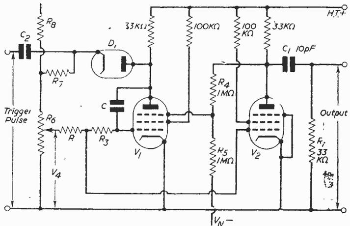
Fig. 2.—The Miller-Sanatron circuit.
