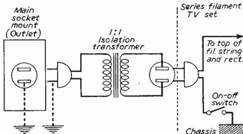
Fig. 4.—A mains transformer removes the chassis from "earth."
