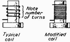
Fig. 2.—Comparison between R.F. and I.F. coils.
