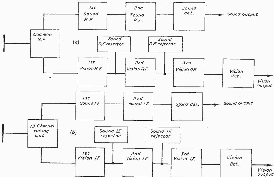
Fig. 1.—The top illustration is a block diagram of a straight receiver, and the lower one of a superhet receiver.
