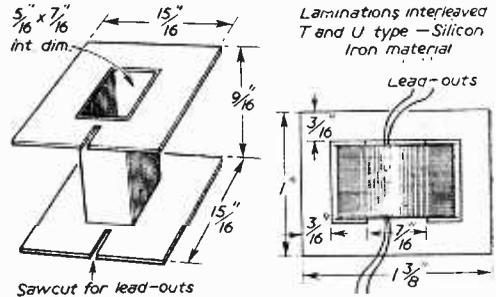
Fig. 15.—Transformer constructional details.
