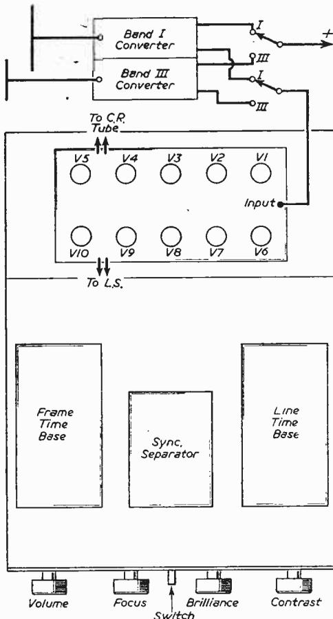
Fig. 3.—A block schematic diagram of the set.
