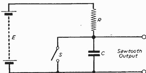
Fig. 8.—Simplified circuit of sawtooth voltage generator.
