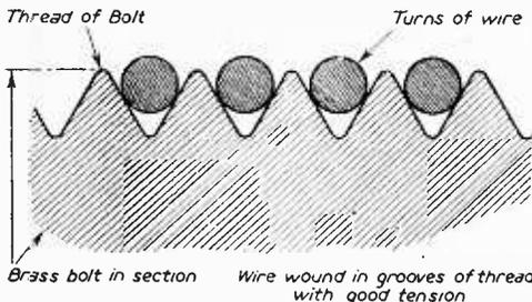
Remove finished coil by holding coil ends and unscrewing bolt from coil
