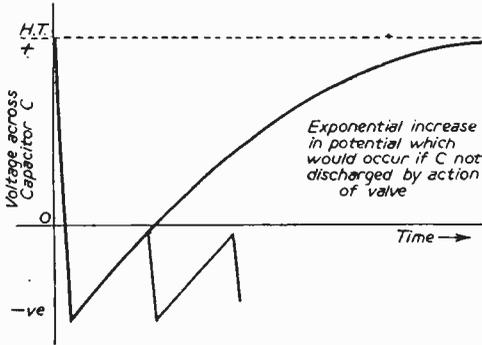
Fig. 13.—Variation in potential across C during the scanning cycle.
