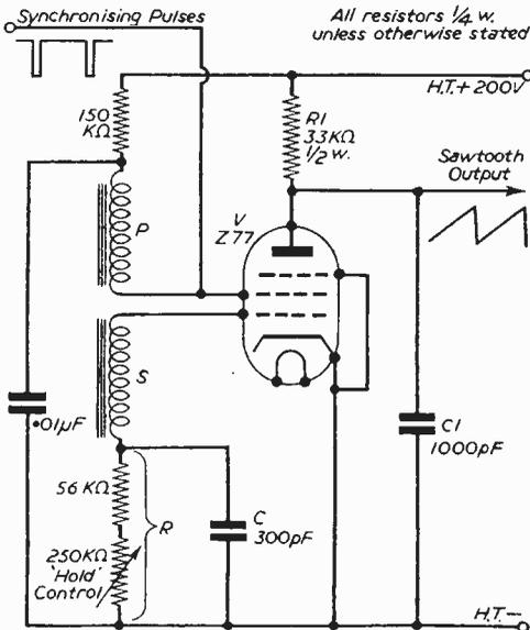
Fig. 14.—Practical line blocking oscillator circuit.
