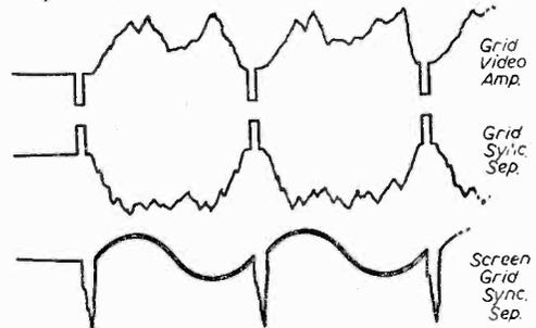
Fig. 5.—Sync waveforms.
