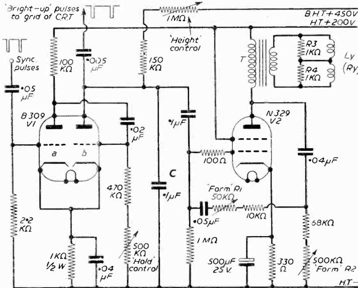
Fig. 23.—Complete scanning circuit for frame deflection of a wide-angle tube. Resistors are 1/2 w. unless stated otherwise.
