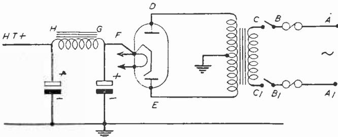
Fig. 1.—Points at which an A.C. power pack may be tested by means of the screwdriver.
