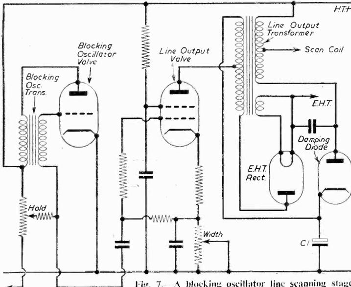
Fig. 7. A blocking oscillator line scanning stage.
