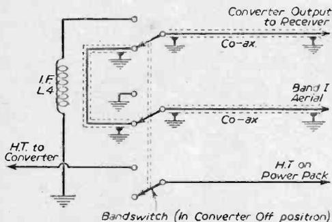
Fig. 3.—Bandswitch circuitry.
