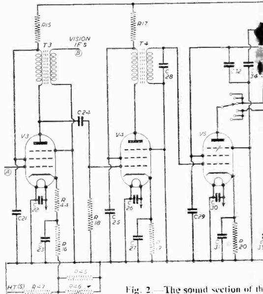
Fig. 2.—The sound section of the receiver.
