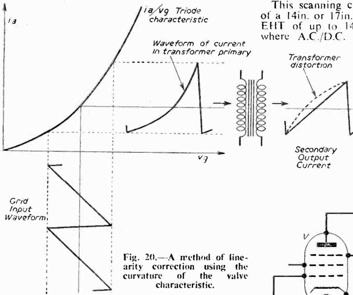
Fig. 20.—A method of linearity correction using the curvature of the valve characteristic.
