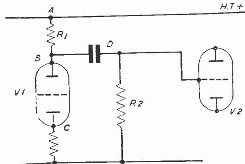
Fig. 2.—Testing at the valveholder in a receiver.
