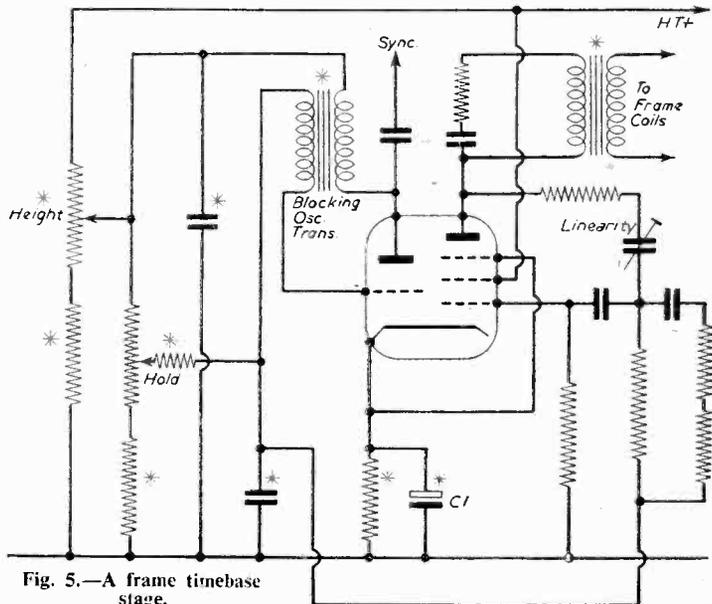
Fig. 5.—A frame timebase stage.
