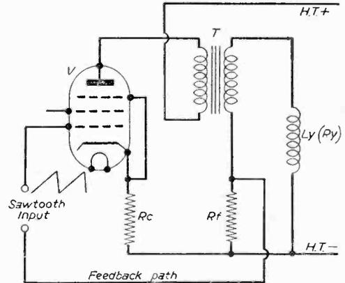
Fig. 22.—Linearisation by the use of negative feedback.
