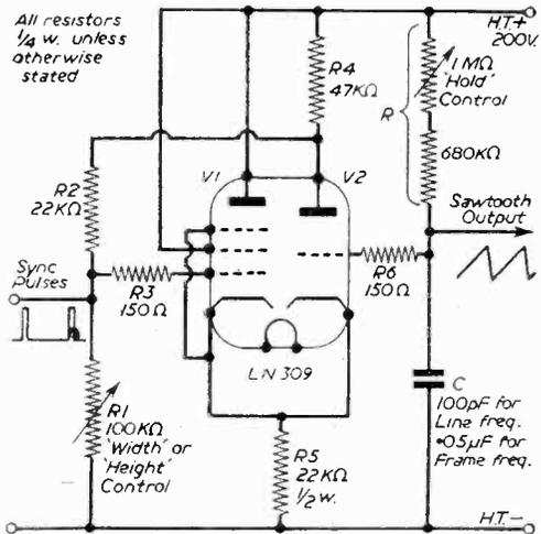
Fig. 16.—Practical multi-vibrator circuit.
