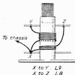
the supplementary coil data for the R.F. 26 converter.
