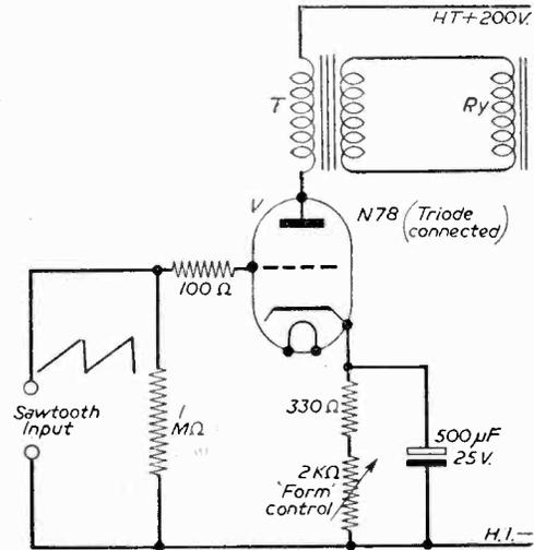
Fig. 21.—Practical circuit of valve curvature linearity correction.
