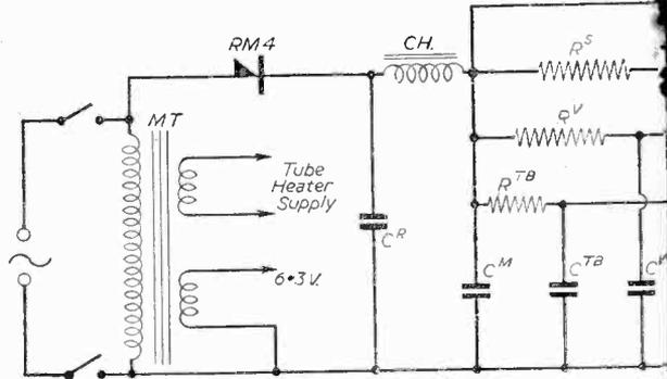
Fig. 4.—The power pack section.
