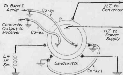
Fig. 2.—Bandswitch wiring details.
