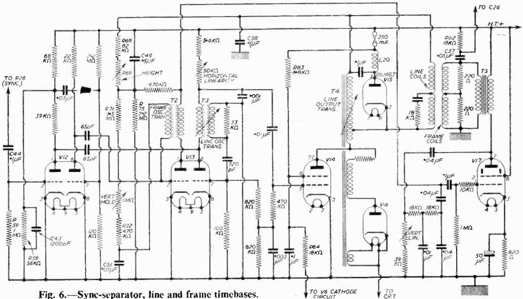
Fig. 6.—Sync-separator, line and frame timebases.
