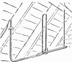
This is a 1 wavelength, 3 element array. Of all alloy construction the aerial is completely assembled and ready for instant mounting in loft, bedroom cupboard, window frame, etc. Price 12/6 plus 2/- post and insurance.
