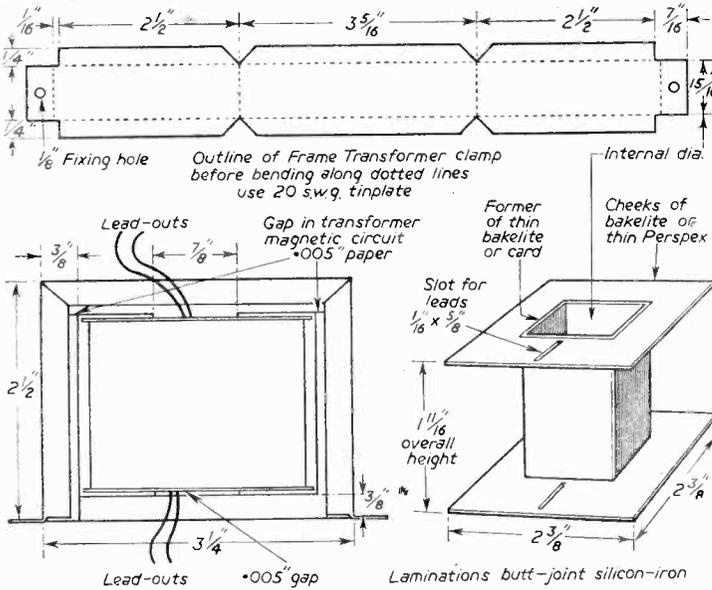
Fig. 24.—Practical details for the construction of a frame transformer.
