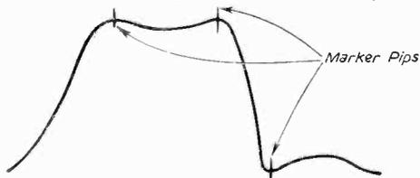
Fig. 1.—A typical I.F. response curve.
