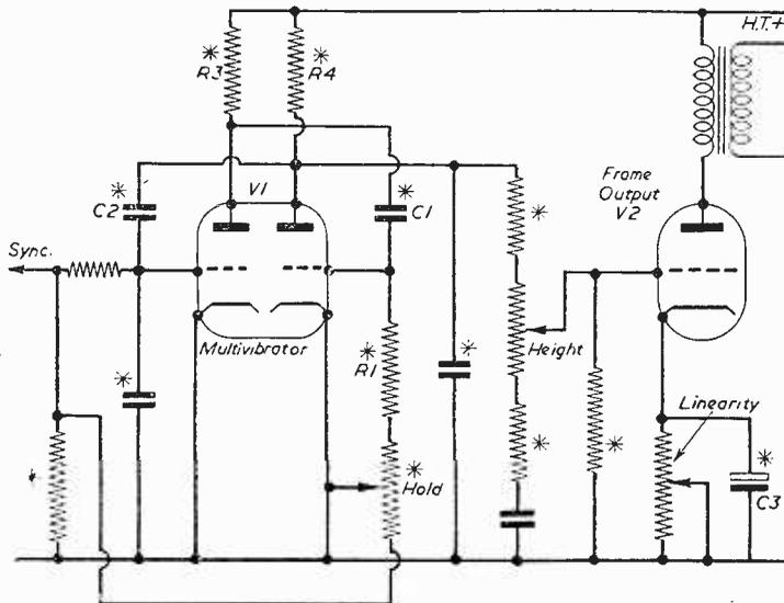
Fig. 3.—Multivibrator using double triode with frame output valve.
