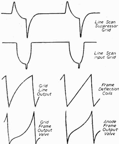
Fig. 4.—Some typical waveforms from the timebases.
